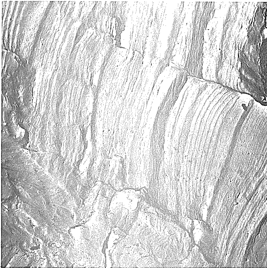
FIG. 17 TWO EXAMPLES OF FATIGUE STRIATIONS AS OBSERVED BY THE ELECTRON MICROSCOPE.
