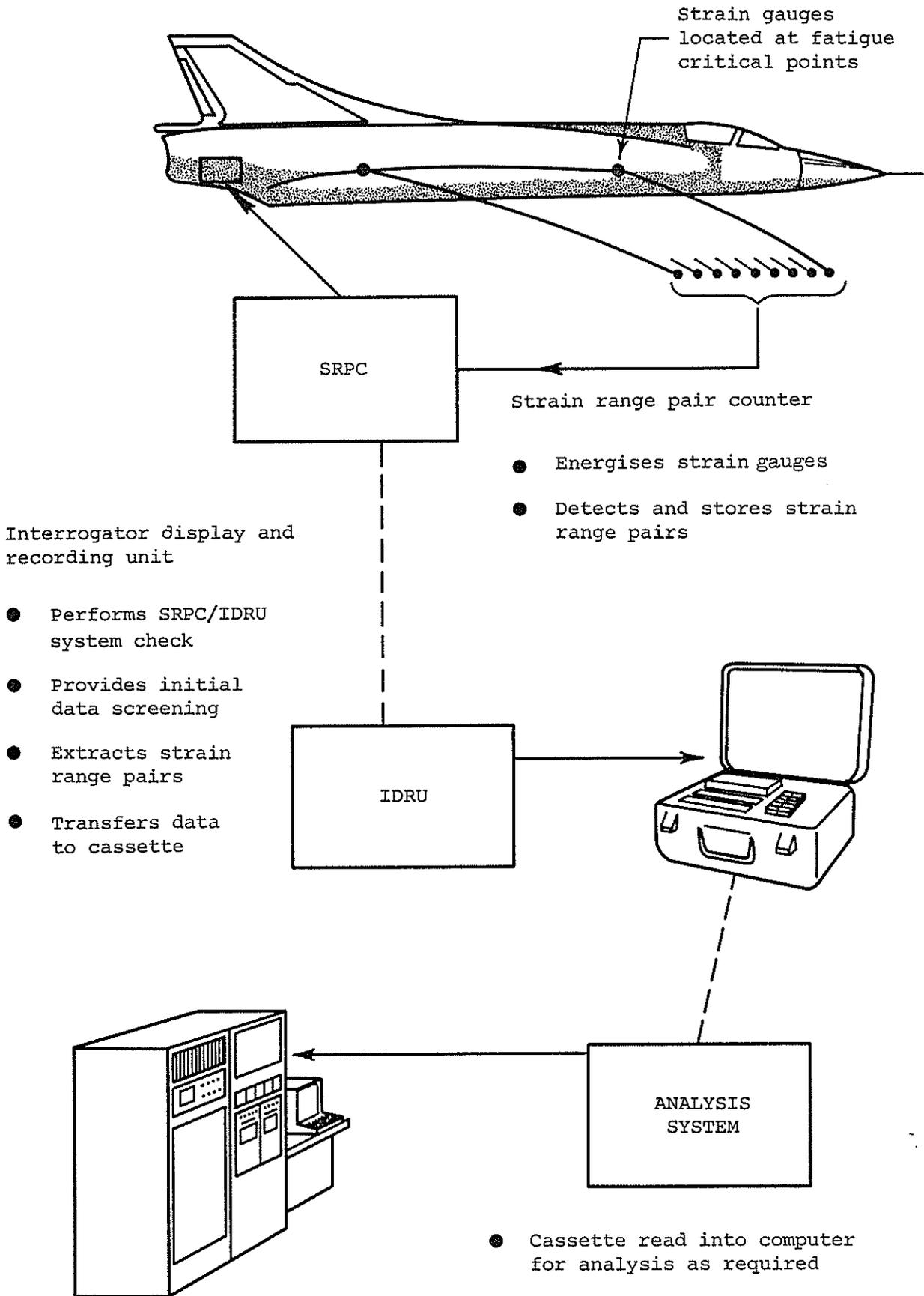
FIG. 17 THE AIRCRAFT FATIGUE DATA ANALYSIS SYSTEM (AFDAS)
