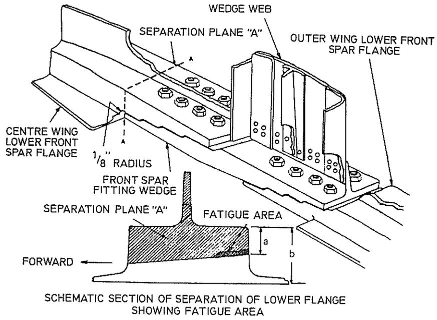
FIG. 7 MARTIN 2-0-2 WING ROOT FITTING FATIGUE FAILURE (Ref. 98)
