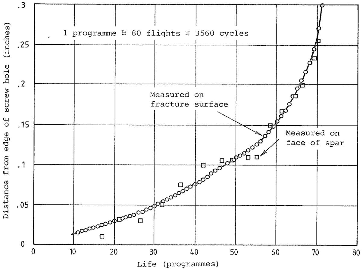
FIG. 13(b) CRACK LENGTH VERSUS LIFE, "VAMPIRE" SPAR (Ref.188)
