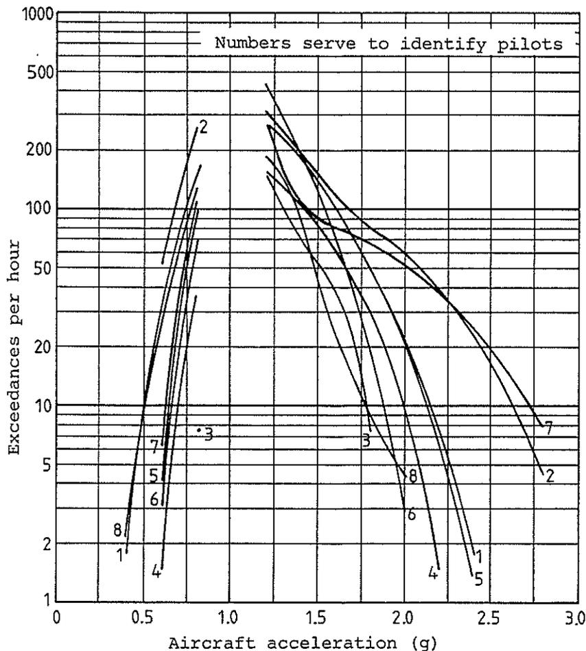
FIG. 16 VARIABILITY IN LOAD HISTORY CAUSED BY DIFFERENT PILOTS
