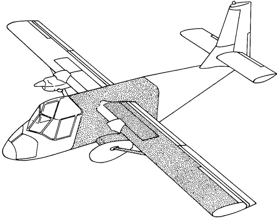
FIG. 21 GAF "NOMAD N22" (Shaded area shows extent of structural fatigue test article)
