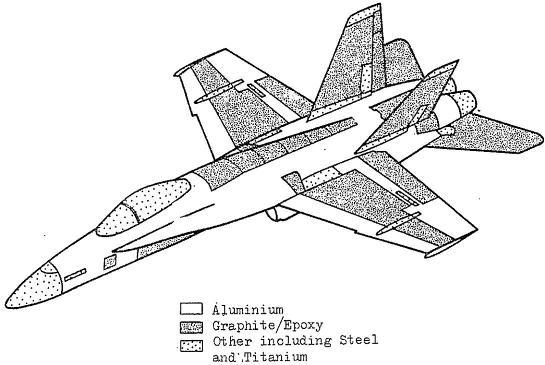
FIG. 23 F/A-18, INDICATING APPLICATIONS OF GRAPHITE/EPOXY COMPOSITES
