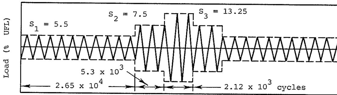
(a) Program block 3-load-level test (vibration rig)
