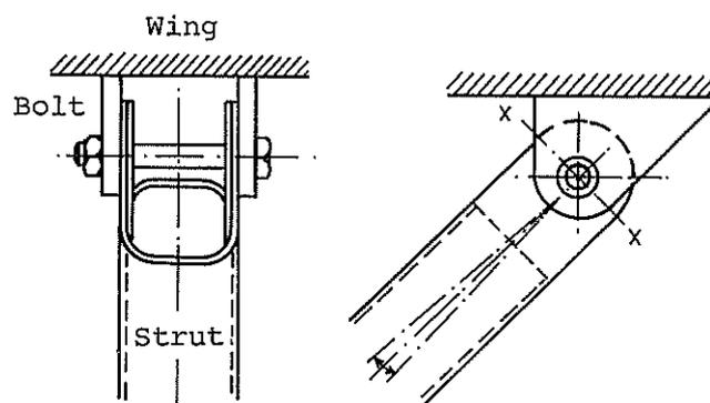
FIG. 3 (b) DORNIER "MERKUR" WING/STRUT ATTACHMENT (Ref. 28 )
