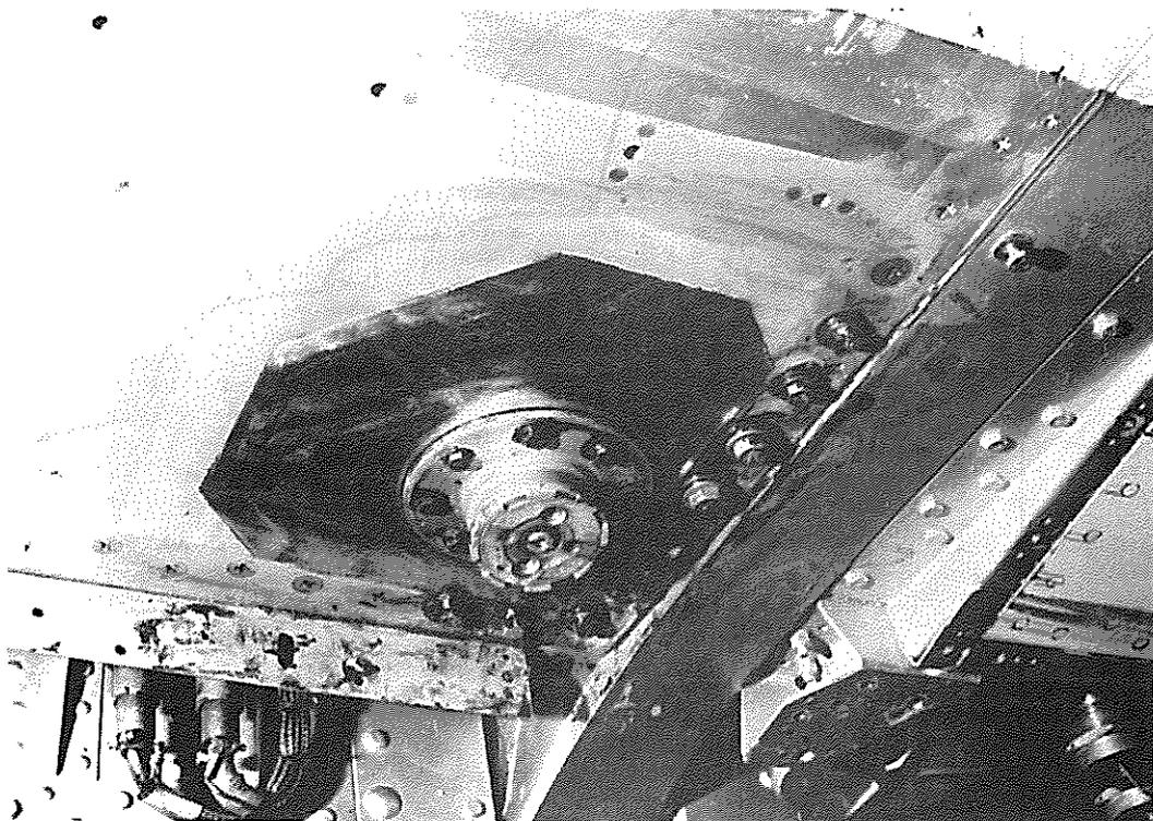
FIG. 20 BFRP PATCH FOR MIRAGE DECANT HOLE FATIGUE CRACKING
