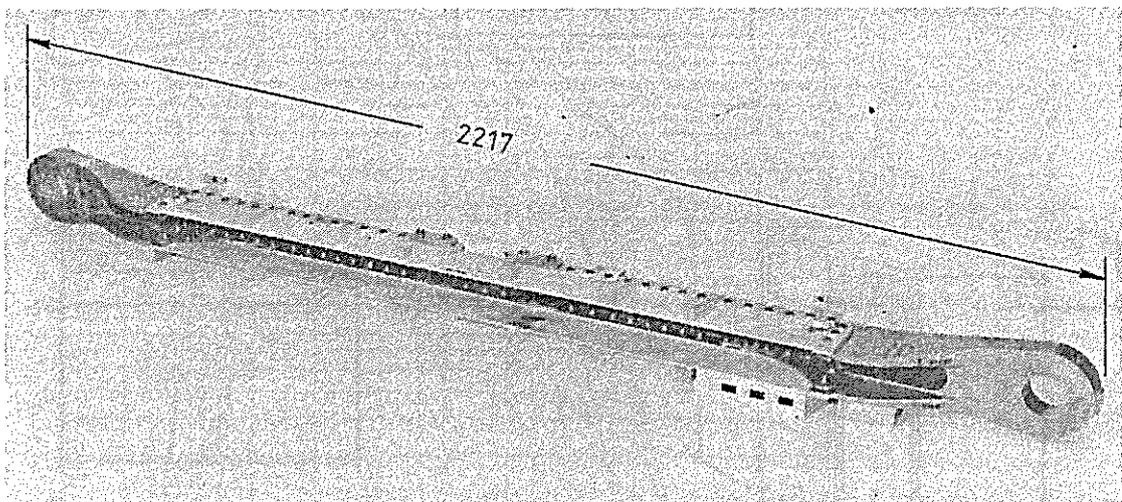
FIG. 19 (b) D6AC STEEL "HUMPHRIES" SPECIMEN
