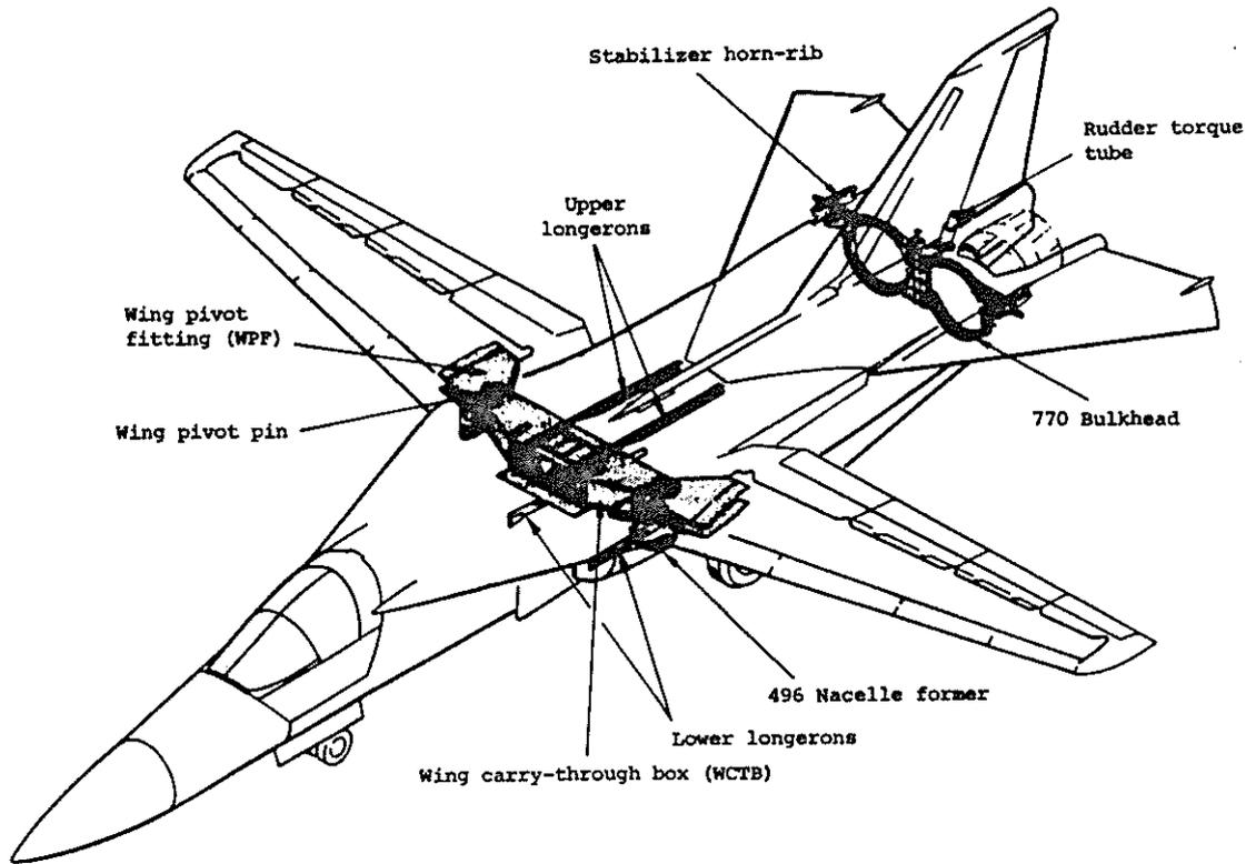
FIG. 19 (a) D6AC STEEL STRUCTURAL MEMBERS IN F-111
