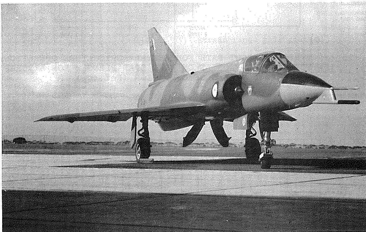
FIG. 14 RAAF MIRAGE AIRCRAFT A3-76 SHOWING ARL DESIGNED GUST PROBE
