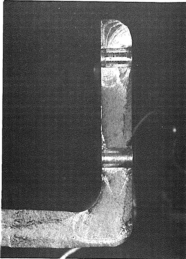
FIG. 8 FATIGUE FAILURE IN SPAR BOOM OF "DOVE" VH-AQO
