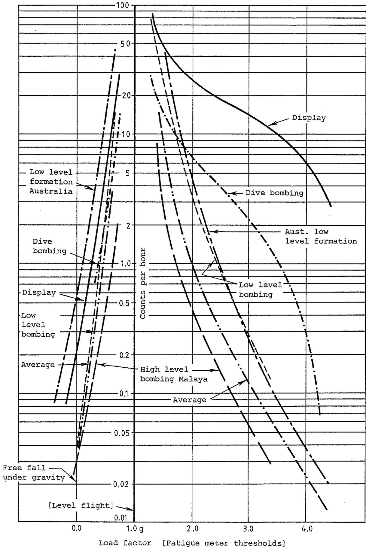
FIG. 12 LOAD-FREQUENCY CURVES FOR R.A.A.F. CANBERRA AIRCRAFT (Ref. 170)
