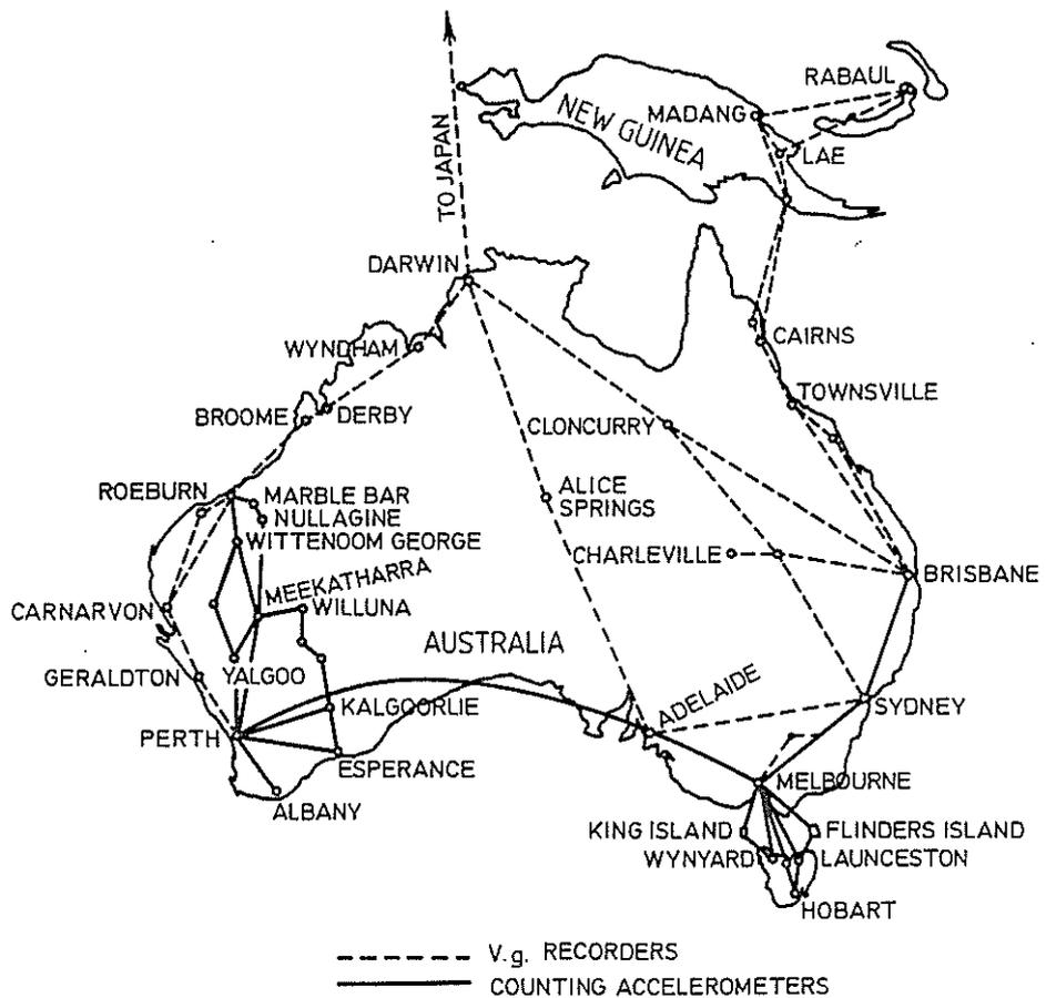
FIG. 10 FLIGHT LOADS MEASUREMENTS, AUSTRALIAN ROUTES-EARLY 1950's (Ref.133)
