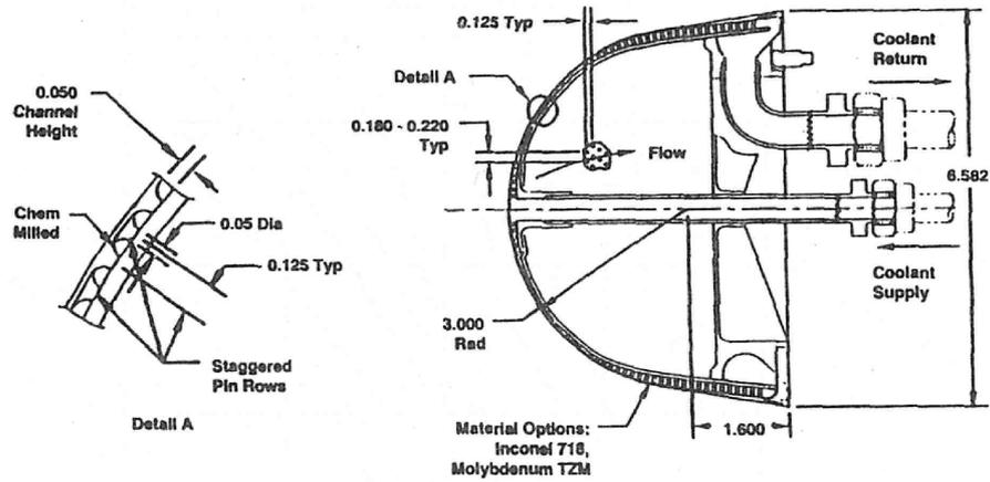
Figure 18 Actively Cooled Nose Tip
