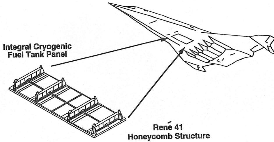
Figure 20 Boeing Hot Structure
