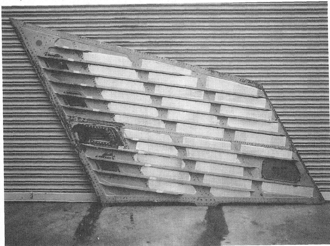
Figure 7 Constrained Layer Damping Treatment
