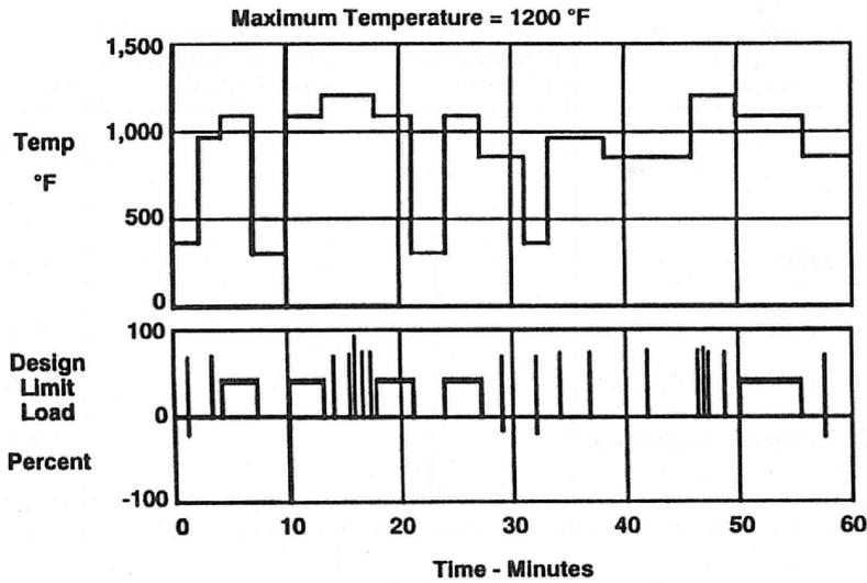
Figure 12 Aerospace Vehicle Profile
