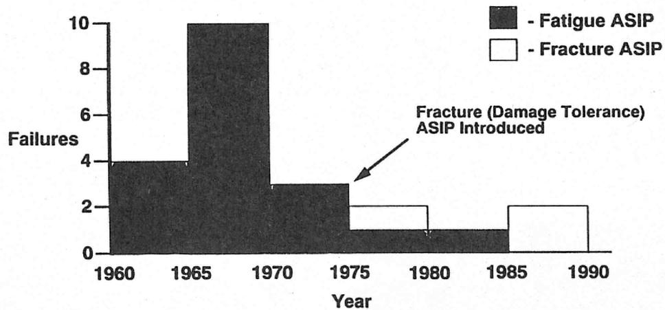
Figure 2 Aircraft Structural Failures
