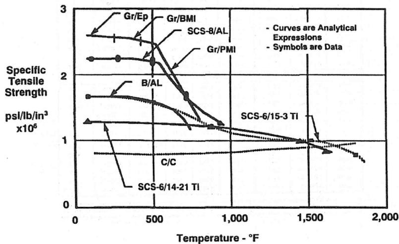
Figure 15 Structural Efficiency of Materials
