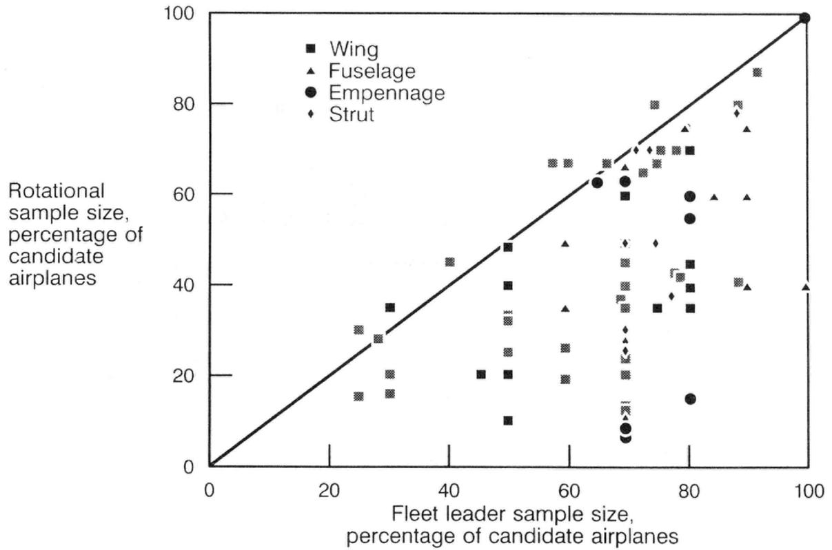
Figure 40. Fleet Sampling Efficiency Comparisons
