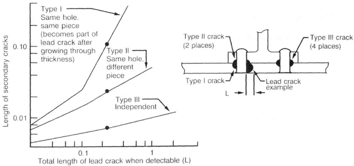
Figure 11. Multiple Site Damage (MSD) Size Analysis Guidelines
