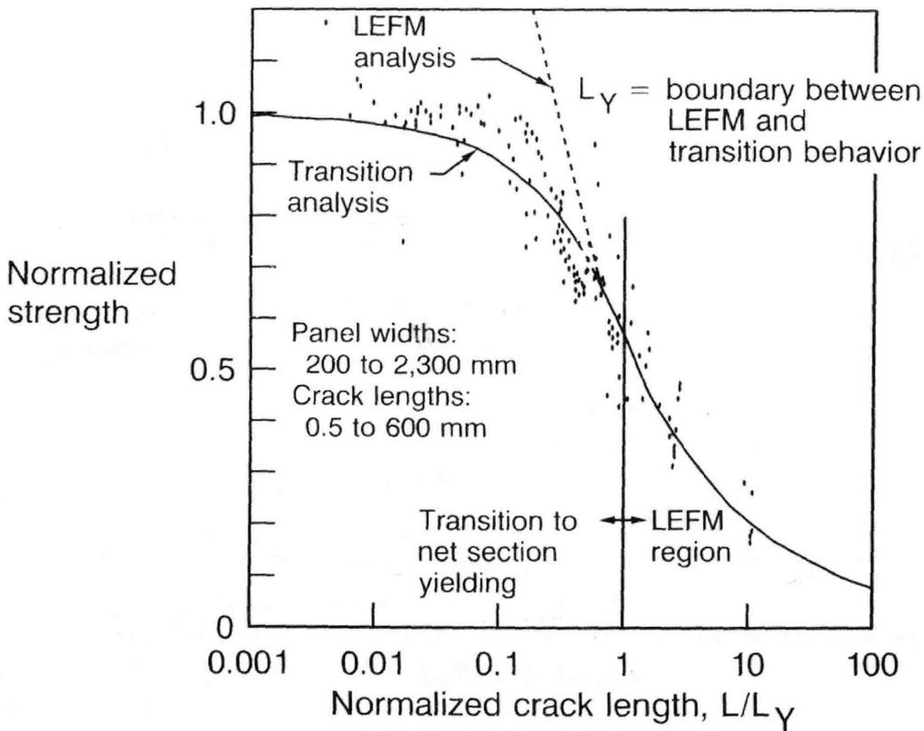
Figure 6. Residual Strength Test Verification Examples
