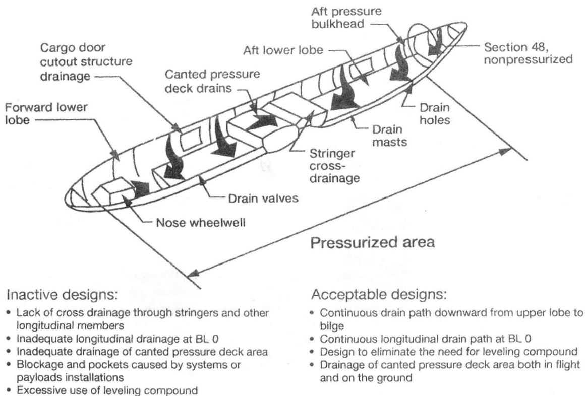
Figure 76. Lower Lobe Drainage Examples in Corrosion Prevention Design Handbook
