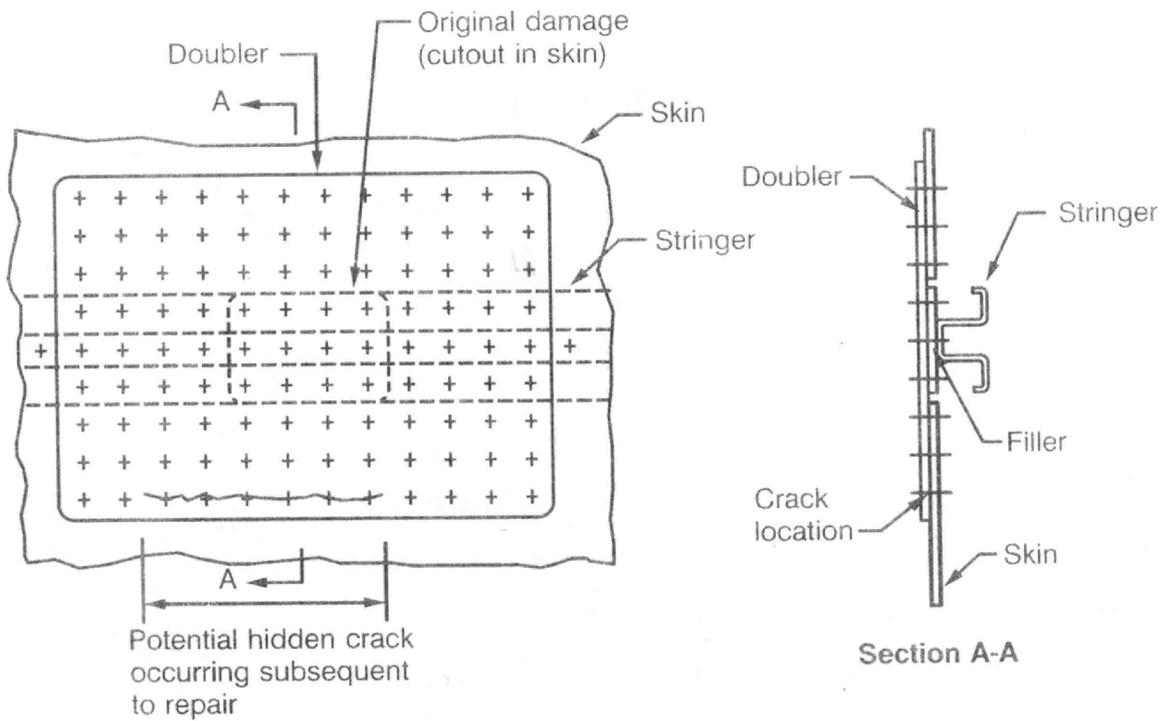
Figure 94. Typical Fuselage External Skin Repair
