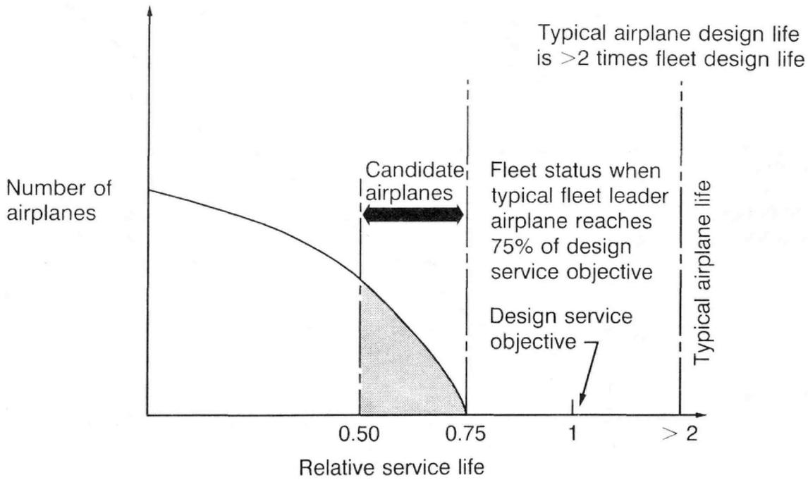
Figure 38. Supplemental Inspection Candidate Airplane Criteria
