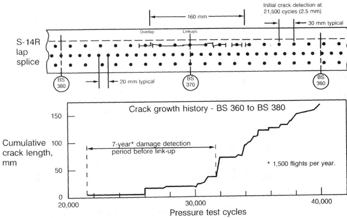
Figure 18. 747-100SR Fuselage Lap Splice Test Results—Stringer 14R
