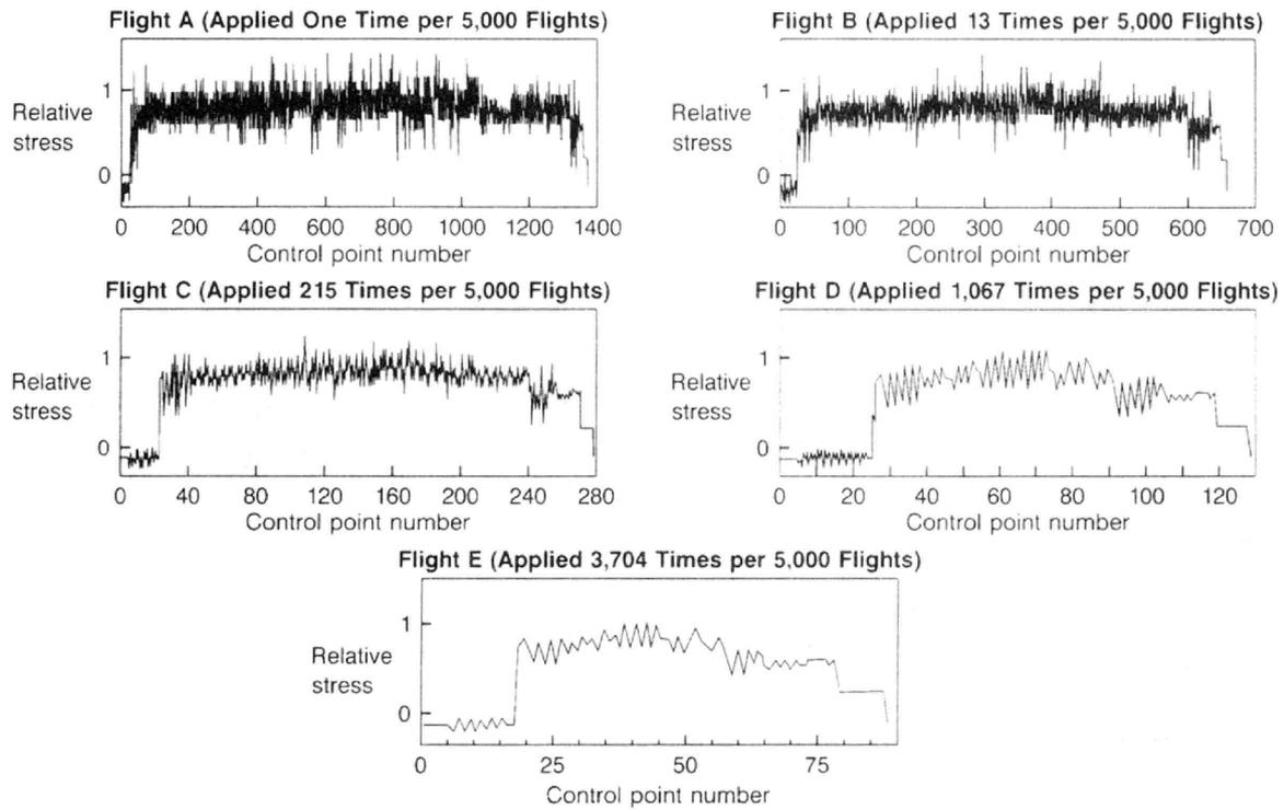
Figure 13. Wing Lower Surface Spectrum Example
