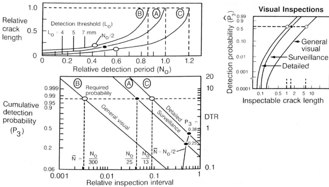
Figure 50. Cumulative Detection Probability—Inspection Type/Detection Threshold Variation
