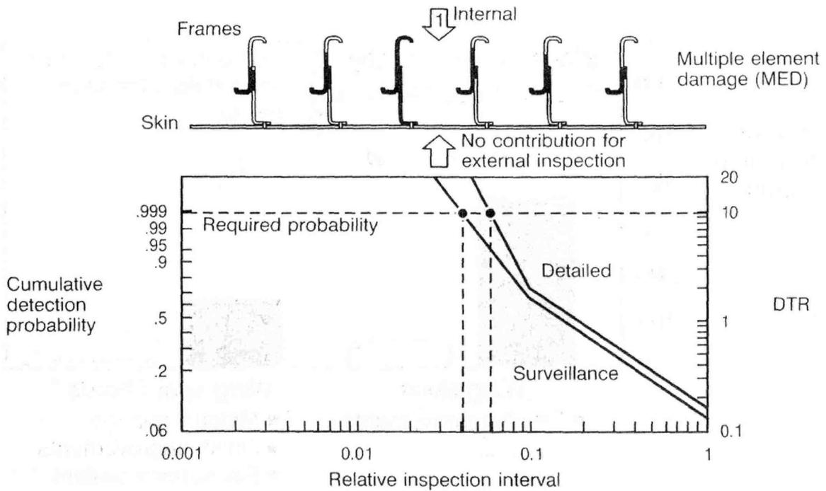
Figure 80. Example of SSID Inspections of Failed Internal Frames
