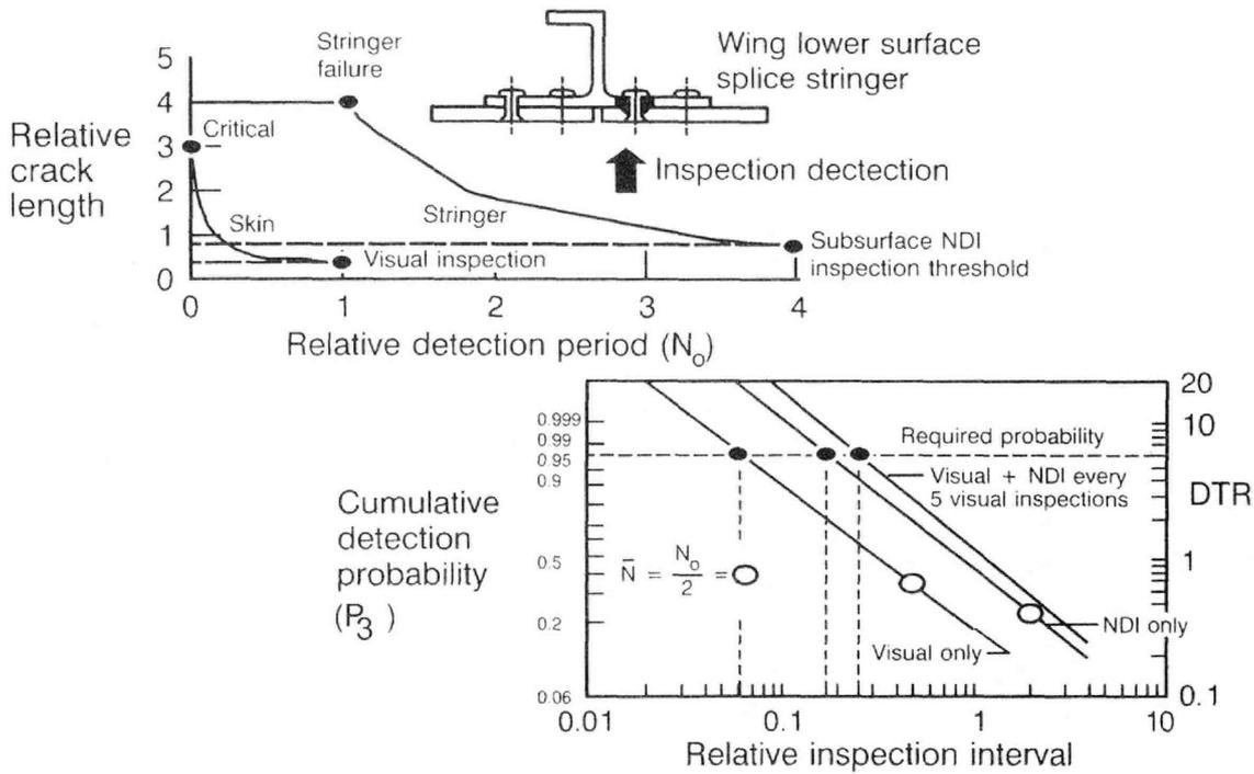
Figure 53. Cumulative Detection Probability—Inspection Method Variation
