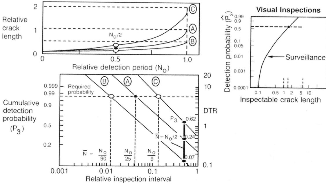
Figure 49. Cumulative Detection Probability—Critical Crack Length Variation
