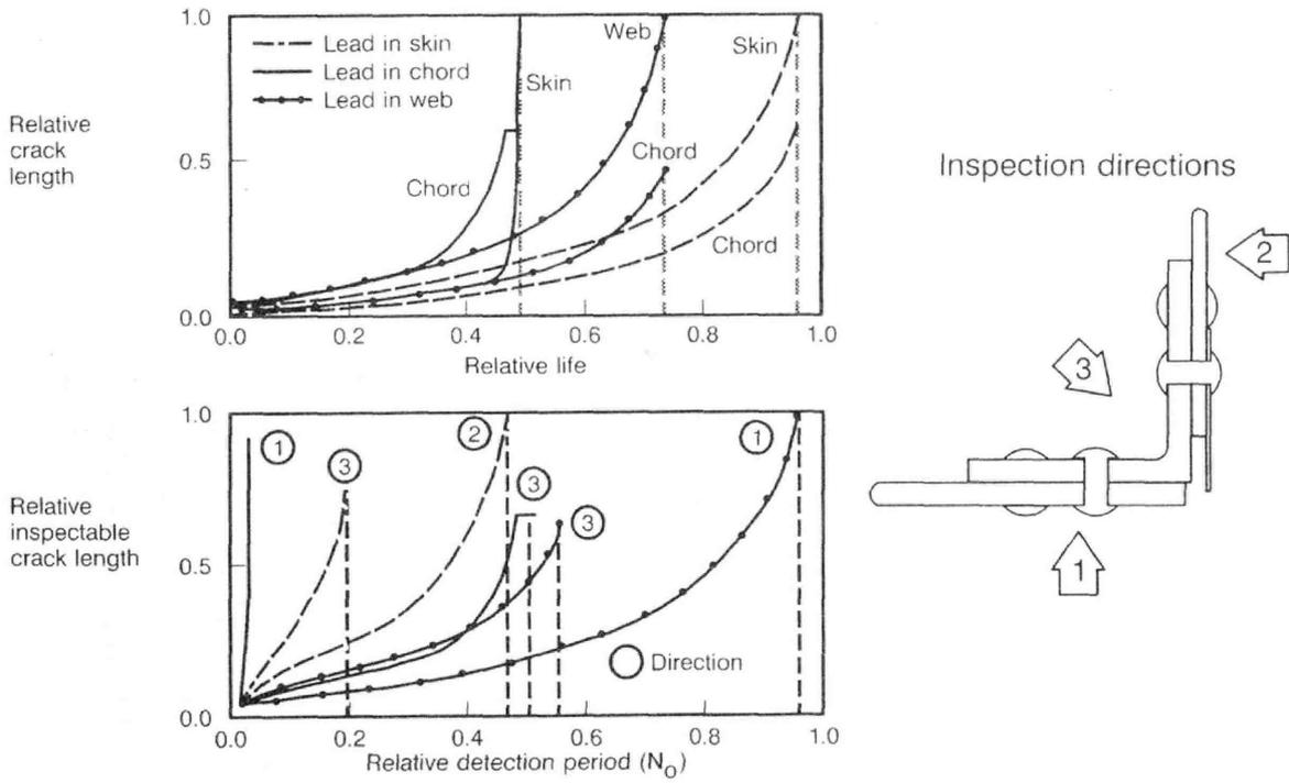
Figure 55. Spar Chord Crack Growth Curve Examples—Wing Center Section
