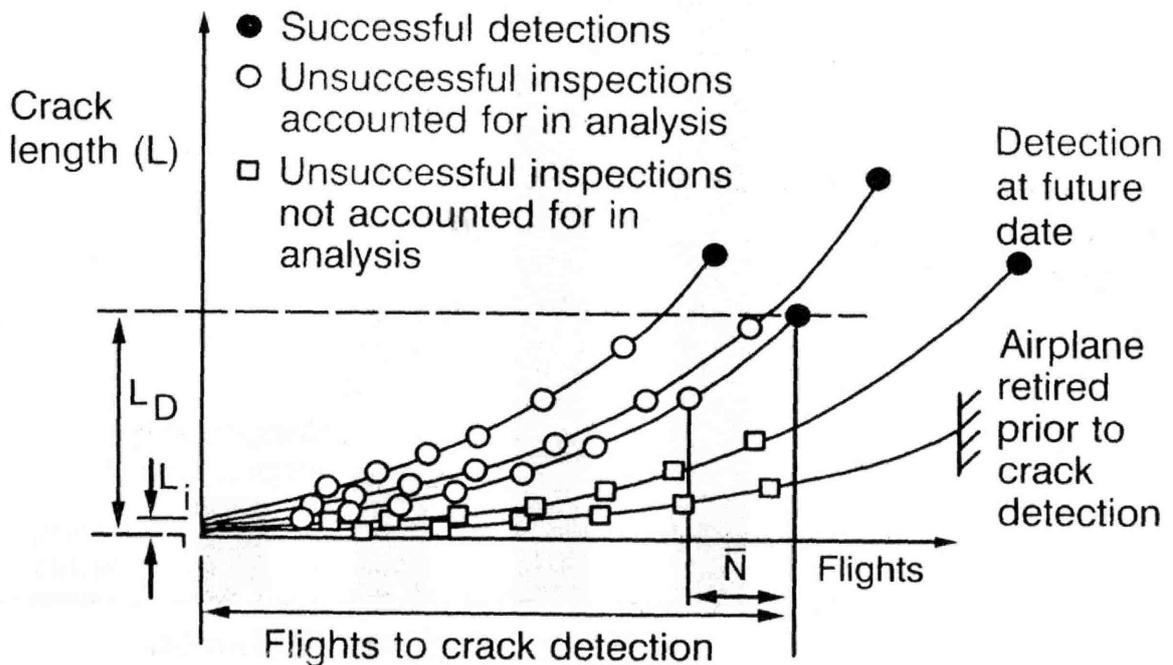
Figure 29. Detection and Non-Detection Events
