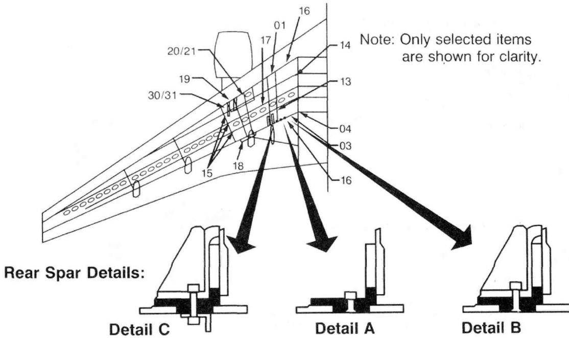
Figure 45. Structurally Significant Item Examples for Wingbox
