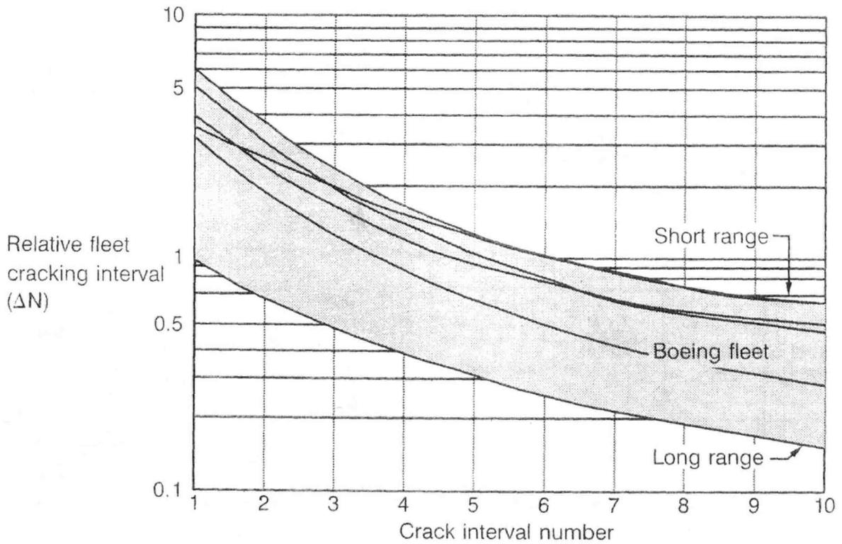
Figure 60. Fleet Cracking Variation— $\Delta N$
