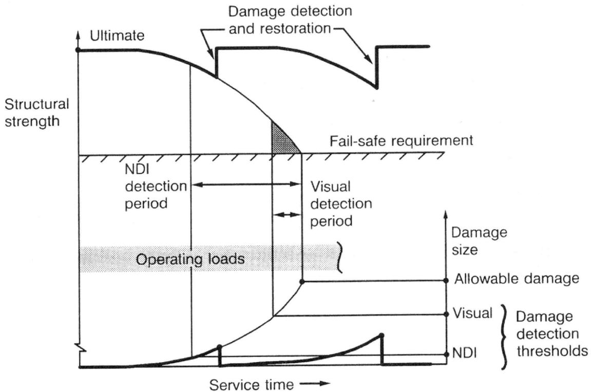
Figure 1. Strength Requirements for Damage Tolerant Structure
