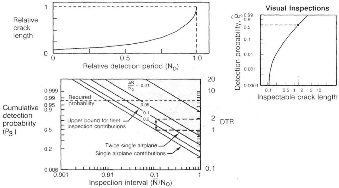
Figure 63. Cumulative Detection Probability—Fleet Inspection Detection Contributions
