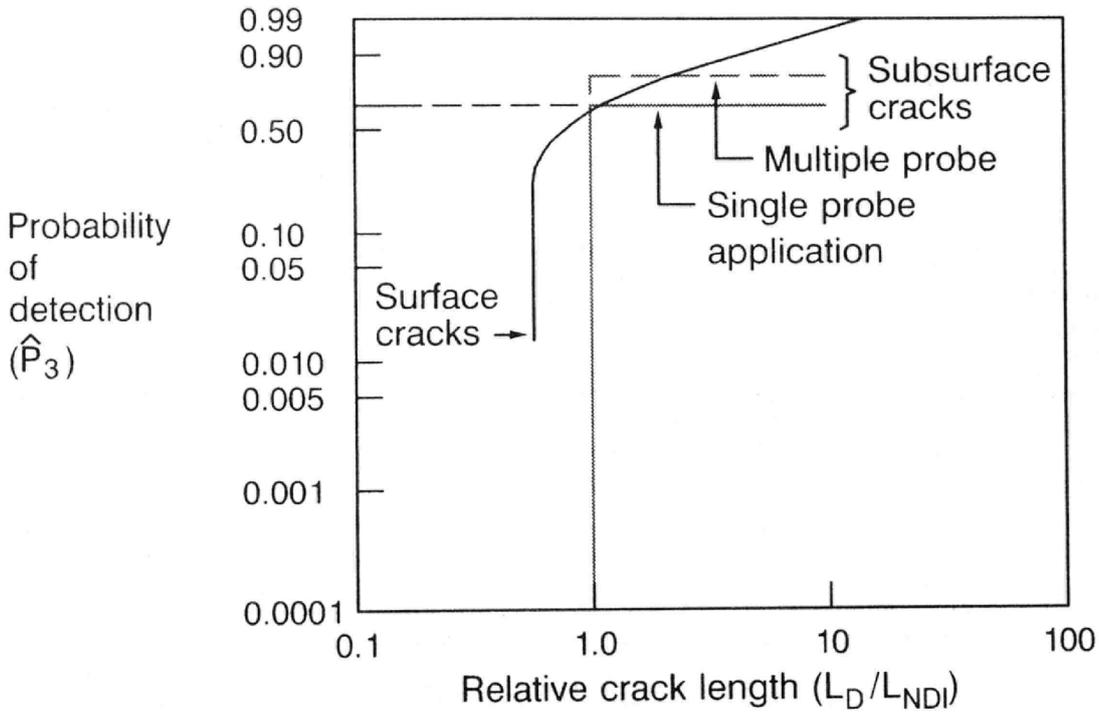
Figure 22. Probability of Detection for NDI Inspections
