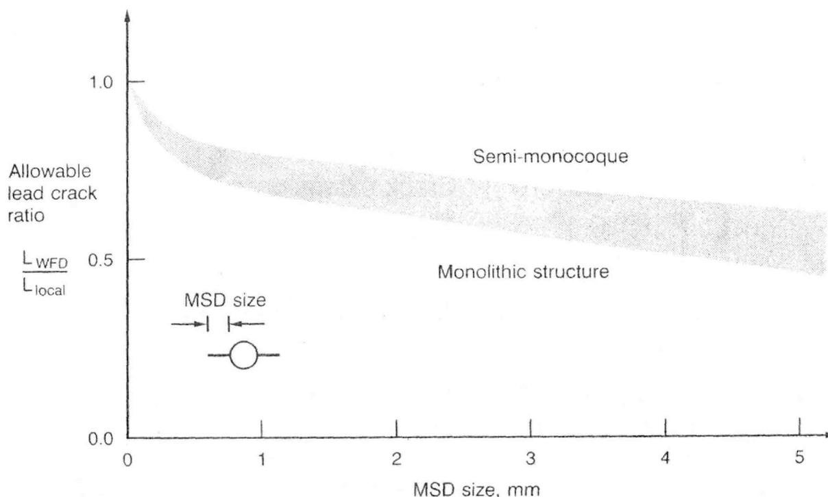
Figure 82. MSD Influence on Allowable Lead Crack Size
