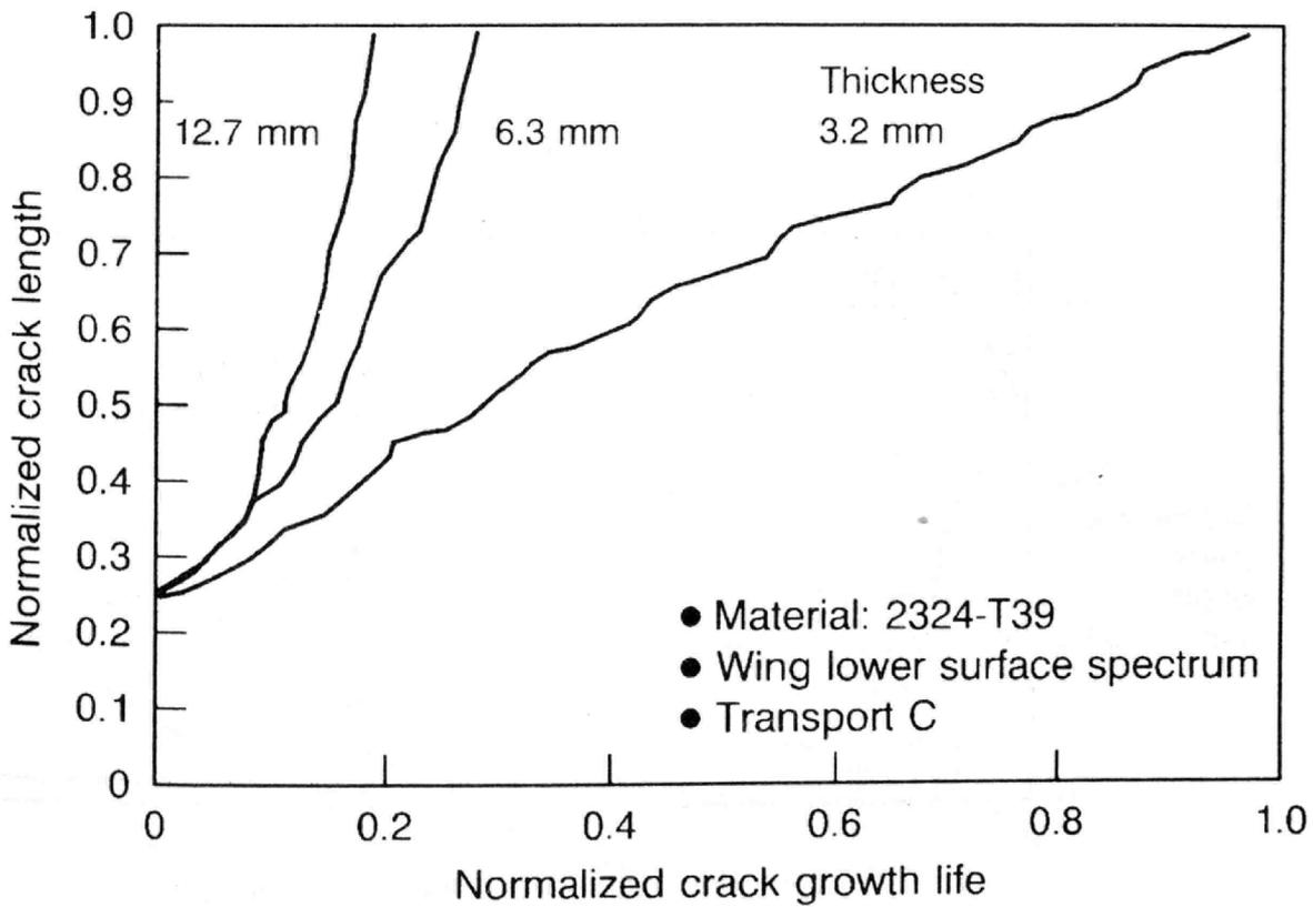
Figure 15. Thickness Effect on 2324 Aluminum Crack Growth
