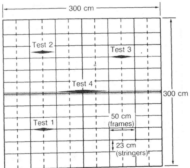
Figure 8. Typical Fuselage Pressure Test Panel
