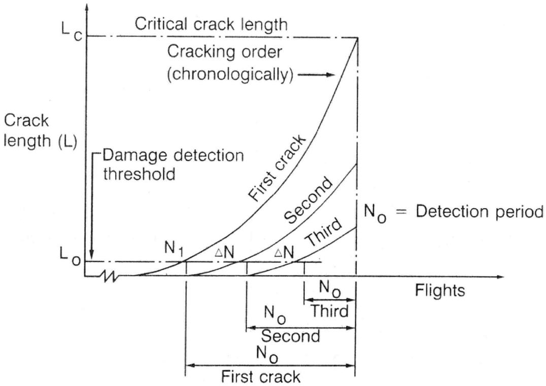
Figure 61. Multiple Cracking in the Fleet
