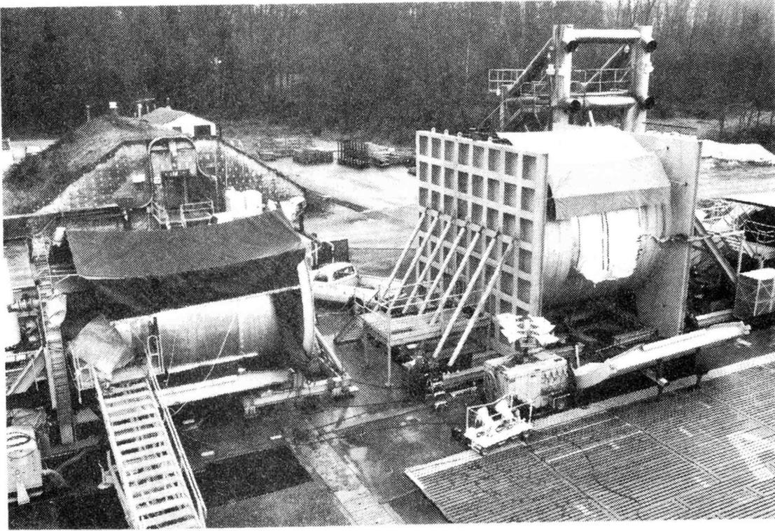
Figure 7. Fuselage Pressure Test Fixtures
