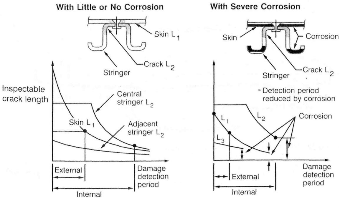
Figure 70. Corrosion Effects on Fatigue Damage Growth
