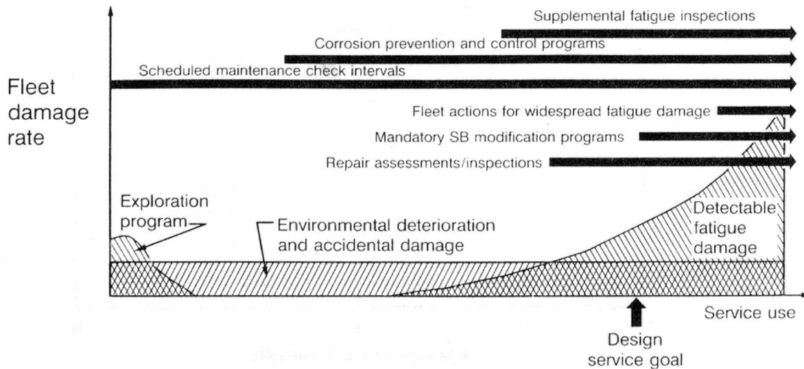
Figure 33. Fleet Damage and Maintenance Program Phases
