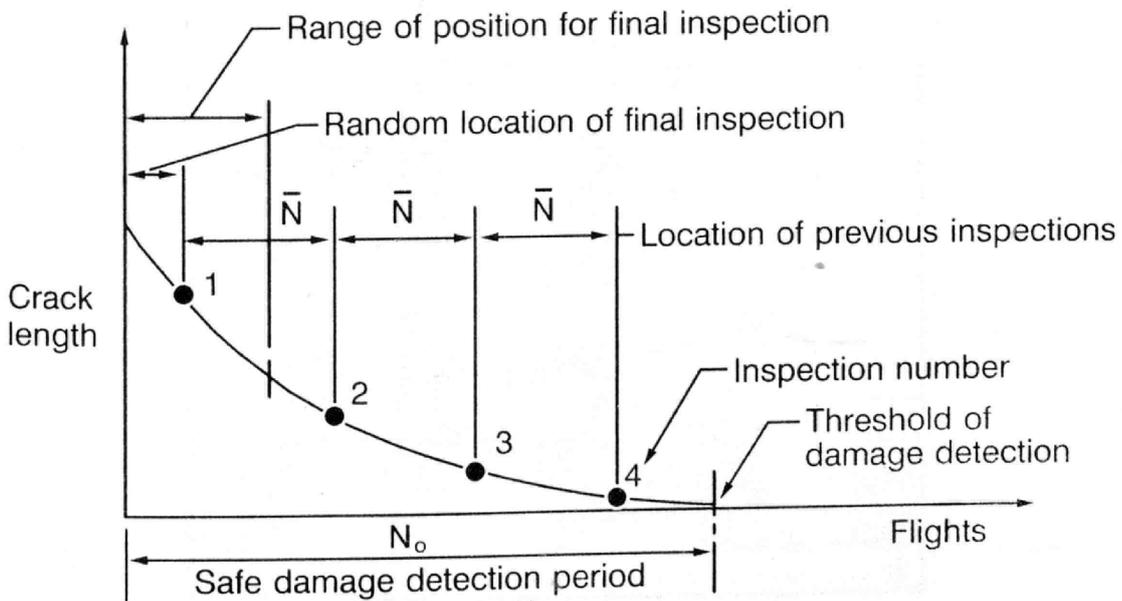
Figure 23. Multiple Inspection Detection Consideration
