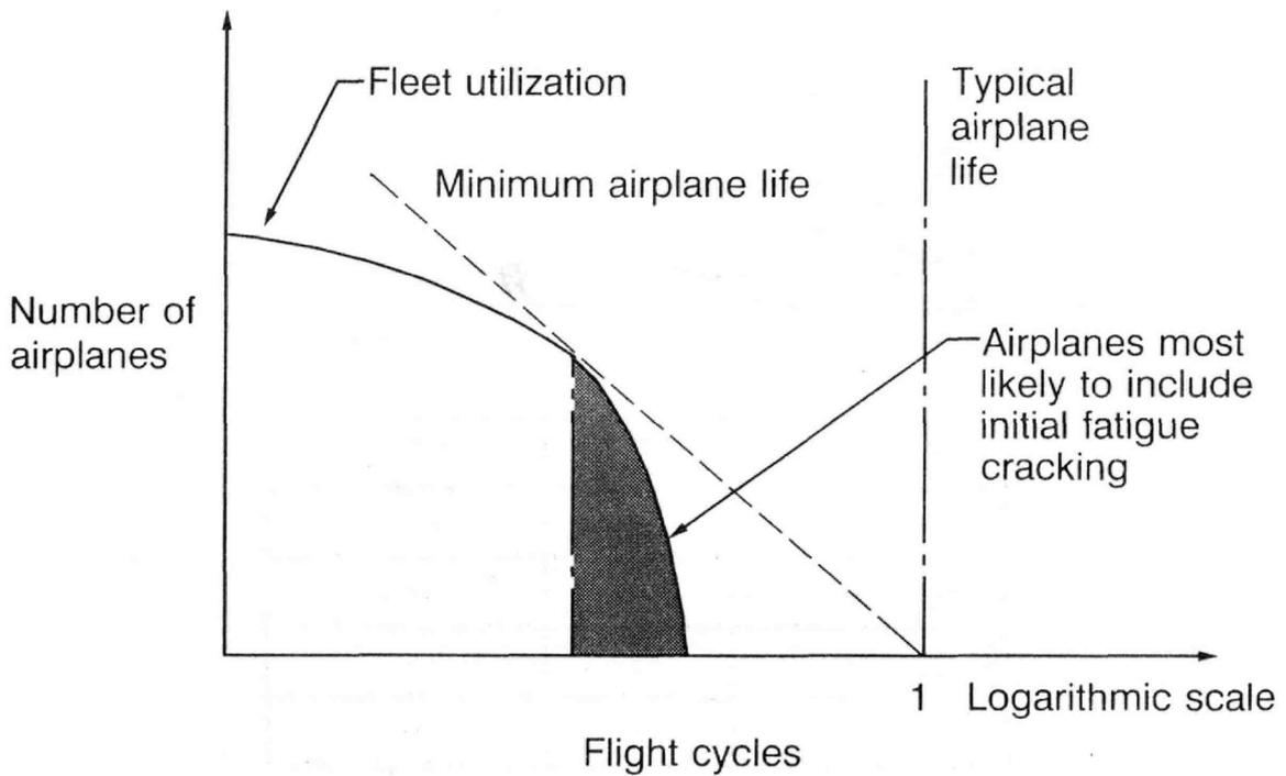
Figure 37. Fleet Cracking Order Based on Fatigue Life Distribution
