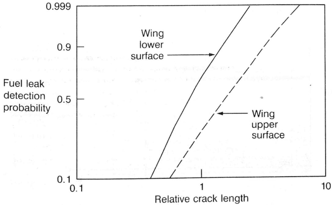
Figure 31. Probability of Fuel Leak Detection
