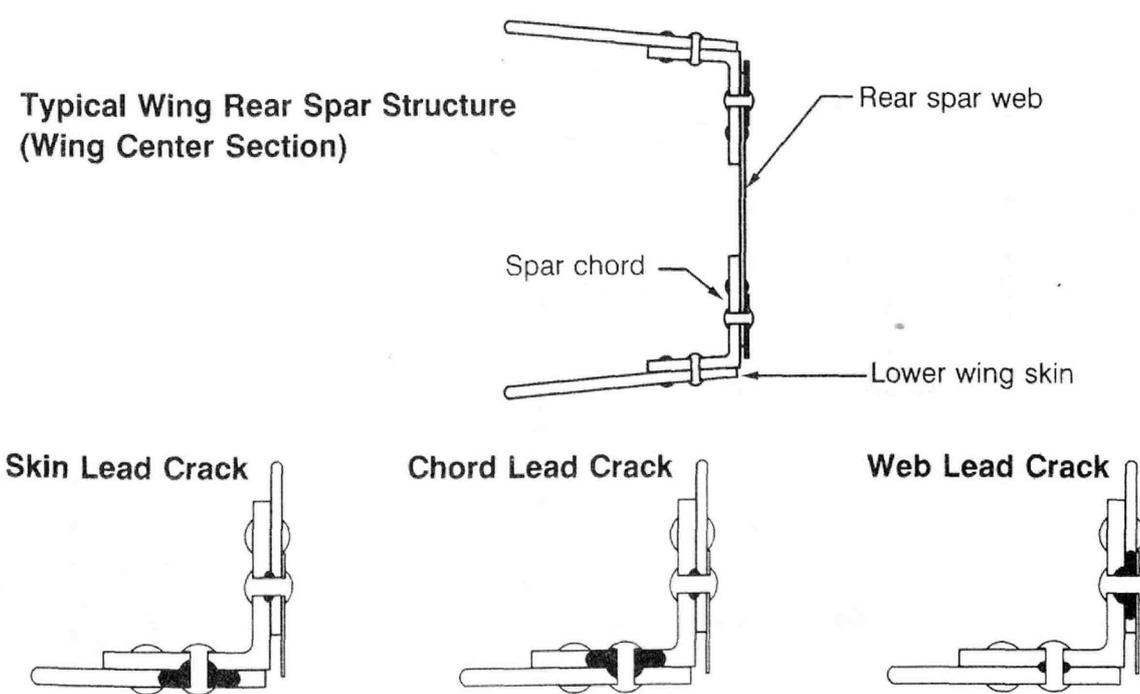
Figure 54. Wing Spar Chord Cracking Pattern Examples
