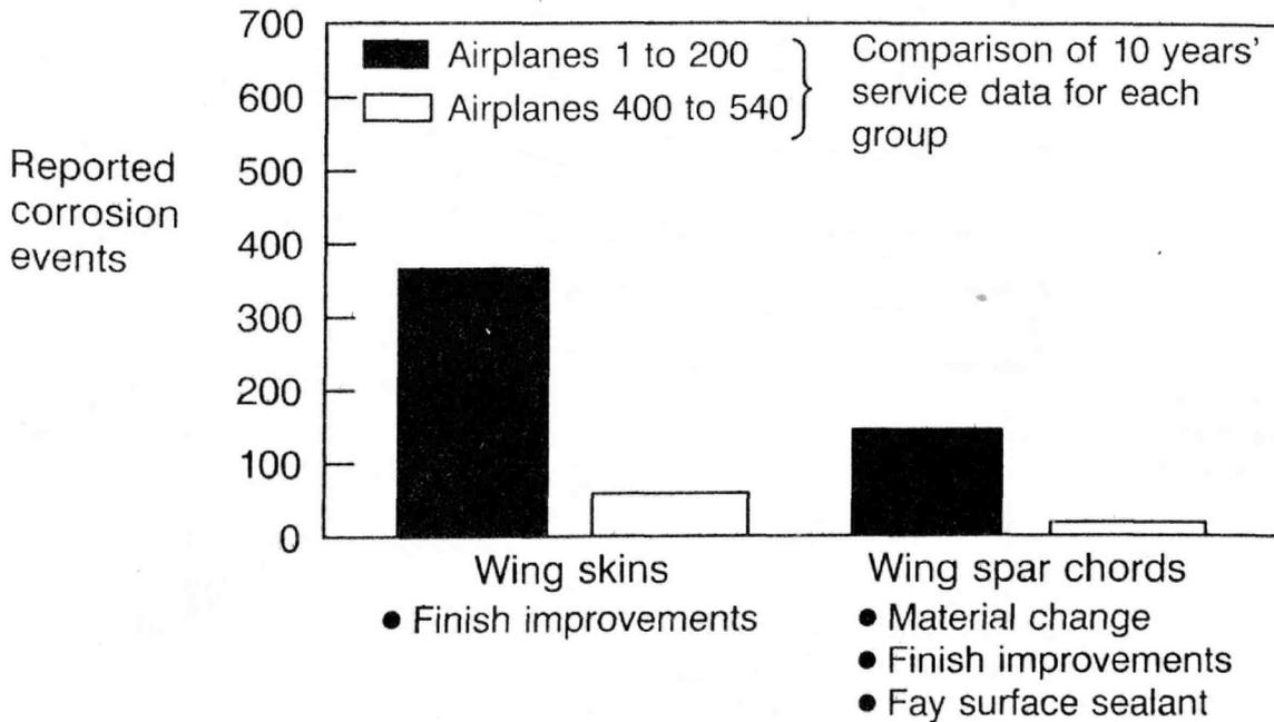
Figure 78. Corrosion Prevention Design Improvements Examples—Model 747
