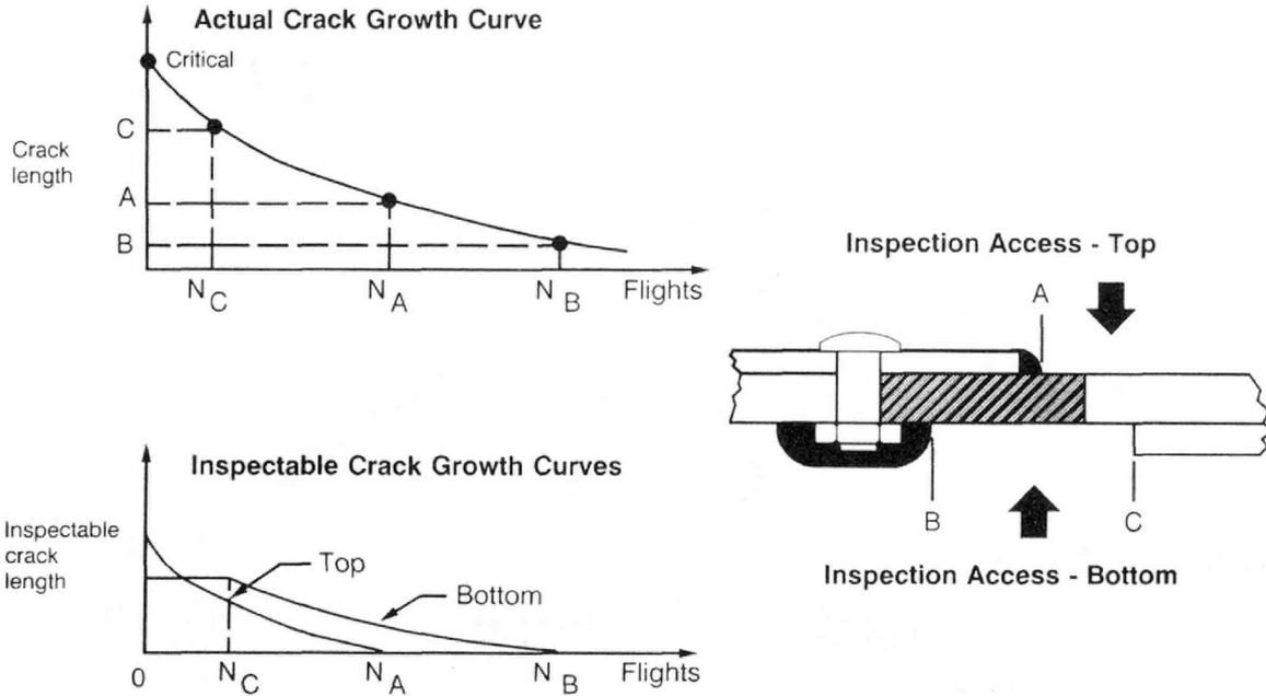
Figure 47. Inspectable Crack Length Considerations
