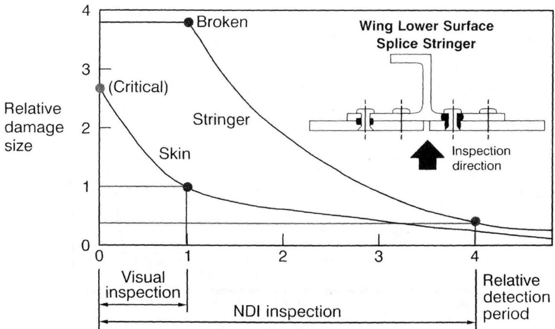
Figure 21. Visual Versus NDI Damage Detection Periods
