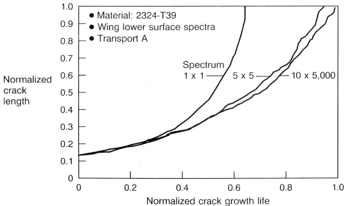
Figure 14. Effect of Spectrum Complexity on Crack Growth
