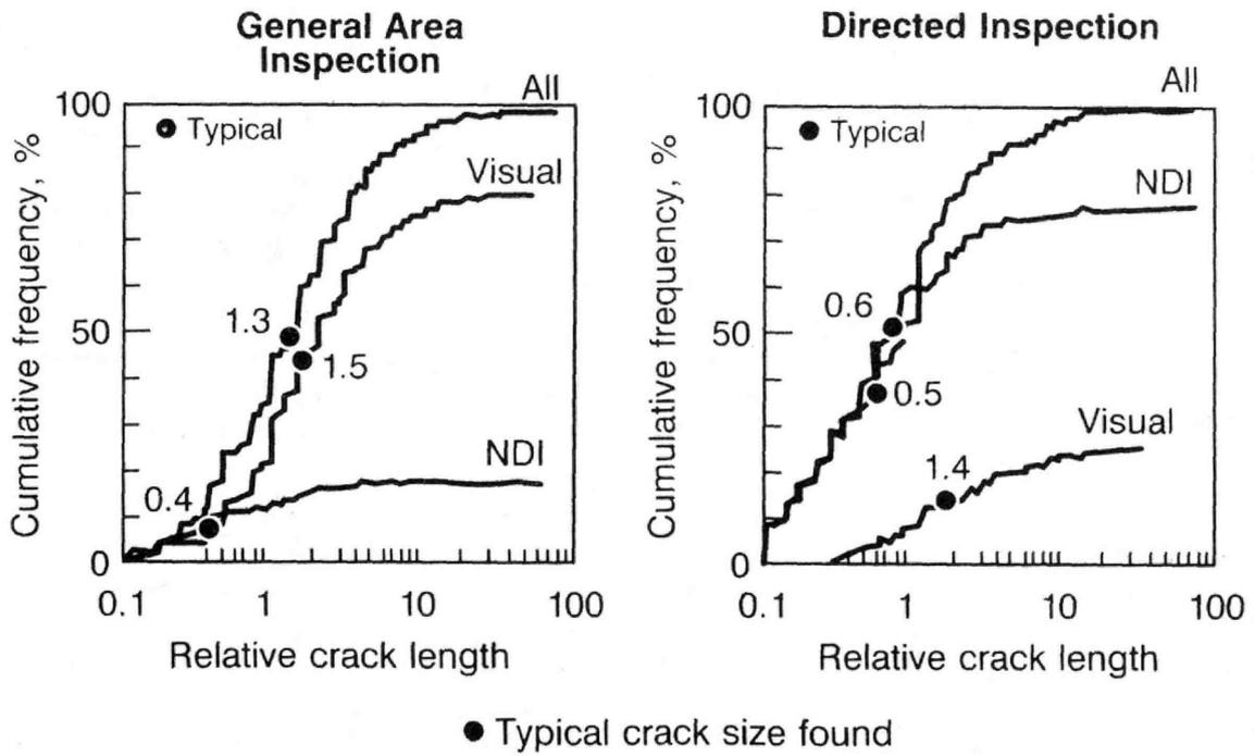
Figure 28. Distribution of Cracks Found in Service
