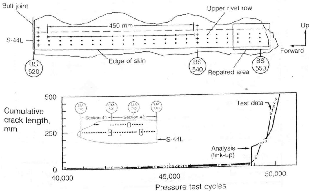
Figure 19. 747-400 Fuselage Lap Splice Test Results—Stringer 44L
