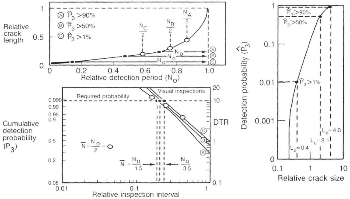
Figure 51. Cumulative Detection Probability—Detection Threshold Probability Variation
