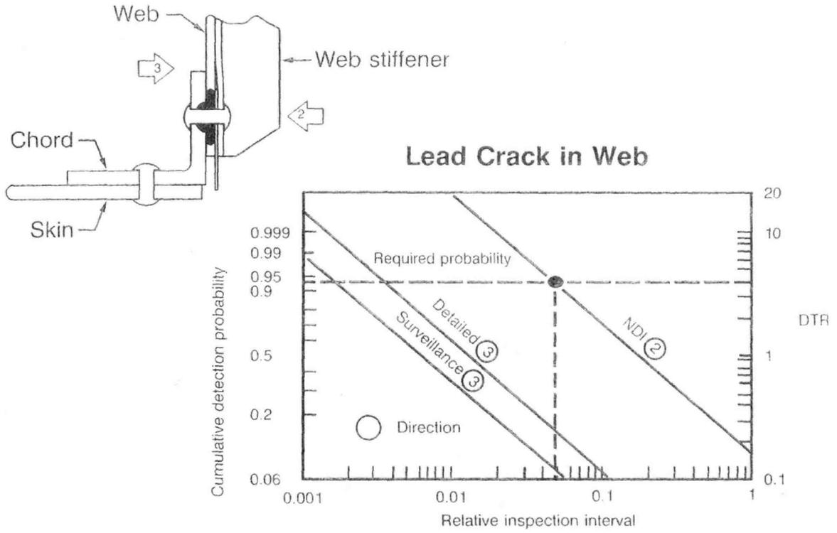
Figure 59. Cumulative Detection Probability Locally Hidden Web Details
