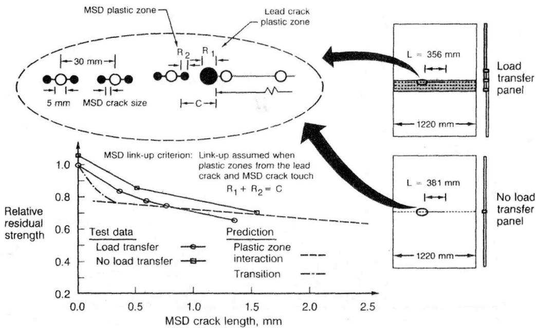
Figure 90. Test and Prediction of Failure Stresses for Flat Panels Containing MSD at Each Fastener Hole
