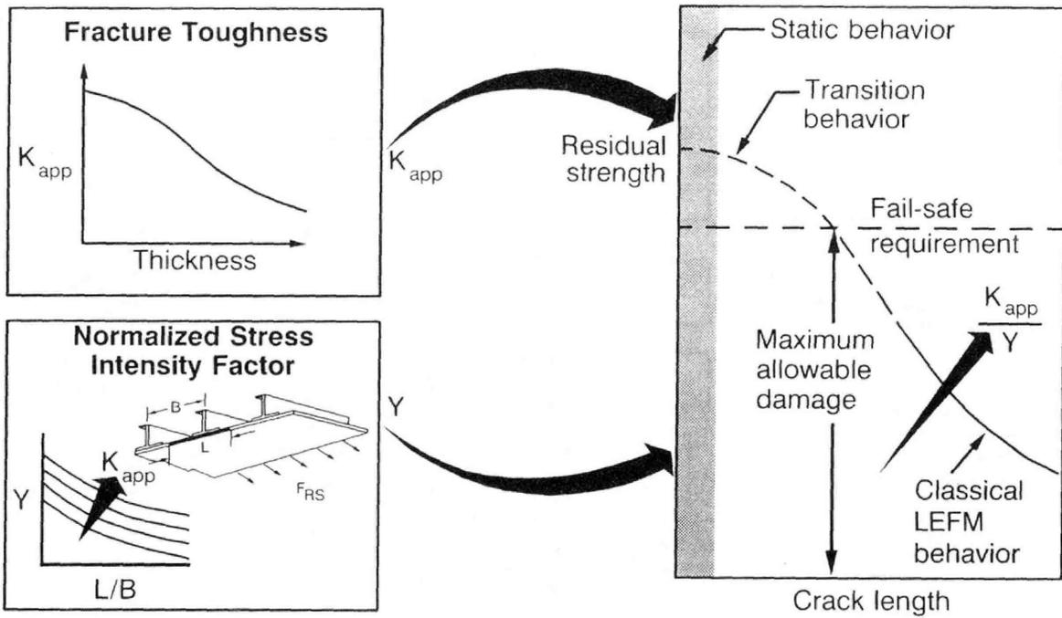
Figure 5. Residual Strength Technology Standards
