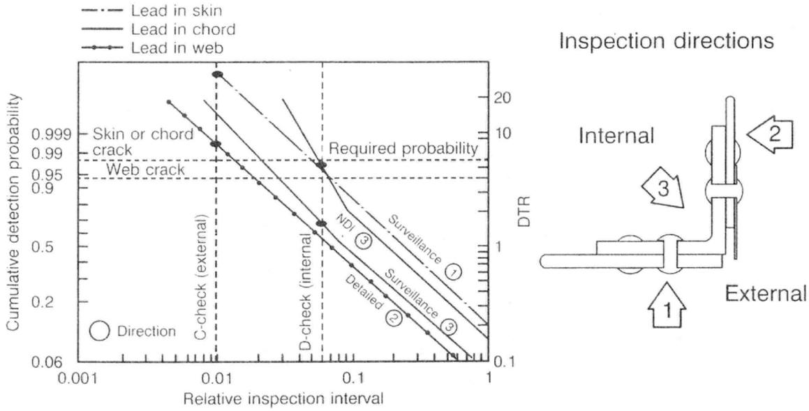
Figure 57. Cumulative Detection Probability—Cracking Pattern/Inspection Direction Combinations
