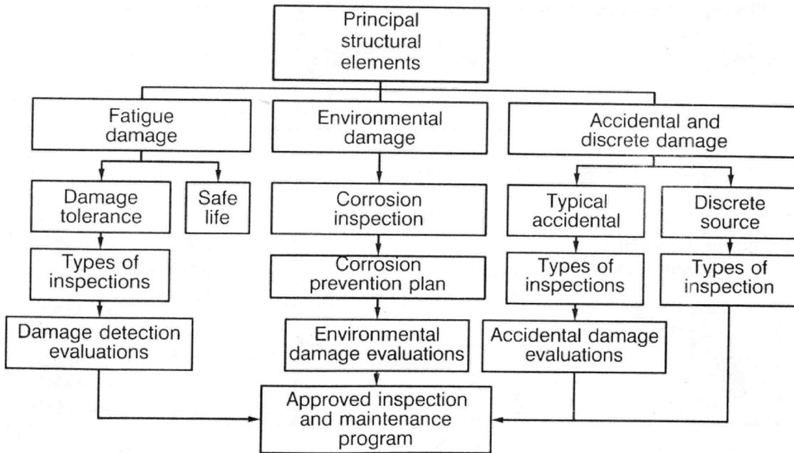
Figure 3. Principal Damage Sources for Maintenance Planning Considerations
