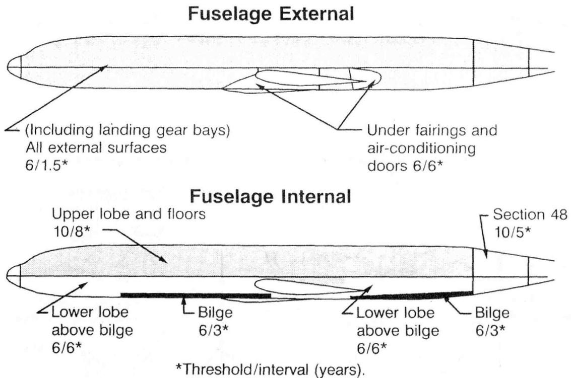
Figure 72. 727 Corrosion Control Program—Example
