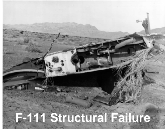
Figure 1. The outer wing section of the F-111 aircraft that failed due an undetected forging defect (rogue flaw) in the D6AC high strength steel pivot fitting under a 4 g loading.
