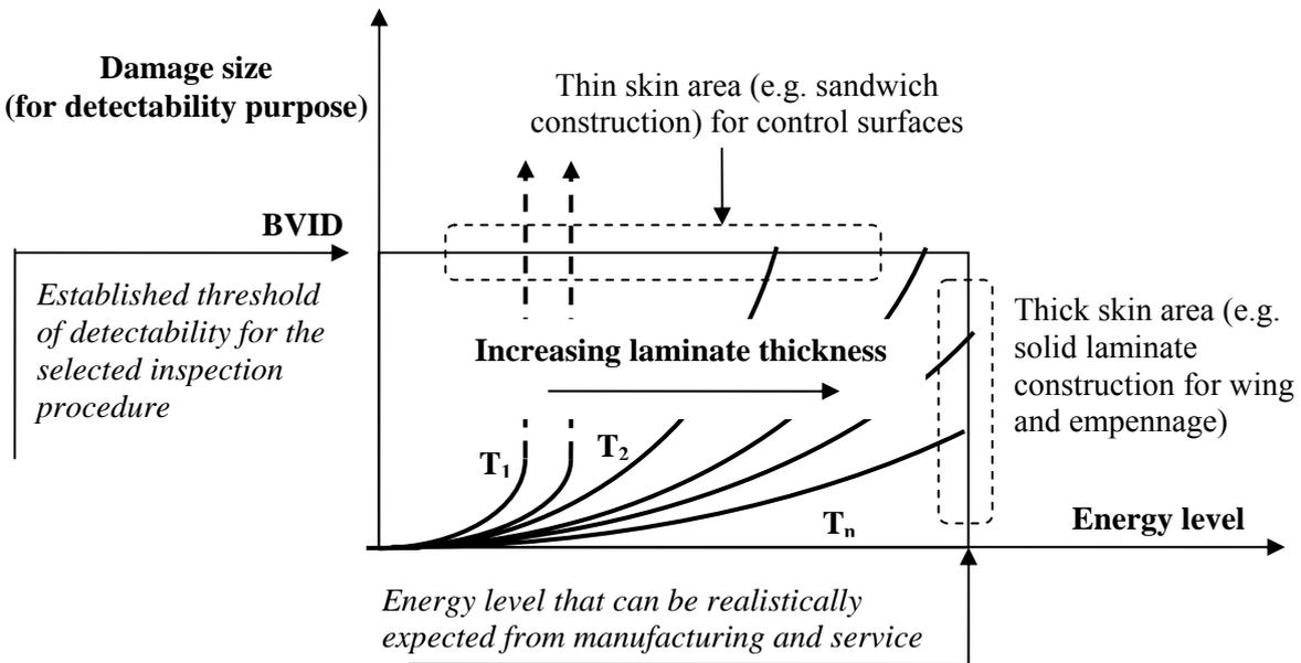
Figure 14: Illustration of the AC 20-107A, § 6g
