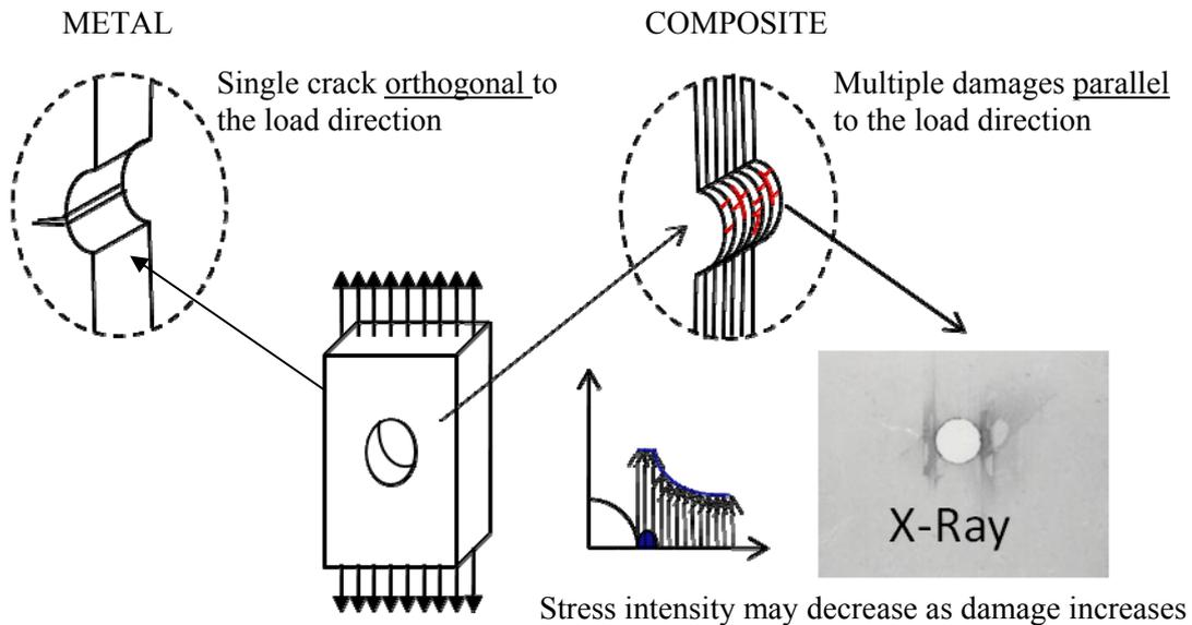
Figure 2: Fatigue initiation and damage growth around a hole
