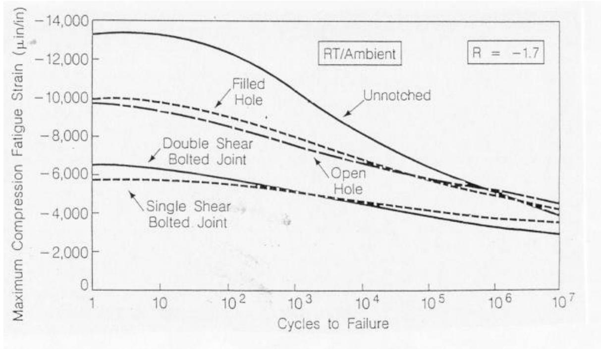
Figure 3: General fatigue behaviour of composites (Whitehead, ICAF 1987)
