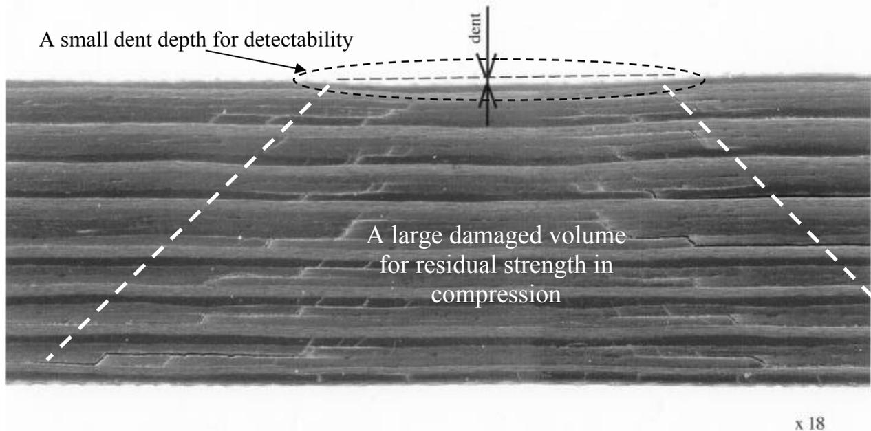
Figure 13: Low velocity impact damage micrography
