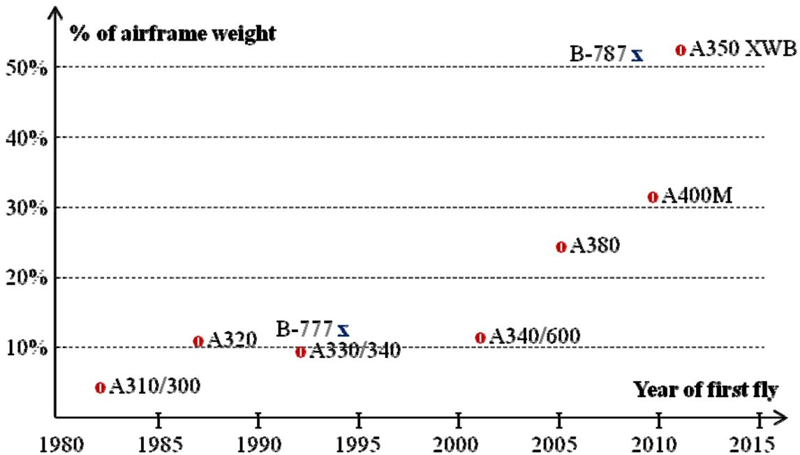
Figure 1: Evolution of the composite ratio on commercial aircraft
