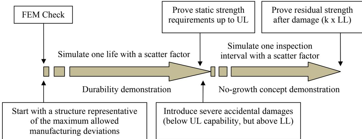
Figure 10: The full-scale test protocol
