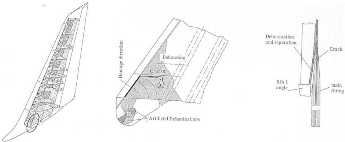
Figure 4: Fatigue failure by disbonding in the test of a vertical fin
