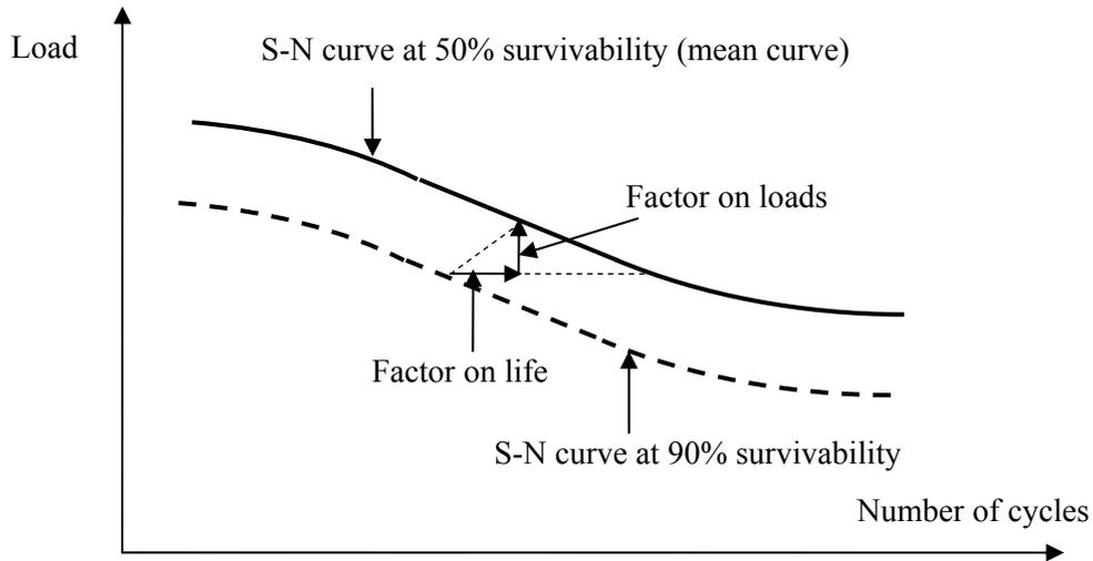
Figure 6: Load/life factor principle to cover a 90% reliability
