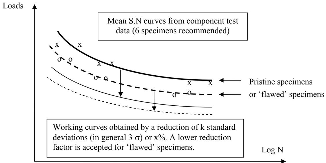
Figure 8: Fatigue substantiation principle for rotorcraft elements
