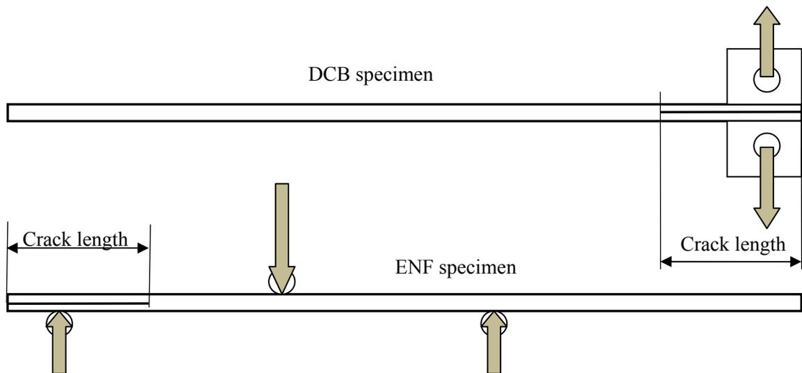
Figure 5: DCB and ENF specimens for delamination studies (static and fatigue)
