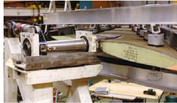
Abt. 800 initial flaws installed in full-scale component testing
