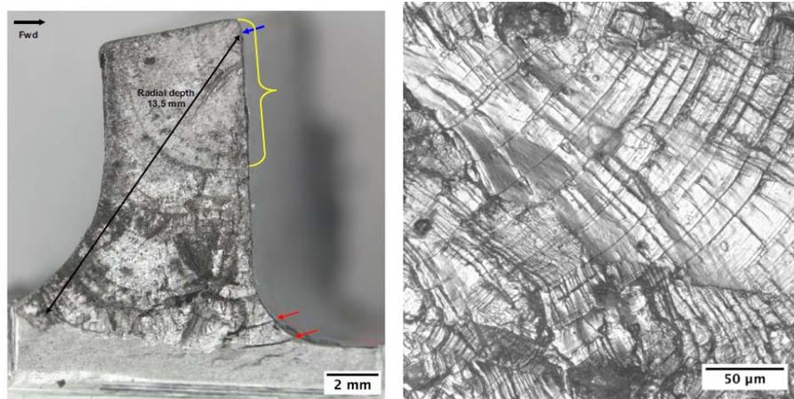
Figure 2. *Fatigue cracking direction and visible progression marks*
