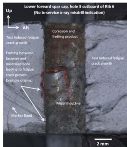
Figure 2. Fractography of the main spar cap primary failure location which contained a miss-drill not identified in-service.
