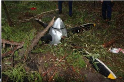
Figure 2. Propeller as found
