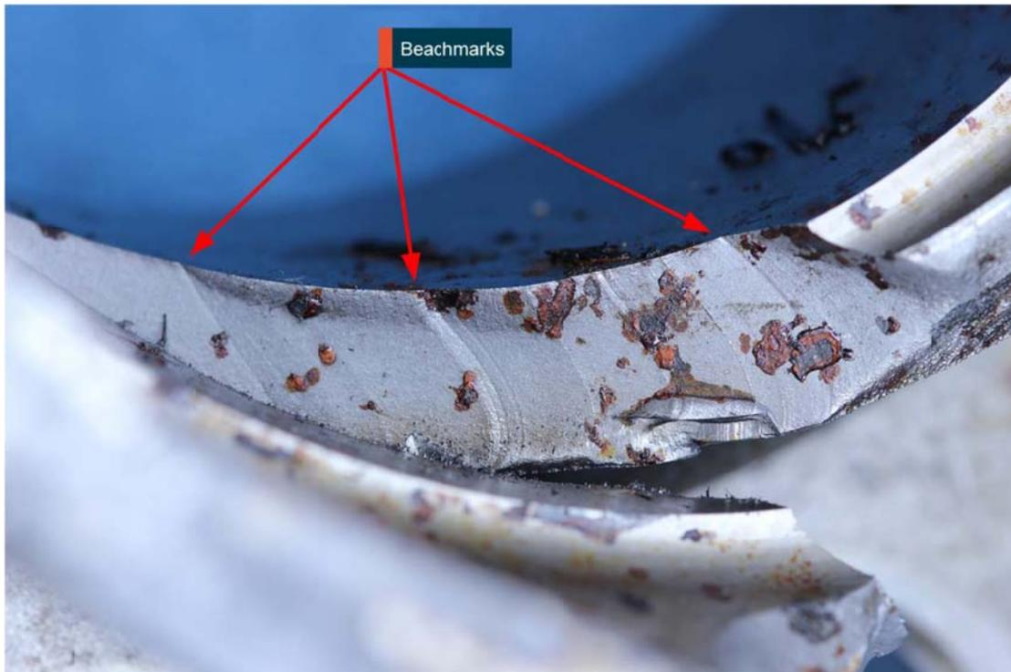
*Figure 5. Image shows the beachmarks on the fracture surface, which was indicative of a fatigue failure mechanism. Source: ATSB*
