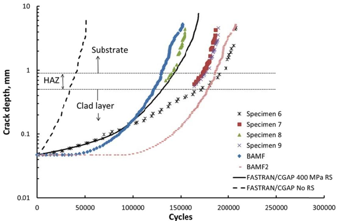
Figure 2. Modelling results for crack propagation through compressive residual stress field in case of laser cladding repair of AerMet®100 steel
