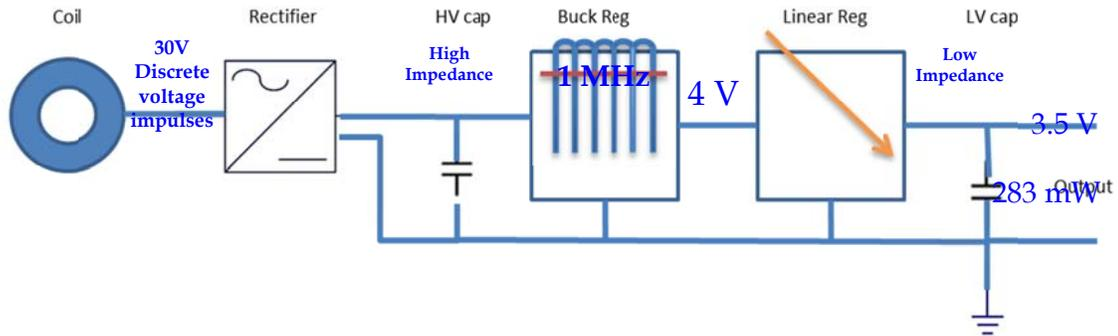
Figure 2. Energy harvester functional block diagram
