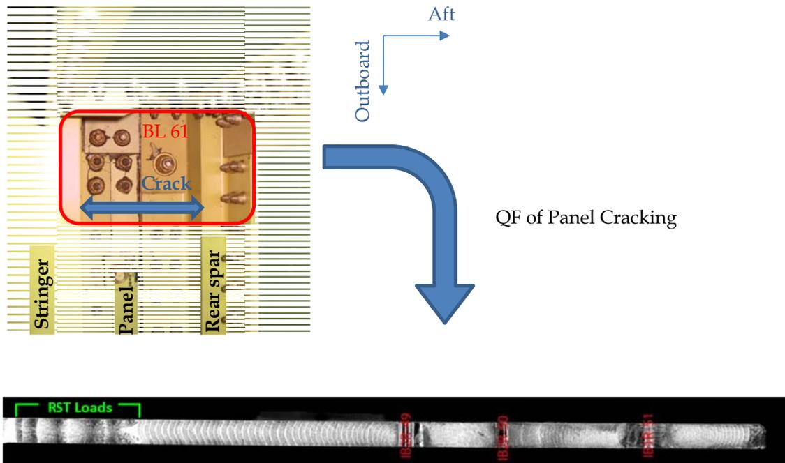
Figure 2. Example teardown location and fracture surface picture ready for QF in the BL 61 region (centre wing to fuselage attachment point at the rear spar cap)
