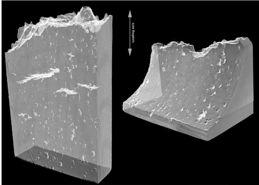
Figure 1. X-Ray synchrotron CT reconstructions of corroded low- $k_t$  (left) and high- $k_t$  (right) fatigue specimens of aluminium alloy 7050-T7451. Each specimen is approximately 5 mm wide.
