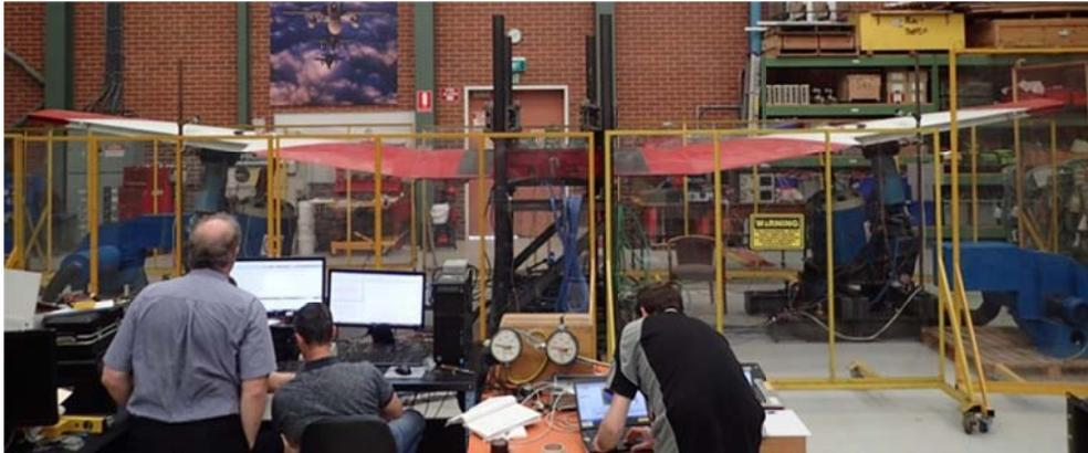
Figure 1. The PC-9/A wing enhanced teardown test rig at DST Fishermans Bend, Melbourne
