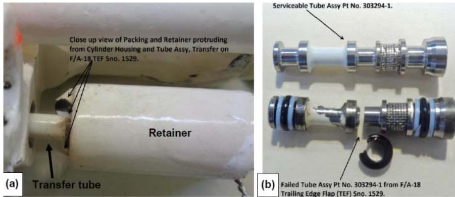
Figure 1. Location of cracking
