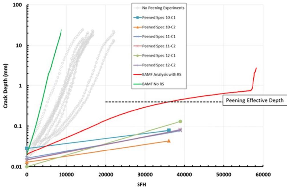
Figure 4. Crack growth predictions vs experiment for with and without shot peening
