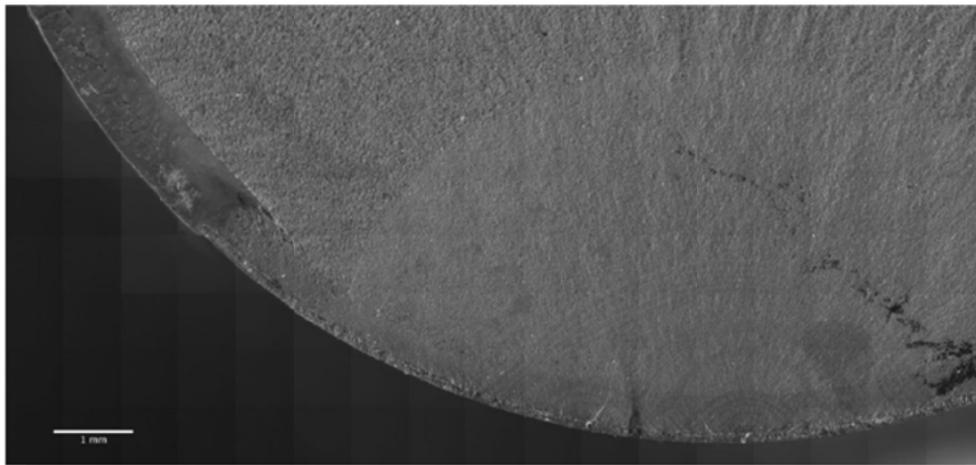
Figure 1. The LAD repaired specimen from [2]
