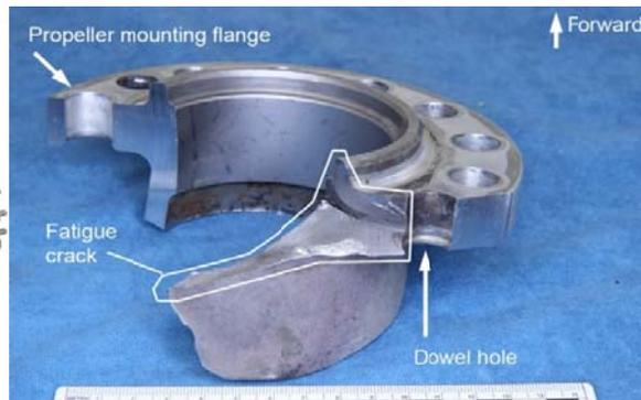
Figure 4. Section of propeller shaft
