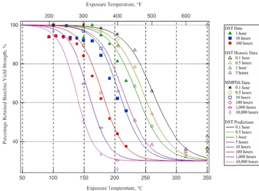
Figure 1. DST Group retained strength model predications for AA7050 tested against independent data
