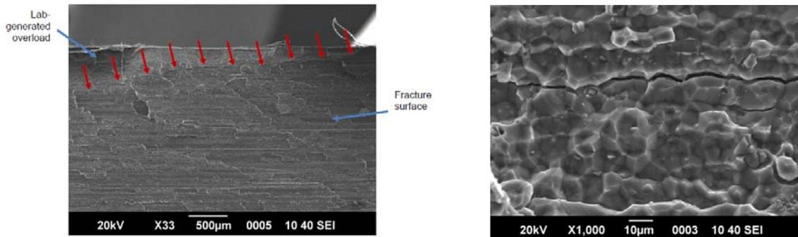
Figure 3. The intergranular nature of the fracture surface
