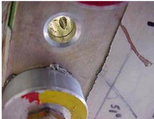
Figure 1. Miss-Drill Damage at Spar Cap Hole
