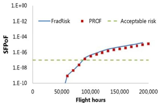
Figure 1. Comparison of FracRisk and PROF results using tabulated stress exceedance data for C-130J CW-3A location
