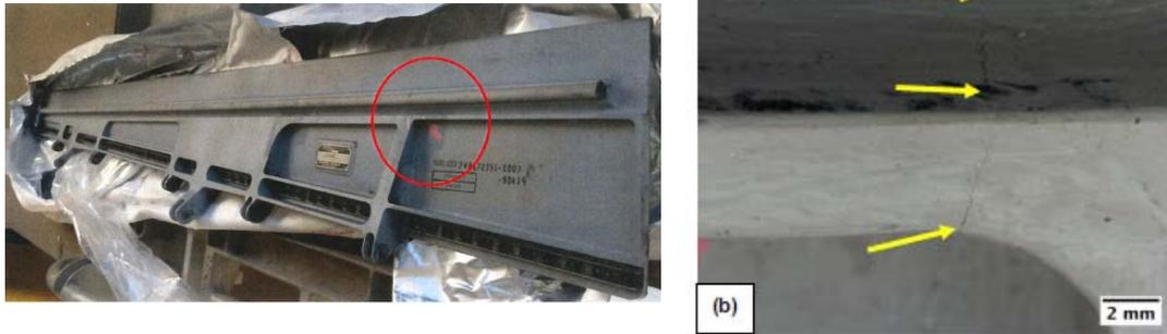
Figure 1: *Location of cracking*
