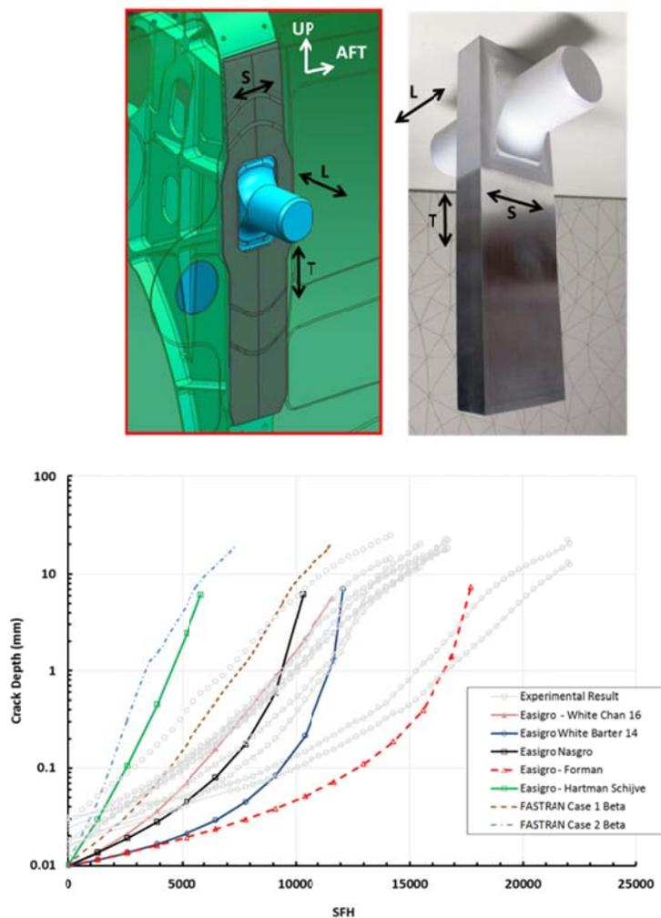
Figure 1. The shear tie post (top), an integral part of a centre fuselage former on a combat aircraft, represented by a symmetric coupon (top right) Note: transverse, long and short relate to plate
