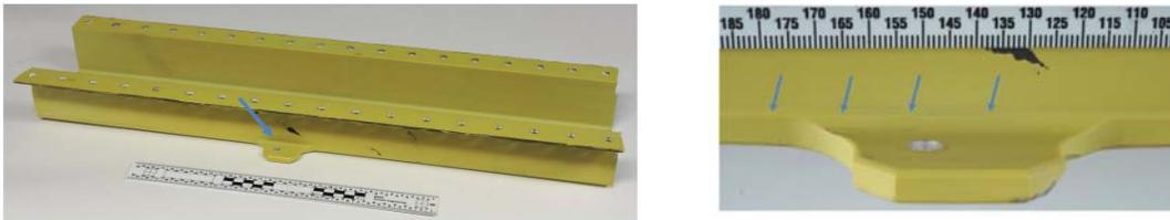
Figure 2. Location of cracking along tab
