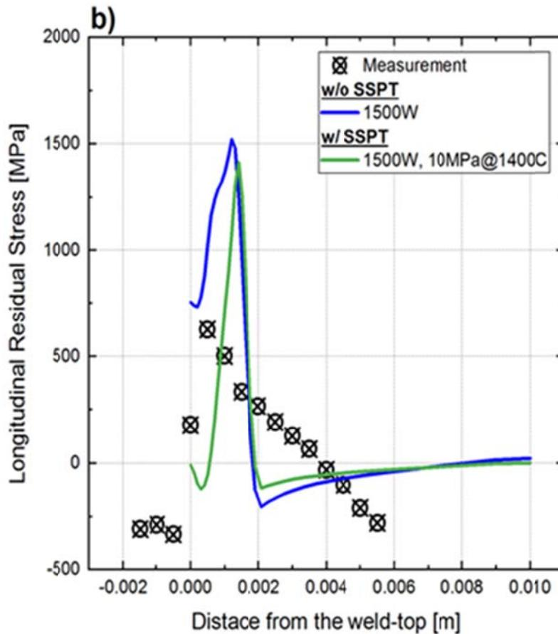
Figure 3. Residual stress profile comparisons, with and without SSPT
