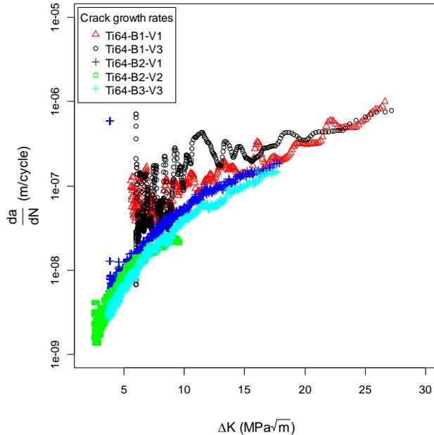
Figure 1. Crack growth rates for the vertically and horizontally built CT specimens of AM Ti-6Al-4V containing numerous lack-of-fusion defects.
