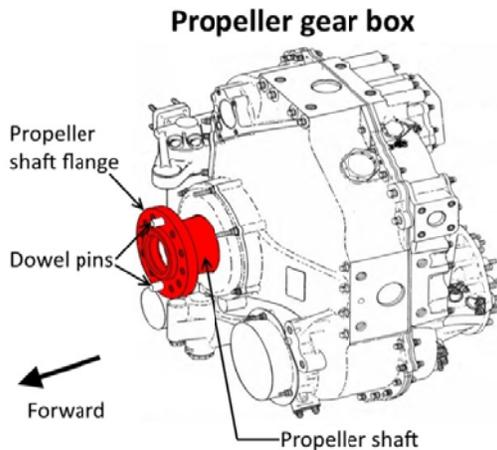
Figure 3. Gear box schematic
