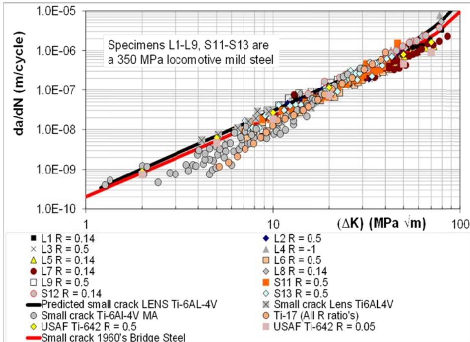
Figure 2. Comparison of crack growth rate data for some Conventionally Manufactured Materials as well as various AM repaired specimens using LAD and Cold Spray (SPD)
