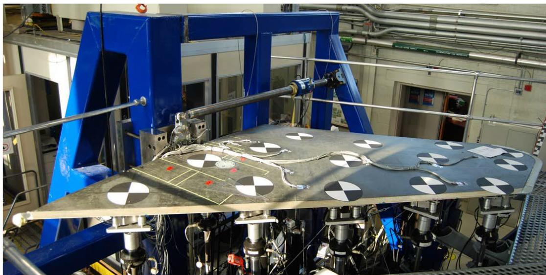
**Figure 10 FTS2 test article with optical marker tracking at actuator locations**
