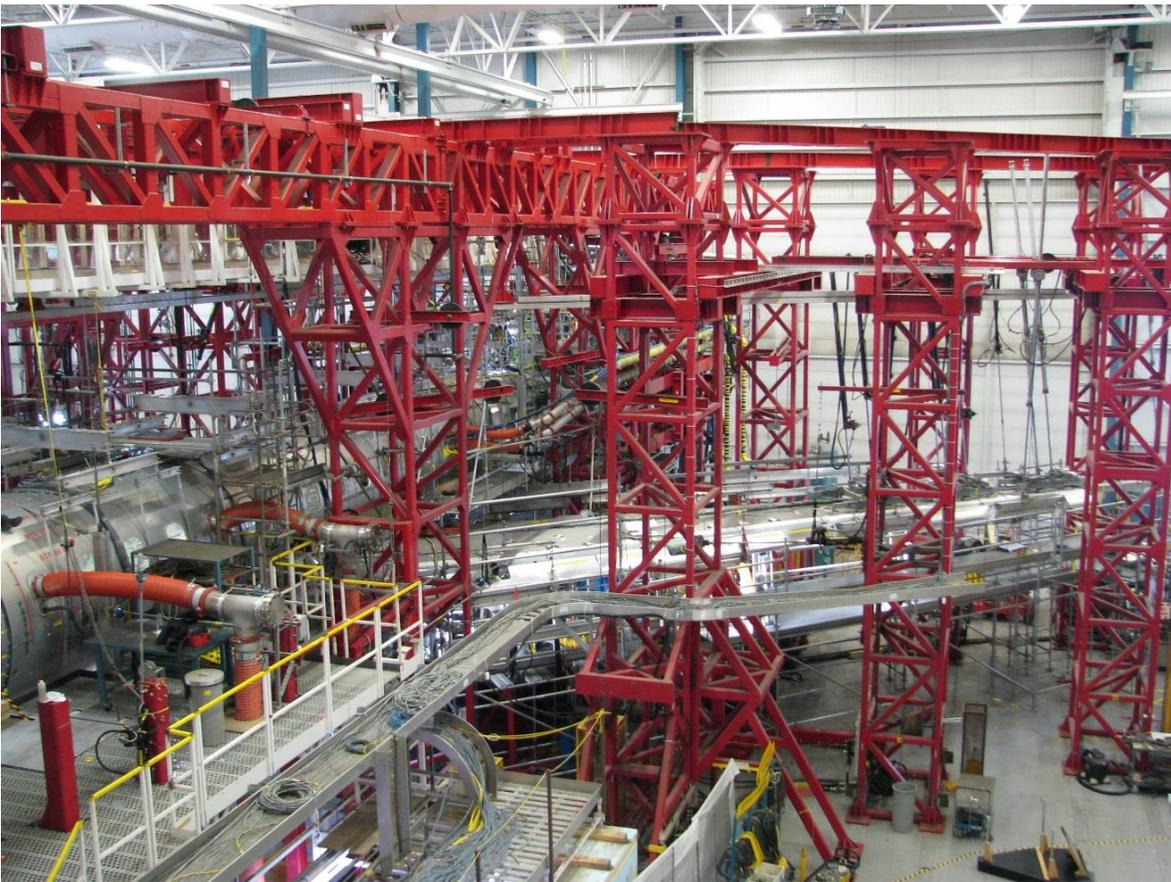
**Figure 1 Global 7500 durability and damage tolerance tests in Montreal, Canada
