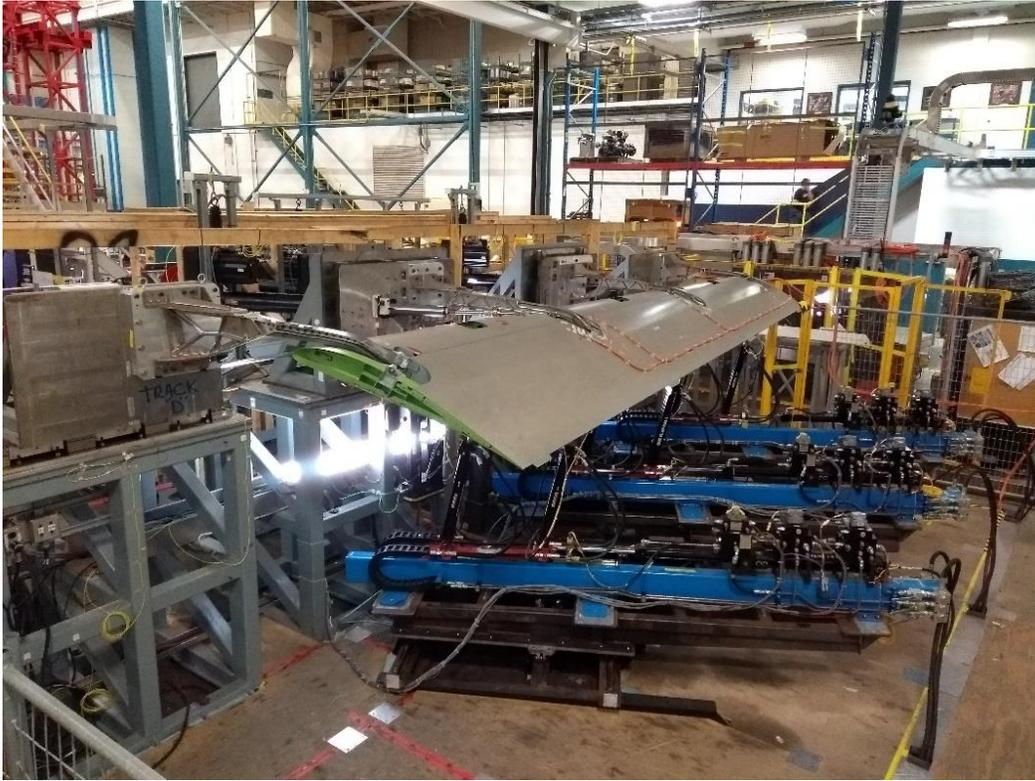
**Figure 6 Outboard flap test rig**
