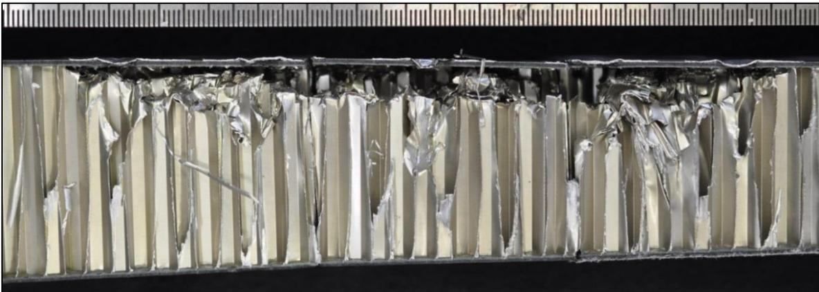
**Figure 17 CF-188 FT905 H-Stab lengthwise section cut showing induced damage with no growth at edges**
