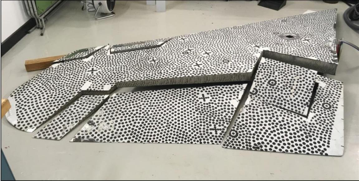
**Figure 16 CF-188 FT905 H-Stab following initial sectioning for tear-down inspection**
