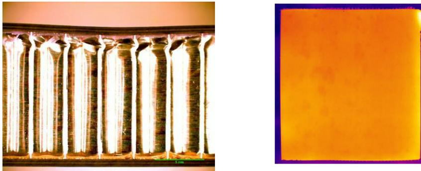
**Figure 45 a) Cross-section of an impact location with an intact adhesive bond, b) thermographic image of the surface of the impact region**
