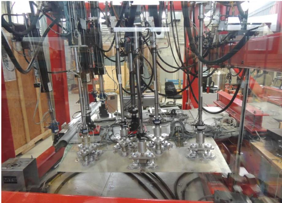
**Figure 13 Aileron test (FT370) article and test rig**
