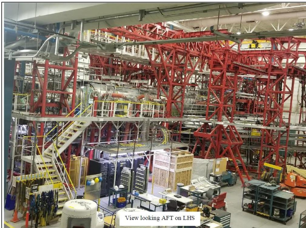
**Figure 8 Global 7500 DADTT test setup (view AFT on LHS)**
