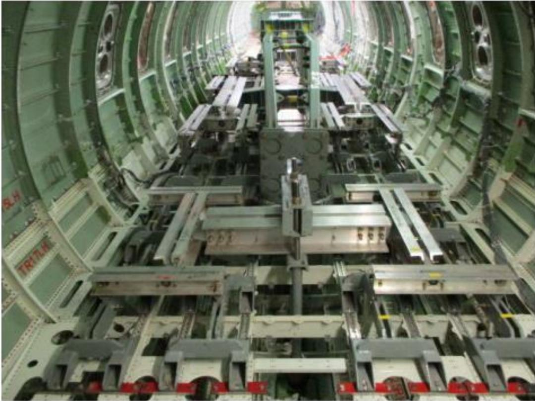
**Figure 4 Close-up of fuselage test setup**
