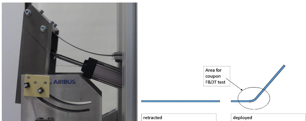
Figure 22: Test bench and schematic principle of bending test
