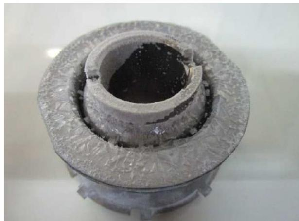
b) bearing after salt spray test
