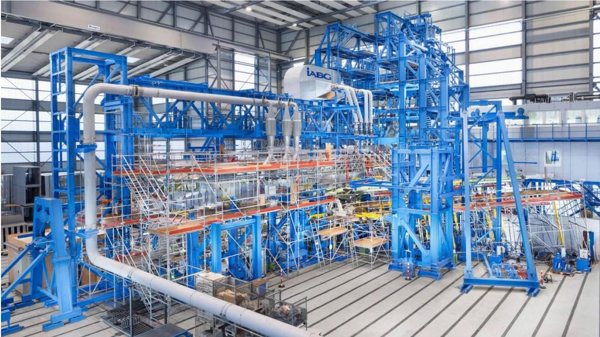
Figure 4: The BD500 Fatigue Test Set-up at IABG in Dresden
