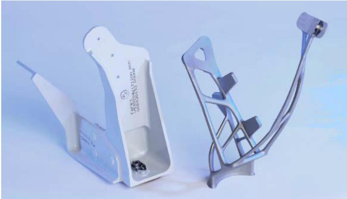
Figure 19: Secondary Structure (Bracket) developed by Premium Aerotec GmbH. Conventional design (milling plus riveting) compared with topologically optimized design developed for the Additive Manufacturing (53% weight saving, 40% cost saving).
