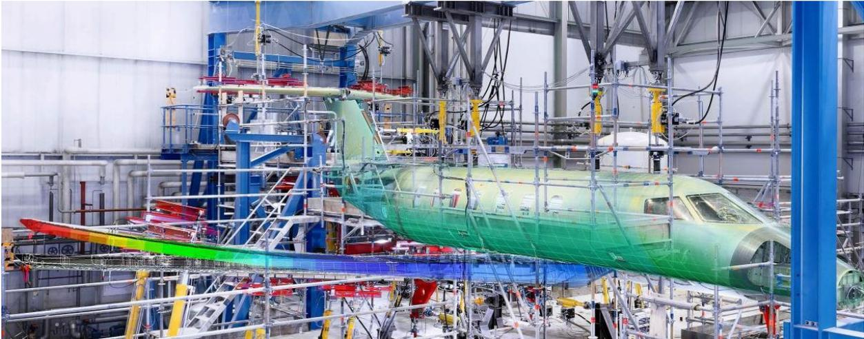
Figure 5: Full-Scale Fatigue Testing
