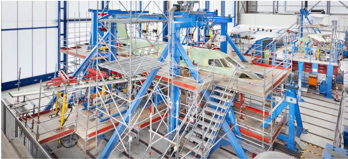
Figure 1: PC-24 FSFT - Test Overview (with FSEFT and GLC in background)
