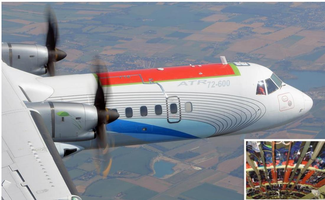
Figure 6: Flight test of the composite crown panel on an ATR 72-600 with a network of 94 sensors developed by Fraunhofer LBF. © ATR/Alenia Aermacchi(Leonardo)
