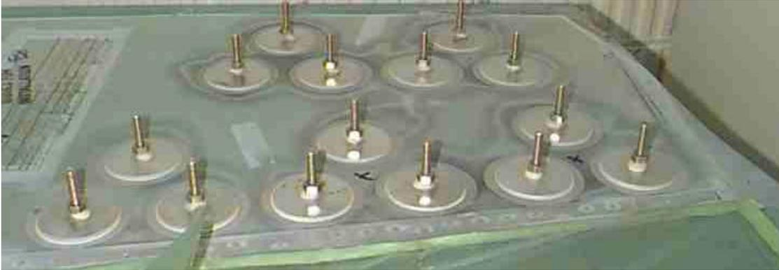
Figure 5. Example of Thin Disc Loading Pads
