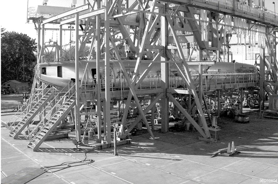
Figure 121. 737-800 Full Scale Fuselage Fatigue Test Setup
