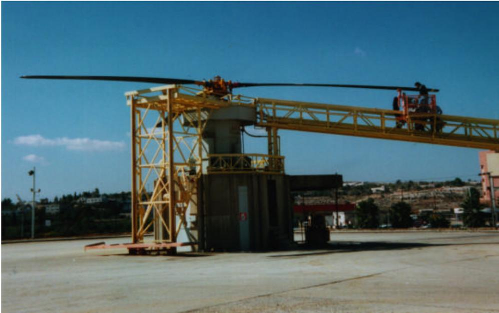
Figure 18. Dynamic Testing of Helicopter Blade
