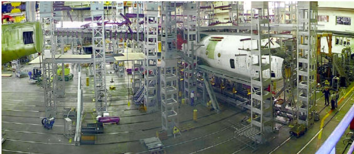
Figure 32 : Transall full-scale fatigue test
