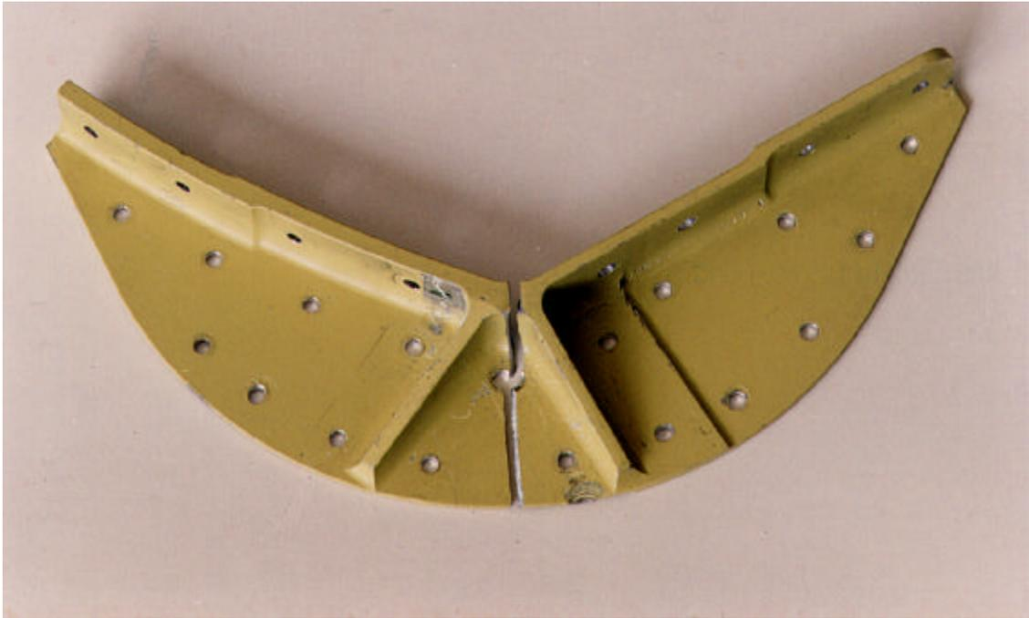
Figure 28 : TBM 700 fatigue failed component after taking-down
