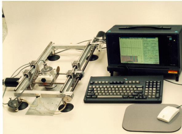
**Figure 151. Pulsed-Eddy Current (PEC) Device**
