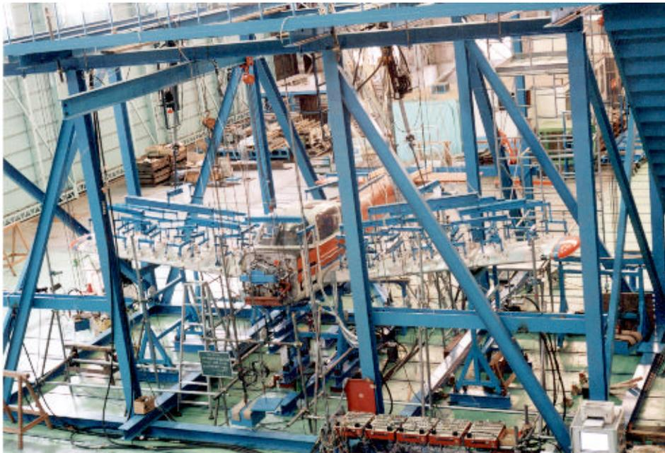
**Figure 40 Static test set-up.**
