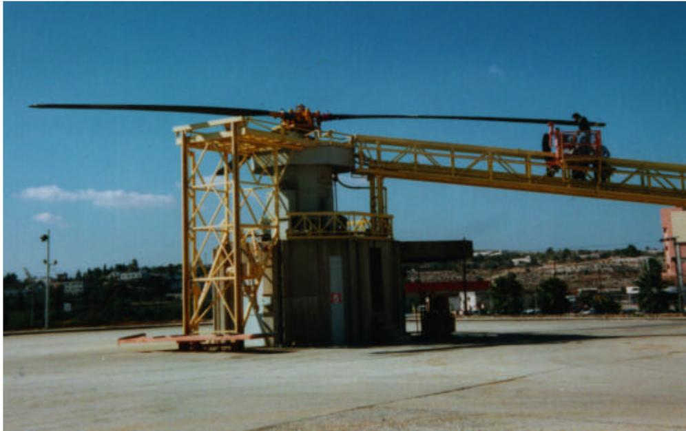
Figure 18. Dynamic Testing of Helicopter Blade
