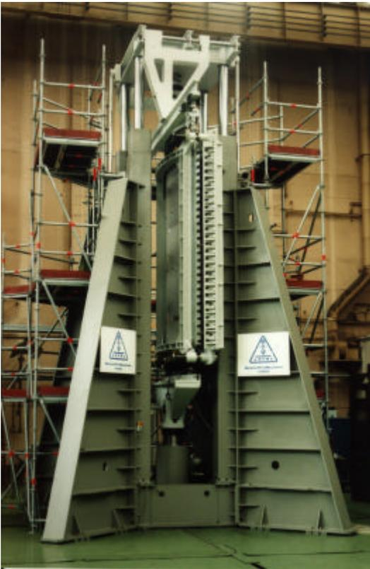
Fig. 31: Test facility for curved fuselage panels.
