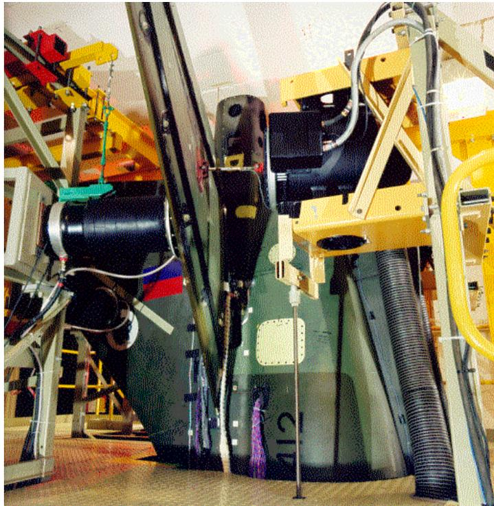
Figure 24 View showing Harrier empennage buffet test; tailplane in the foreground, steady load air actuator to left and electromagnetic shaker providing dynamic excitation to right of picture
