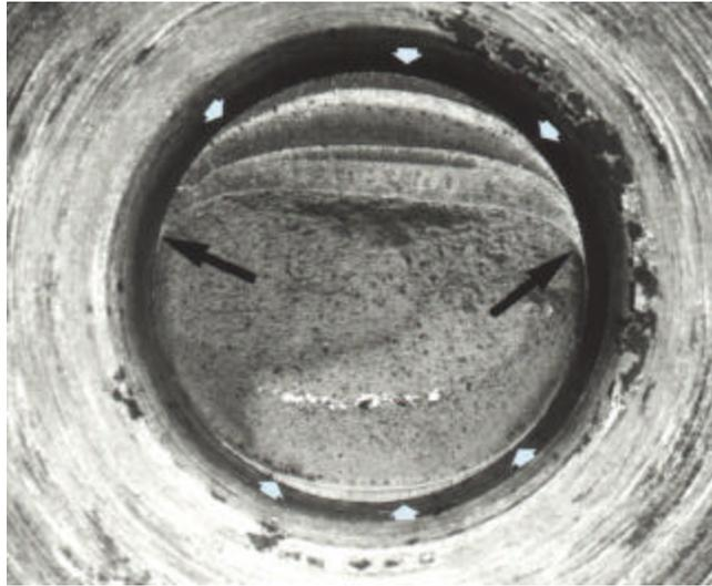
**Fig. 4.5.3 Fatigue crack surface of cracked bolt**
