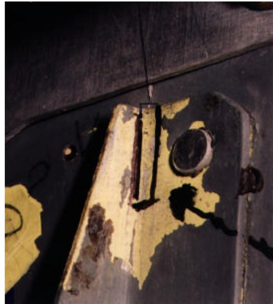
Figure 30 : Fatigue damage at the Gazelle bulkhead
