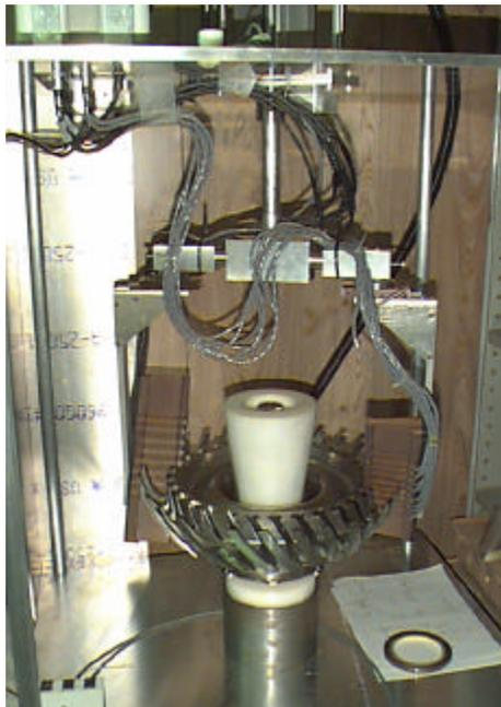
**Figure 162. ETC Portable Scanner Applied to AlliedSignal Engine Component**
