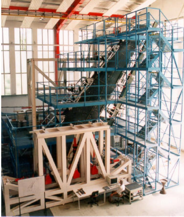
Fig. 41: Test setup for fatigue tests on the CFRP vertical stabilizer, A330-200.
