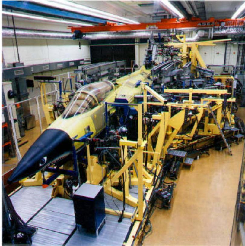
**Figure 26** Photograph of the full-scale fatigue test of the Gripen single seater
