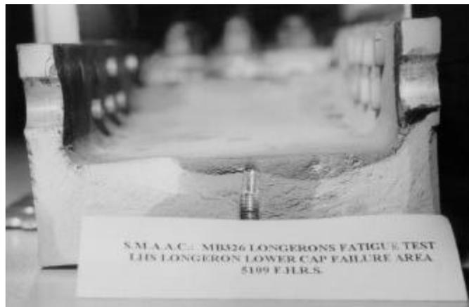
Fig. 28 Fracture surface of LH spar cap
