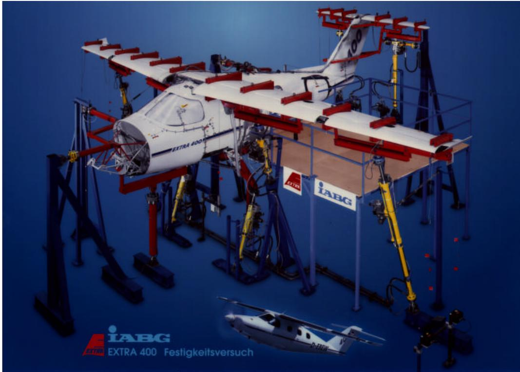
Fig. 38 Completely assembled test set-up containing the EA-400 test article.
