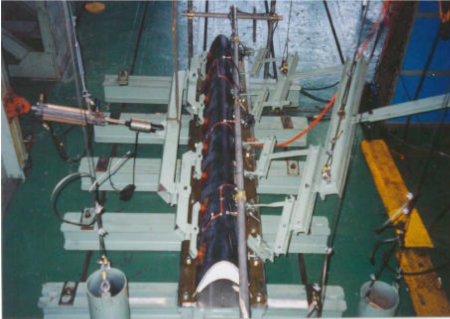
**Figure 31 Test set-up for a vertical stabilizer leading-edge.**
