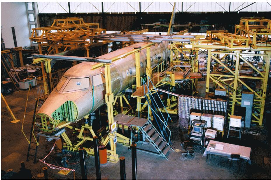
**Figure 13: Galaxy Full-Scale Fatigue Test Aircraft in Loading Fixture**
