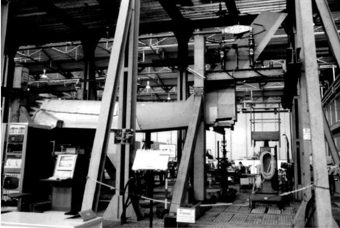
Fig. 24 Assembly for fatigue test of the EH-101 rear tail end fittings
