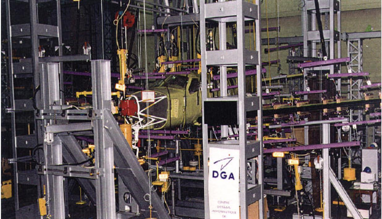
Figure 26 : TBM 700 full-scale fatigue test
