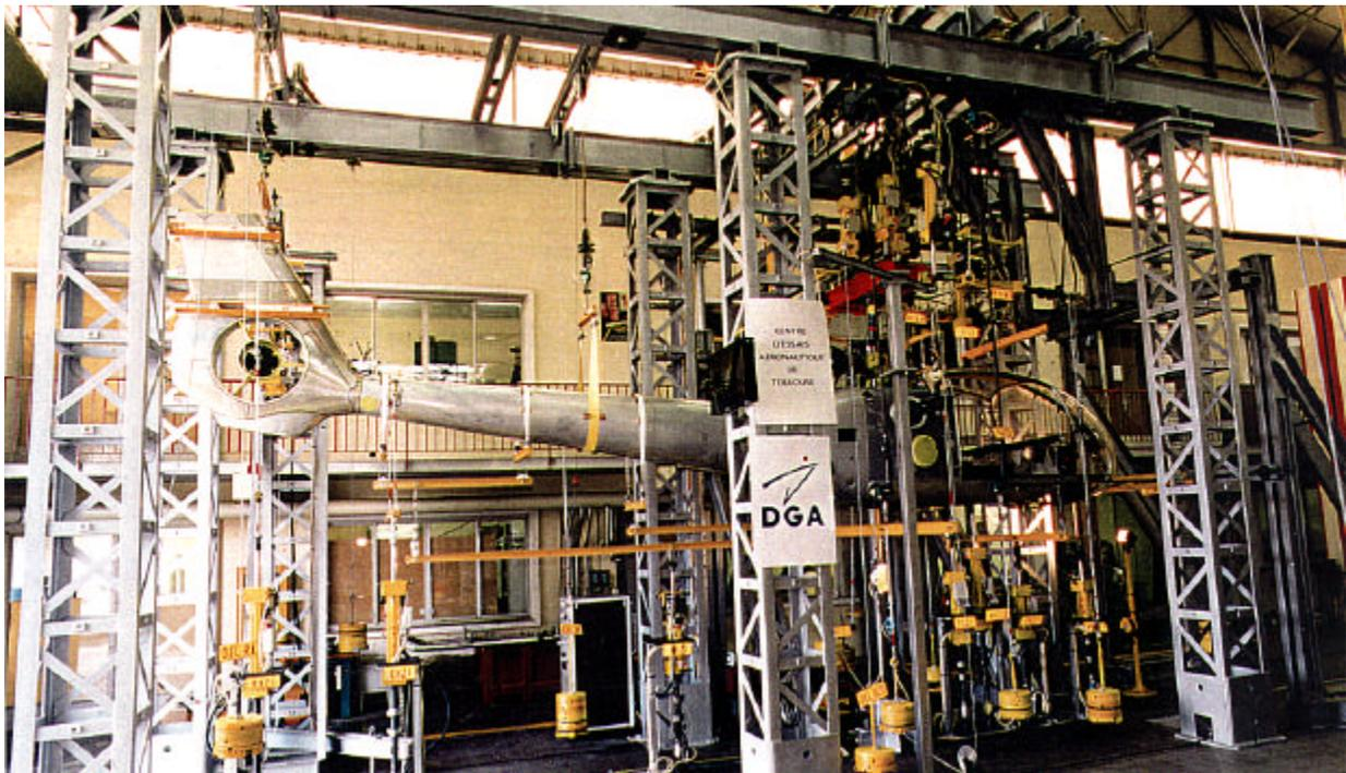
Figure 29 : Gazelle helicopter full-scale fatigue test
