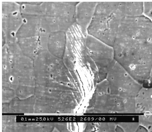
(a) crack growing along a single shear band
