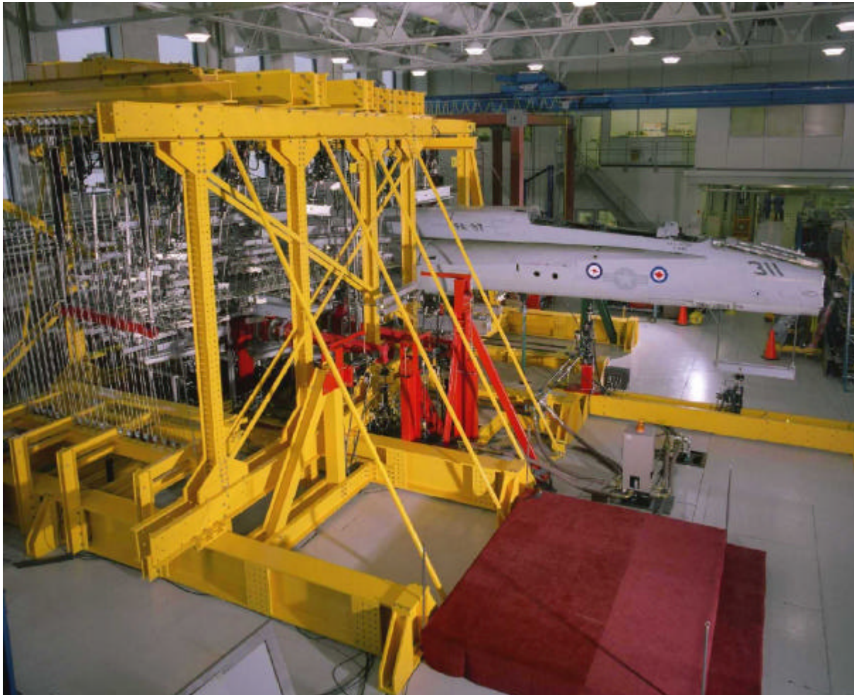
Figure 1. Overall View of FT-245 Wing Fatigue Test.
