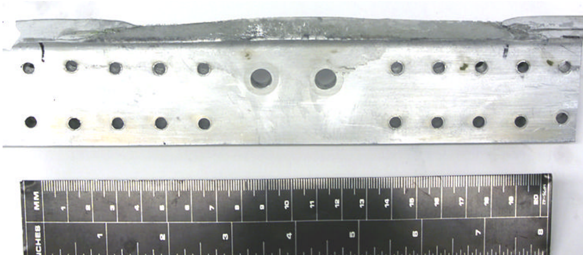
Figure 18. Overall view of the surface of the 7.5 in. long crack at F.S. 497 on the horizontal member of the CC130307 drag angle. With the part as shown, the aft end of the drag angle is towards the left.
