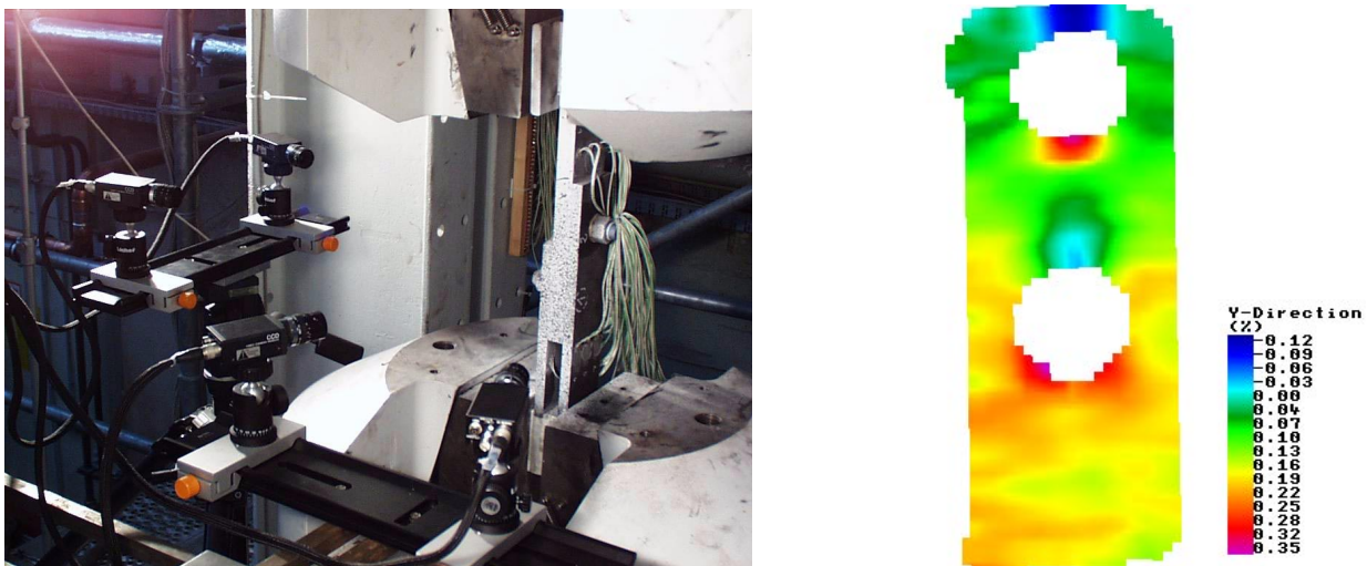
Fig. 22: Test set-up with bolted specimen and optical measurement system (left) and strain distribution on the specimen surface (right).
