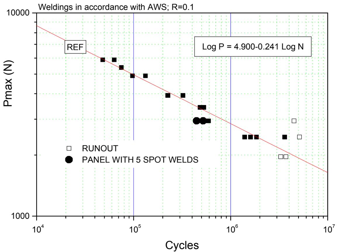
Fig. 29 – Fatigue test results on AISI 301 spot welded joints.
