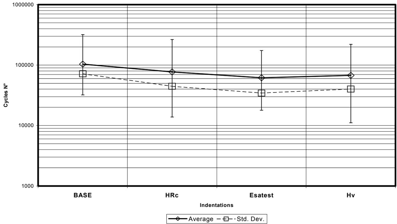
Fig. 7 - Fatigue results of smooth and indented specimens in 4340 steel (R=0.1).
