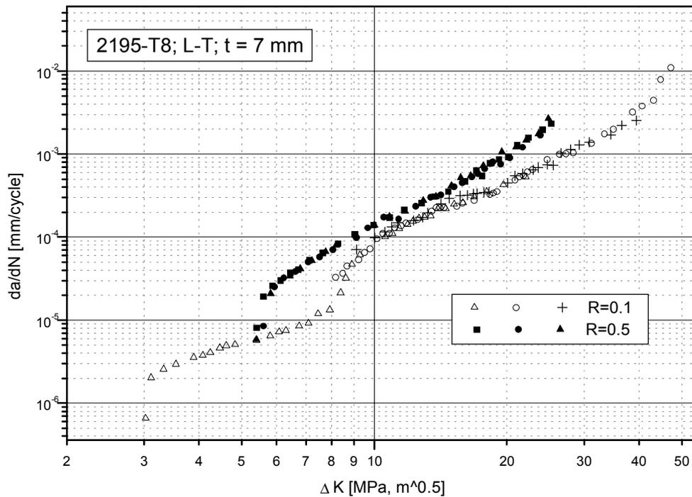
Fig. 12 – Fatigue crack propagation results in Al-Li 2195-T8 alloy.
