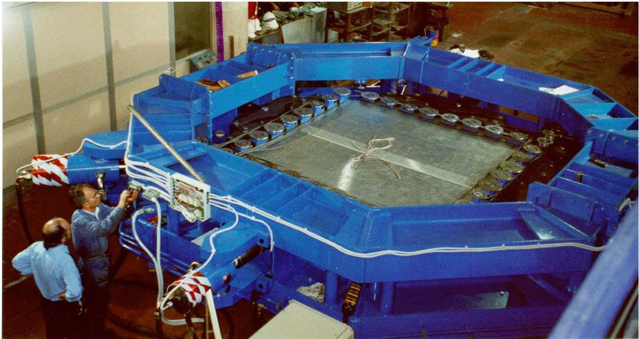
**Fig. 22 – Tri-axial machine for testing flat Glare fuselage panel.**
