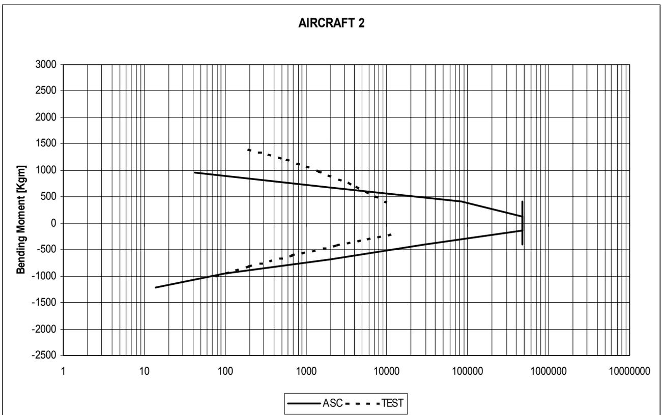
Figure 2 – Example of fin root bending moment spectra for MB-339CD aircraft.
