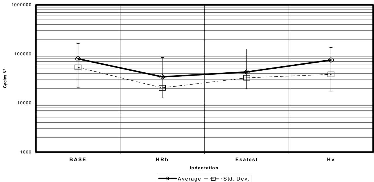
Fig. 8 - Fatigue results of smooth and indented specimens in 15-5 PH stainless steel (R=0.1).
