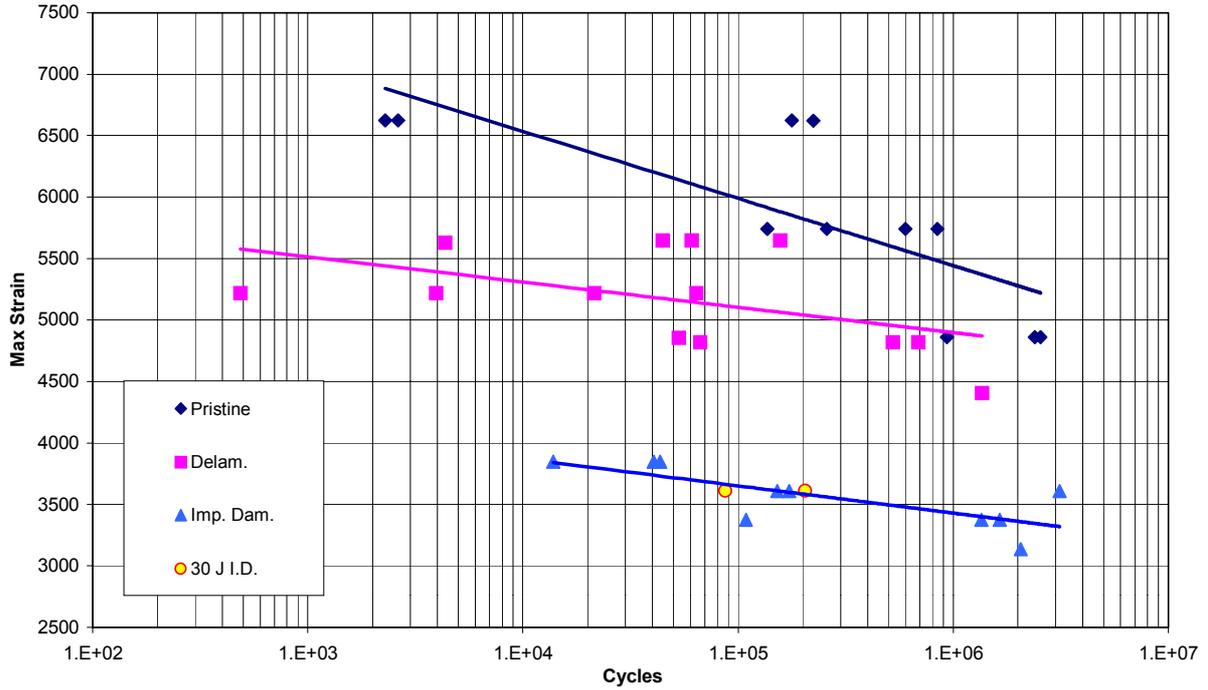
Fig. 17 – Results of fatigue tests of composite sandwich panels tested in FPB (R=5).
