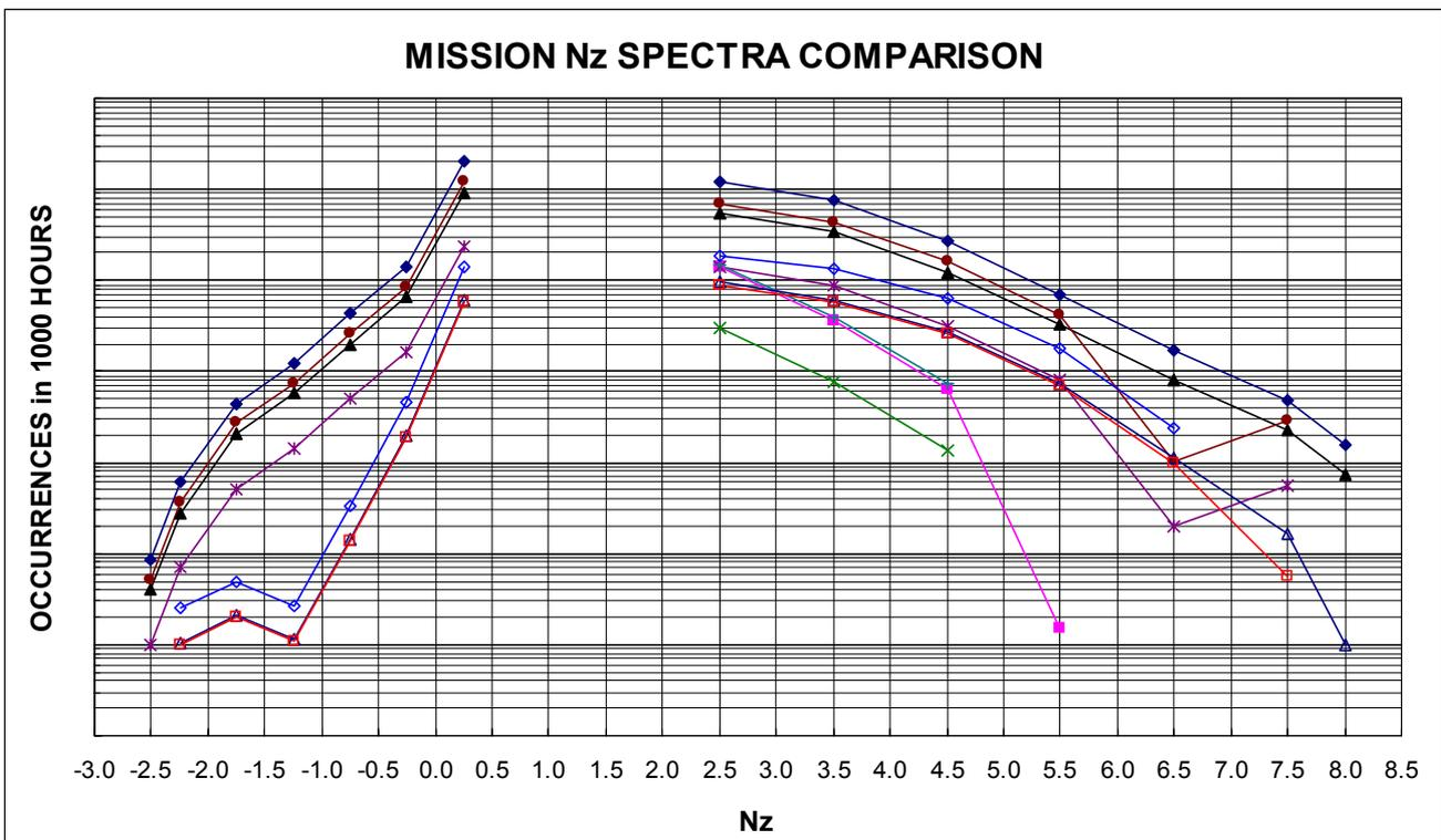
Figure 4 –  $N_z$  spectra developed for different M-346 aircraft missions.
