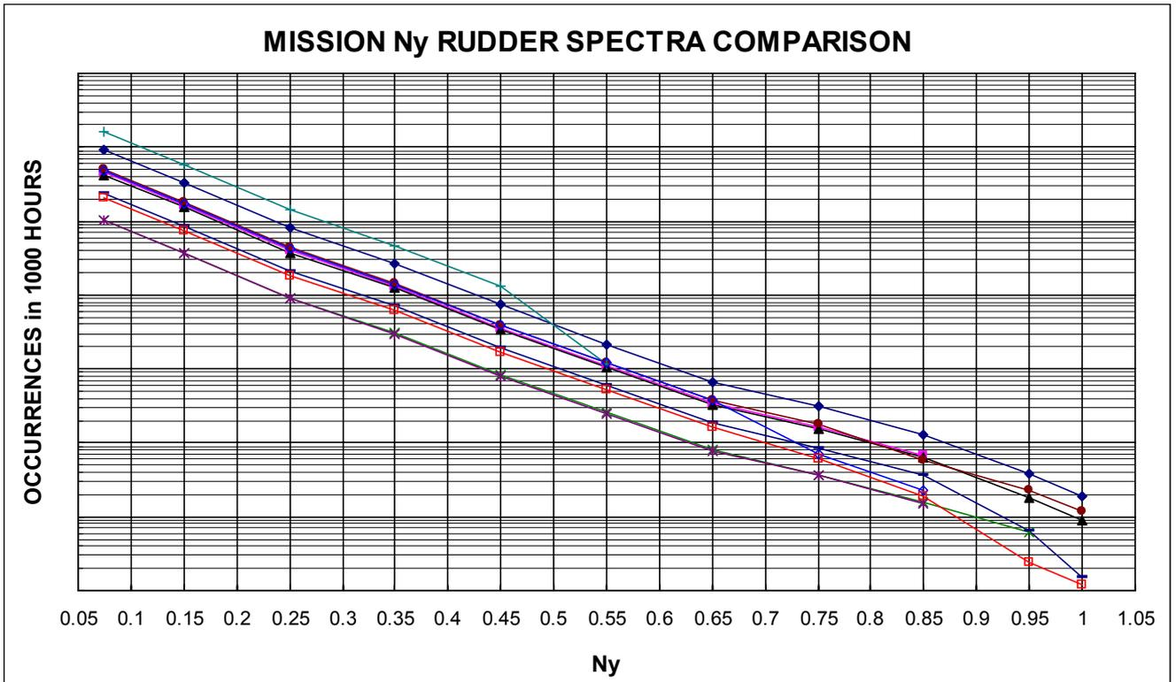
Figure 5 – Ny spectra developed for different M-346 aircraft missions.
