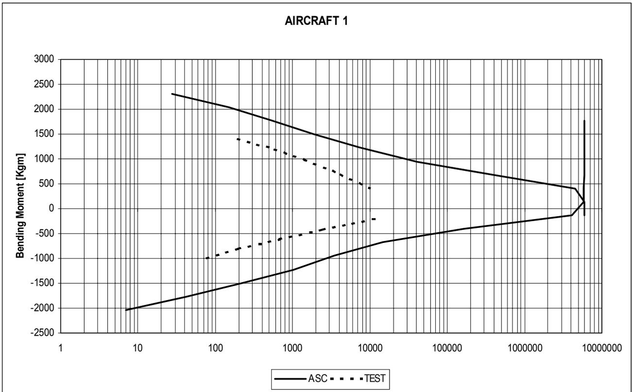
Figure 1 – Example of fin root bending moment spectra for MB-339CD aircraft.
