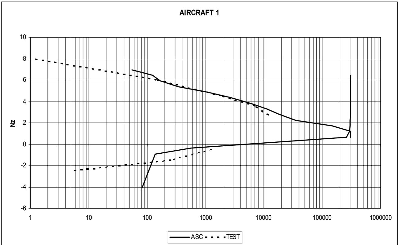
Figure 3 – Vertical load factor ( $N_z$ ) spectrum for MB-339CD aircraft.
