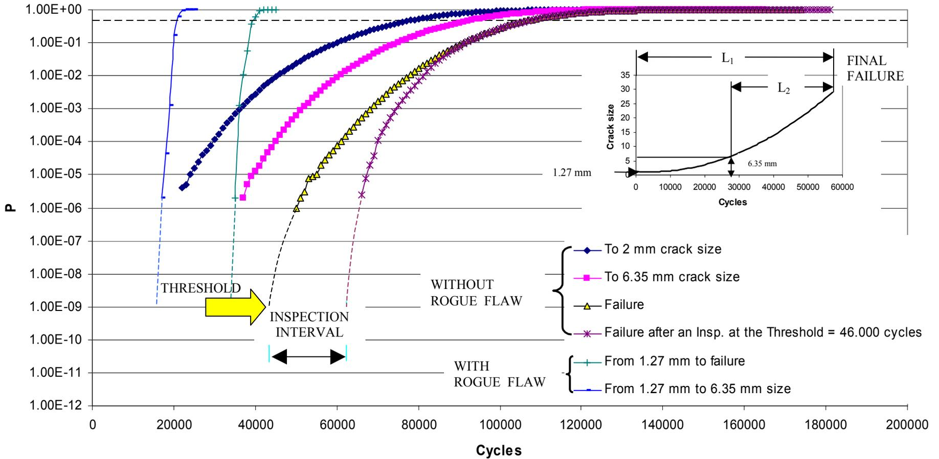
Fig. 19 – Strategy for definition of the threshold inspection
