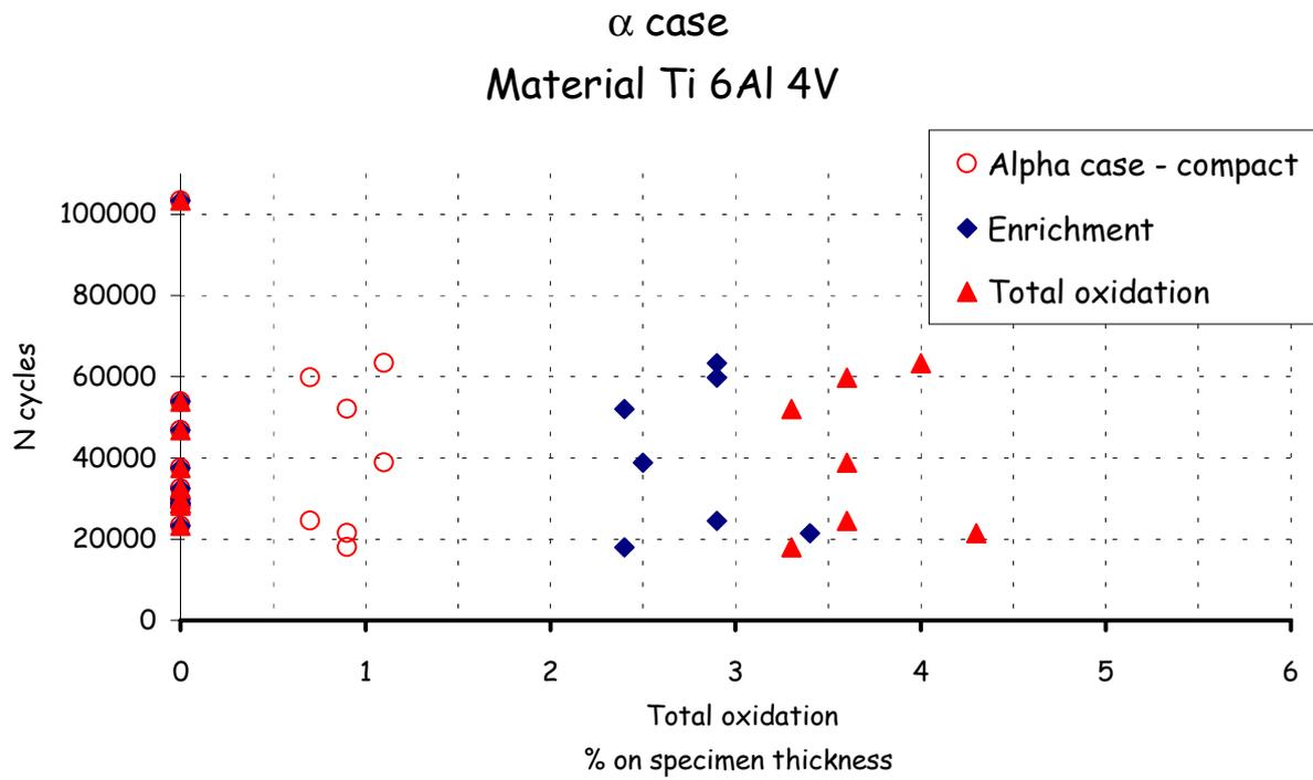
Fig. 9 – Fatigue test results of coupons with different alpha phase presence, SPF Ti-6Al-4V.
