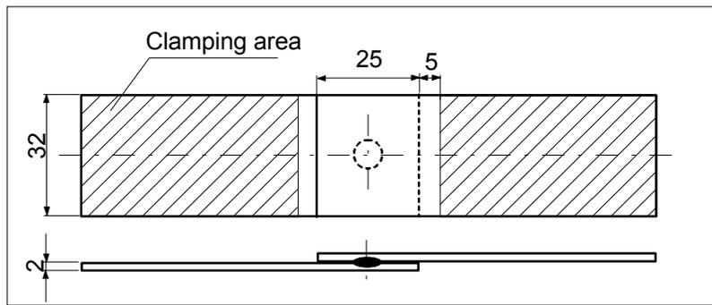
Fig. 28 – Spot-weld specimen.
