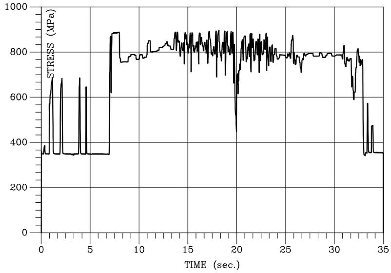
**Fig. 13 - Part of the AMX turbine load spectrum.**
