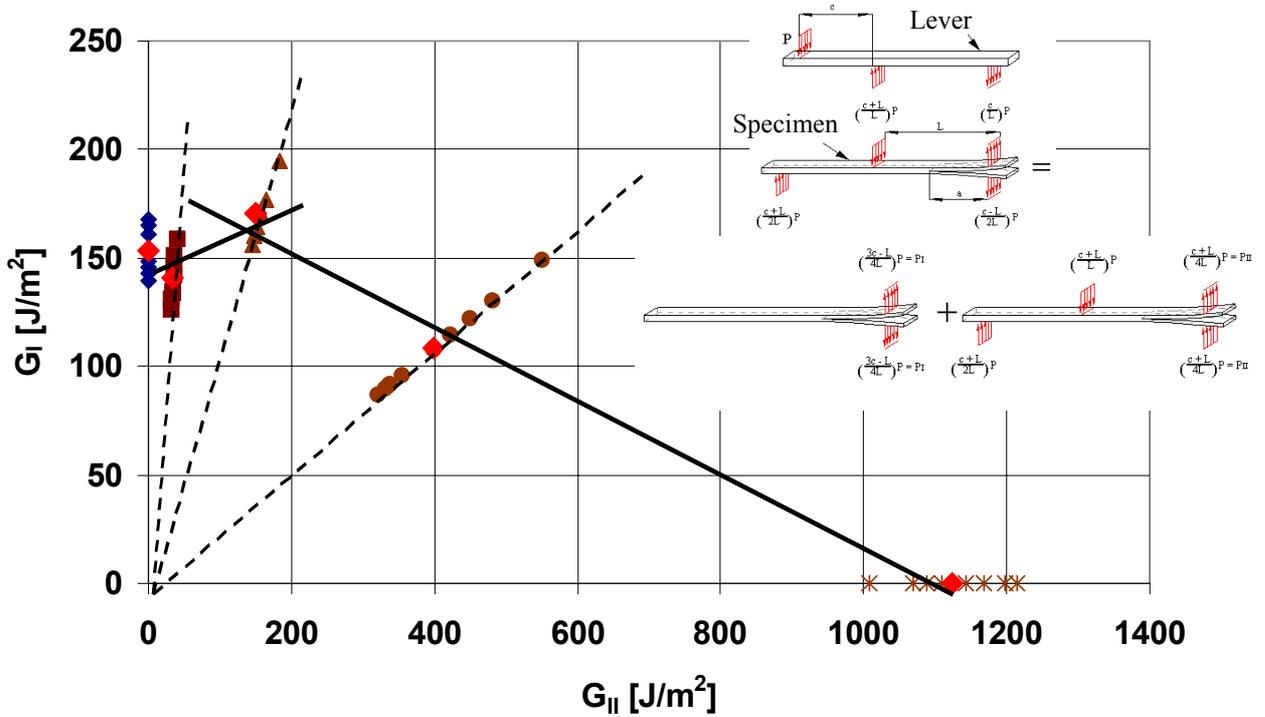
**Fig. 16 – Results of mixed mode tests for interlaminar fracture toughness of Cyanamid 985-GT6-135.**
