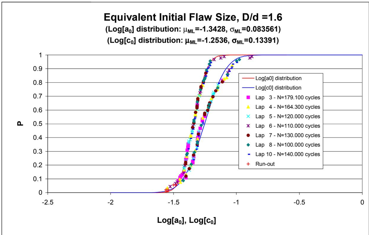
Fig. 20 – Equivalent Initial Flaw Size distribution from fractographic examination of lap joints fracture surfaces, (2024-T3, constant amplitude fatigue loading: S<sub>max</sub> 100 Mpa, R=0.1).
