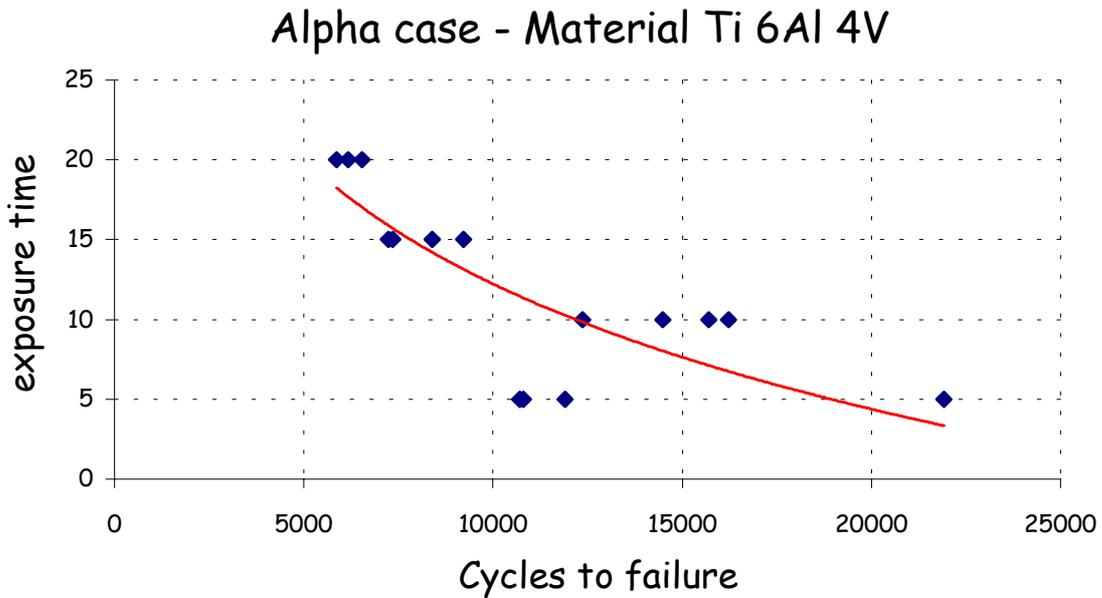
Fig. 10 – Fatigue test results of SPF Ti-6Al-4V coupons, with different exposition times at high temperature.
