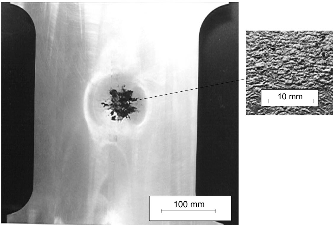
Fig. 25 – Panel in 2219-T851 after high velocity impact.
