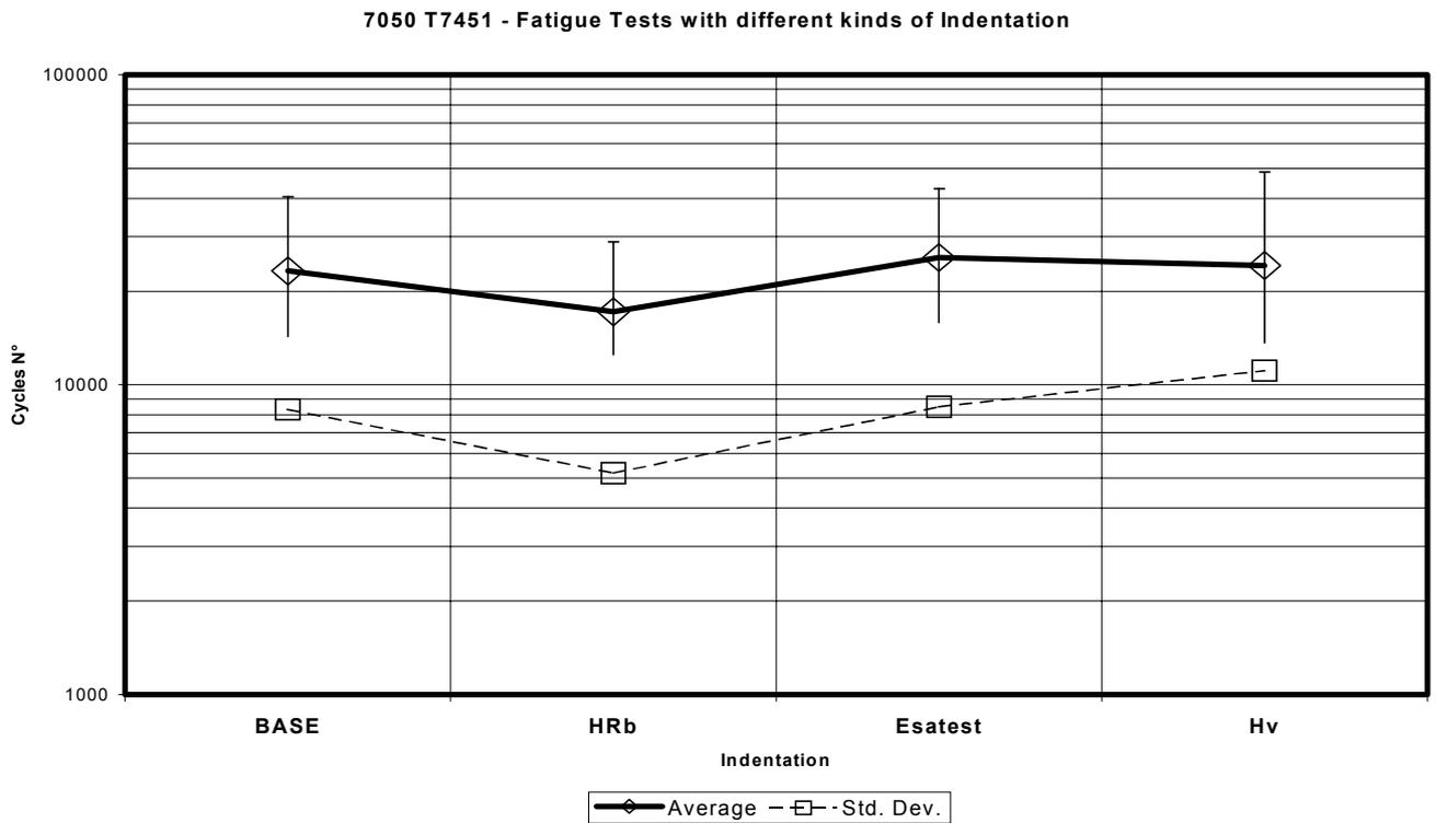
Fig. 6 – Fatigue results of smooth and indented specimens in 7050 alloy (R=0.1).
