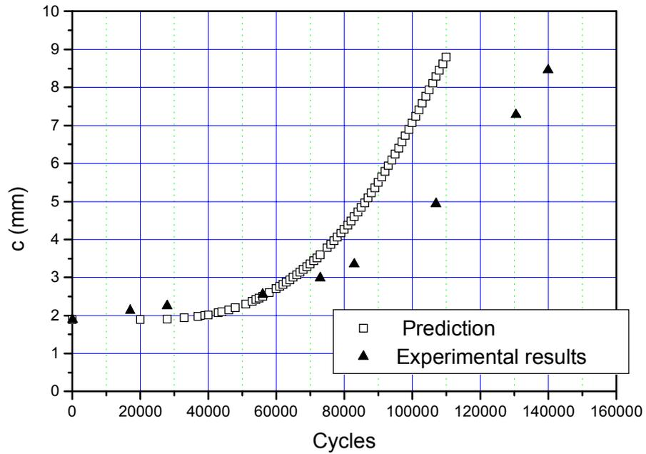
Fig. 11 – Comparison between AFGROW prediction and test data for fatigue crack growth under combined tension and bending loading.
