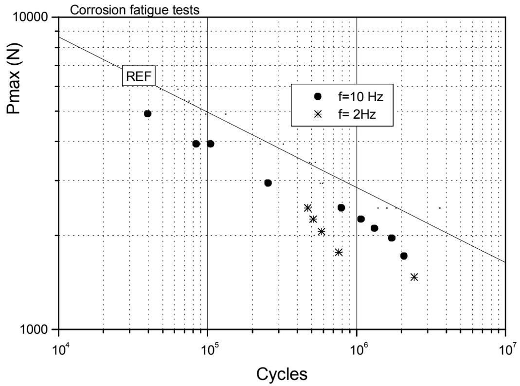
Fig. 30 – Influence of frequency on the fatigue test results in a corrosive environment.
