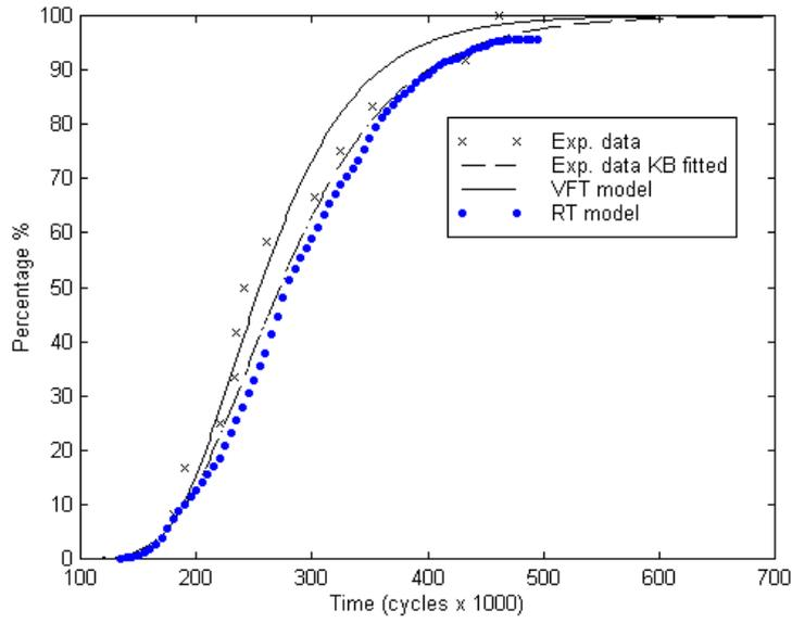
**Fig. 15 - Crack length probability versus time.**
