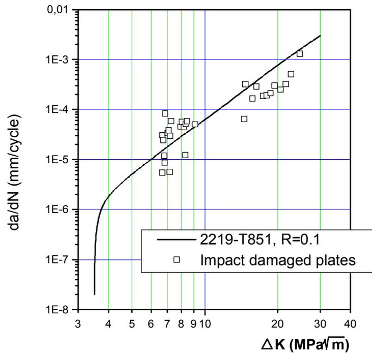
Fig. 27 – Comparison between base metal and impact damaged plates, keeping secondary bending into account in the K expression.
