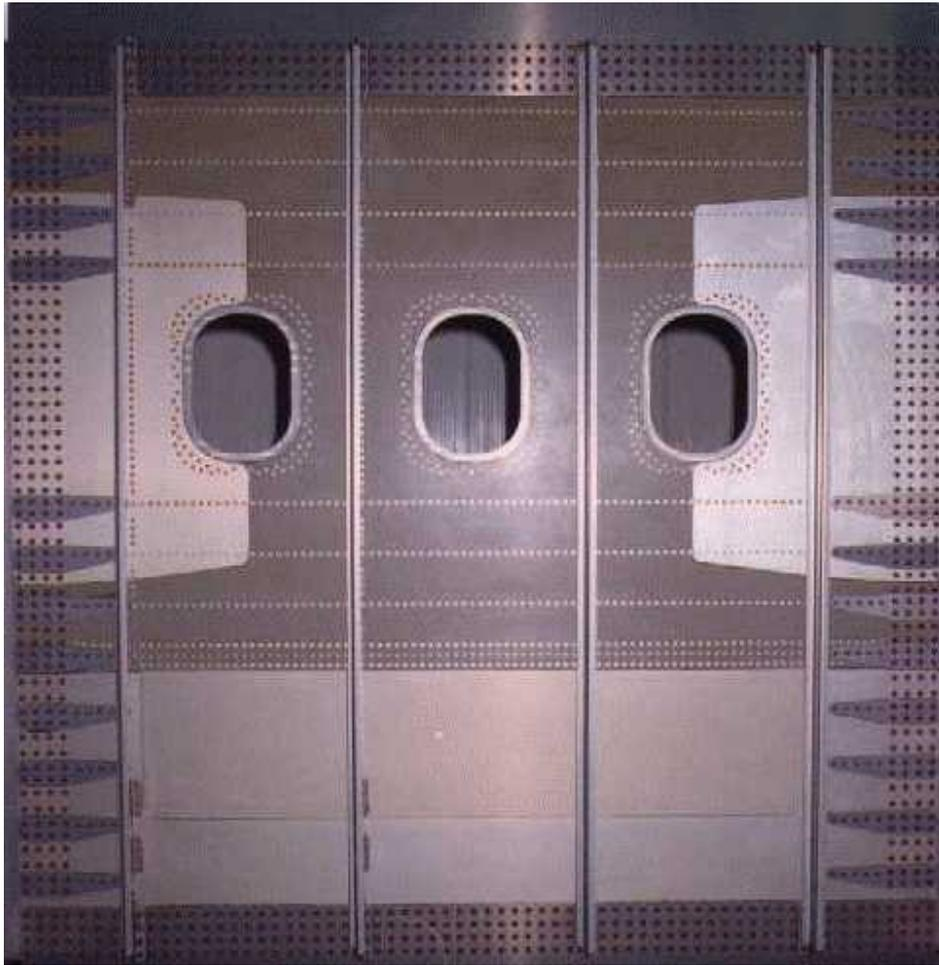
**Fig. 21 – Fuselage side panel manufactured in Glare.**
