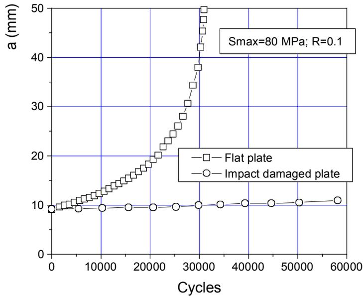
Fig. 26 – Fatigue crack growth results, for a defect at the centre of the bump.
