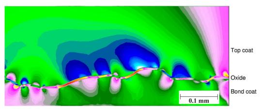
Figure 9. Contour plot of strains in 1.0 mm top coat near free edge (located at the righthand side of the plot) during simulation.
