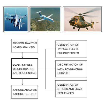
Figure 1. Phases in the aircraft loads and fatigue analysis process
