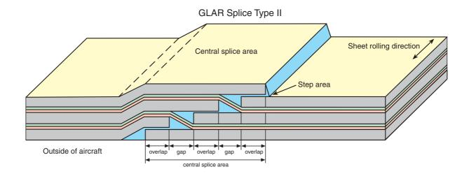
Figure 7. CLARE splice configuration
