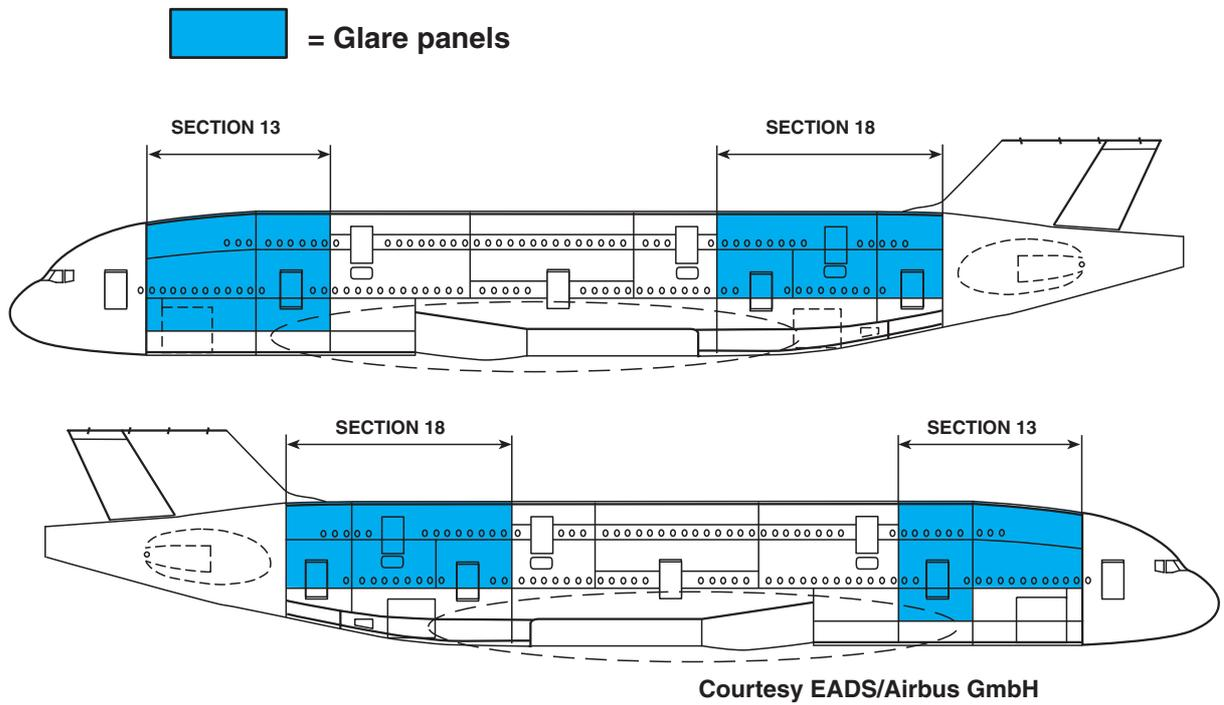
Figure 5. Application of Glare on the Airbus A380
