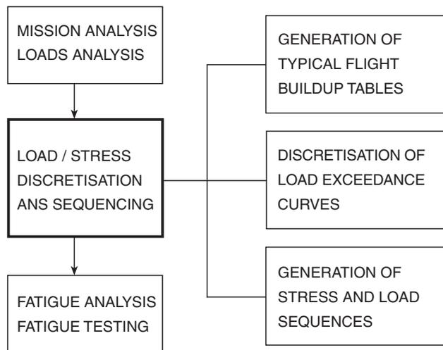
Figure 1. Phases in the aircraft loads and fatigue analysis process
