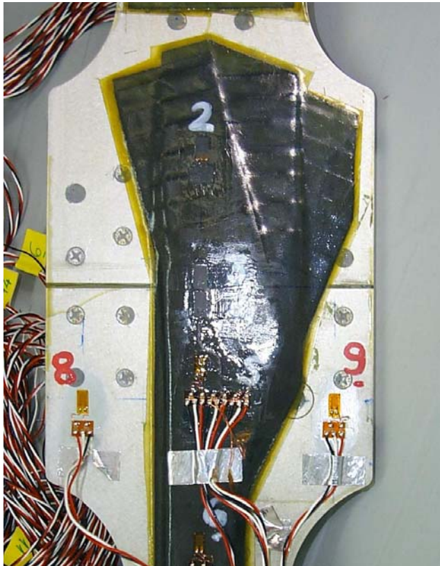
Figure 10: Static test specimen before and after failure
