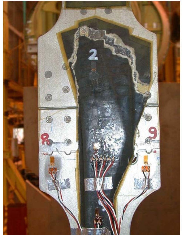
Figure 10: Static test specimen before and after failure
