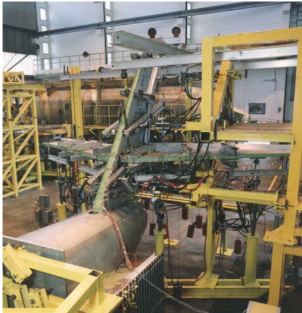
Figure 5: G200 Empennage – Fatigue and Damage-Tolerance Test
