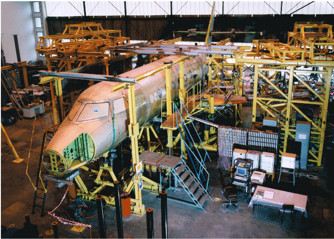
Figure 4: G200 Full-Scale Fatigue Test Aircraft
