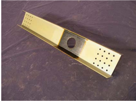
Figure 11: Typical Bonded Composite Repair that was Experimentally Evaluated
