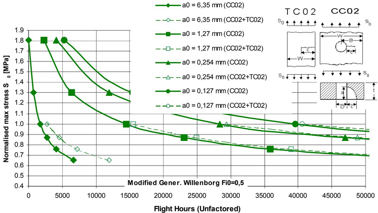
Fig. 41 – Example of damage tolerance design curve for a critical detail of the M346 trainer.
