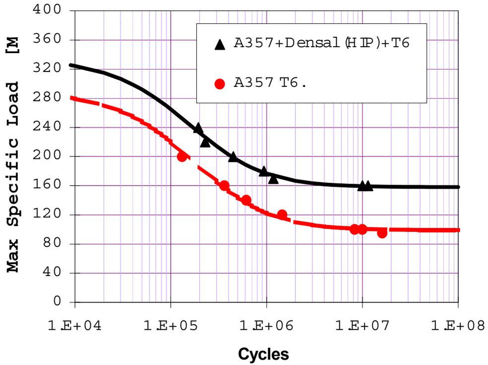
Fig. 9 – Effect of HIP treatment on S-N curves relevant to A357 specimens, cut from cast rods.
