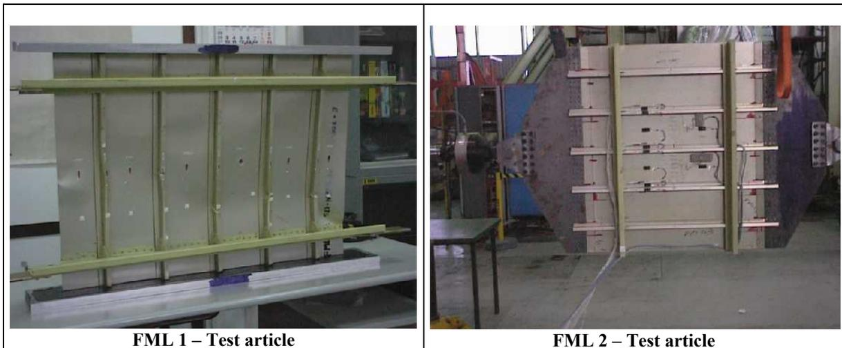
Fig. 27 - TANGO development phase test articles, manufactured by Alenia.
