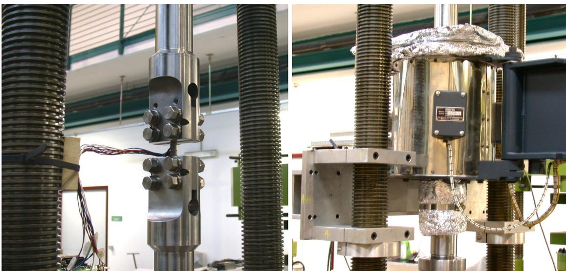
Fig. 31 - Loading bars and grips (a) and resistance furnace (b) of the test set-up for carrying out fatigue tests at high temperature (500 °C).
