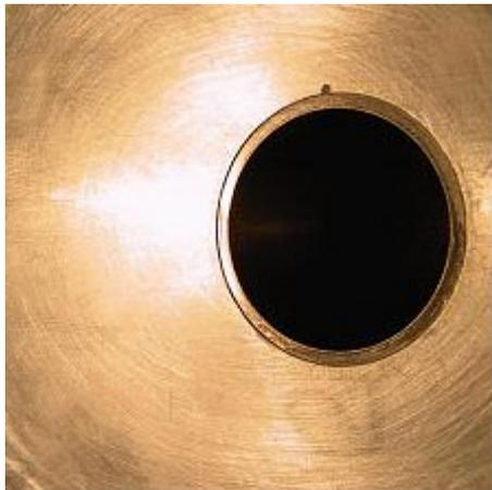
Fig. 15 - Example of the defects introduced into the specimens for a first Damage Tolerance assessment of M346 wing-to-fuselage attachment. The photo is deformed by the fish-eye lens.
