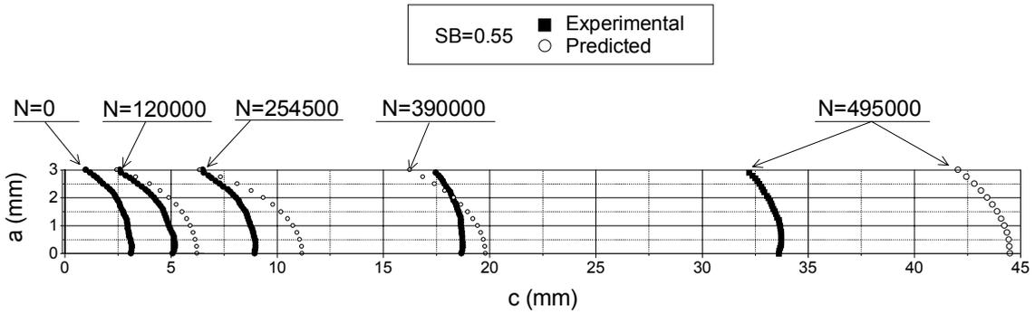
Fig. 22 – Comparison of experimental vs. predicted evolution of crack front under combined tension and bending stresses.
