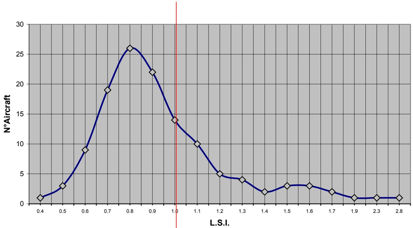
Fig. 1 – Load Severity Index distribution for the AM-X fleet.
