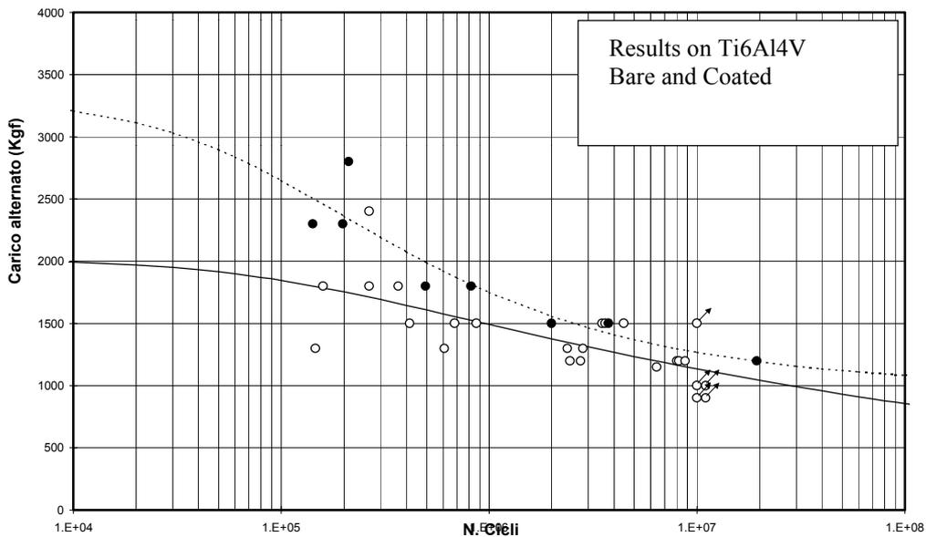
Fig. 14 - Fatigue S-N curves and experimental points relevant to non coated (solid circles/ dashed line) and coated (open circles/solid line). Tests were run at variable R: fixed static load of 2500 Kg<sub>r</sub> and various alternating loads as shown on the Y-Axis
