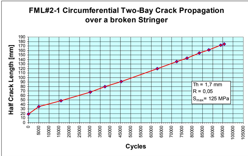
Fig. 28 – Results of a TANGO development test. Fatigue crack growth in a stiffened panel (Alenia).
