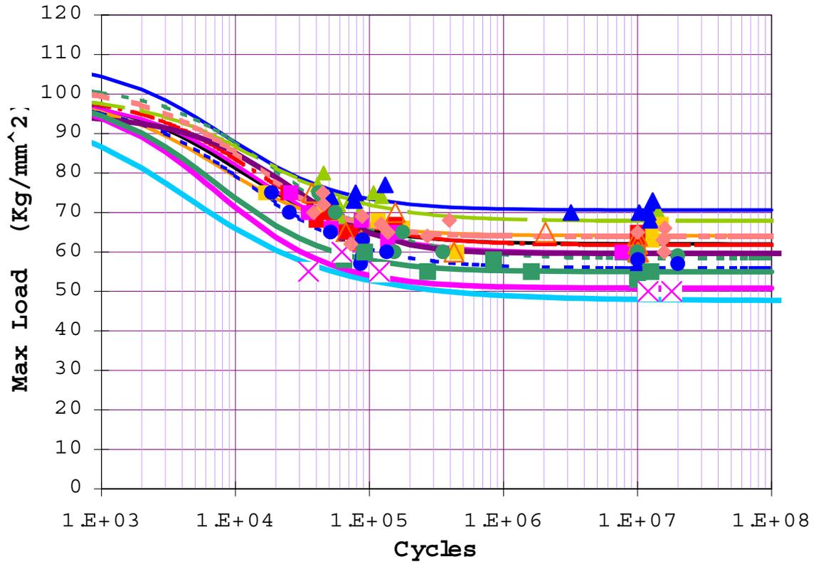
Fig. 11 – S-N curves for different batches of AISI 301 stainless steel, R=0.1, unnotched.
