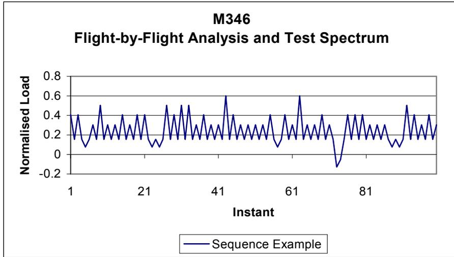
Fig. 24b – Detail of the Flight by Flight M346 wing sequence.
