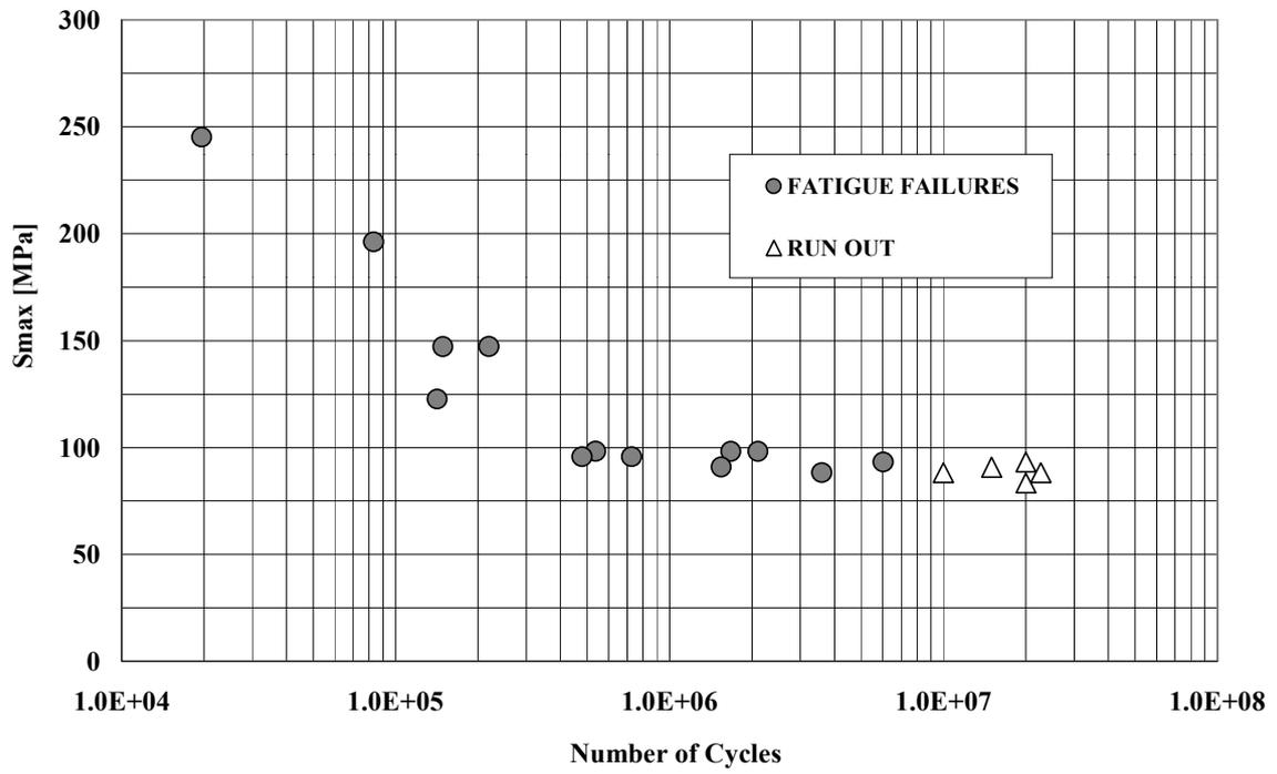
Fig. 7 – Fatigue test results of unnotched coupons of micro cast A357 alloy (R=0.1)
