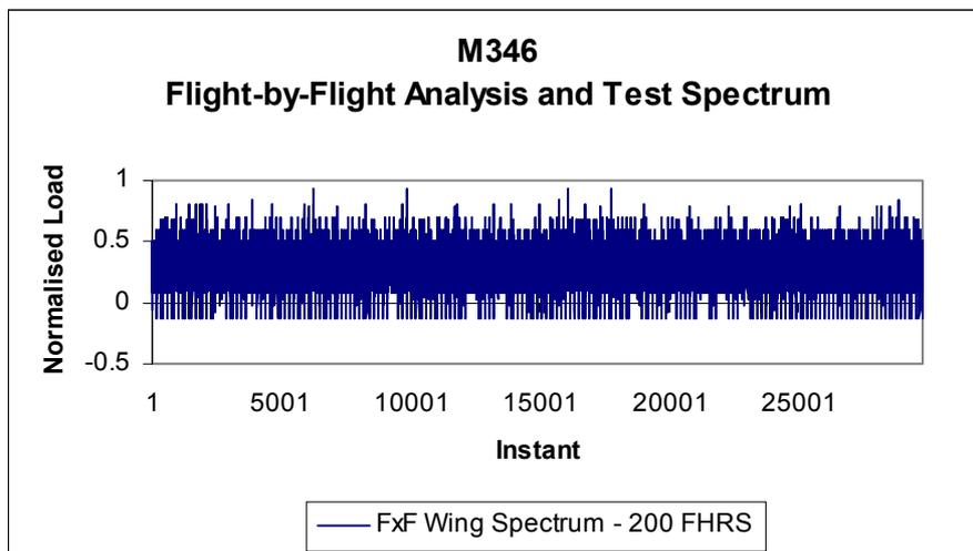
Fig. 24a – Flight by Flight M346 wing spectrum (200 flight hours)
