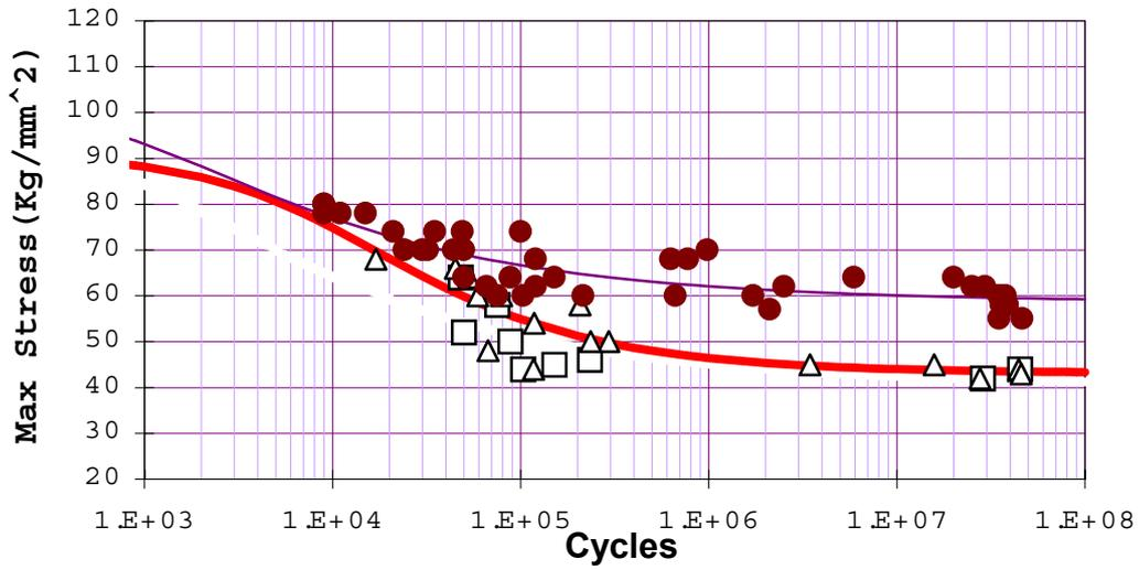
Fig. 13 – Comparison of fatigue results from Ti-6Al-4V (ELI) annealed (triangle), with Beta Solution Treated and OverAged (solid symbols). The open square symbol refers to BSTOA condition applied to a blank of excessive thickness.
