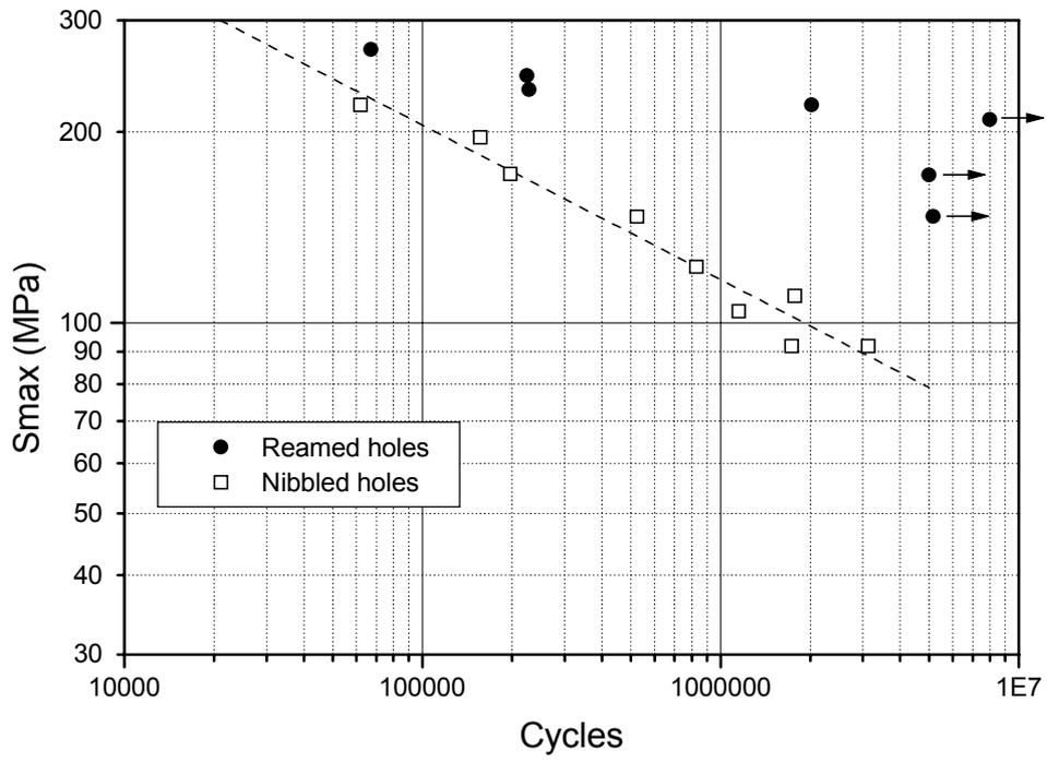
**Fig. 44 – Comparison of fatigue test results from open hole specimens in AISI 304, R=0.02; effect of the hole manufacturing technology**
