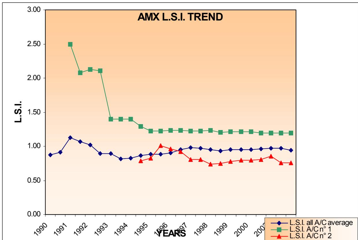
Fig. 2 – Examples of different fatigue life consumption rate for different AM-X aircraft.
