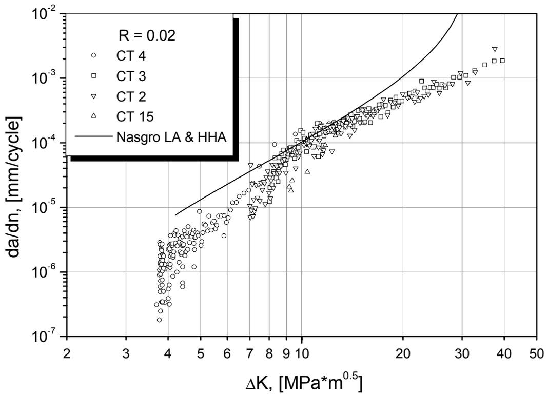
Fig. 23 – Fatigue crack growth results for 7050-T7451, thickness 42 mm.
