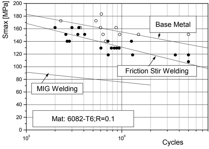
Fig. 42 – Results of fatigue tests on FSW butt joints in 6082-T6.
