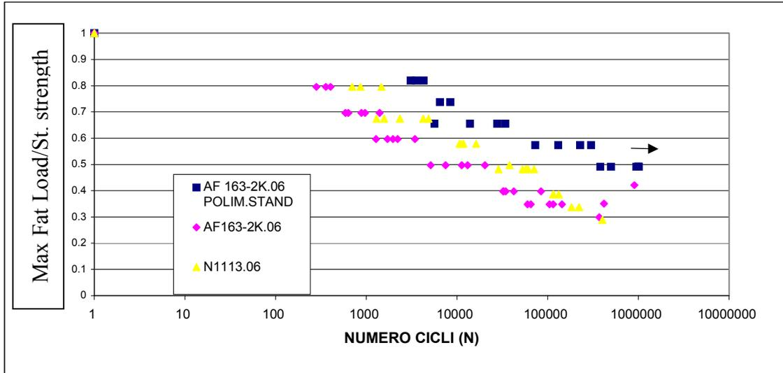
Fig. 26 - Fatigue test results from adhesive bonded single lap joints, obtained with various curing variants. Black square refer to Standard curing, triangles and diamonds data points refer to two different adhesives and curing at lower temperature.
