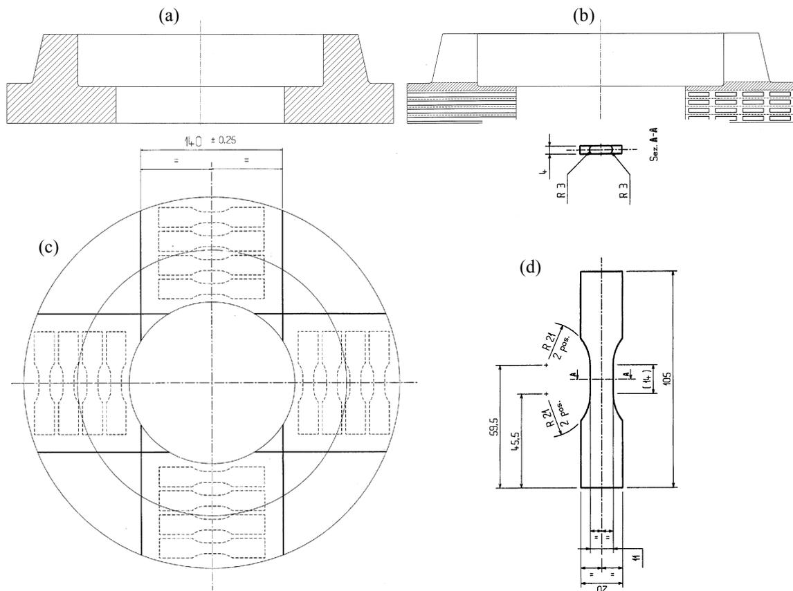
Fig. 30 – Specimen machining from IN718 disc forging for the MANHIRP program.
