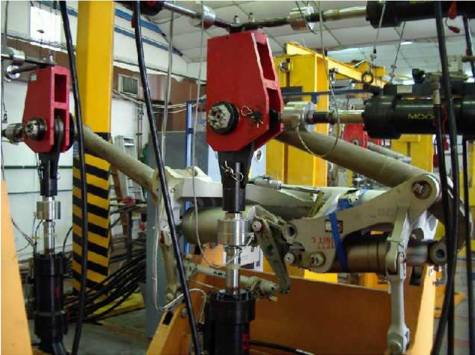
**Fig. 38 – C 27-J Main Landing Gear test set-up.**
