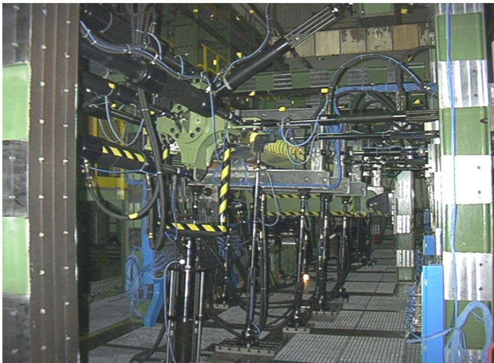
**Fig. 39 – BA609 Tiltrotor: wing fatigue test set-up.**
