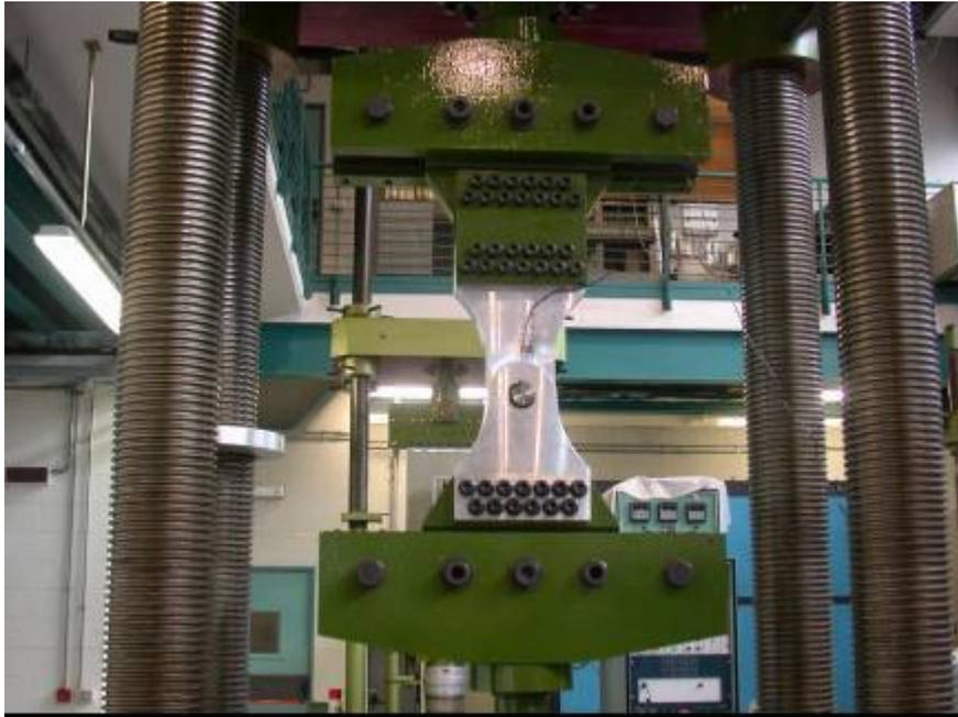
**Fig. 16 - One of the 14 joint specimens available assembled on the test machine. The geometry of this specimen is representative of the M346 wing-to-fuselage attachment lugs.**
