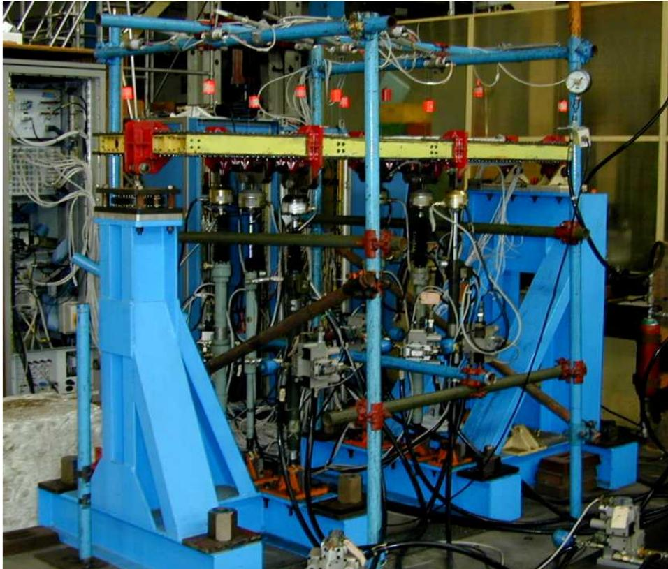
**Fig. 35 – EF Typhoon: fatigue test of the outboard region pressure box**
