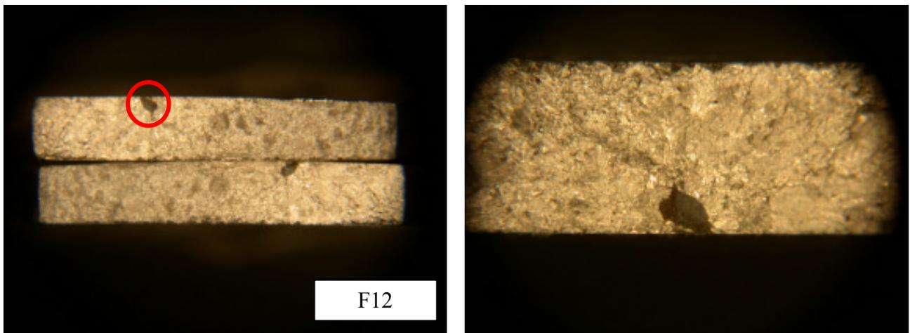
Fig. 8 – Evidence of defects, due to micro casting, in A357 material.
