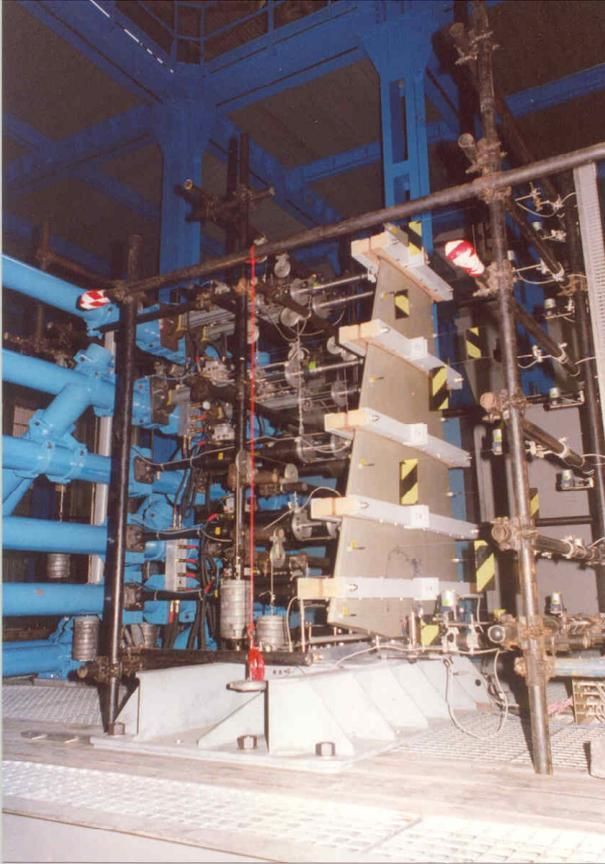
**Fig. 32 – Test rig for the M346 Horizontal Tail fatigue test**
