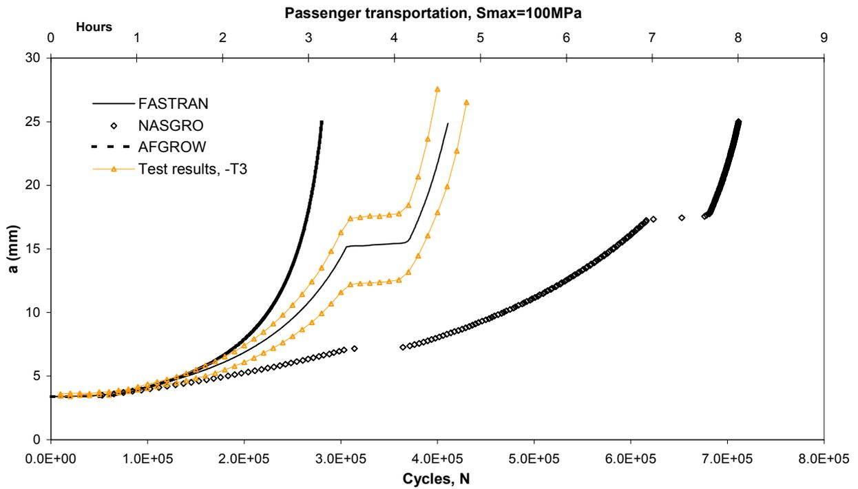
Fig. 18 – Comparison of VA test results with predictions (2024-T3, Passenger transport mission, Smax 100 MPa).
