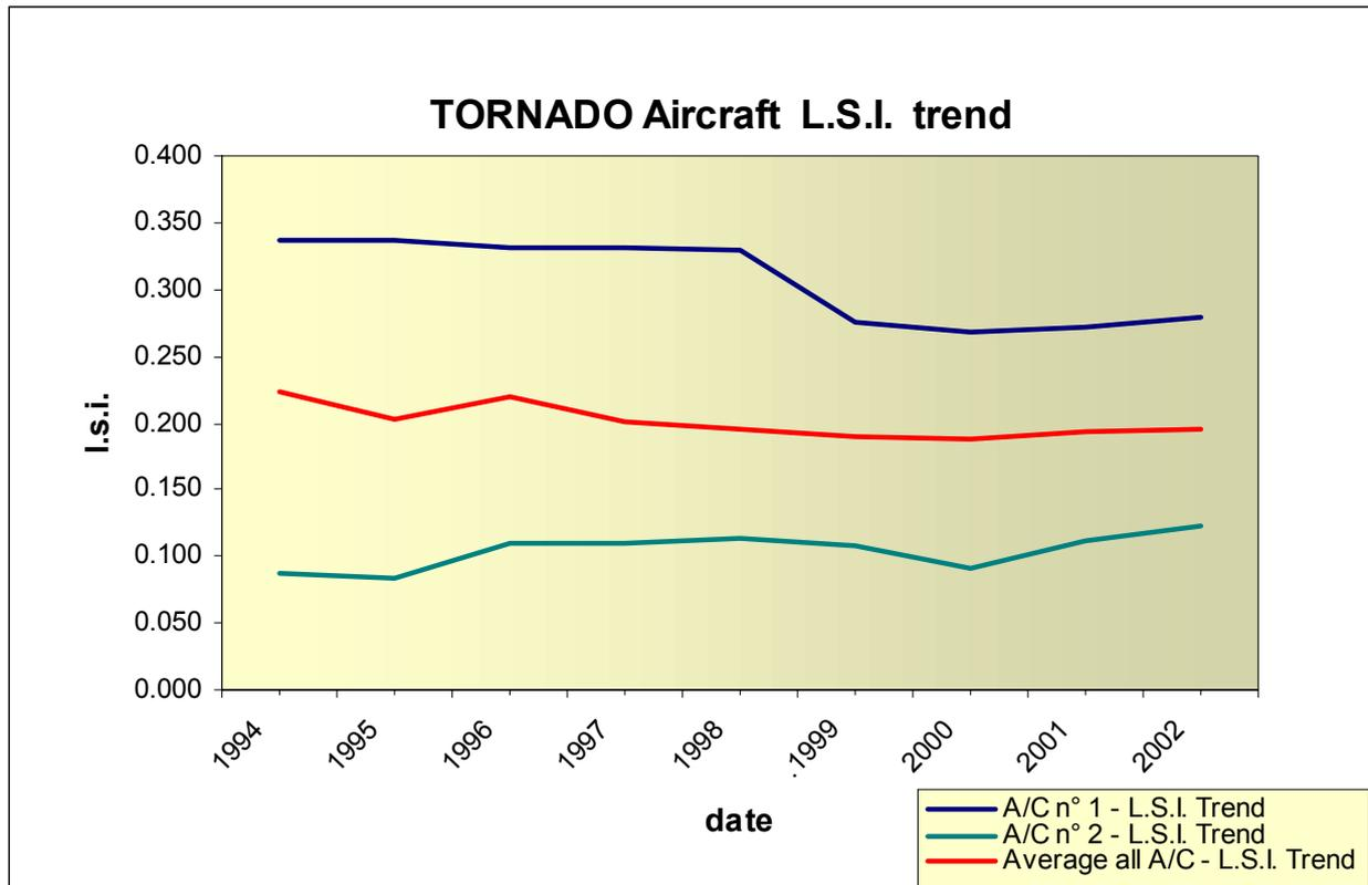
Fig. 4 – Examples of different fatigue consumption rates for individual Tornado aircraft.
