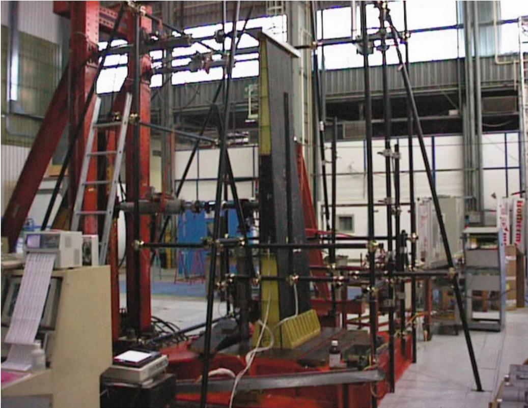
**Fig. 36 – Test set-up for the central pylon housing box of the EF Typhoon**
