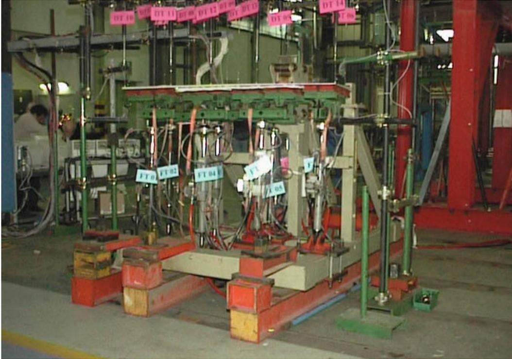
**Fig. 34 – Test set-up for the Typhoon outboard flaperon**
