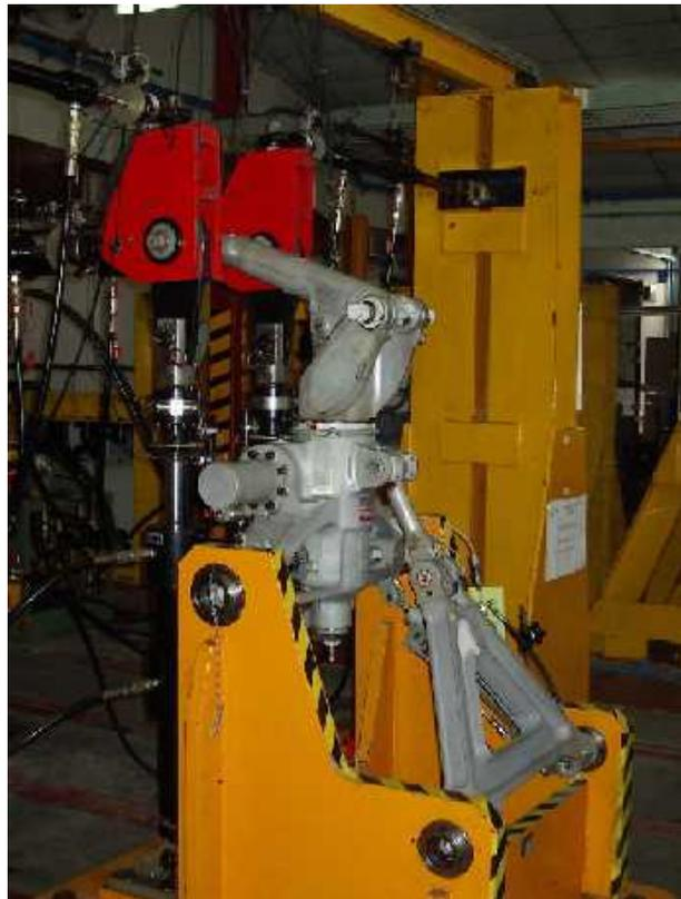
**Fig. 37 – C 27-J Nose Landing Gear fatigue test set-up.**
