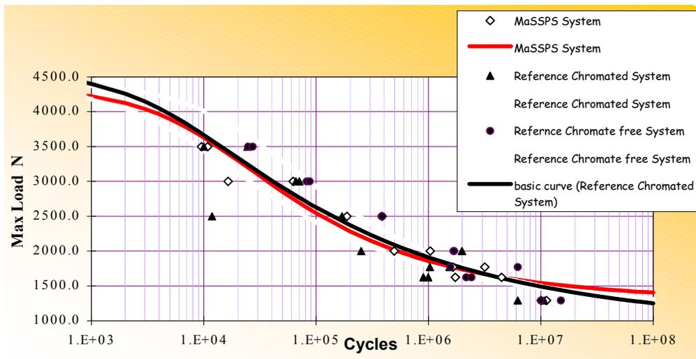
Fig. 29 – Fatigue test results after conditioning of specimens subjected to three protection systems (two chromate free and one with chromate), compared with reference results from specimens not exposed to fluids and corrosion.
