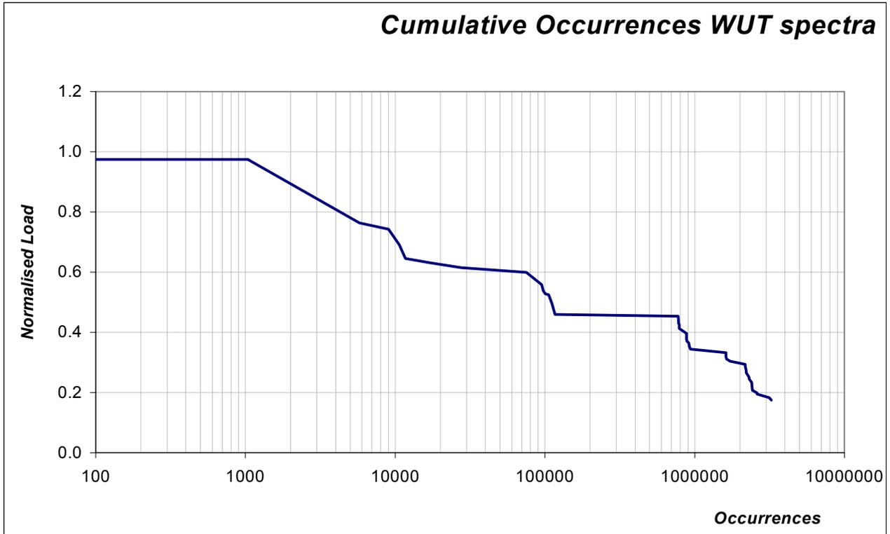
Fig. 5 – Buffet spectrum for the fin of the M346 trainer.
