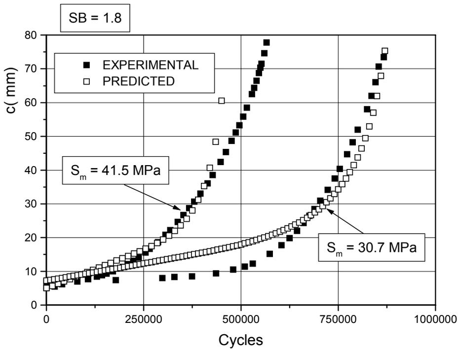
Fig. 21 – Comparison of experimental vs. predicted crack growth under combined tension and bending stresses.
