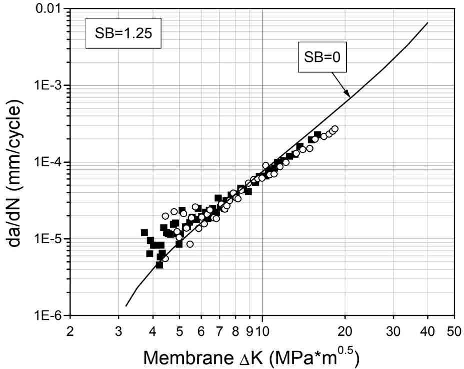
Fig. 19 – Comparison of fatigue crack growth data obtained under tension and bending loads with basic material properties. Case of low secondary bending (SB).
