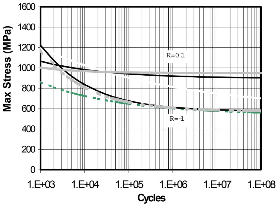
Fig. 10 – S-N curves for different nitrated steels, for two stress ratios. The green lines refer to the Al based Nitralloy (AMS 6475), while the grey and black lines refer to 32CDV13 (AMS 6481) subjected to nitriding under different process parameters.
