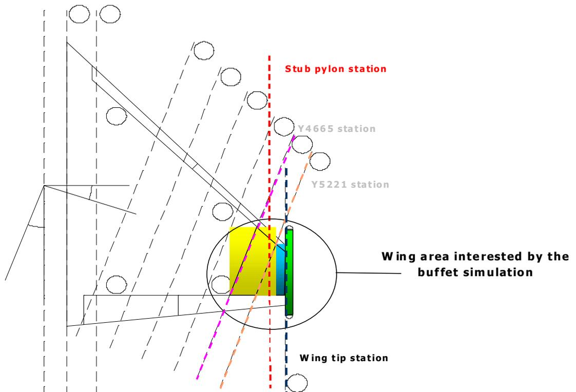
**Fig. 33 – Area of the EF Typhoon wing where the buffet loads are significant.**
