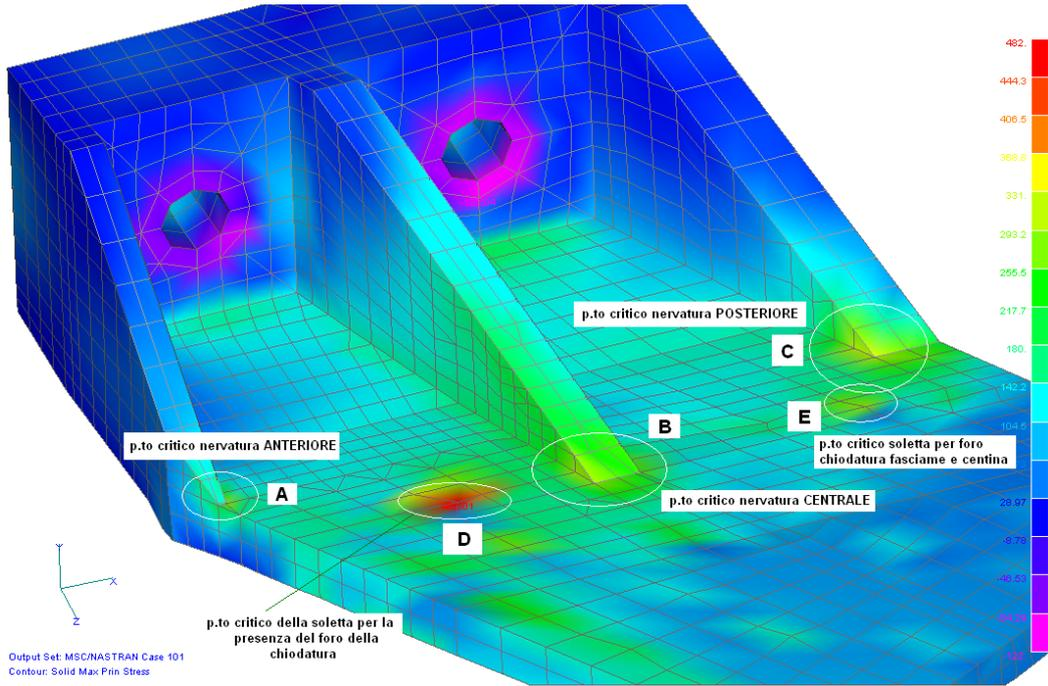
Fig. 40 – Detail of a FEM stress analysis of the fin-fuselage attachment fitting in the M346 aircraft.
