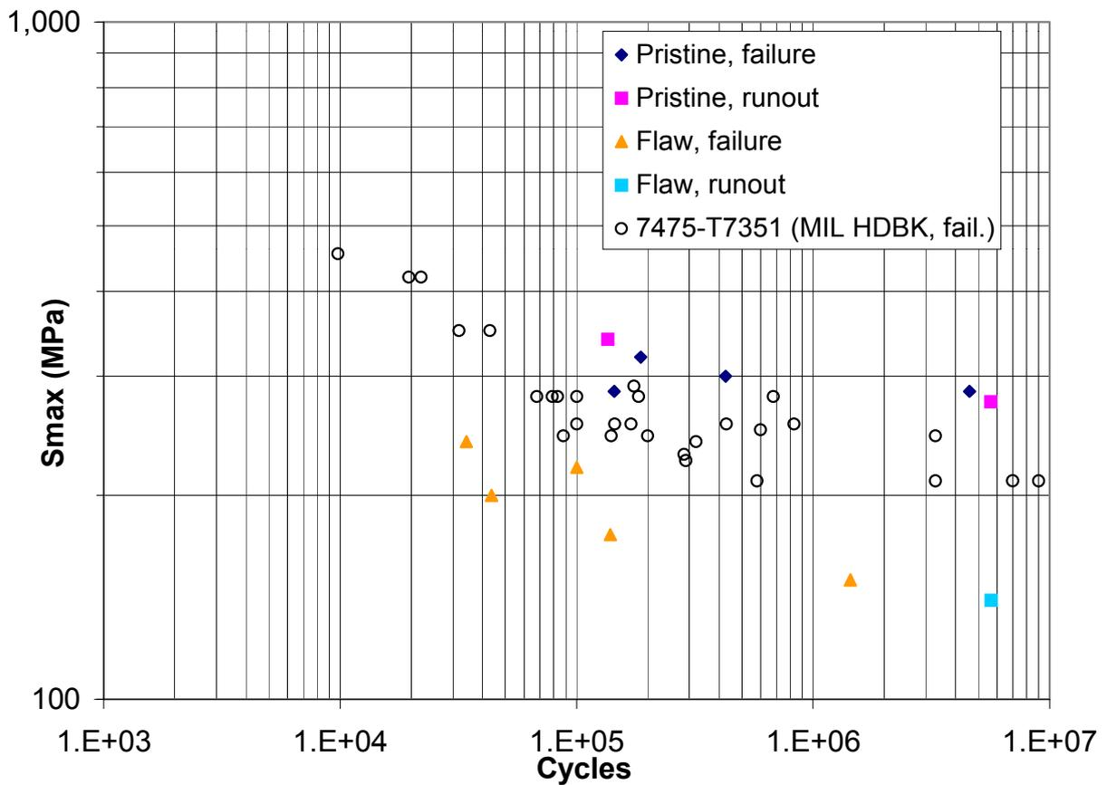
Fig. 6 – CA results for a typical fatigue critical helicopter detail, in 7475-T7351 (R=0.05).
