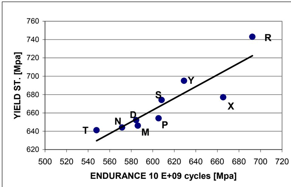
Fig. 12 – Correlation between endurance limit and yield stress for various batches of AISI 301 stainless steel, 1/4 hard.
