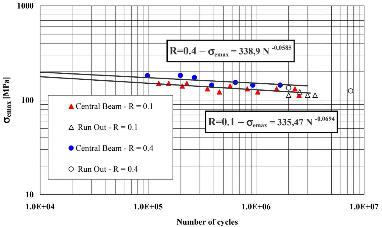
Fig. 43 – Results of fatigue tests on welded specimens made of thin steel sheets.
