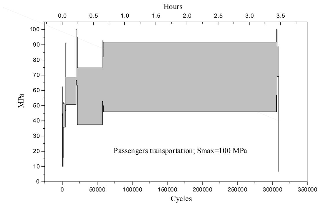
**Fig. 17 – Typical helicopter fuselage spectrum sequence.**
