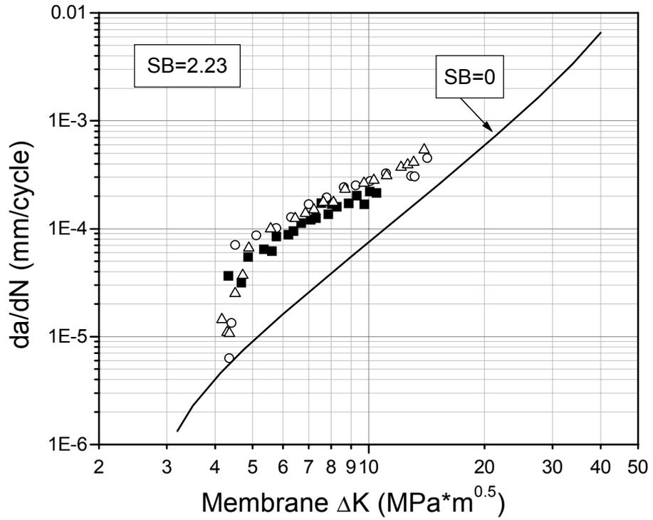
Fig. 20 – Comparison of fatigue crack growth data obtained under tension and bending loads with basic material properties. Case of high secondary bending (SB).
