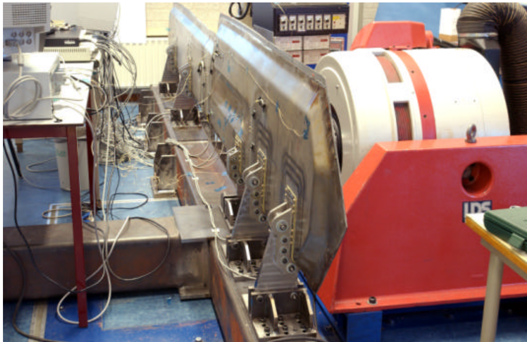
Fig. 11 Test set-up acoustic fatigue of a Fibre Metal Laminate (FML) weapon bay door (see subsection 1.6.2)
