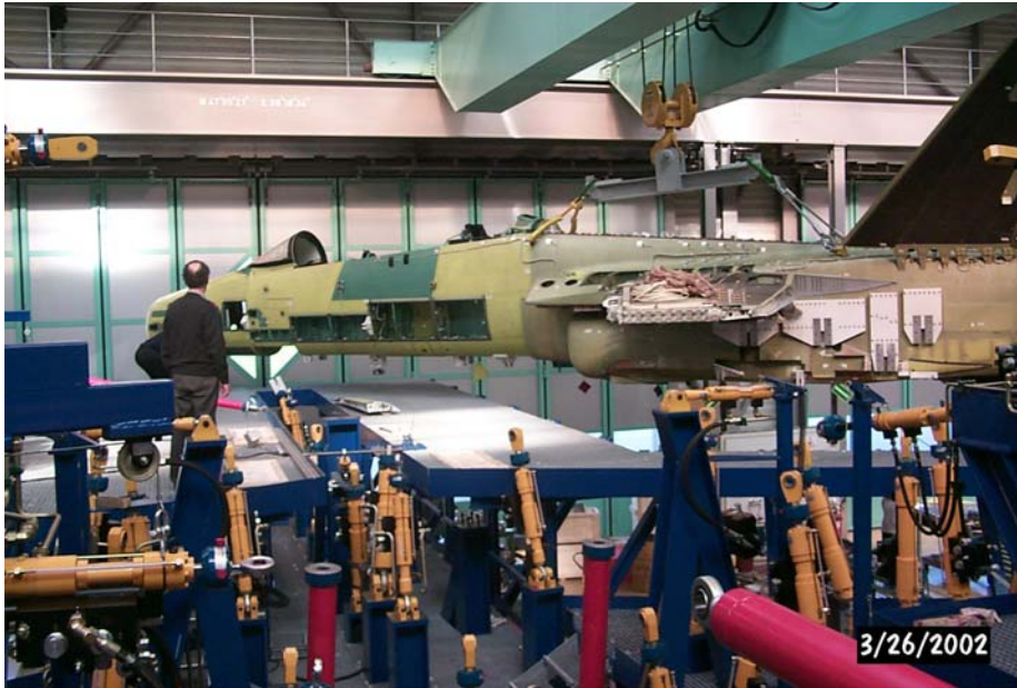
Figure 4.7_4: Lifting the test article into the rig.
