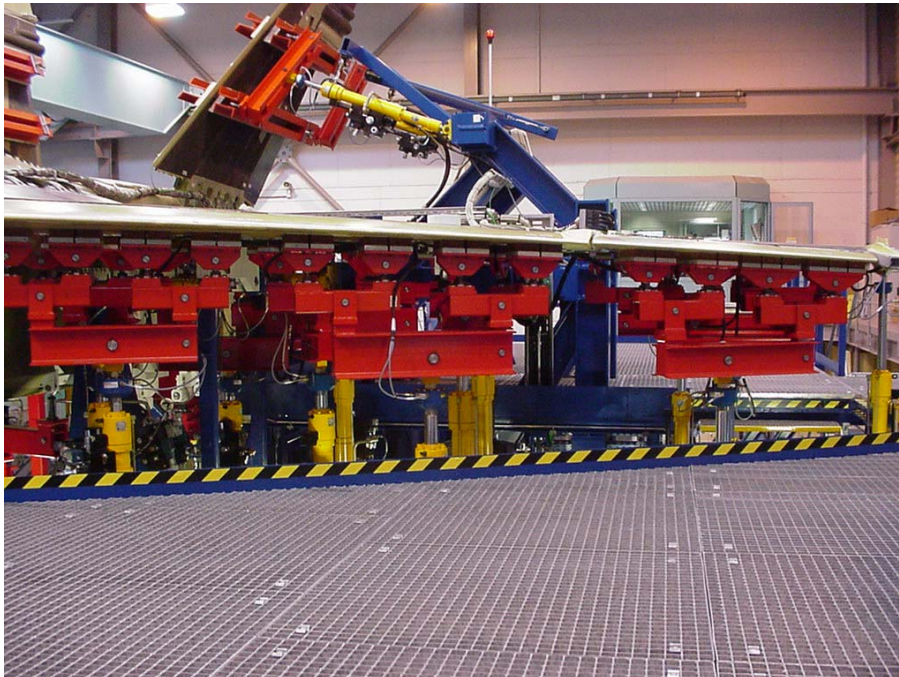
Figure 4.7_3: Wing whiffle trees to simulate distributed loads and simple vertical tail load introduction system.
