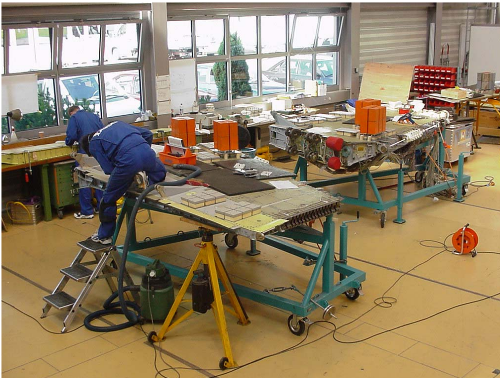
Figure 4.7_1: Pad application on the inner wing torsion box bonded by IABG
