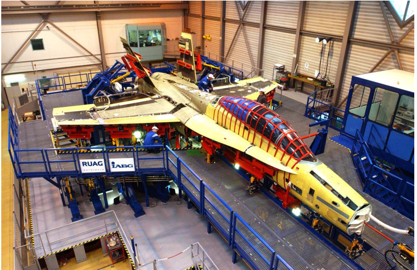
Figure 4.7_11: Test-set up during fatigue cycling at RUAG Aerospace in Emmen.
