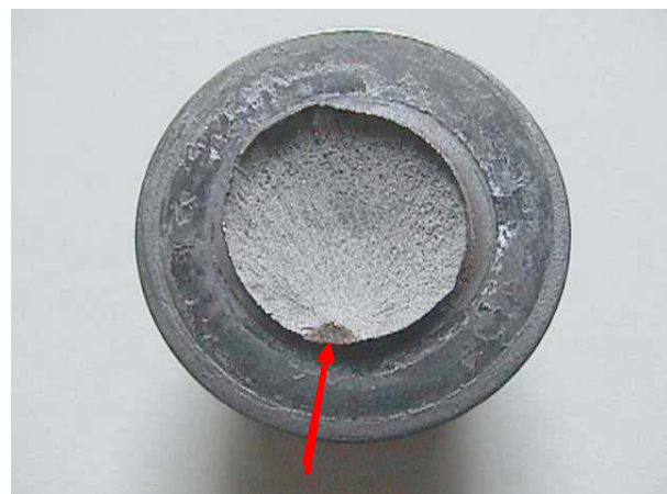
Figure 4 Failed forward attachment bolt (2 nd case). Arrow indicates the corroded crack origin.
