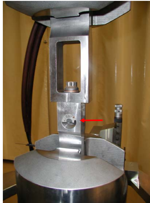
Figure 2 Crack retardation test setup for the aft location of F.S.284 splice with the test specimen at the bottom
