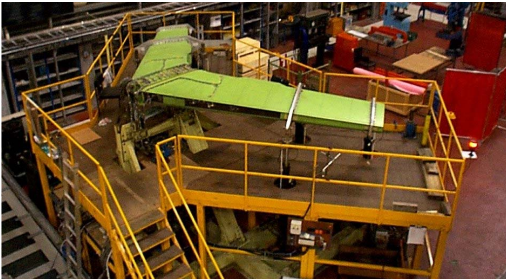
FIGURE 12 Global Express Horizontal Stabilizer Metallic Centre Box Subcomponent DADT Test
