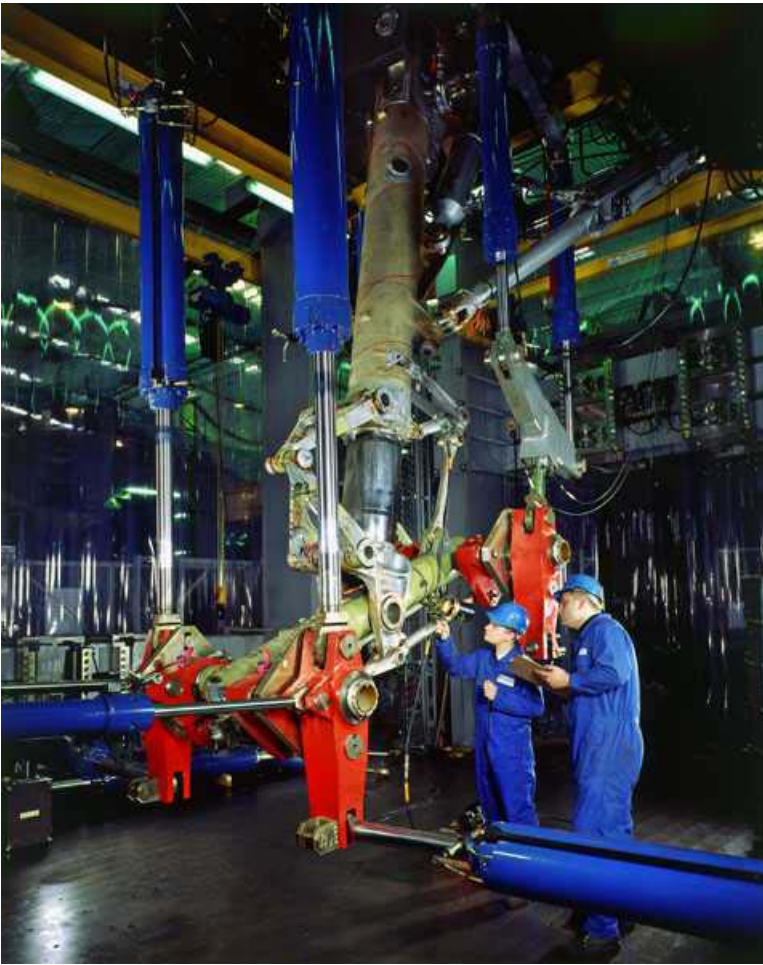
FIGURE 15 A340 landing gear fatigue test in the new test facility
