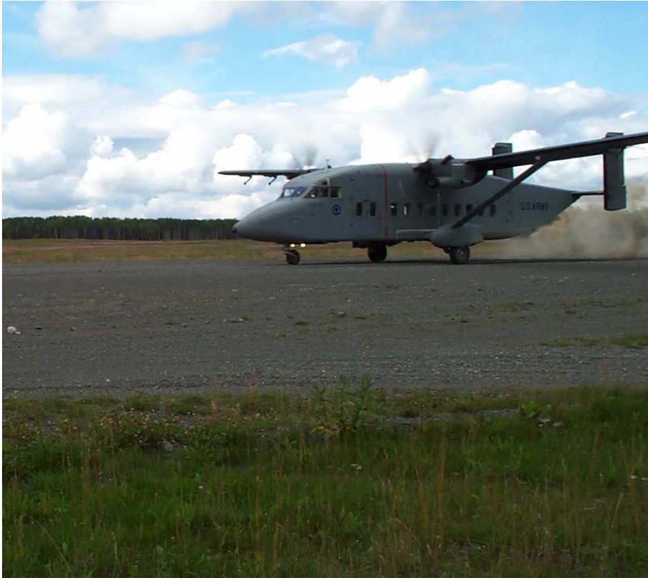
FIGURE 3 C23B/B+ Aircraft Clearance for Operation on Gravel Runways
