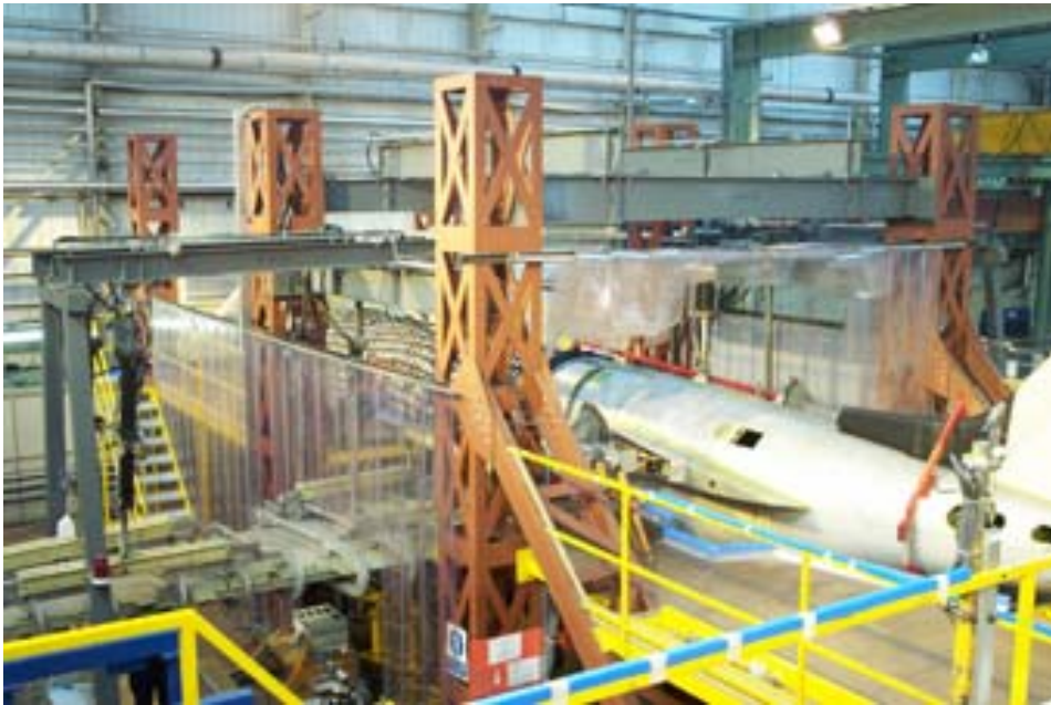
FIGURE 13 Learjet 45 wing and fuselage test article (designated TA05)
