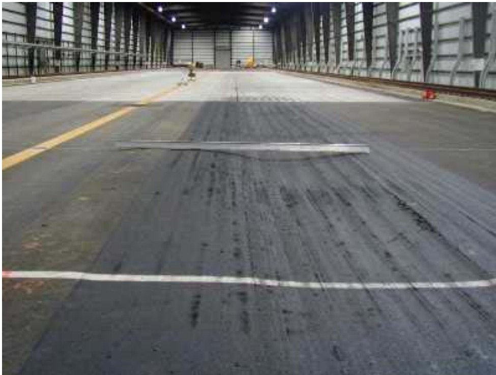
Figure 9.9.6.2 Results after repeated passes of the test vehicle
