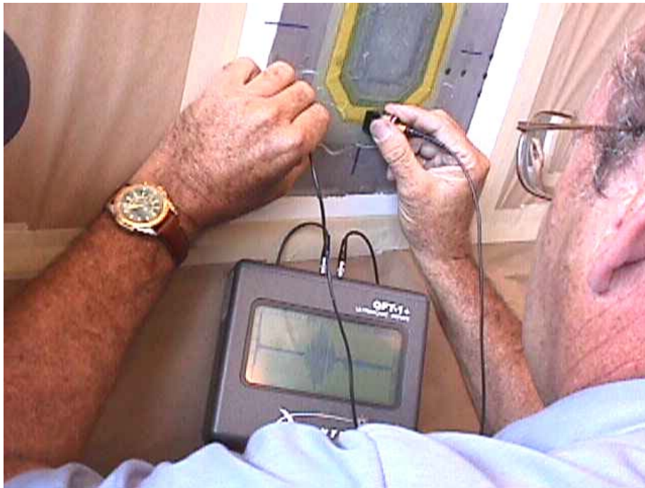
Figure 9.11.4.2 Ultrasonic inspection of repair
