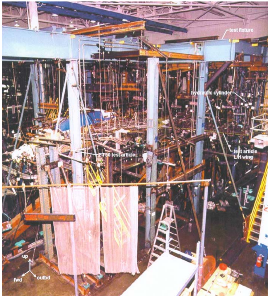
Figure 9.9.3.2 F/A-18E/F full-scale fatigue test article in the test fixture
