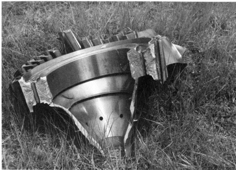
Figure 9.13.3.2 Uncontained fan disk failure due to an abusively machined bolthole
