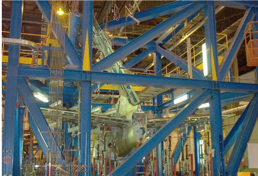
Figure 9.9.1.2 S-3B Viking empennage test airframe installed in reaction frame (vertical tail shown partially folded for inspection) – Lockheed Martin Structural Test Laboratory, Marietta, Georgia – Fatigue testing span: 13 December 2001 to 21 August 2002
