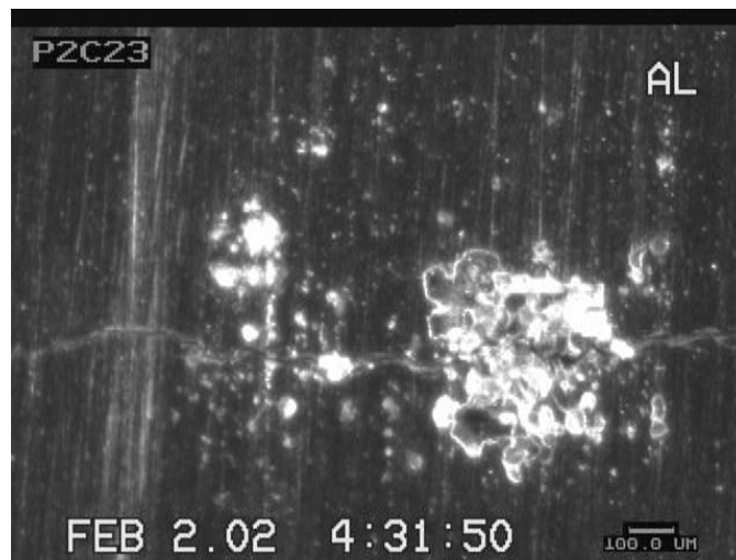
Figure 9.8.3.1 Example of crack originating at a corrosion pit
