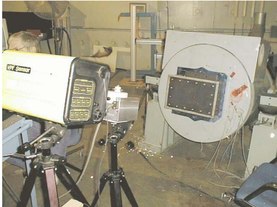
Figure 9.10.5.1 Blackglas™/Nextel 312 panel mounted to shaker for test
