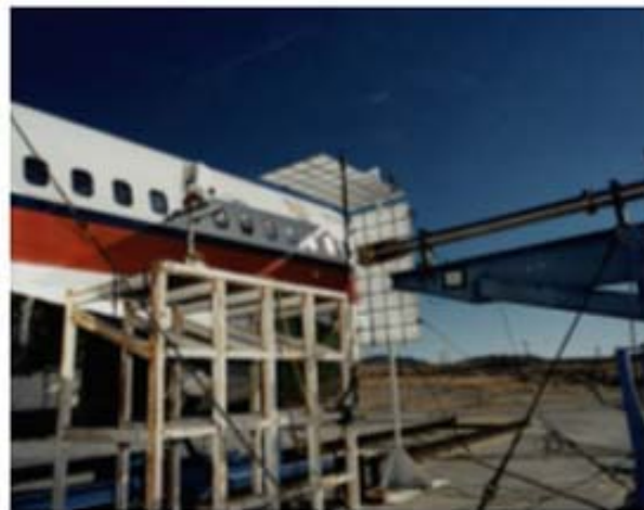
Figure 9.13.4.1 Fuselage air-gun test facility
