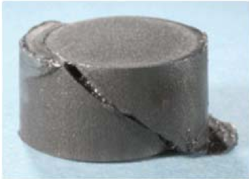
Figure 9.13.4.2 Photograph of Ti-6Al-4V sample after testing
