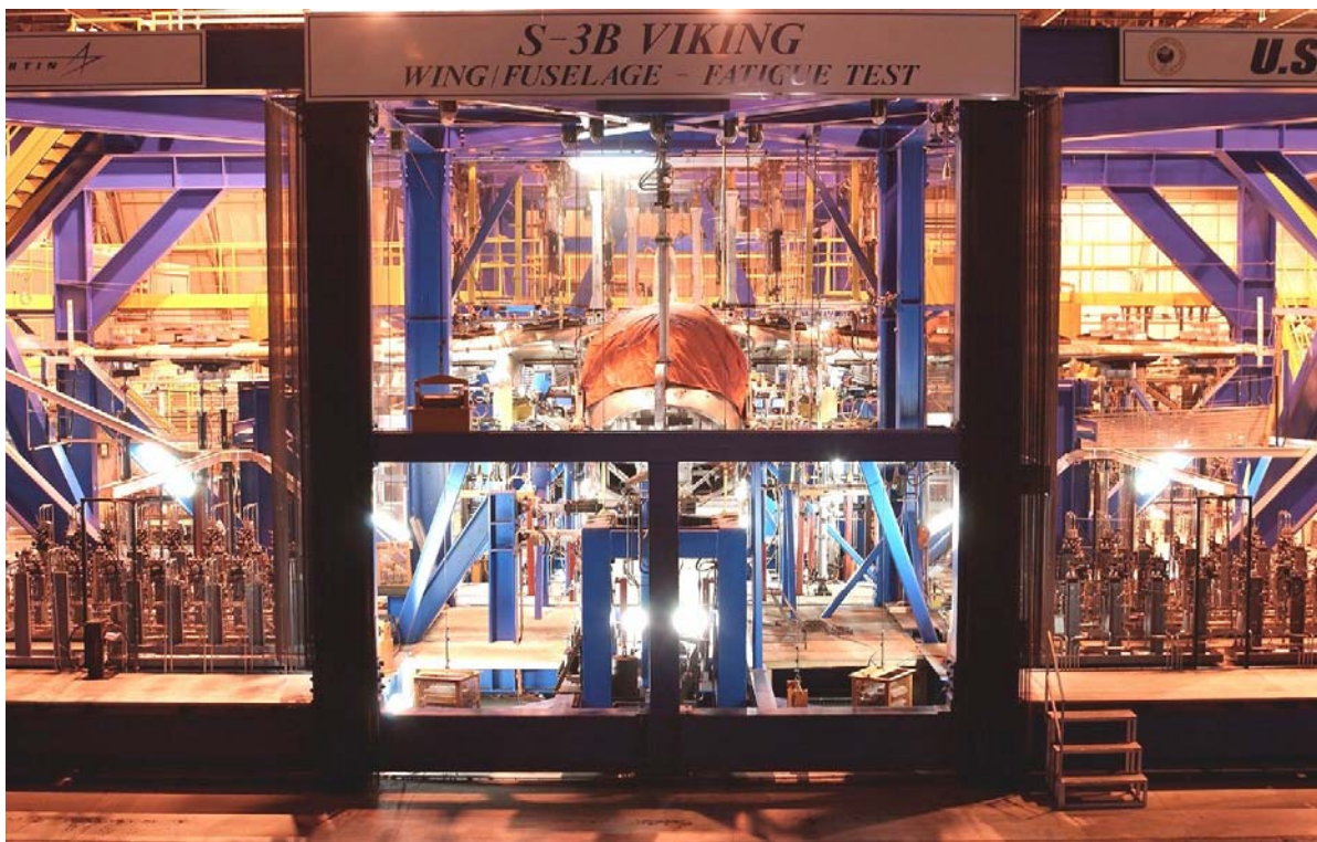
Figure 9.9.1.1 S-3B Viking wing/fuselage test airframe installed in reaction frame – Lockheed Martin Structural Test Laboratory, Marietta, Georgia – Fatigue testing span: 17 September 2001 to 11 November 2002
