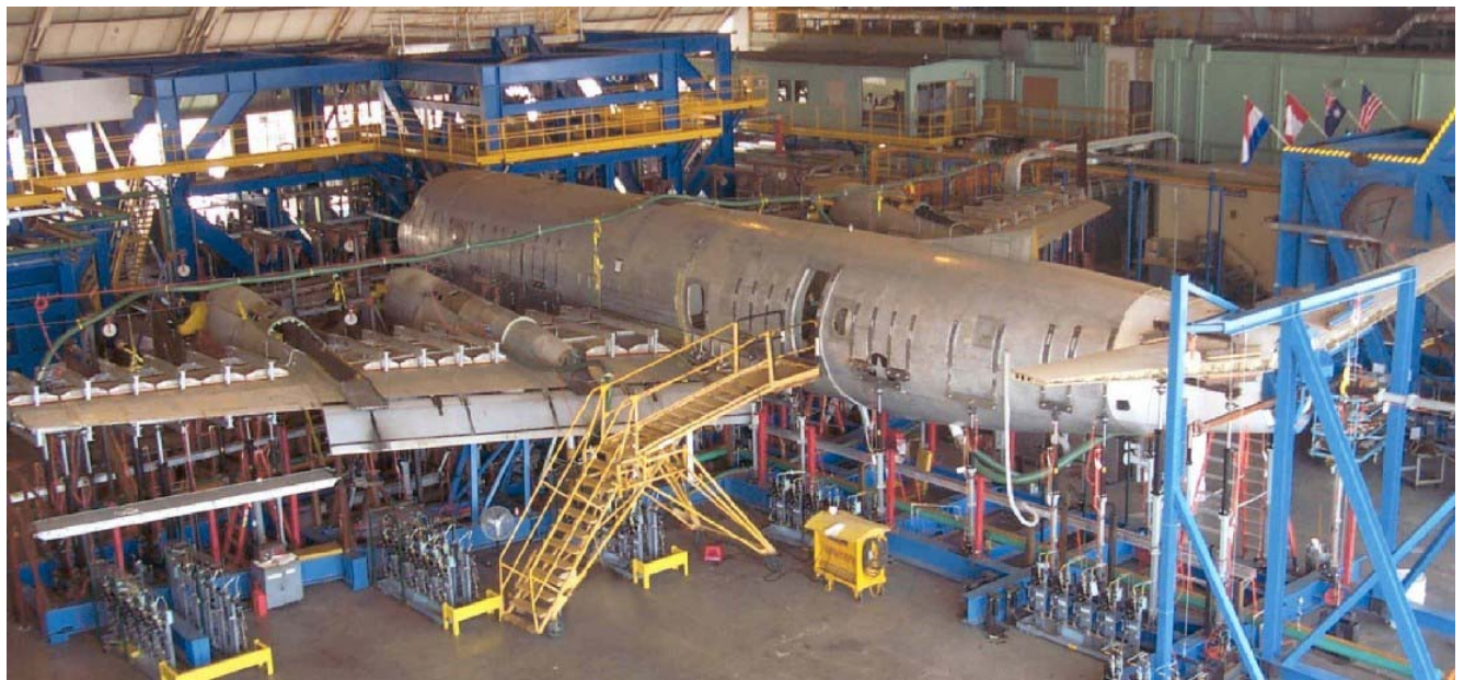
Figure 9.9.2.1 P-3C wing/fuselage test airframe mounted on structural test floor – Lockheed Martin Structural Test Laboratory, Marietta, Georgia – Fatigue testing span: 30 October 2001 to 2 December 2002
