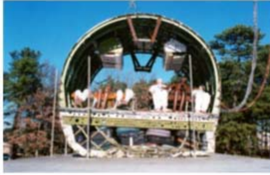
Figure 9.9.4.2 Results of fuselage drop test
