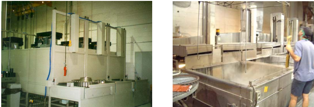
Figure 9.12.5.2 (a) Oven dryer that contains three furnaces and (b) Flash-dry tank used to process components prior to FPI
