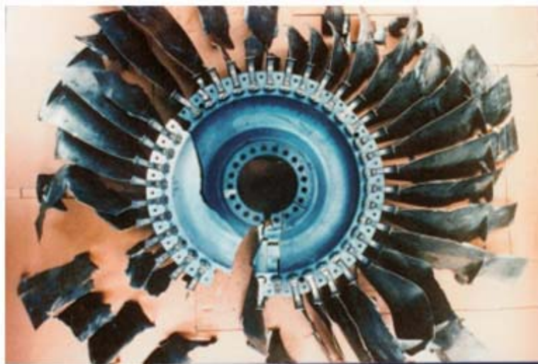
Figure 9.13.2.3 UEDDAM disk burst analysis
