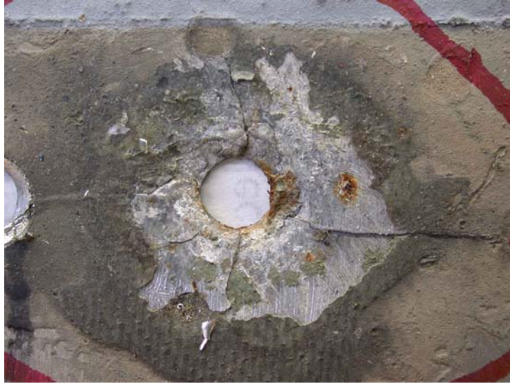
Figure 9.8.3.2 Example of damage found in fuselage panel rivet holes
