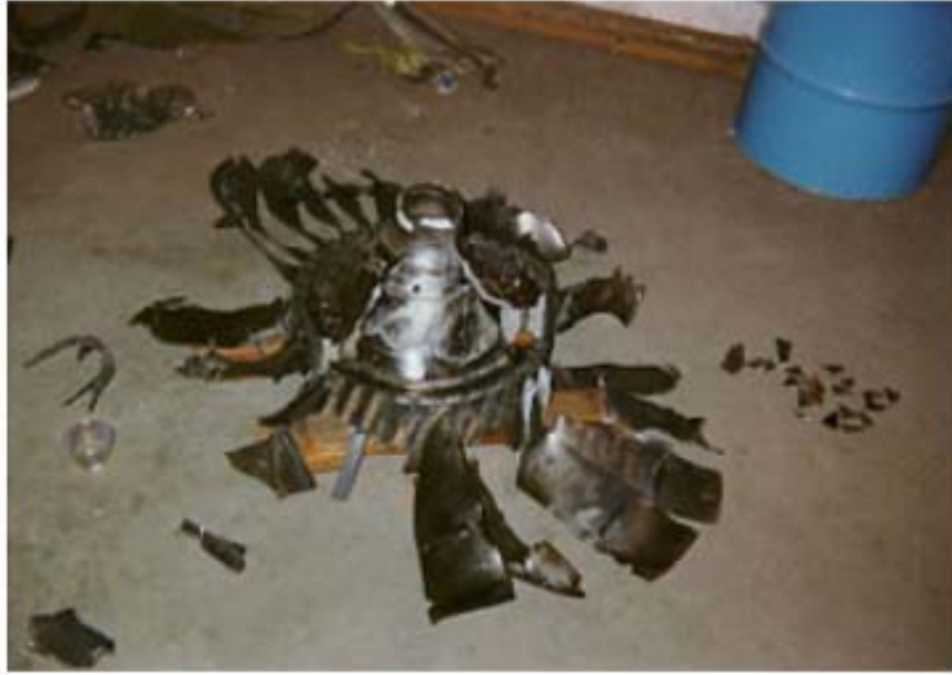
Figure 9.13.1.1 Uncontained engine fan disk
