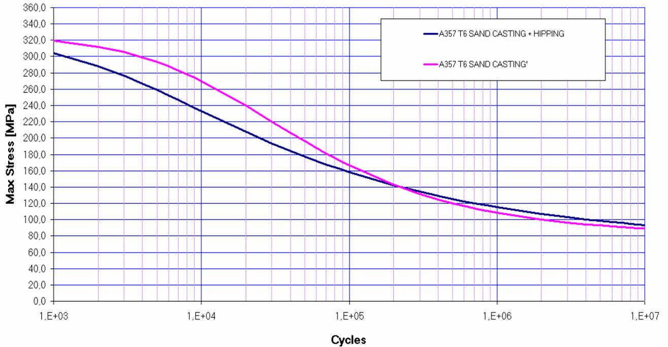
Fig. 14 - Fatigue test results of complex shape specimens in cast A357 alloy (R=0.1).
