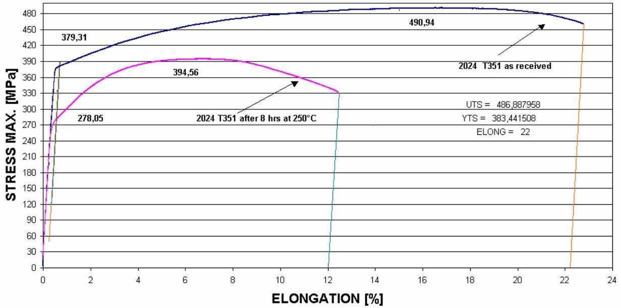
Fig. 15 - Static properties of 2024-T351, before and after soaking 8 hrs at 250 °C; tests at RT.
