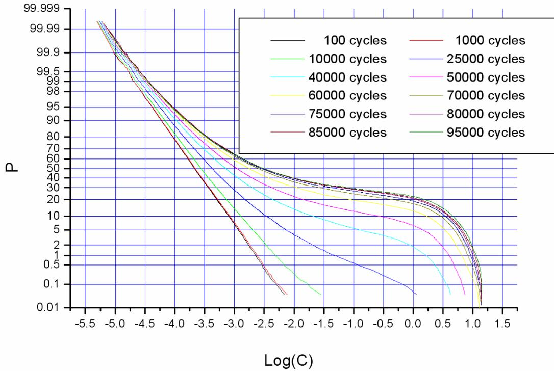
Fig. 34 - Crack distribution in a lap joint at given number of cycles ( $c$  = crack length, mm).
