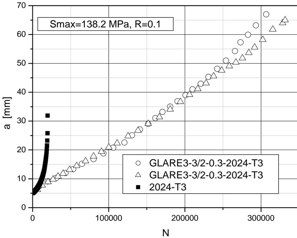
Fig. 37 - Fatigue crack propagation in monolithic and FML panels.
