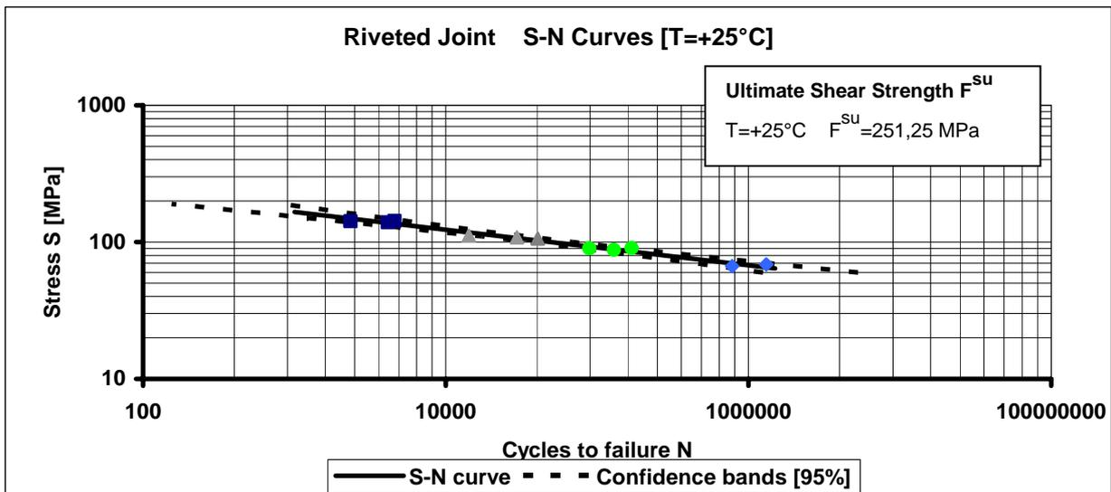
Fig. 43 - Fatigue strength of a riveted joint in FML3.
