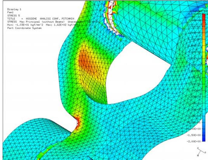
**Fig. 52 - Component stress concentrations evaluated by FEM technique**
