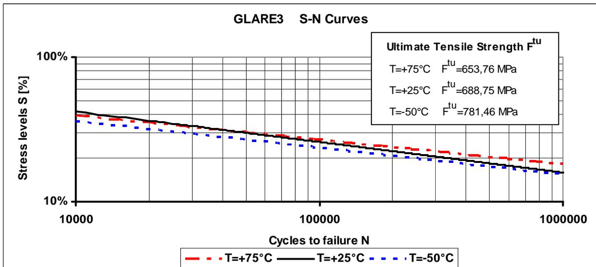
Fig. 40 - Basic fatigue property of FML3-3/2-0.3, at various temperatures.
