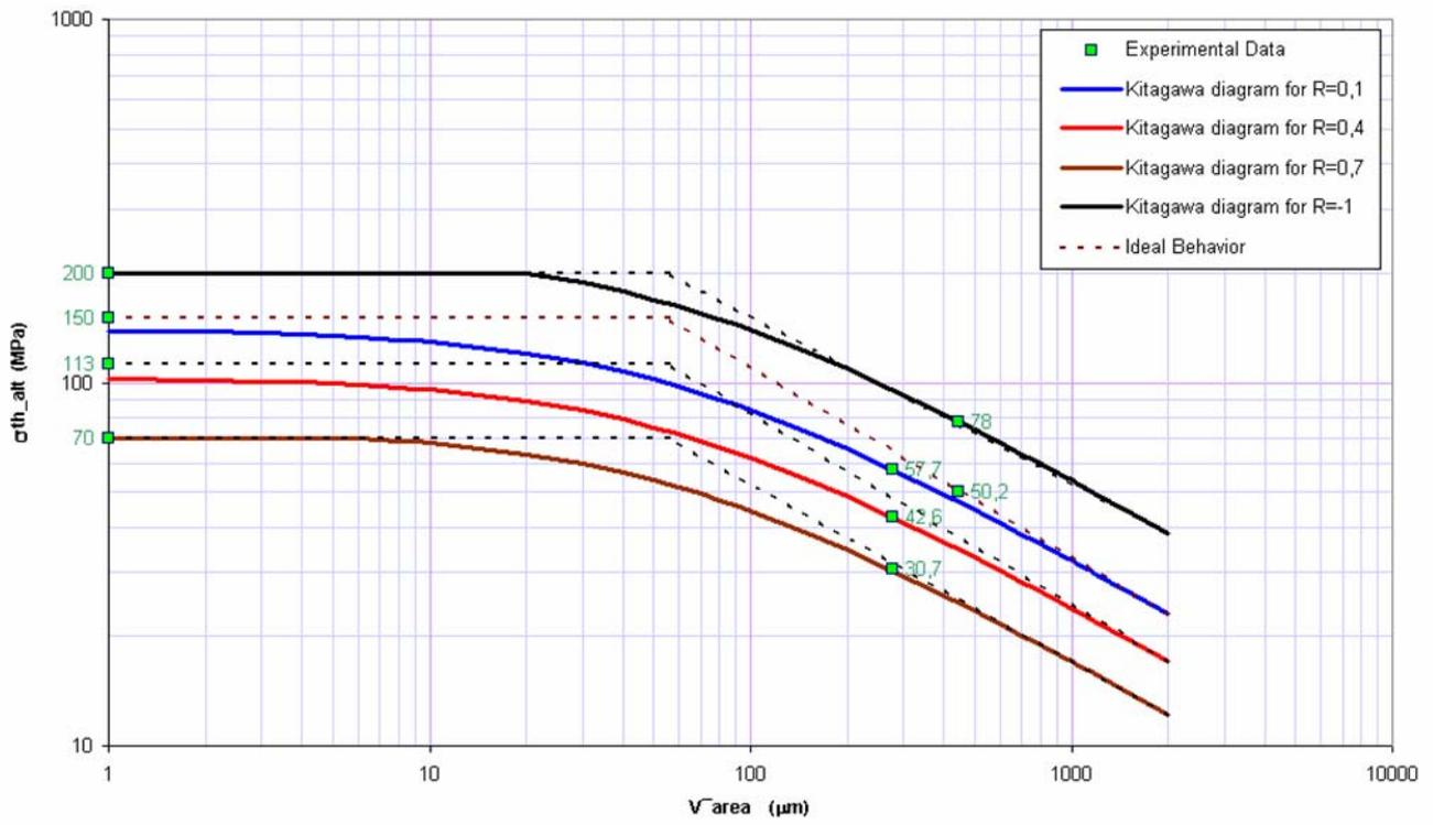
Fig. 33 - Kitagawa diagram for 7475-T7351, for various stress ratios.
