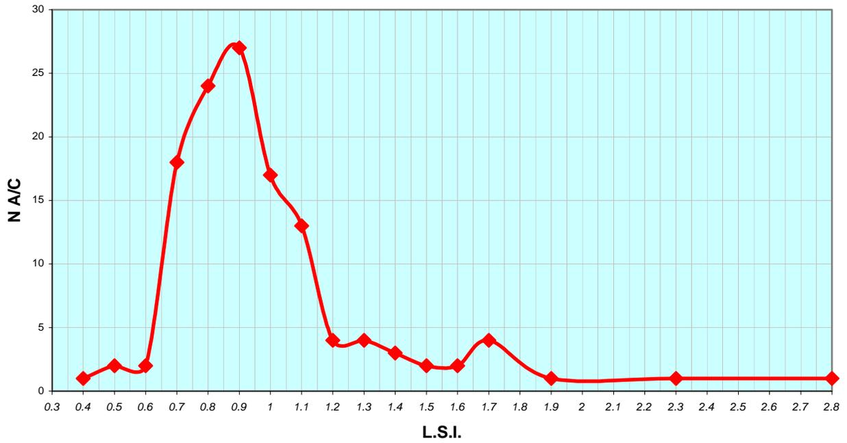
Fig. 1 – Load Severity Index distribution for the AM-X fleet.
