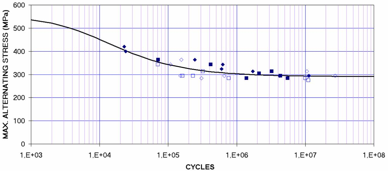
Fig. 36 - Fatigue test results ( $R=0.1$  and  $K_t=1$ ) from specimens taken from forging of 2009-T4 alloy reinforced with 15% SiC particles. Open data points are relevant to anodised specimens, solid to not anodised, diamonds are referred to longitudinal and squares to transverse specimens.
