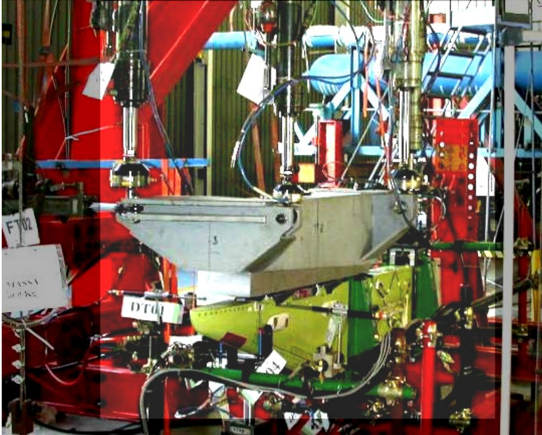
**Fig. 48 - Fatigue test of the EF Typhoon wing inboard pylon.**
