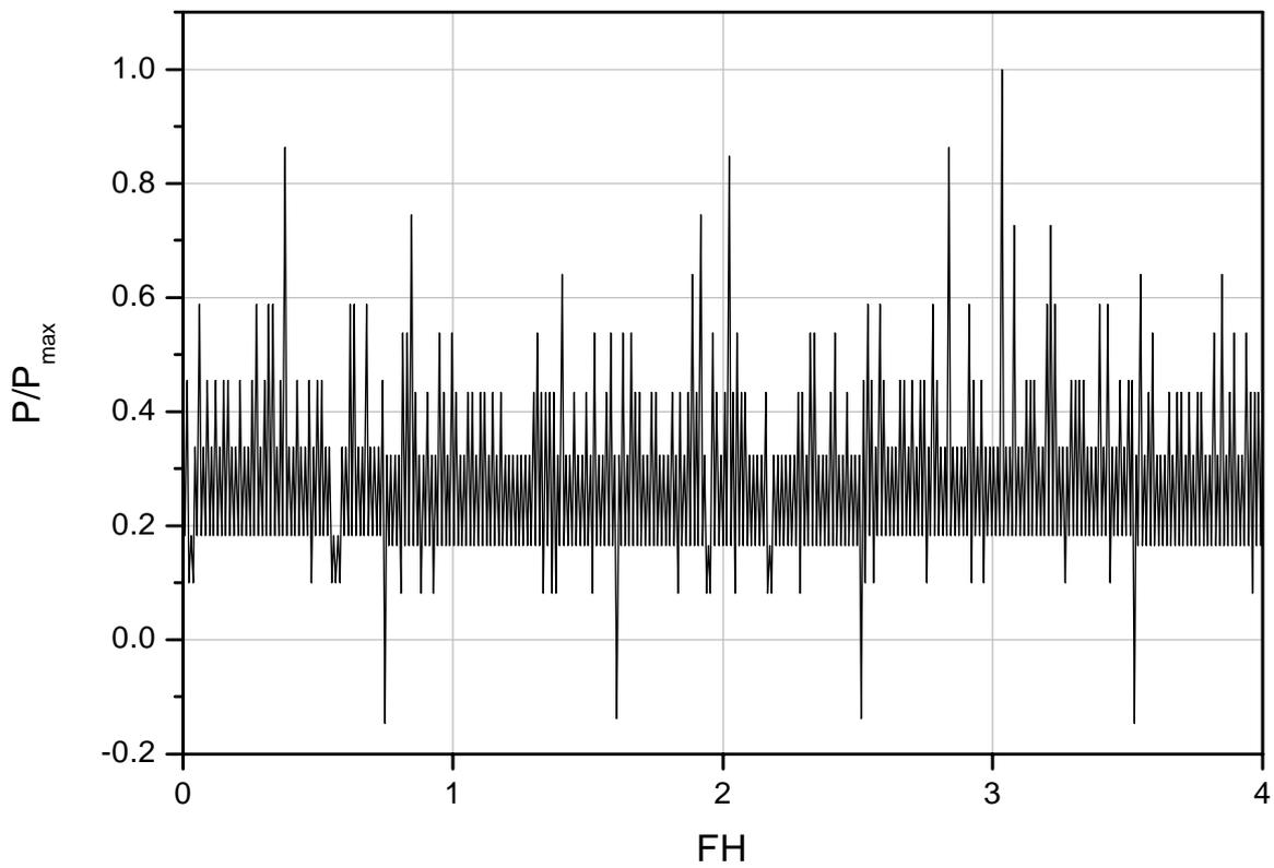
Fig. 30 – First flights of the flight-by-flight sequence of the M346 wing-to-fuselage attachment.
