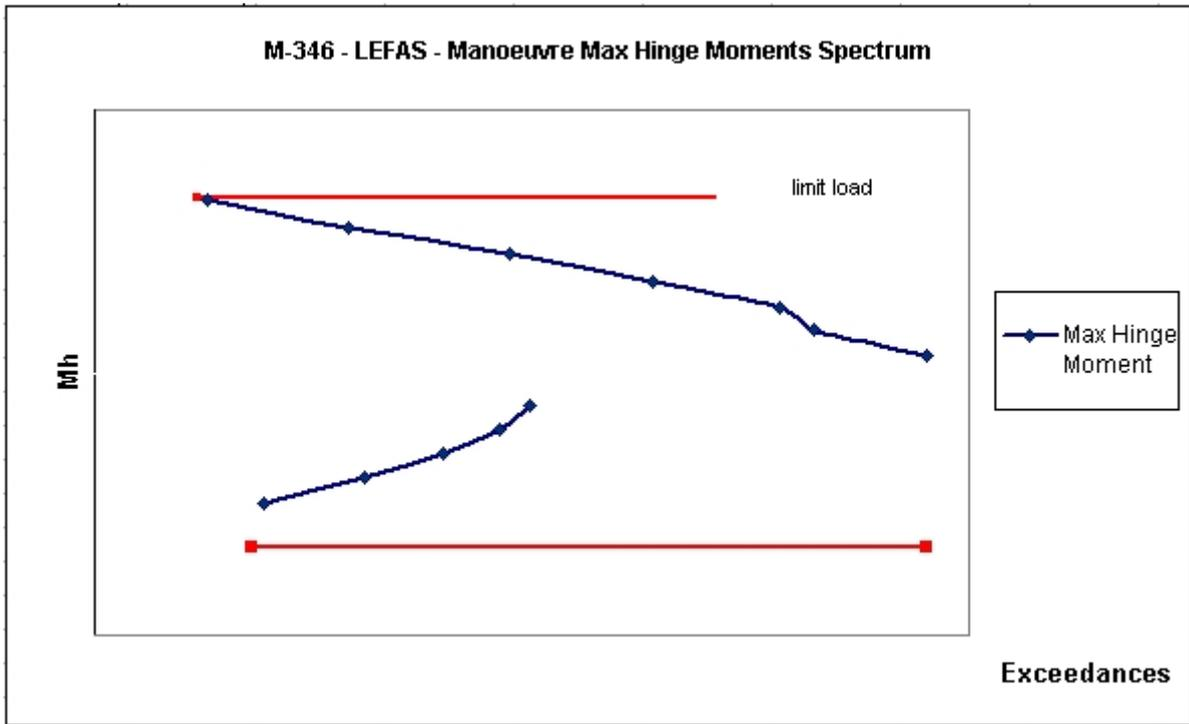
Fig. 50 - Leading Edge Flap Actuation System spectrum for fatigue substantiation.
