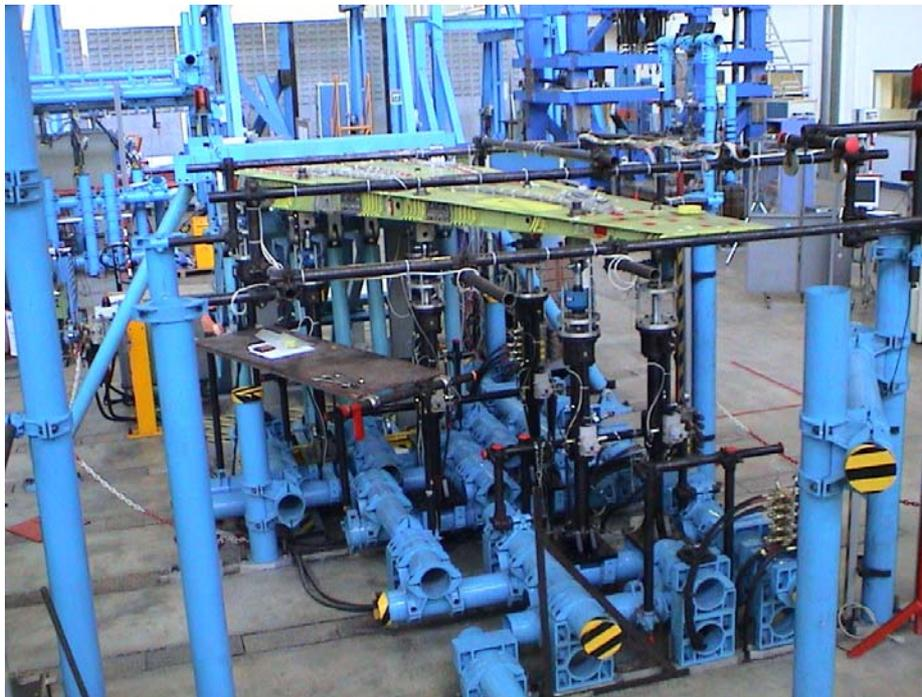
Fig. 47 - Development fatigue test of the LH wing of the M346 trainer.
