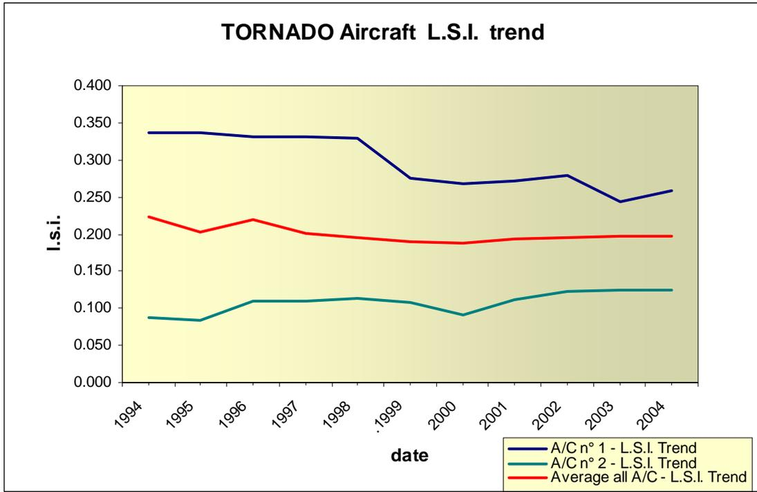
Fig. 3 - Examples of different fatigue consumption rates for individual Tornado aircraft.
