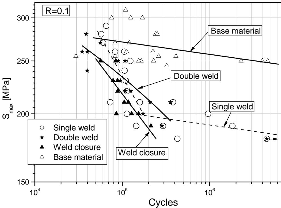
Fig. 24 - Fatigue resistance of FSW joints in 2195-T8.
