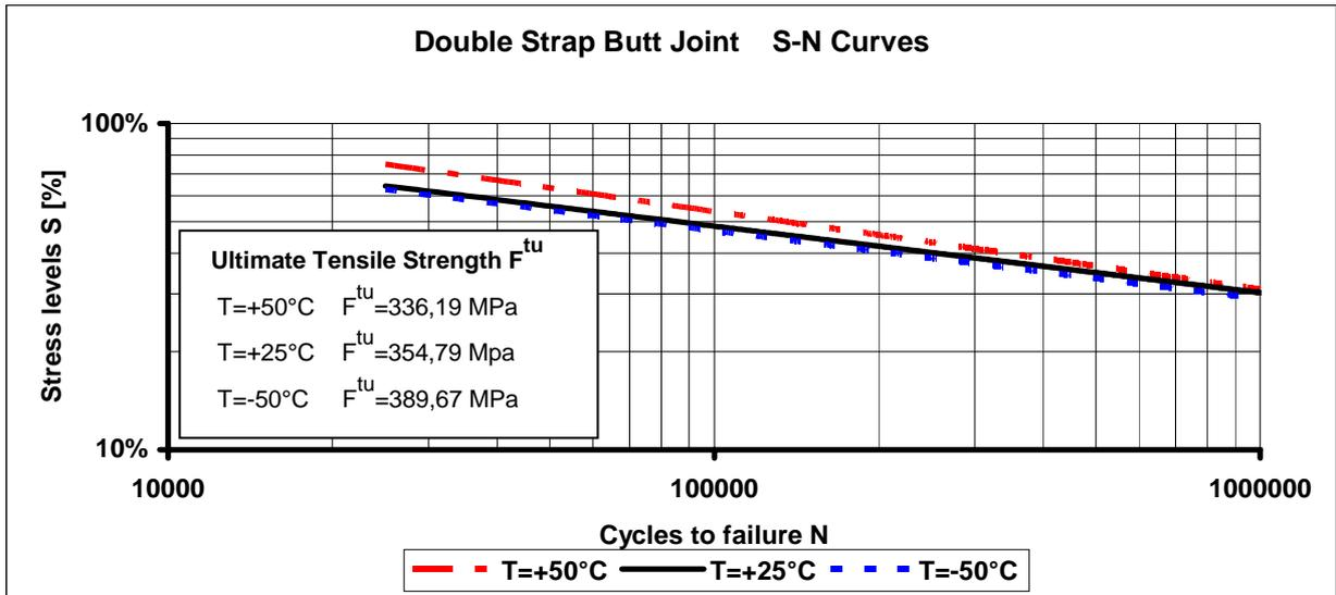
Fig. 41 - Fatigue strength of double strap butt bonded joint in FML3, at different temperatures.
