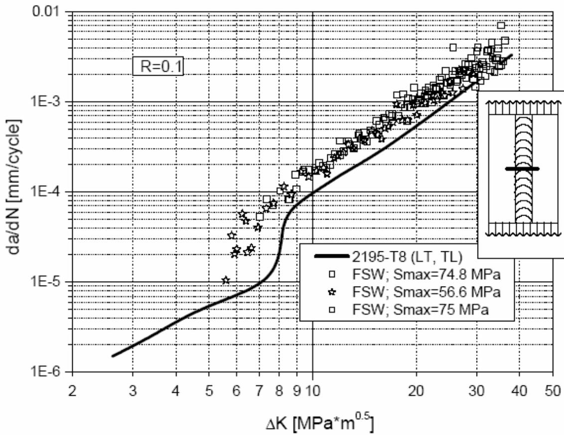
Fig. 27 - Fatigue crack propagation in 2195-T8, R=0.1, across the friction stir weld bead.
