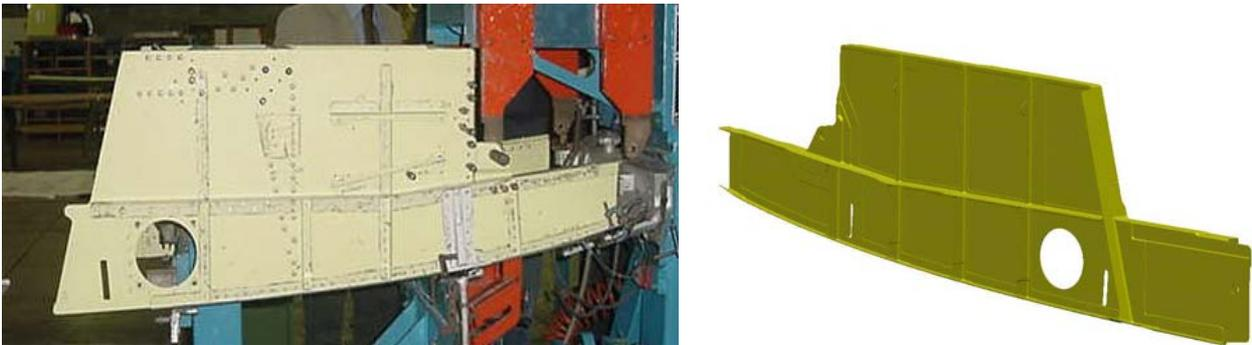
Fig. 51 - P.180 nose landing gear sidewall: change to an integral solution.
