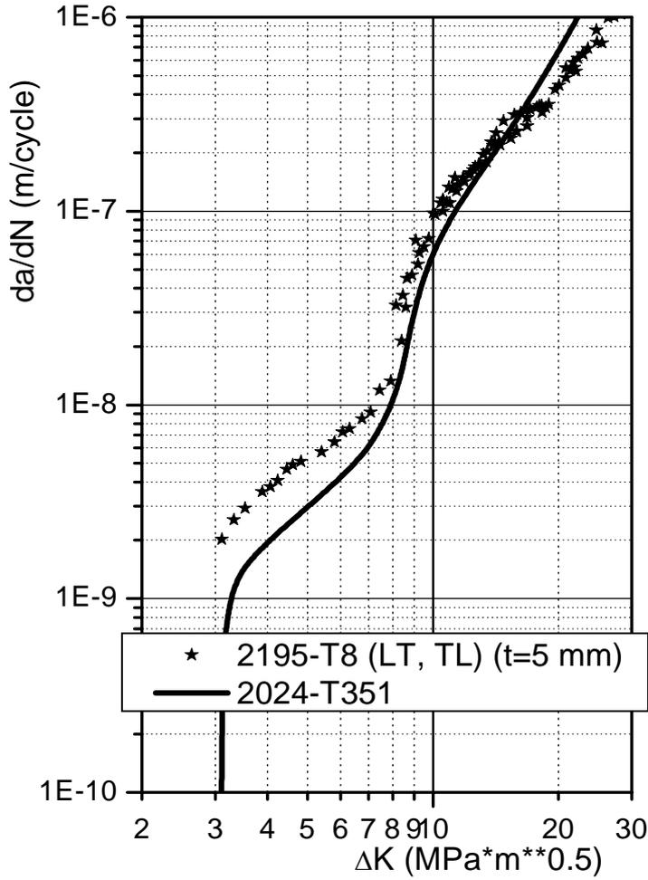
Fig. 25 – Fatigue crack propagation in 2195-T8, R=0.1
