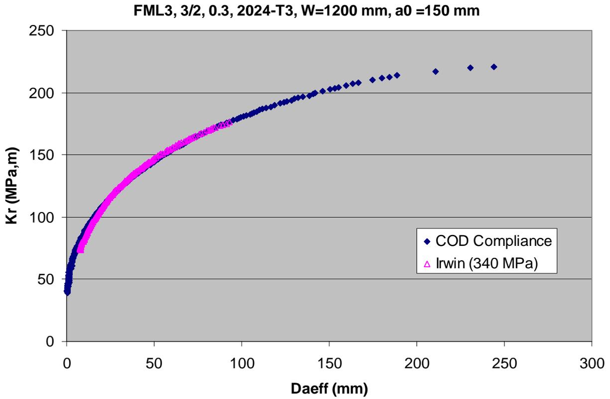
Fig. 39 - Comparison of R-curves obtained from the same test, using different data analysis procedures.
