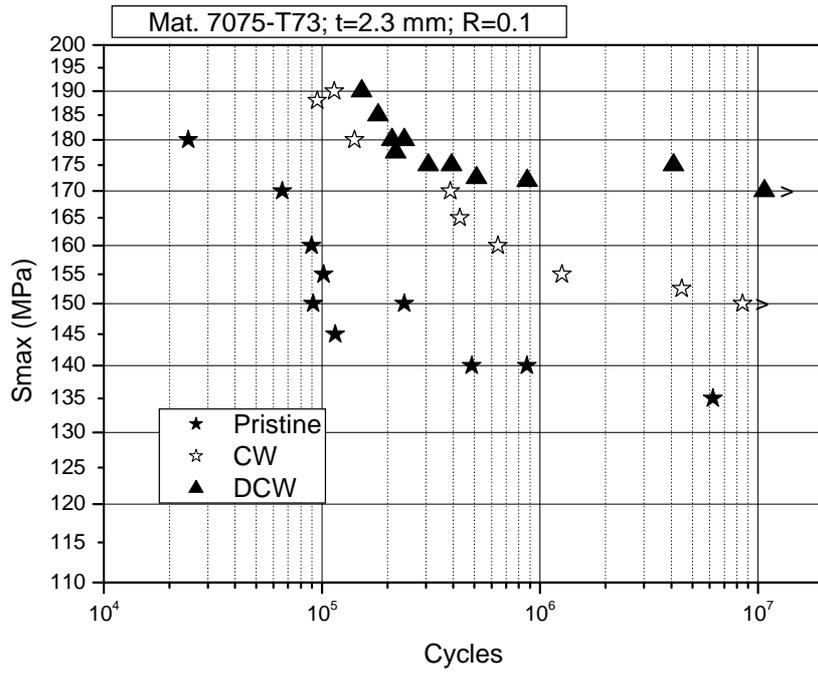
Fig. 11 - S-N curve of pristine, cold-worked and double cold-worked open hole specimens.
