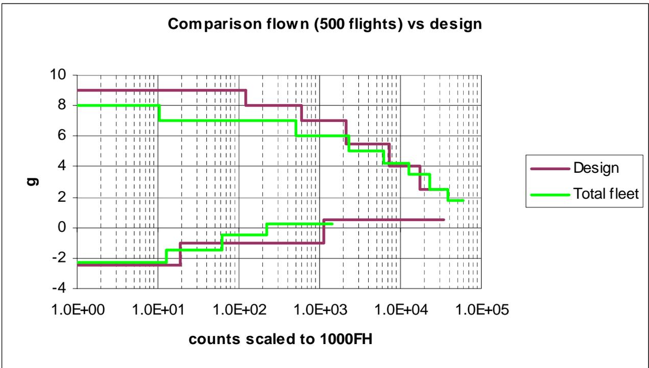
Fig. 4 - IAF EF Typhoon fleet flown spectrum, compared with the design one.
