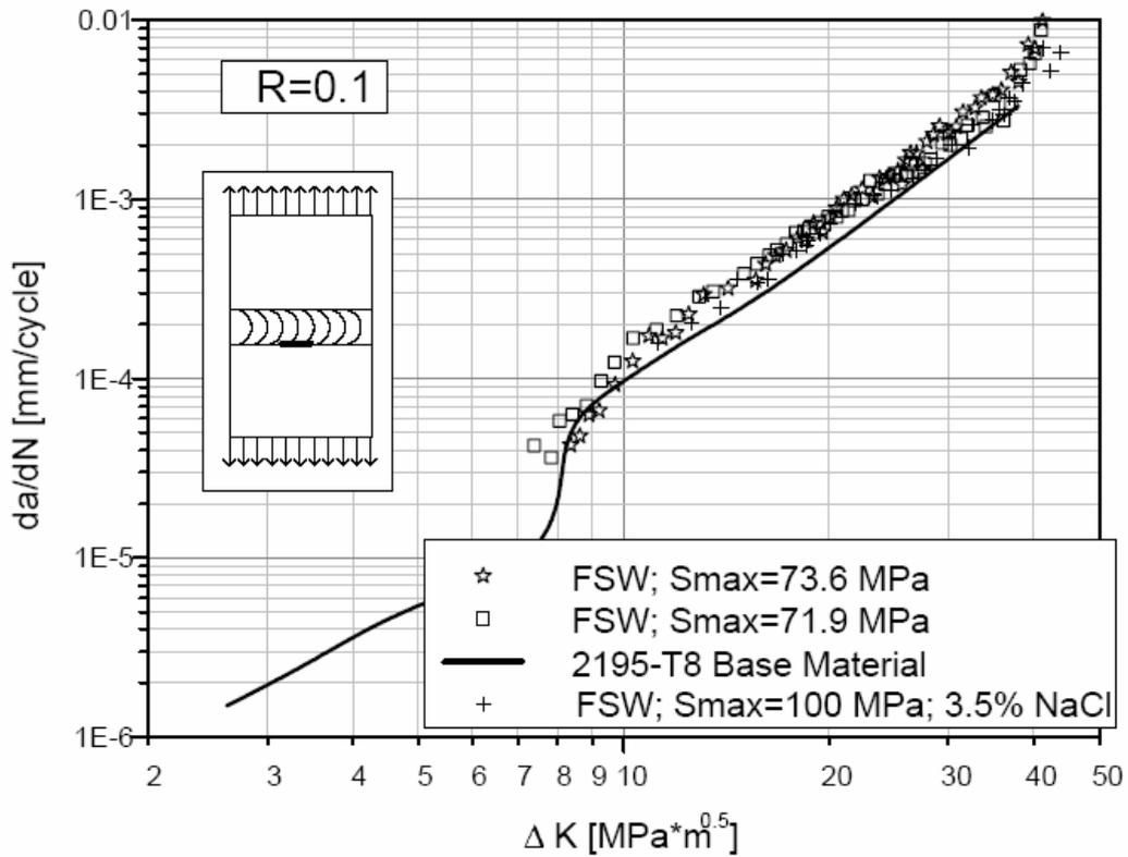
Fig. 26 - Fatigue crack propagation in 2195-T8, R=0.1, along the friction stir weld bead.
