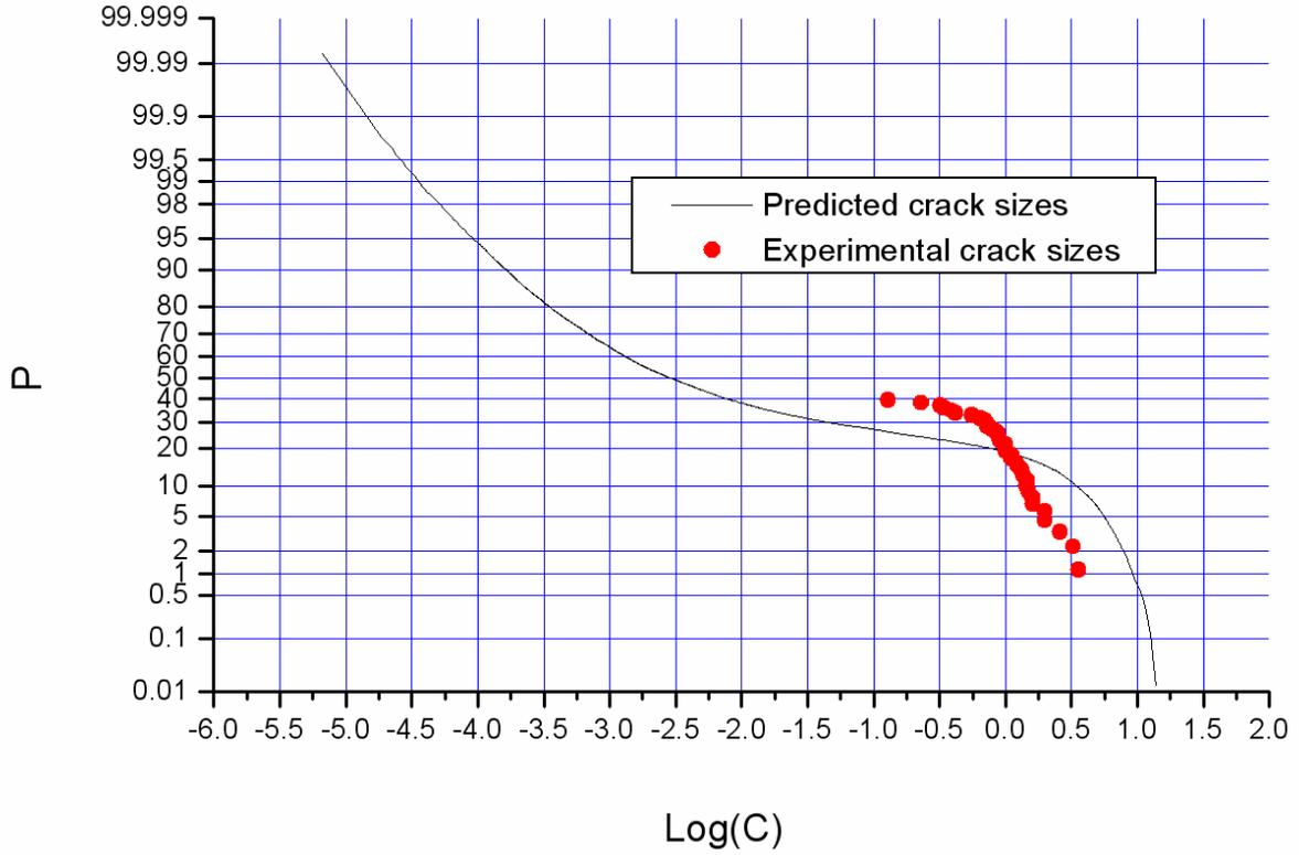
Fig. 35 - Comparison between experimental and predicted crack sizes at 75000 cycles (same example as previous figure).
