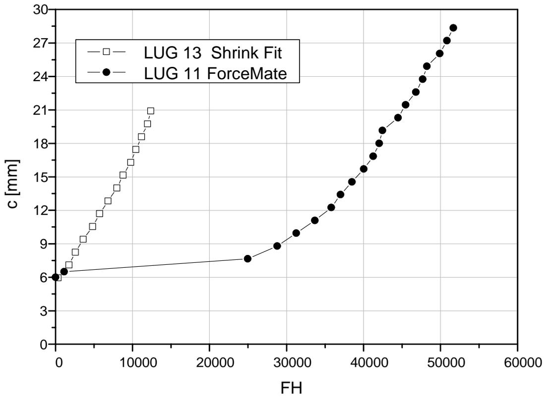
Fig. 31 - Fatigue crack propagation in specimens having a shrink fit or a ForceMate bush installed.
