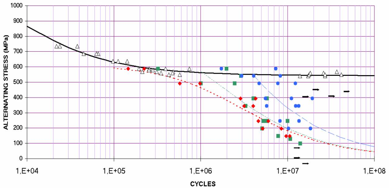
Fig. 20 - Fatigue tests results. Substrate is 4340 steel AMS6415, L direction, 1150-1250 MPa condition. Open triangles are the substrate data points in air, green squares refer to Cd plating in salt environment, blue circles refer to ZnNi, red diamonds to ZnCoFe all in salt environment. The various interpolation lines are also shown.
