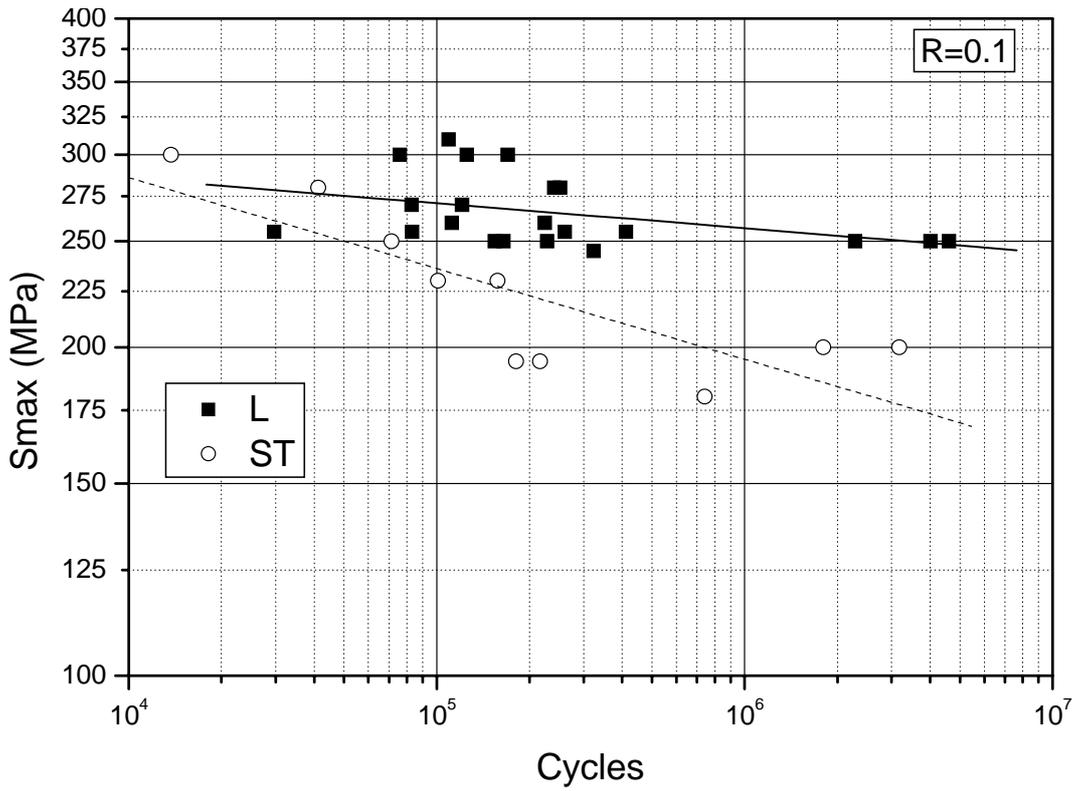
Fig. 23 - Fatigue resistance of 2195-T8 un-notched specimens, machined in different orientations.
