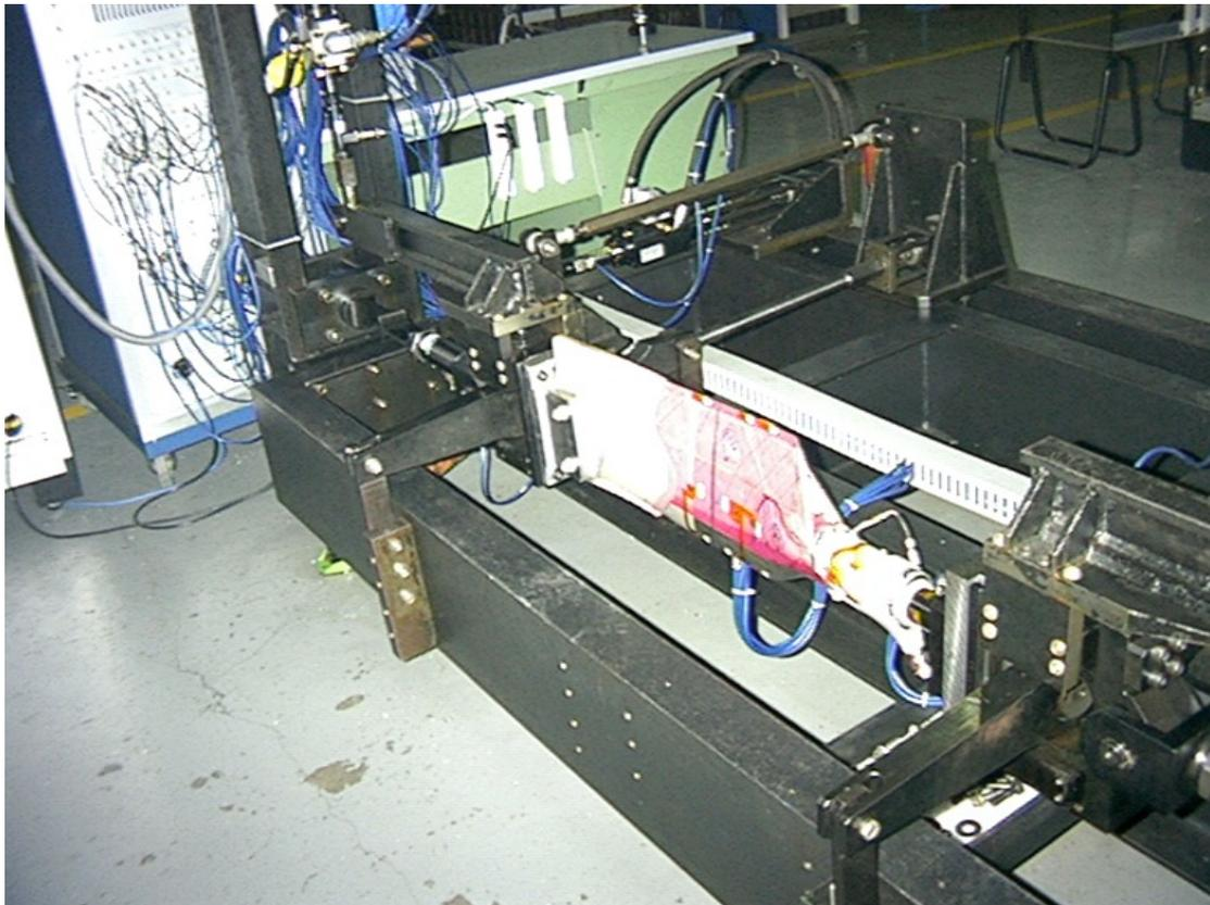
**Fig. 49 - Test rig for the fatigue test of the Tail Rotor blade of the A109 helicopter.**
