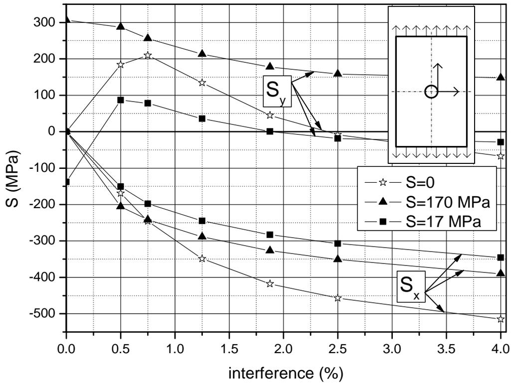
Fig. 10 - Circumferential (y) and radial (x) stress distribution in the critical location of a hole with a pin fitted with various interference levels.
