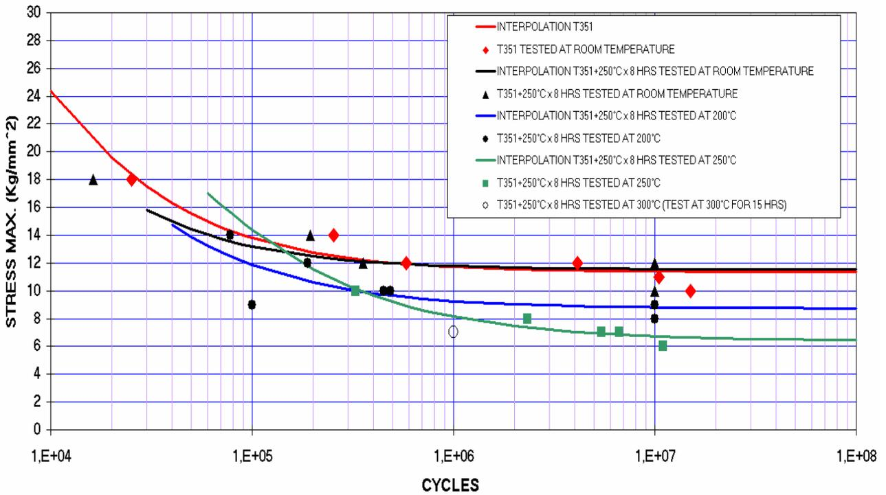
Fig. 16 – S-N curves for 2024-T351 tested at RT and at Elevated Temperature, after different thermal exposure.
