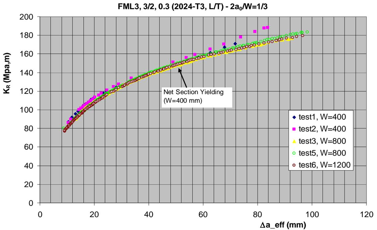
Fig.38 – Comparison of R-curves of FML panels of different width (Irwin correction, 340 MPa).
