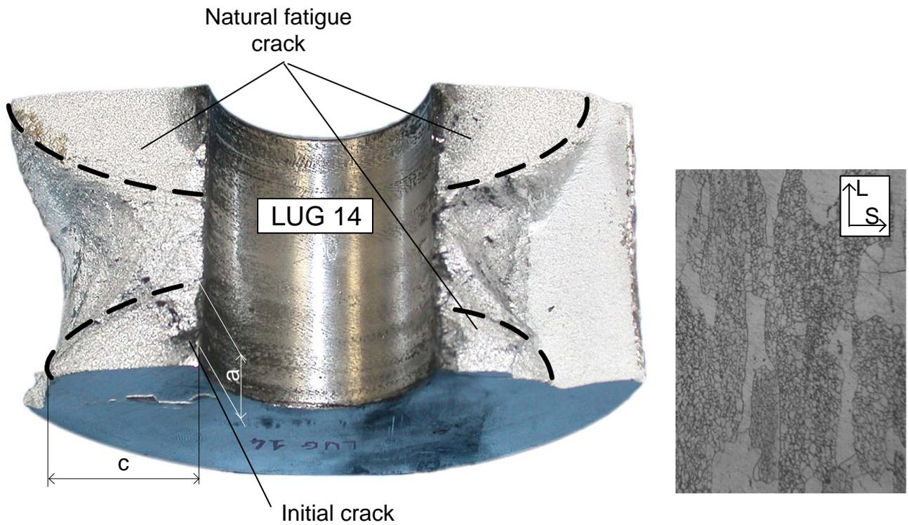
Fig. 32 - Typical fracture surface in a lug/fork specimen and micrograph of the internal structure of the material.
