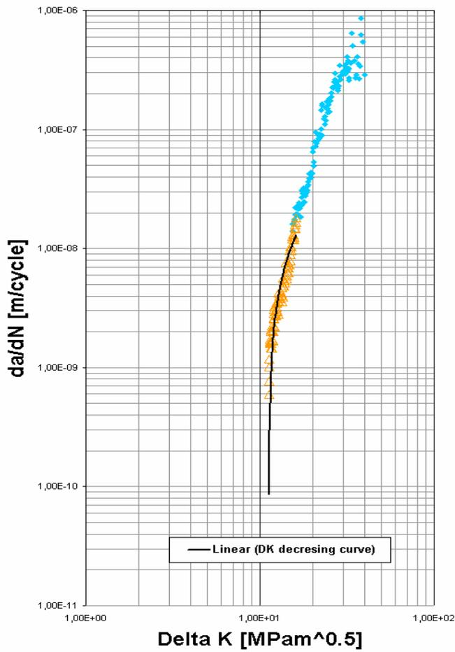
Fig. 19 - Fatigue crack propagation in Beta Solution Treated / OverAged Ti-6Al-4V alloy, R=0.1.
