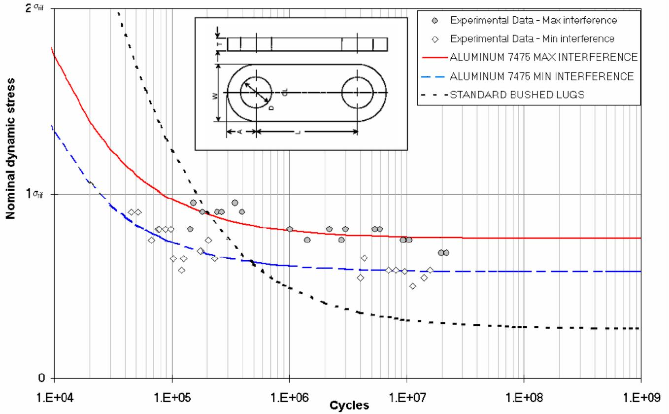
Fig. 21 - Fatigue test data from pristine lugs in 7475-T7351: effect of the Forcemate® bushing installation interference.
