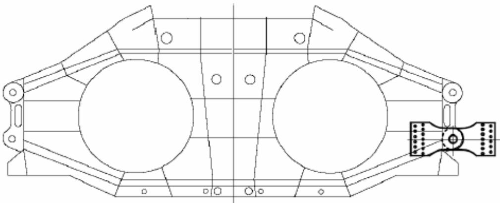
Fig. 28 - Sketch of the M346 fuselage frame with location of the attachment specimen.
