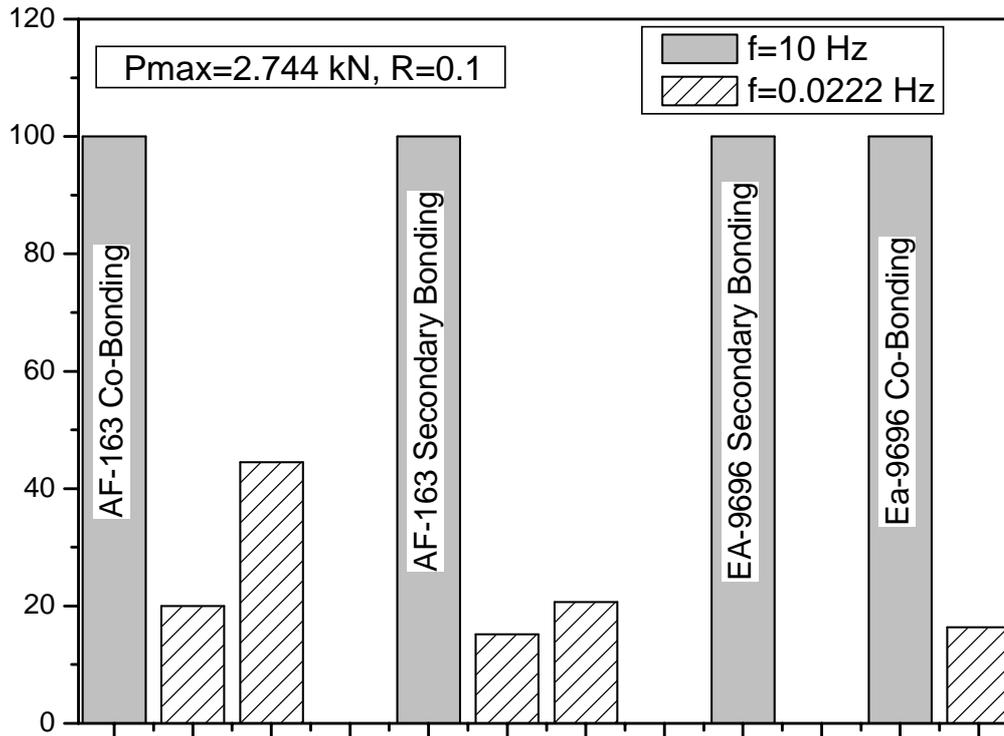
Fig. 46 - Results of the low frequency fatigue tests on "L-Pull" specimens, as a percentage of the respective standard frequency fatigue test results.
