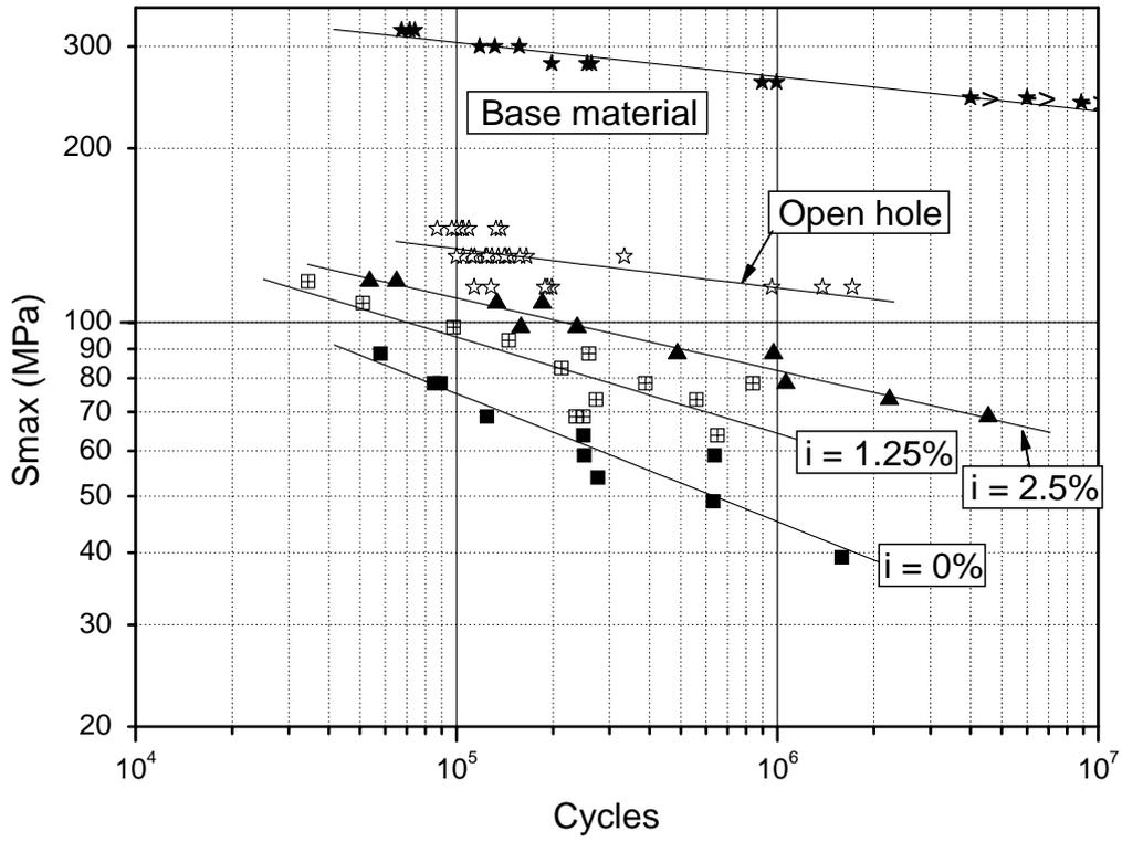
Fig. 9 - Effect of interference on the fatigue behaviour of pin loaded specimens (R=0.1).
