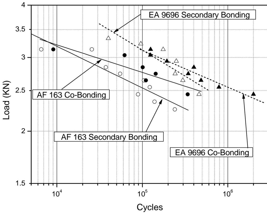
Fig. 45 - "L-Pull" specimen fatigue test results (R=0.1, f=10 Hz).
