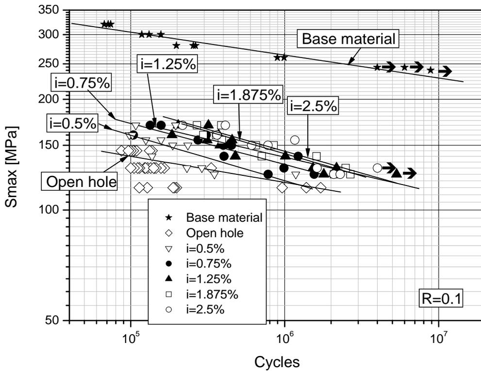
Fig. 8 - S-N curves of specimens having a central hole filled with an interference fit pin.
