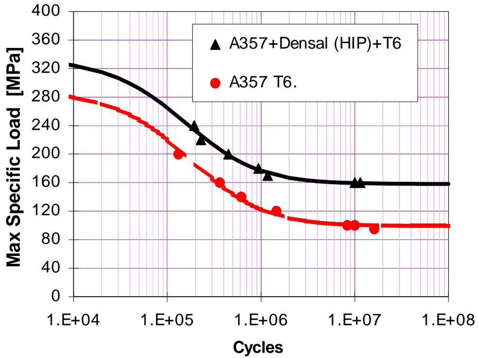
Fig. 13 - Effect of HIP treatment on the fatigue behaviour of A357 specimens, cut from cast rods.
