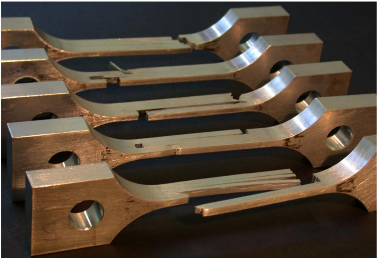
Fig. 22 – Anomalous fatigue cracks pattern in 2195-T8 specimens.
