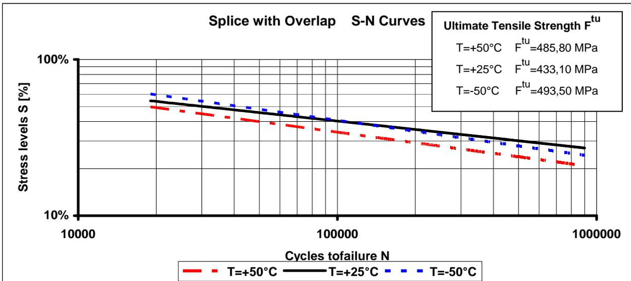
Fig. 42 - Fatigue strength of FML with internal splices (overlap, 12.7 mm), at different temperatures.
