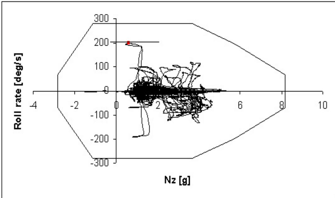
Fig. 5 – EF Typhoon roll rate vs. normal acceleration envelope.
