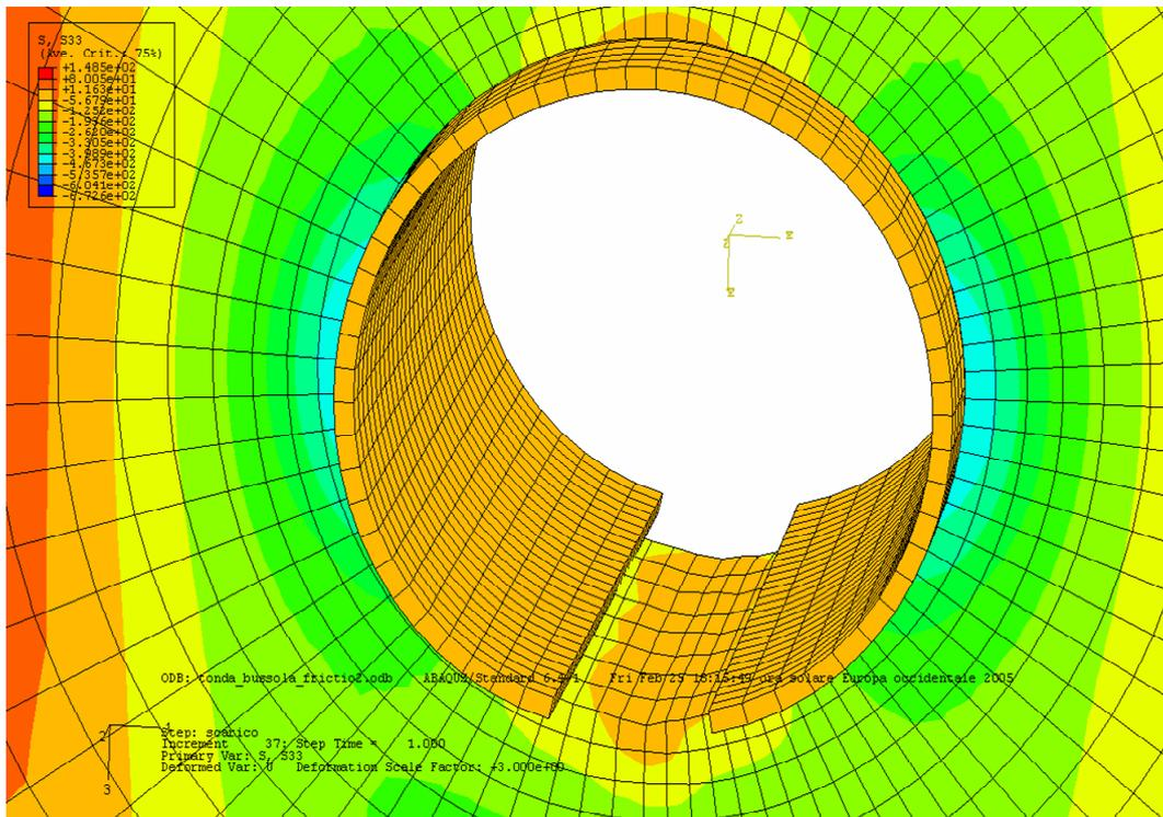
Fig. 12 – Finite Element simulation of the Cold Working process.
