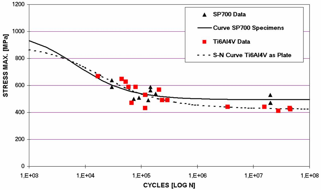
Fig. 17 - Comparison between fatigue (rotating bending,  $K_t=1$ ) results from Ti-4.5Al-3V-2Fe-2Mo and traditional Ti-6Al-4V titanium alloys
