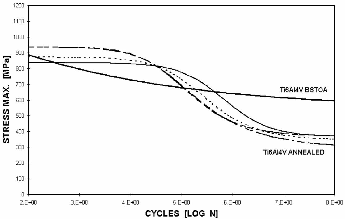
Fig. 18 - Titanium forgings in Ti 6Al 4V Alloy: S-N curves ( $K_t=1$ ,  $R=0.1$ ) comparing annealed condition to the  $\beta$ -solution treated/overaged (BSTOA) condition.
