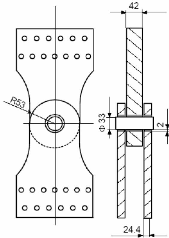
Fig. 29 – Geometry of the specimen simulating the M346 wing-to-fuselage attachment.
