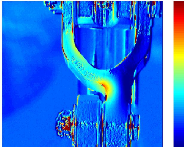
**Fig. 53 - Raw TSA image at 1,8 Hz of the component in the previous figure**
