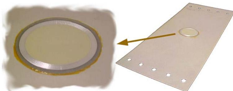
Example of specimen with repair
