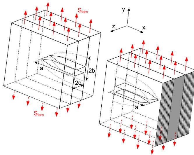
Fatigue crack geometry in Glare
