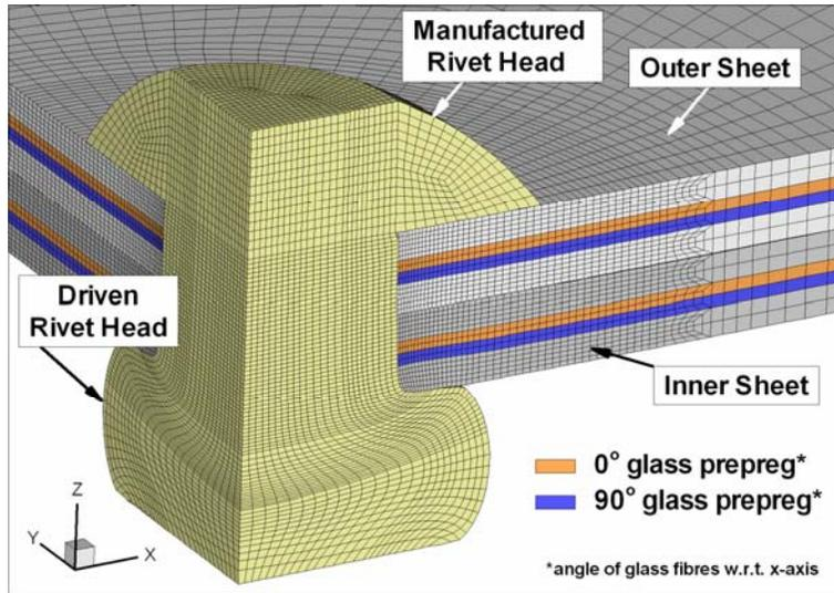
Typical deformed mesh for quarter-symmetry rivet forming model showing lay-up orientation used for GLARE3-2/1-0.3 sheets
