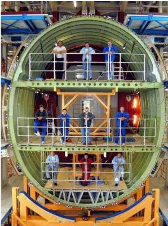
Figure 23 Assembly of barrel specimen completed
