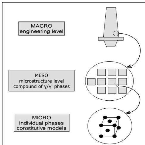
Figure 13 Schematic view of the different levels for investigation of crack forming
