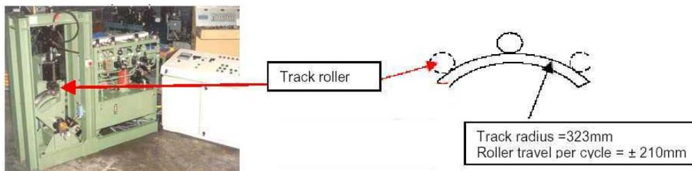
Figure 25 Dassault Falcon F7X track roller test set-up
