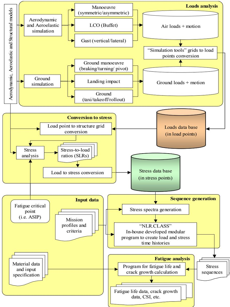
Figure 2 Schematic for a load database system for fatigue analysis
