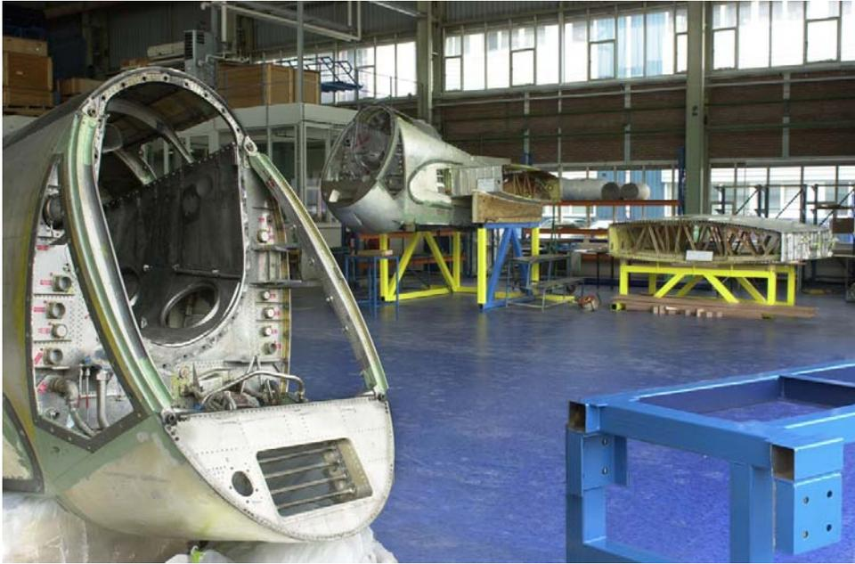
Figure 10 Part of the P3-C Orion ready for the teardown
