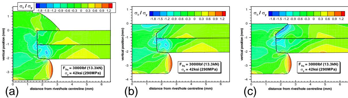
Comparison of residual tangential stress distribution in 2024-T3 for (a) universal rivet; (b) flush countersunk rivet; (c) 0.07 mm protruding countersunk rivet
