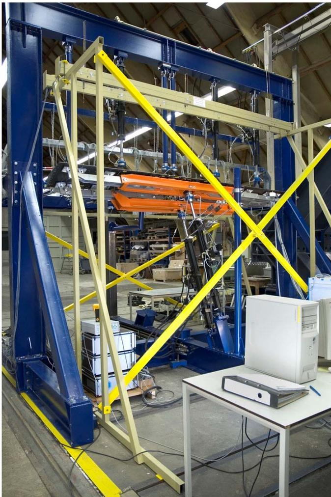
Figure 24 Dassault Falcon F7X aileron fatigue test set-up
