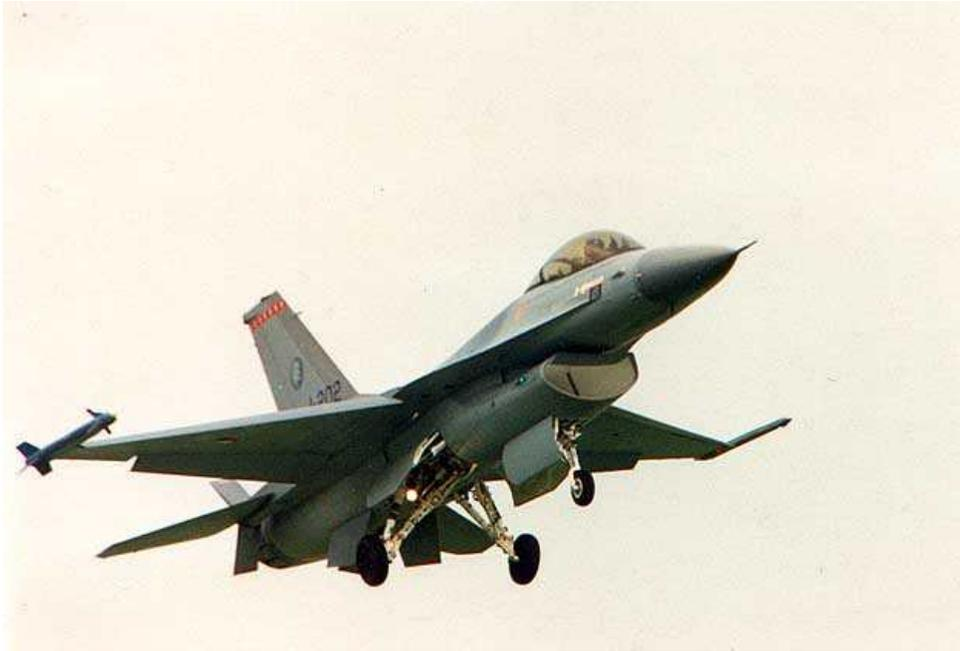
Figure 3 F-16 aircraft with extended landing gears
