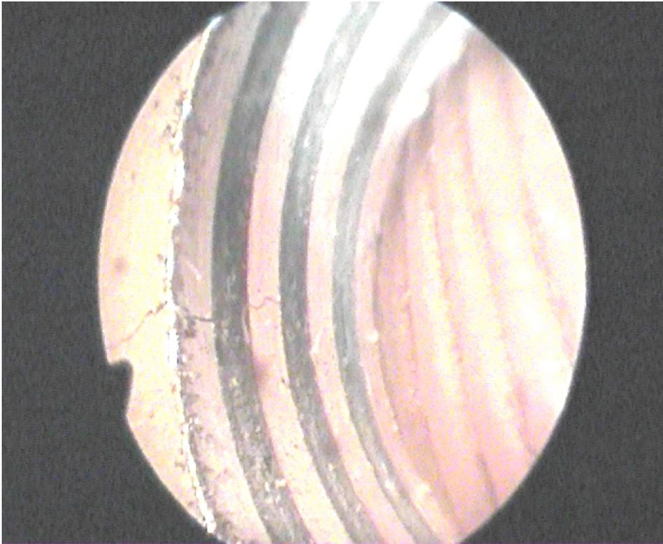
Figure 16 Fatigue cracks in surface and subsurface layers of Glare in a combined bending-tension specimen
