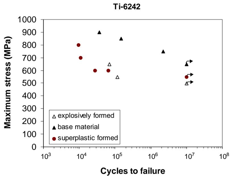
Figure 18 Constant amplitude fatigue test results ( $R=0.1$ ) on smooth Ti-6242 samples. Base material data were obtained from the Technical University Hamburg-Harburg
