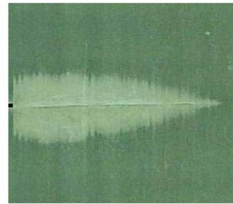
Delamination after etching aluminium
