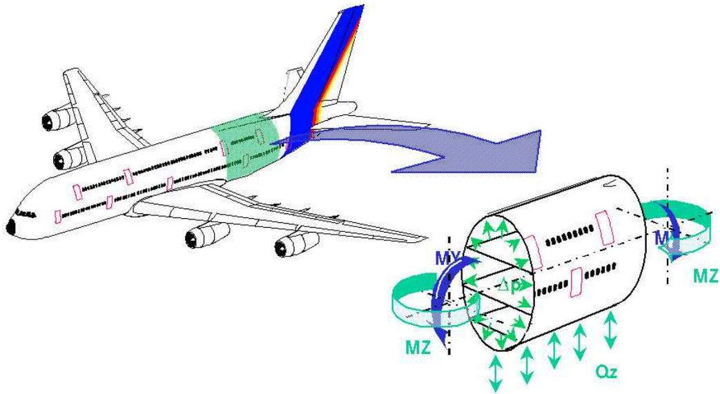
Figure 22 Location of the fuselage barrel section
