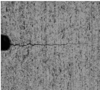
Fatigue crack in aluminium layer of Glare
