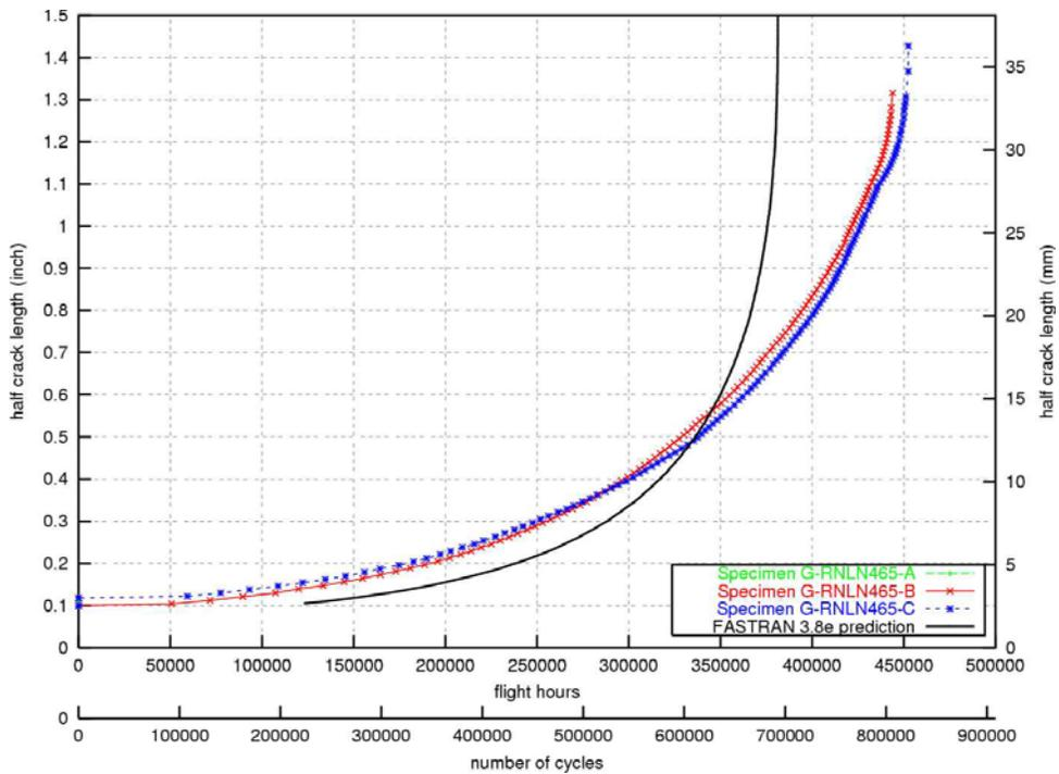
Figure 9 Comparison of crack growth data for P3-C Orion OW WS 209 Spanwise Splice at panels 3 & 4 (outer side of inboard engine) (Black is analysis, Red and Blue are experiments)
