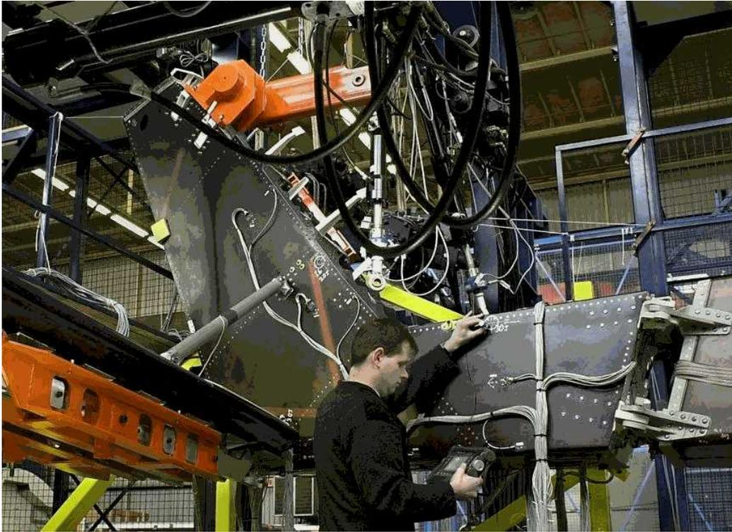
Figure 21 NH 90 helicopter tail section, fatigue test set-up
