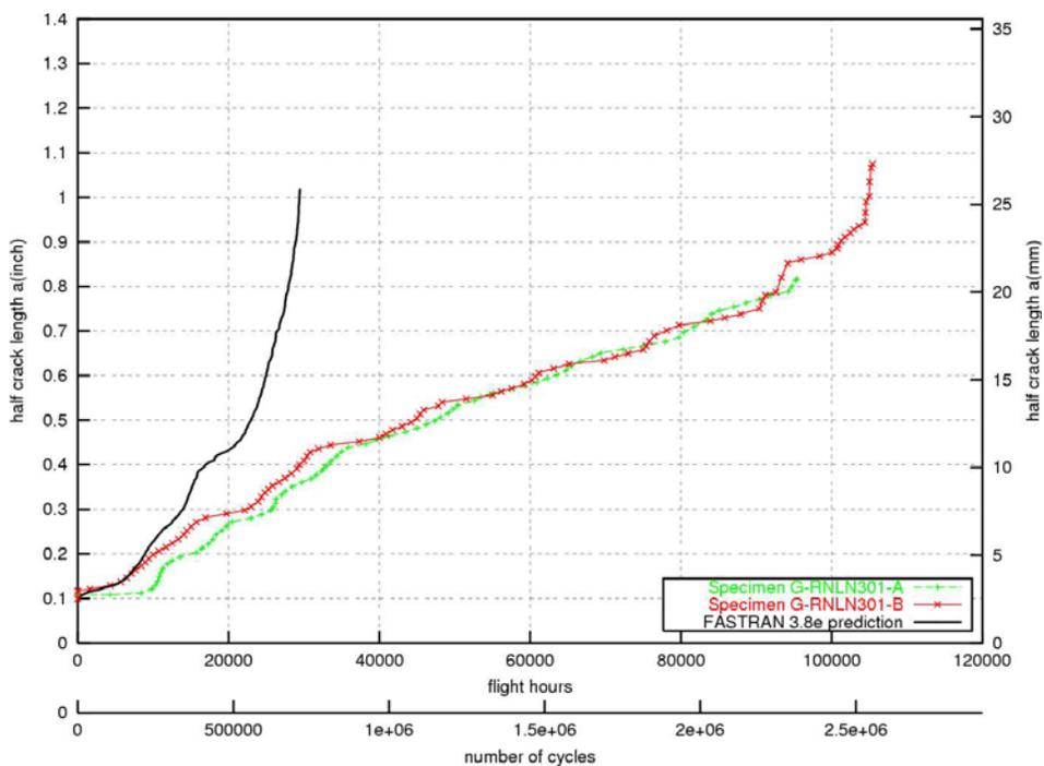
Figure 8 Comparison of crack growth data for P3-C Orion FCA 301 Front spar lower cap at OW WS 65 (wing root). (Black is analysis, Red and Green are experiments)
