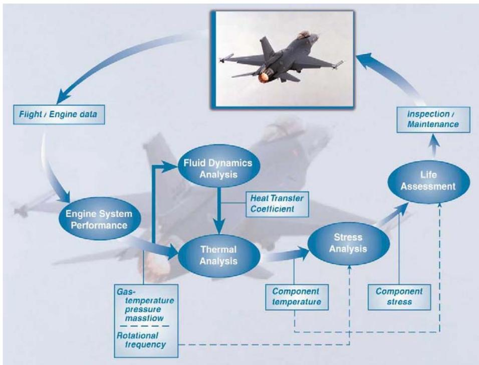
Figure 14 Different disciplines involved in the life assessment of gas turbine components
