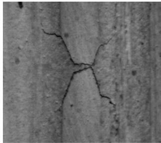
Crack and delamination at interfaces
