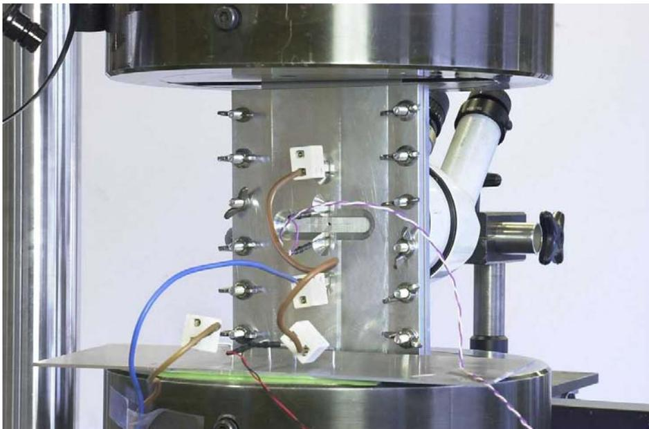
Figure 7 Test set-up for comparison experimental and analytical crack growth data in the framework of the service life assessment programme for the P3-C Orion aircraft
