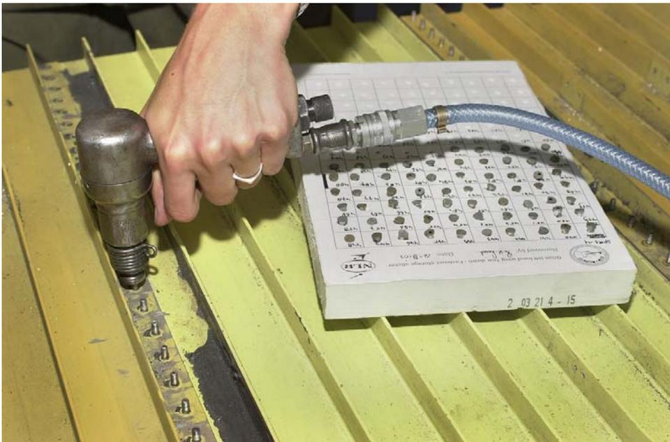
Figure 11 Removing the fasteners to be able to inspect the fastener holes
