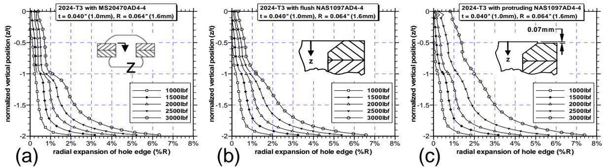
Comparison of radial expansion levels in 2024-T3 for (a) universal rivet; (b) perfectly flush countersunk rivet; (c) 0.07 mm protruding countersunk rivet
