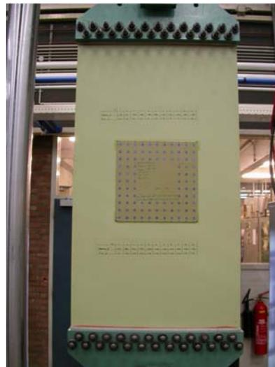
Bonded and riveted patch repair
