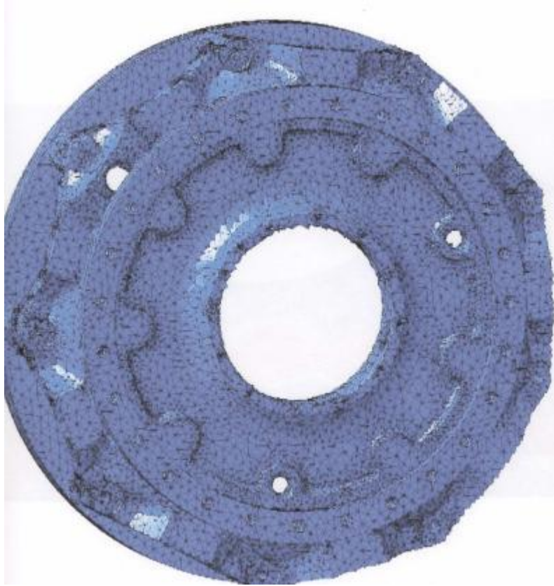
Fig. 11. 3D model of the rear part of crankcase
