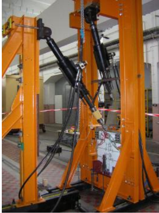
Figure 13. Test set-up with the hinge fitting specimen.
