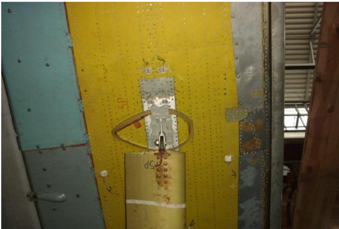
Fig. 2. Right outer wing critical region after the repair which was made before re-starting of the fatigue test. An additional piece of skin and elongated wing bracing fitting can be seen.
