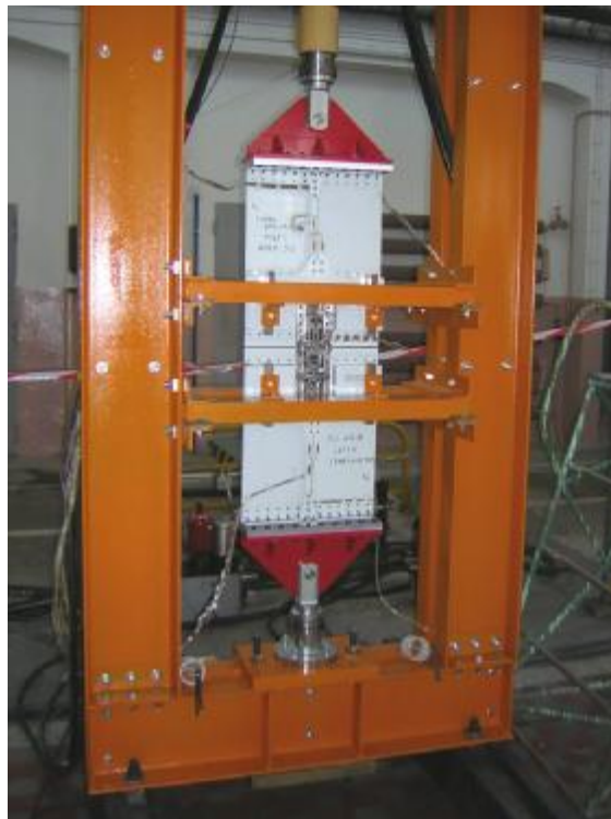
Figure 14. Test set-up with the latch housing specimen.
