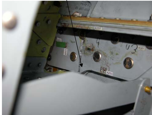
Figure 3. Saab 2000 Residual strength test- artificial saw cut at the inboard section of the horizontal stabilizer.
