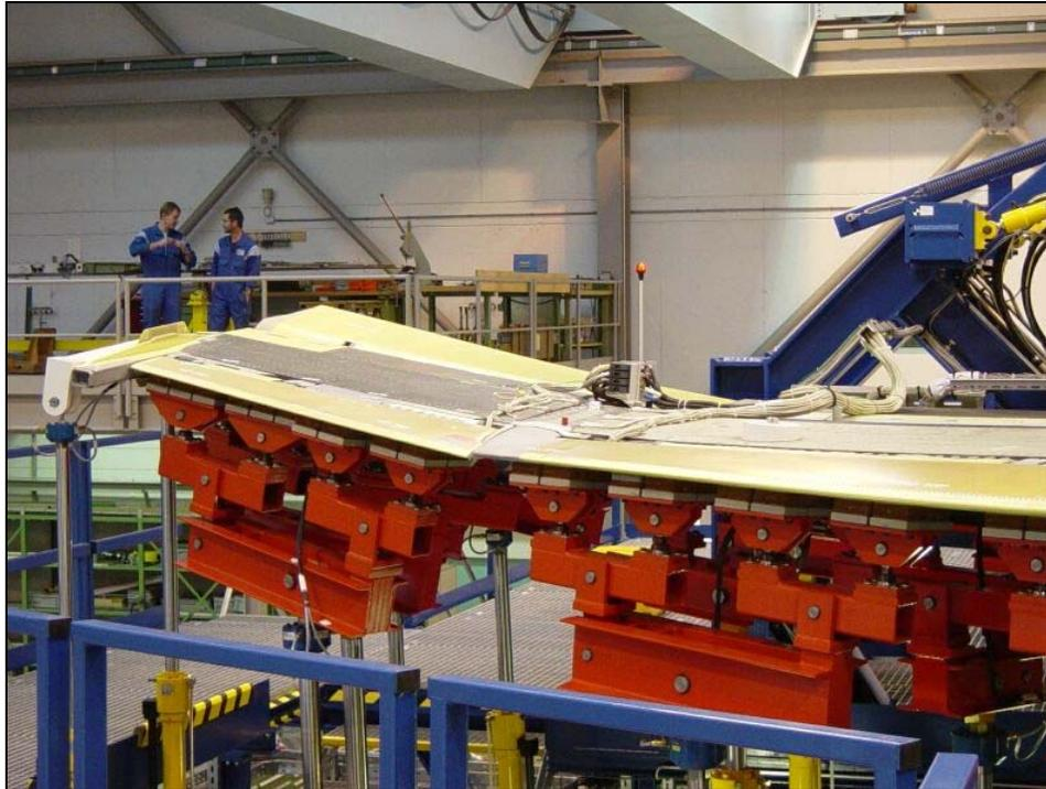
Figure 4.2-2 Wing displacement during strain survey at 70% load level of  $N_z = 8.25g$  symmetric steady state pull up maneuver.
