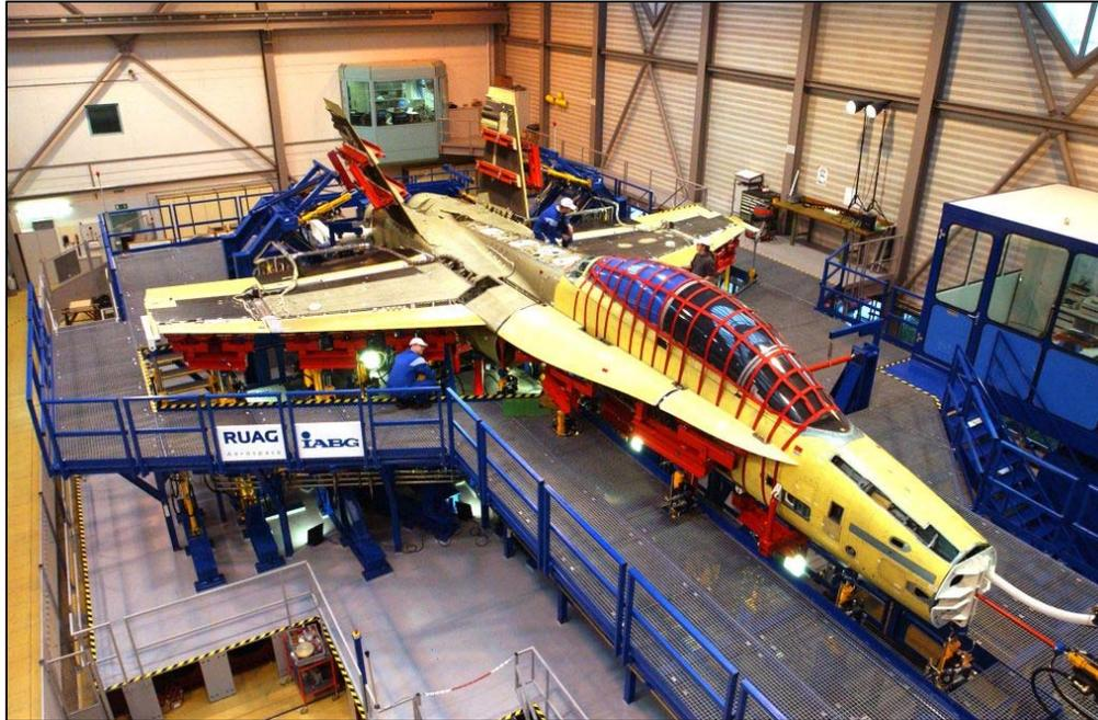
Figure 4.2-1 Test set-up of the Swiss full scale fatigue test.
