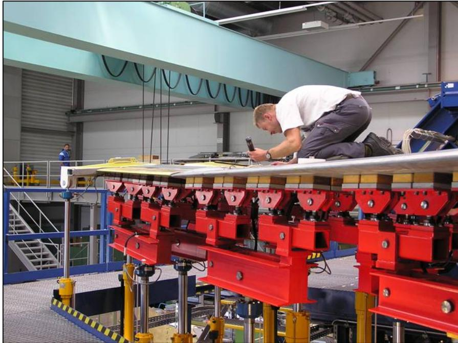
Figure 4.2-3 Inspection at wing fold during fatigue cycling, see deflected wing.
