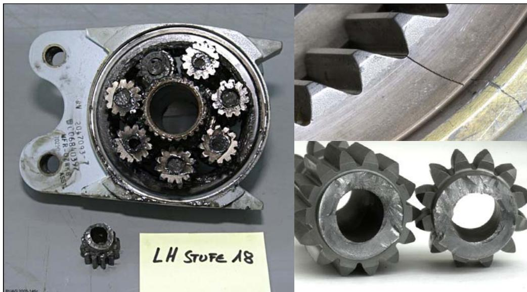
Figure 4.2-10 Cracks observed at wing fold transmission section 18.
