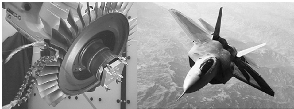
Figure 9.12-1 Production Laser Peening of Integrally Bladed Rotors (IBRs) for the F/A-22 Raptor Commenced at LSP Technologies, Inc. in March 2003. Red Laser Beams are Added Graphics to Illustrate the Process (left); the Actual Infrared Laser Beams are Invisible to the Human Eye. Laser Peening Increases the Damage Tolerance and Enhances the Fatigue Performance of This IBR.
