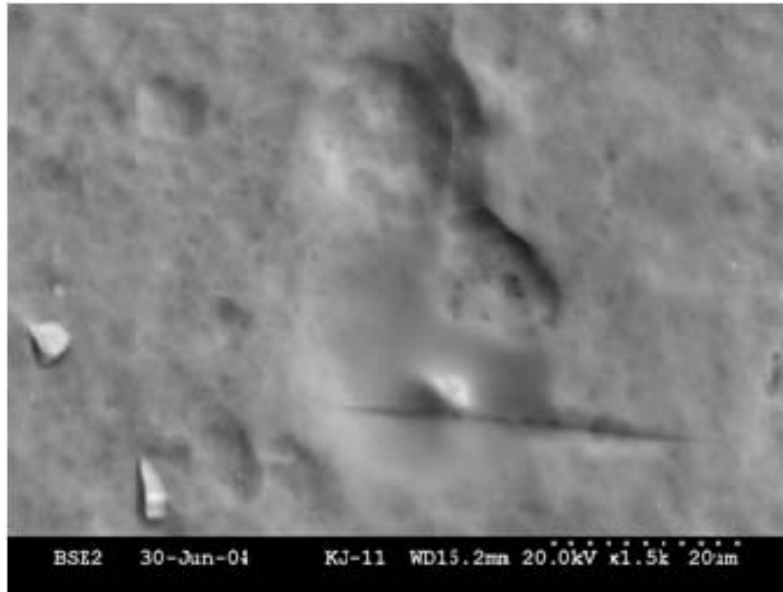
Figure 9.7-25 7075-T6-0.106" Specimen With a Constituent Particle Related Crack: Corrosion Aided in Material Removal Around the Particle, and Subsequently Crack Nucleation.
