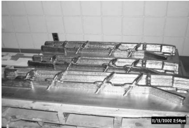
Figure 9.4-13 Sample Laser Deposited Part
