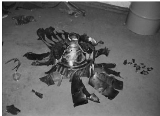
Figure 9.12-6 Fan Disk Failure Debris.
