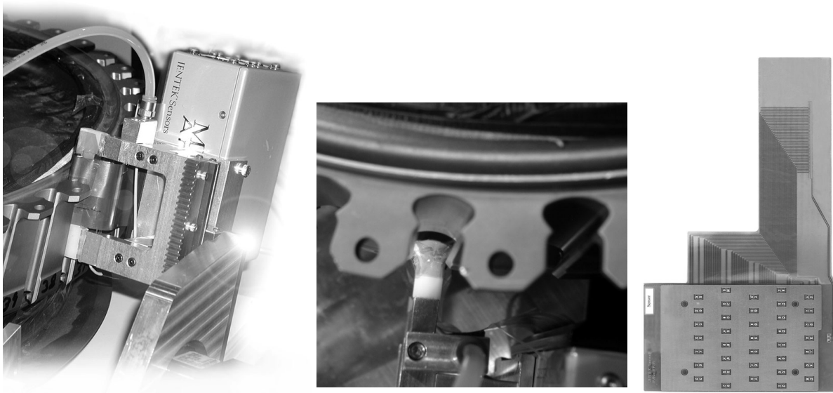
Figure 9.12-17 MWM-Array Probe Scanning Engine Disk Slot (left), Photo, Top View of MWM-Array Scanning Slot (middle), and actual MWM-Array FA35 Used for the Automated Disk Slot Inspection.
