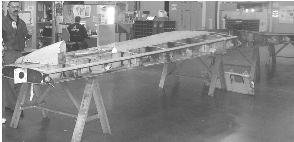
Figure 9.9-17 Horizontal Stabilizer in As-Received Condition.
