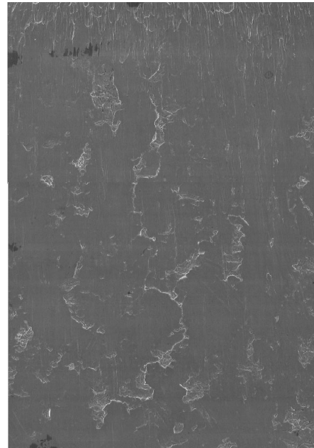
Figure 9.11-25 MWM-Array Response to a Fatigue Crack at the Right Side of the Slot Shown in Figure 9.11-24, and SEM Micrograph Showing the Detected 1 mm Crack.
