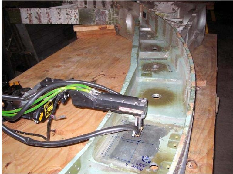
Figure 58 Measuring residual stress on a C-141 998 frame pocket with XRD.
