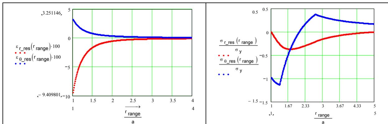
**Figure 18: Closed form solution for (left) residual strain and (right) residual stress after cold expansion**
