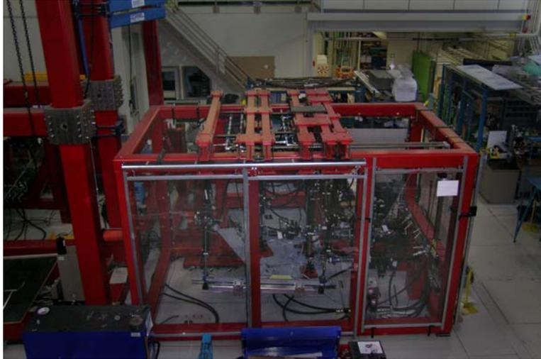
**Figure 2 FT-193 Extended Fatigue Test Set-up**
