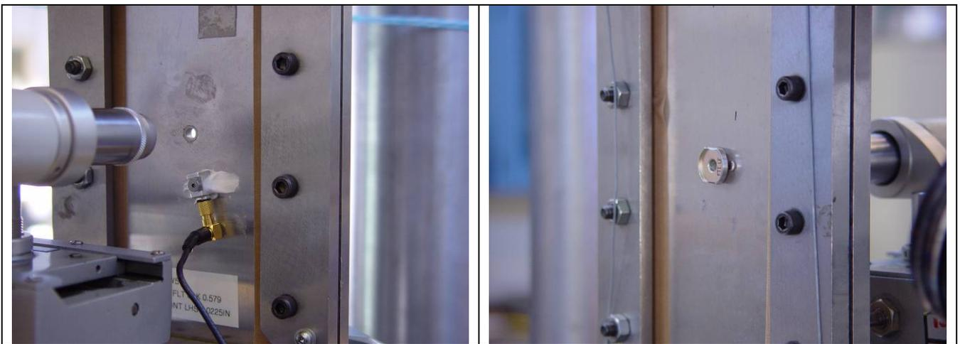
**Figure 56 Large edge margin coupons were assess the fatigue performance of dome nut and satellite rivet holes, versus a pre-cracked fastener hole with cold expanded FTI Forcetek collar.**
