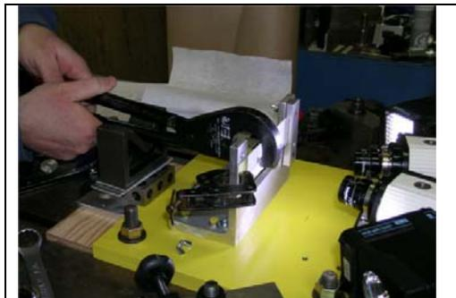
Figure 24: Manual riveting process with a GLARE coupon
