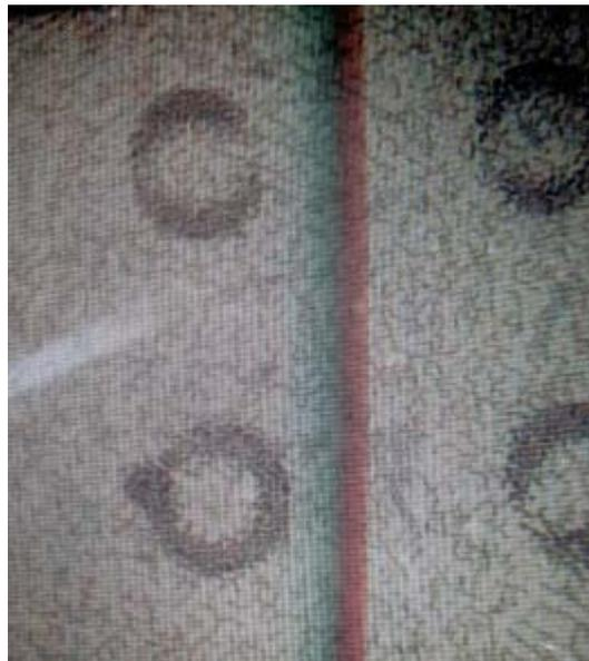
**Figure 70 MOI image of 4 rivet holes inspected.**
