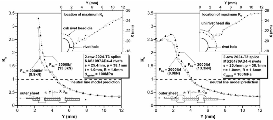
Figure 9: Comparison of maximum secondary bending factor ( $K_b$ ) magnitude and location for countersunk and universal rivet splices.
