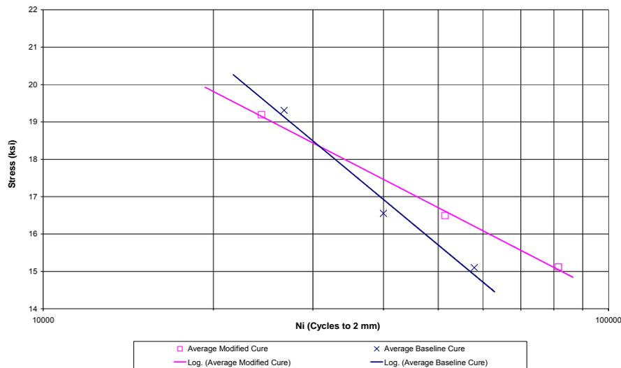
**Figure 37: Summary of low  $K_t$  fatigue test results for NRC-IAR baseline and modified cure cycle FML specimens.**
