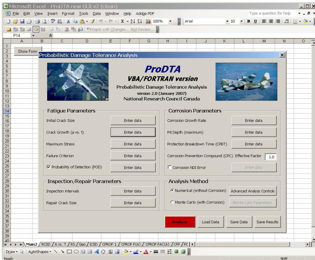
Figure 41. A prototype GUI of ProDTA embedded in MS Excel spreadsheet.
