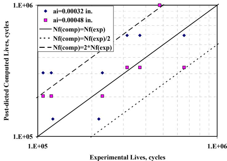
Figure 36. Rivet Lap Joint Computed Lives as Function of Experimentally Measured Lives.
