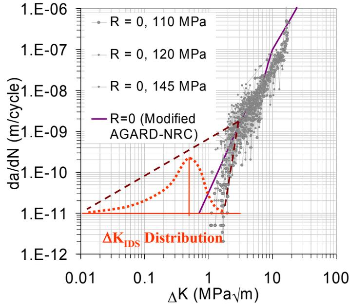
Figure 28 Schematic of a  $\Delta K_{IDS}$  distribution with the modified AGARD-NRC model and some AGARD data.
