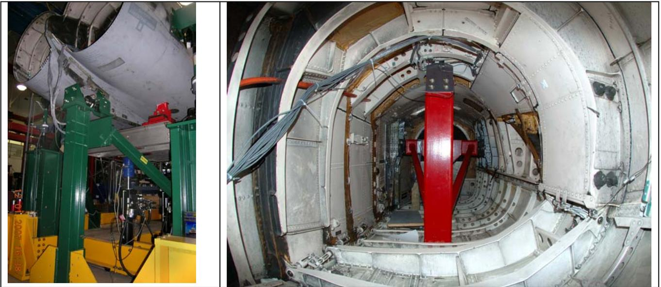
**Figure 6 F/A-18 FT865 CF-18 Aft Engine Mount Structure Fatigue Test Set-up and Starboard Side Attachment**
