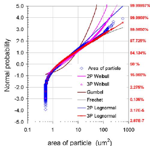
**Figure 42 Goodness-of-fit plot of distributions on Normal probability paper (e.g. unclad 2024-T351 0.063” sheet, ST plane)**
