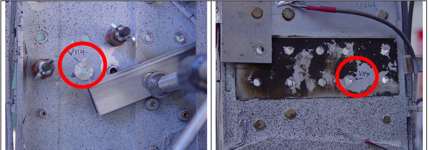
**Figure 55 Repair of hole V114 by offset oversizing followed by hole cold expansion and shrink fit bushing repair (no new cracks redeveloped in this location).**
