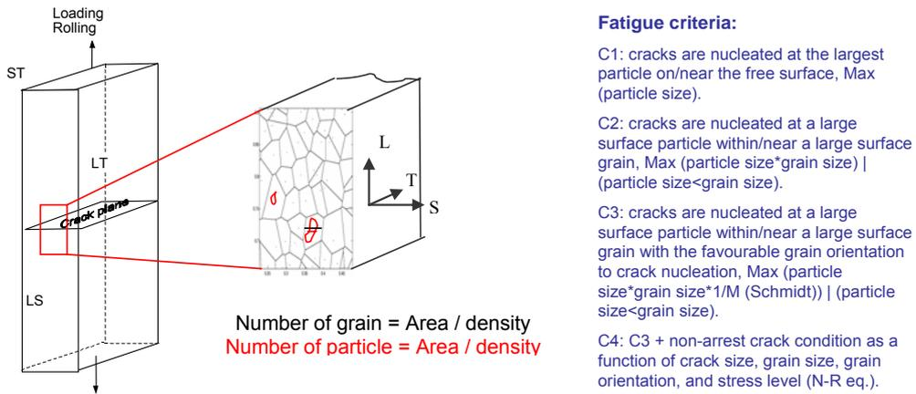
Figure 44 Schematic particle and grain structure on fatigue critical area (LS plane)
