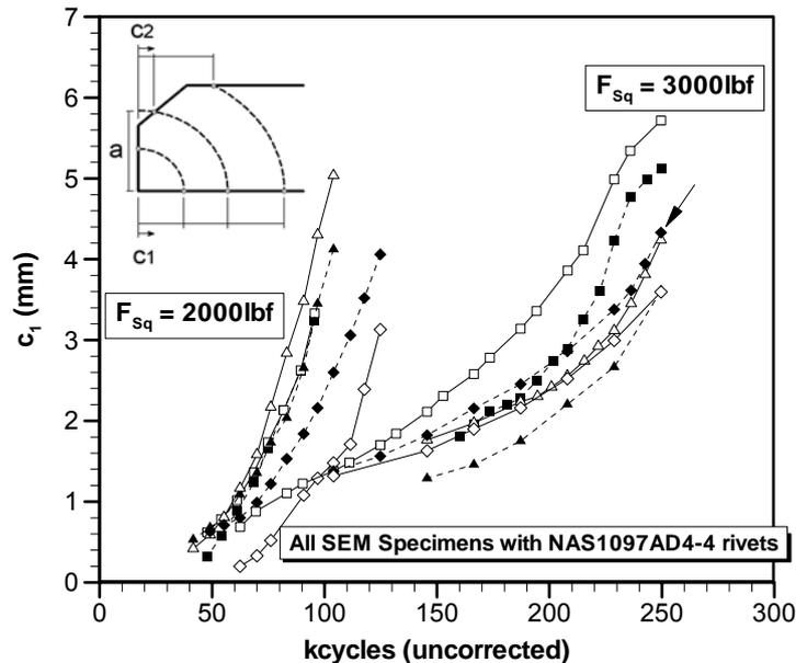
Figure 11: Comparison of crack growth curves for countersunk rivet lap joints.
