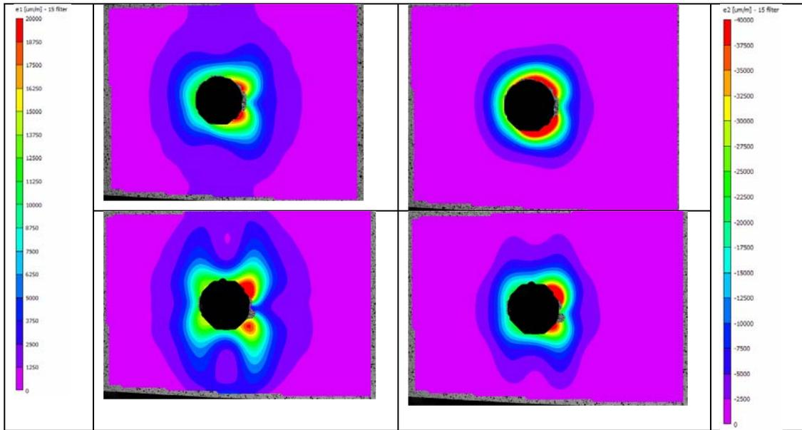
Figure 22: Comparison of cold expansion in aluminum (top) and GLARE (bottom)
