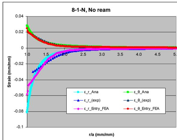
Figure 23: Comparison between experimental, closed form and FEA results
