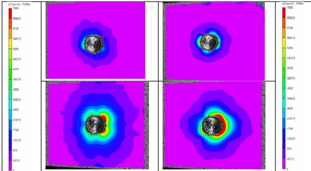
Figure 25: Comparison of riveting in aluminum (top) and GLARE (bottom)
