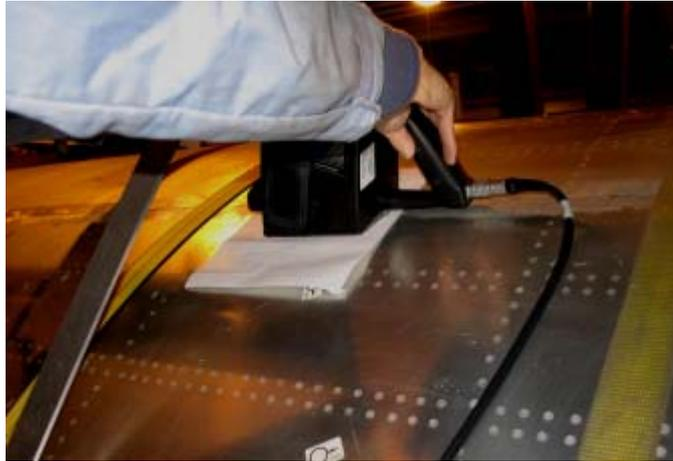
**Figure 69 Magneto-optic inspection head.**
