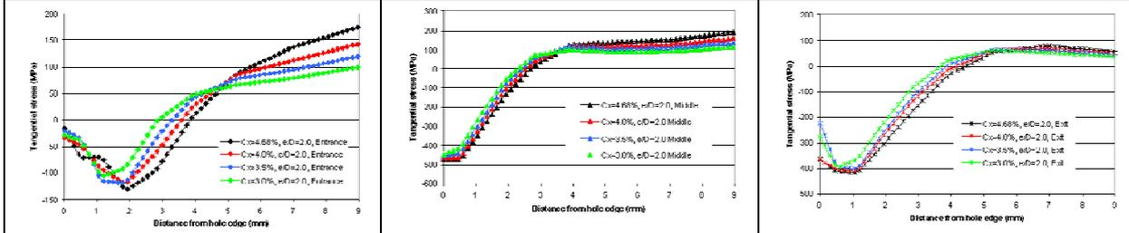
Comparison of residual stresses with different hole cold expansion levels at the entrance (left), middle (middle) and exit (right) surfaces along the narrow edge.
