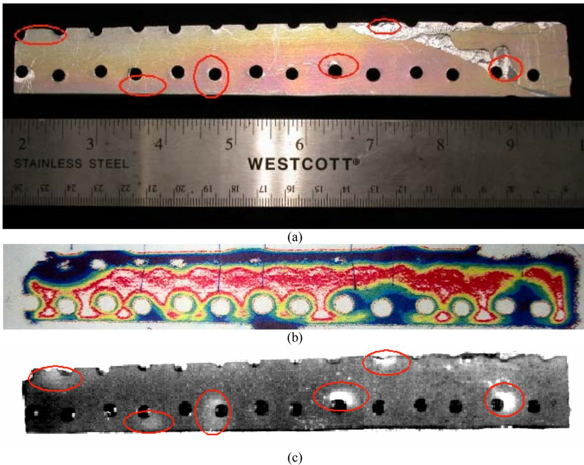
**Figure 65 A photograph of the lower stringer– aft flange containing stress corrosion cracks (a). Ultrasonic C-scan image of the above part (b). Thermal image of the above part obtained by pulsed phase thermography showing stress cracking sites (c).**
