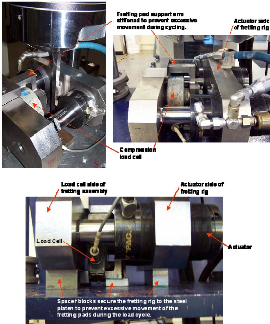
**Figure 31. Photographs of redesigned fretting rig.**
