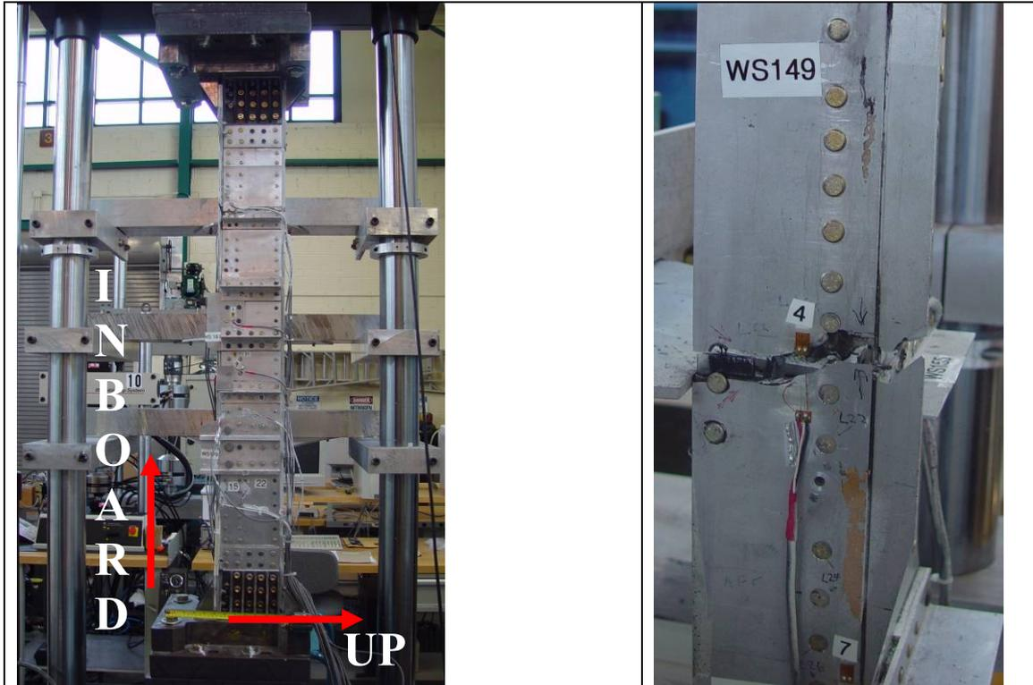
**Figure 54 The WS167 test article: aft view (left) and the failure in the lower wing skin (right).**
