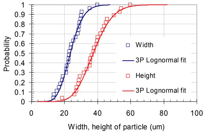
Figure 43 IDS fatigue subsets: combined particle width & height distributions (unclad 2024-T3, 0.063, 0.16, 0.5 at 40, 44, 48 ksi, R0.05, R0.1)
