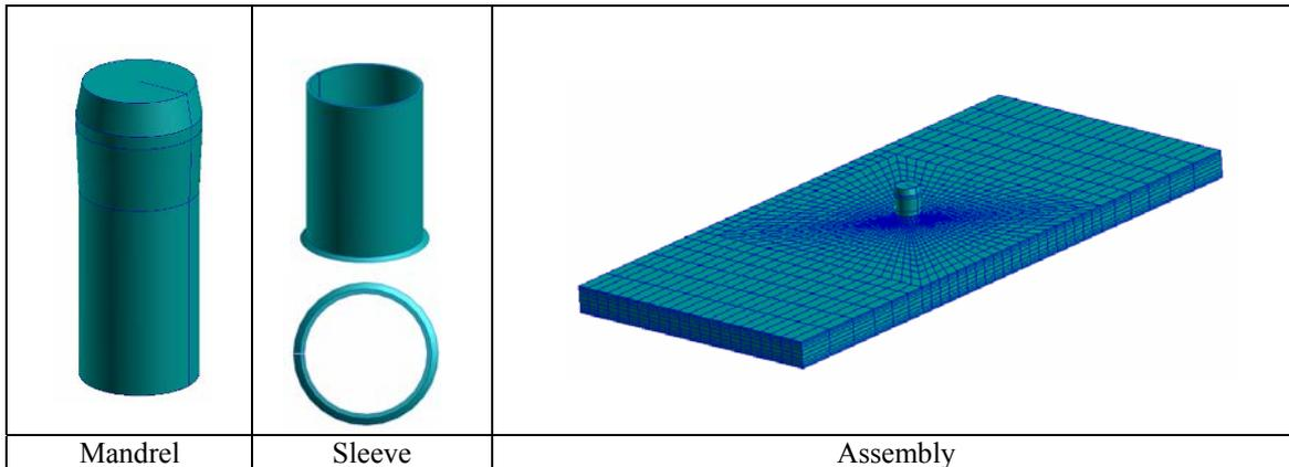
**Figure 14** Parametric finite element models of all aspects of the hole expansion process have been developed and validated with experimental digital image correlation results.
