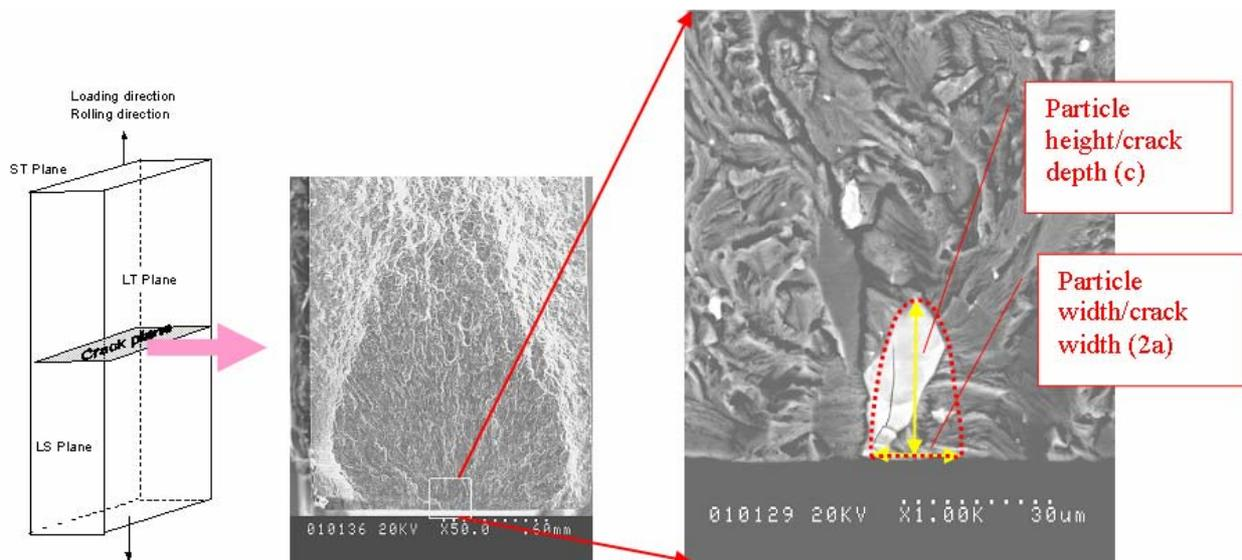
**Figure 27 Fracture surface and crack-nucleating particle based crack model.**
