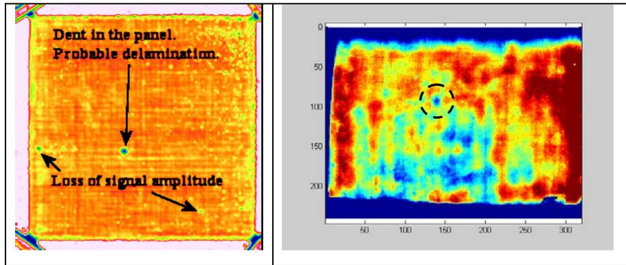
Figure 19: NDI results (left) ultrasonic C-scan (right) thermography
