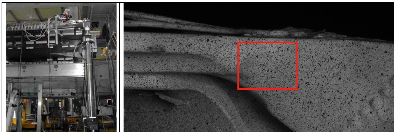
**Figure 4 FT-312 CF-18 Wing-Fold Aft-Spar Shear-Tie Test Set-up and Critical Area Post Blend**
