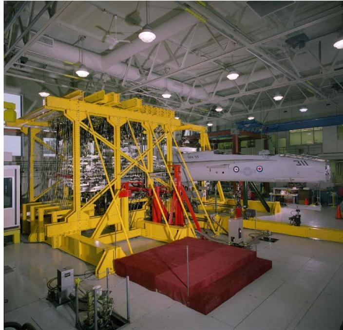
**Figure 1 FT-245 Wing Fatigue Test**
