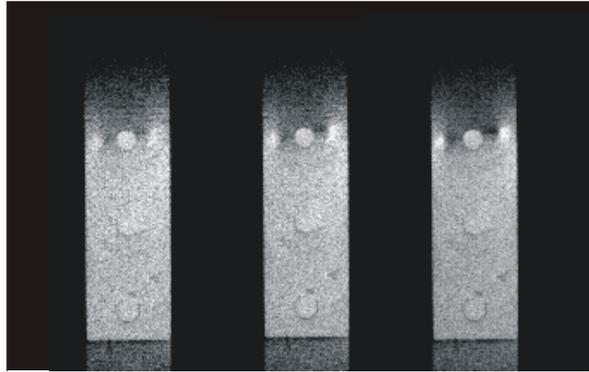
Figure 61. Raw thermal images of specimen #10 during loading at 143,000, 145,000, and 147,000 cycles (from left to right). The crack tips are visible as bright spots (higher temperatures) on either side of the top rivets.
