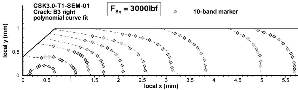
Figure 10: Typical crack front plot resulting from crack reconstruction for a lap joint with high rivet squeeze force.
