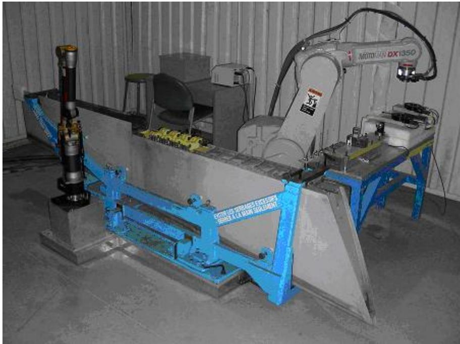
**Figure 51** Robotic Material Removal Modification on the Inboard Leading Edge Flap
