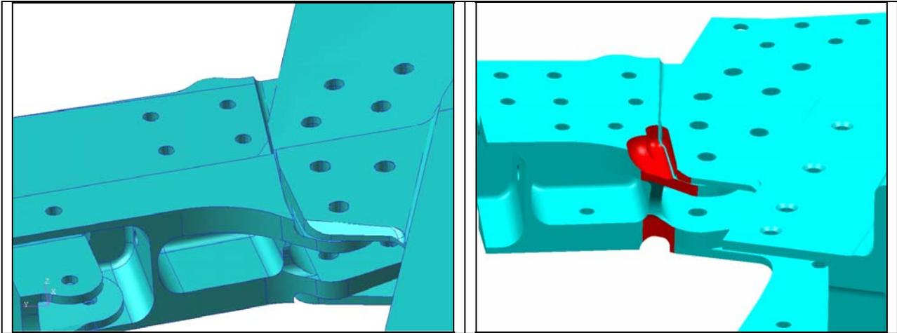
**Figure 48 Outer Wing Front Spar – Pre-Mod & Post-Mod**
