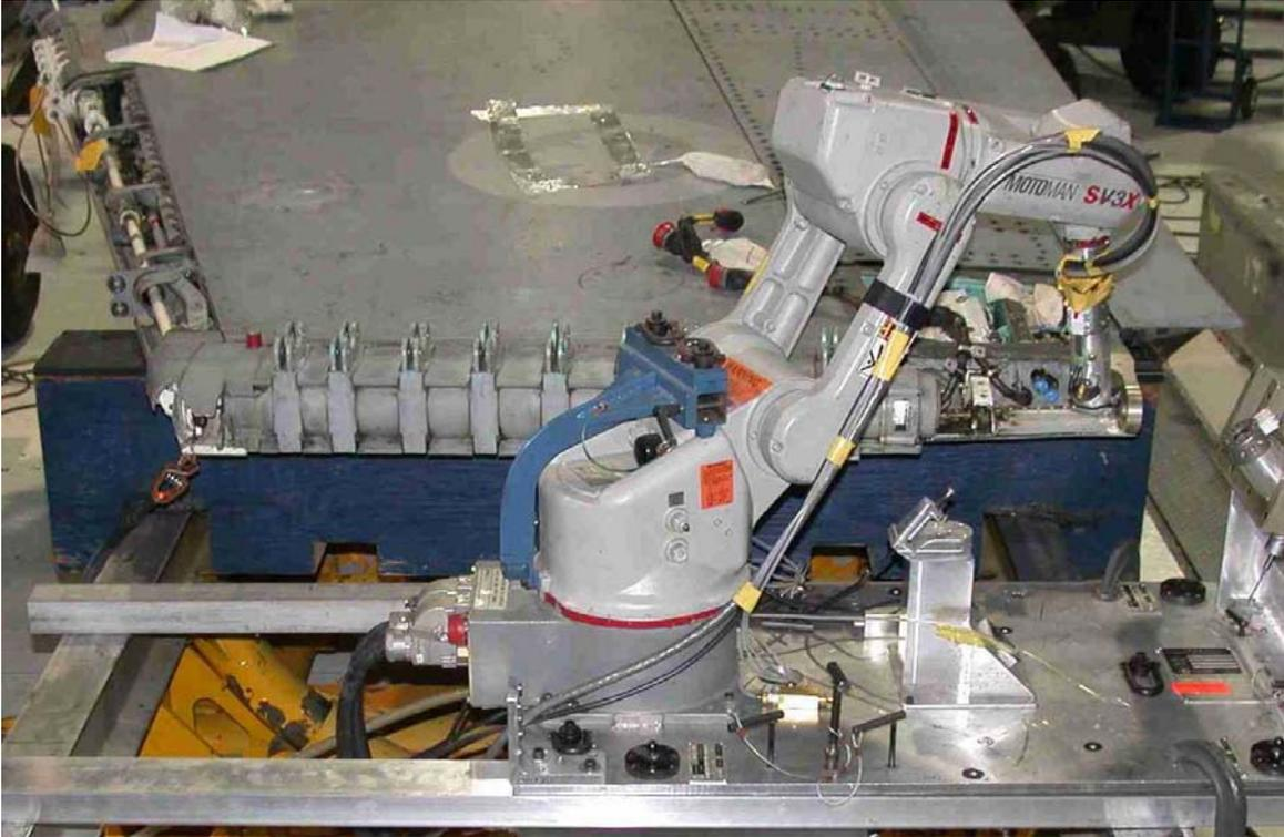
**Figure 50** Robotic Material Removal Modification on the Inner Wing
