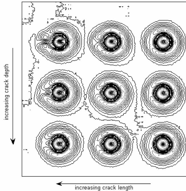
**Figure 68** C-scan contour plot of the overall surface (tangential) magnetic field. Open contours indicate disruption in the magnetic field due to cracks.
