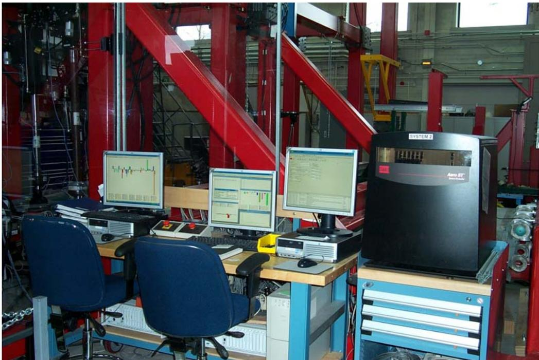
**Figure 8 F/A-18 FT193 MTS's AeroPro™ and SOFFT Control System Set-up Adjacent to the Rig**
