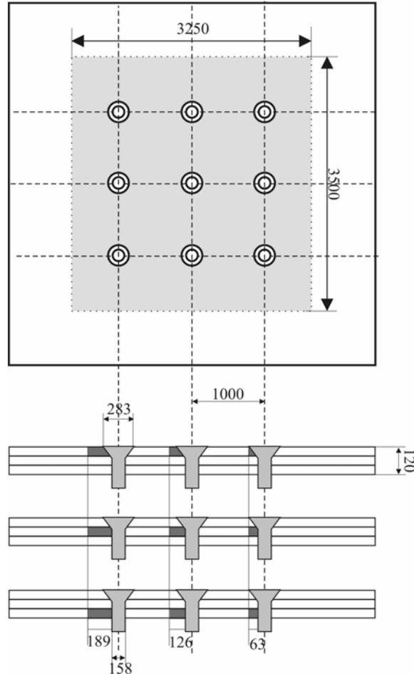
**Figure 67** Schematic diagram of the three-layer lap joint specimen containing simulated cracks (all dimensions are given in thousands of an inch, 1 inch=25.4 mm). Shaded area represents the scanned surface.
