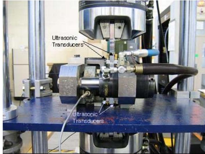
Figure 32. Test setup showing test coupon containing ultrasonic transducers.
