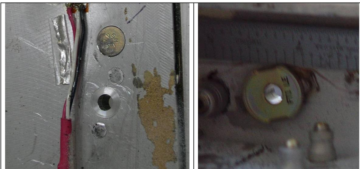
**Figure 57 Two Forcetek Rivetless Nut plates that were successfully tested in the WS167 component spectrum fatigue test.**
