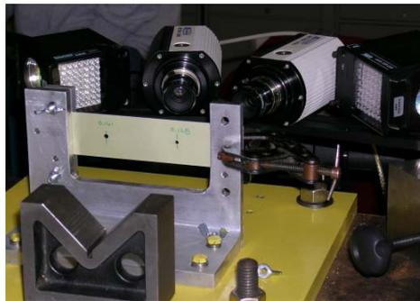
Figure 20: Coupon test fixture with camera and lighting system
