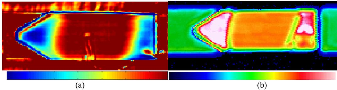
**Figure 66. Pulsed infrared thermal image of disbond (a). Ultrasonic C-scan image of the same disbond**
