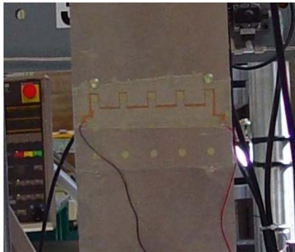
**Figure 35. Passive sensor for the early detection of cracking.**
