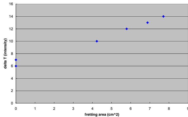
Figure 62. A plot of the difference in apparent temperature (arbitrary units) between the detected hot spots and the surrounding area as a function of the fretting damage measured after teardown.
