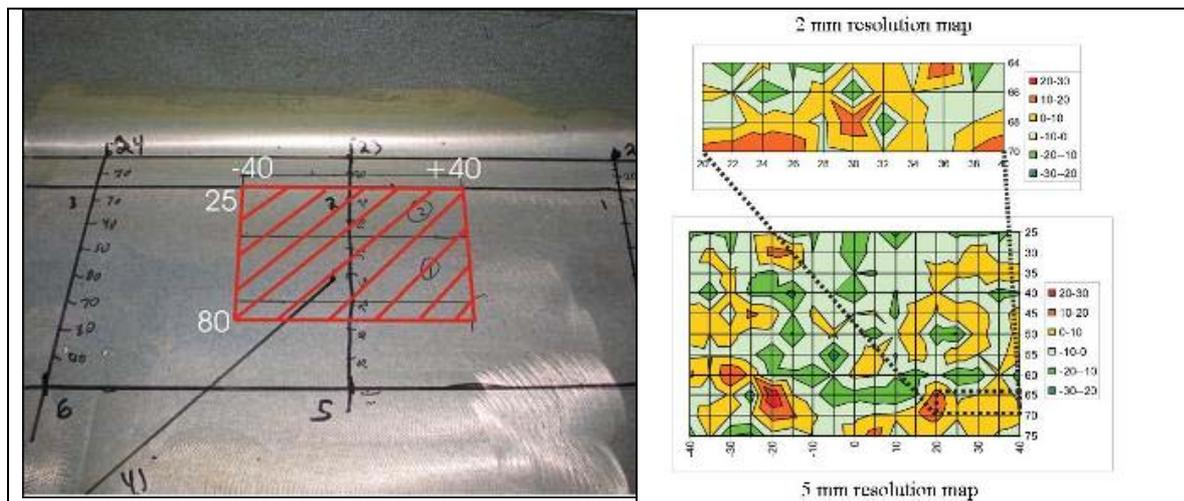
Figure 59 Residual-stress map of C-141 998 Frame pocket.
