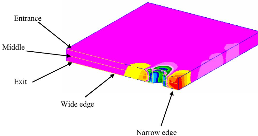
**Figure 15** showing the tangential stress path across the thickness of the parametric FEA model.
