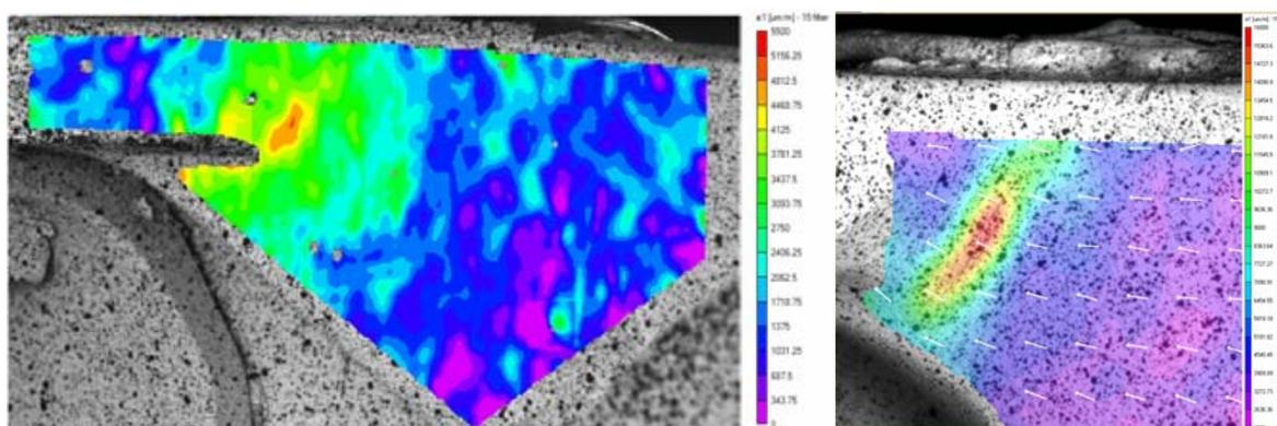
**Figure 5 FT-312 CF-18 Wing-Fold Aft-Spar Shear-Tie Principal Strains Measured Pre-Test and 11201 SFH Post-Modification**
