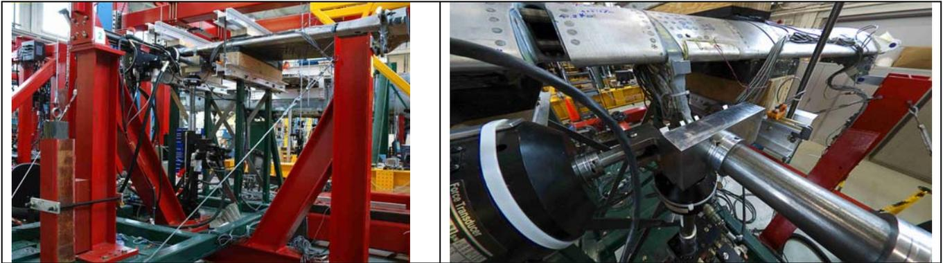
**Figure 7 F/A-18 FT333 CF-18 Trailing-edge Flap Outboard Lug Fatigue Test Set-up and Tri-Axial Lug Hinge Attachment**
