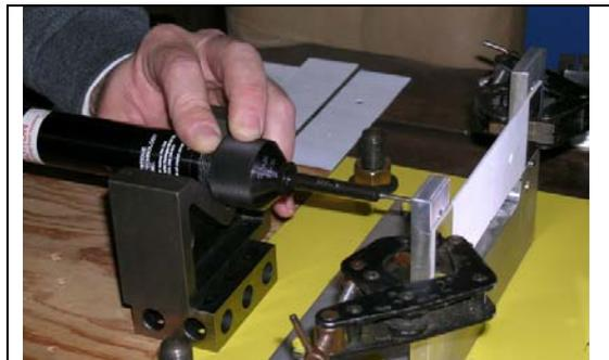
Figure 21: Cold expansion process for aluminum coupon
