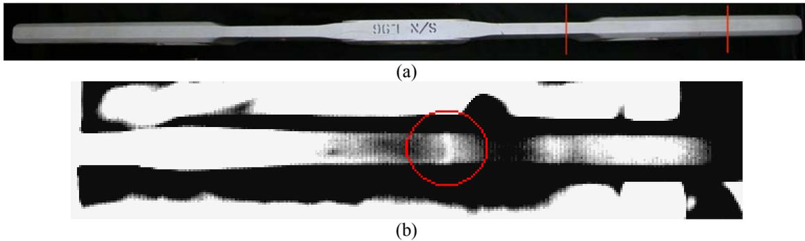
**Figure 64. A photograph of a tail rotor half-hub side view (a). Pulsed thermography inspection results showing crack in carbon fibre frame (b).**
