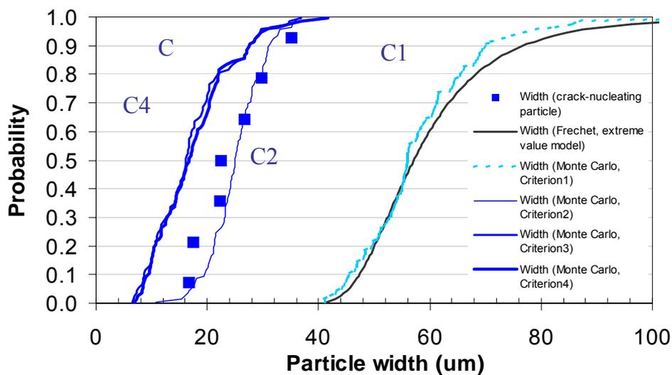
Figure 45 IDS fatigue subsets prediction and test (e.g. 2024-T3/0.063”),  $\sigma_{max}$  44ksi, R0.1, similar results were obtained for 0.063”, 0.16”, and 0.5” at other stress levels.
