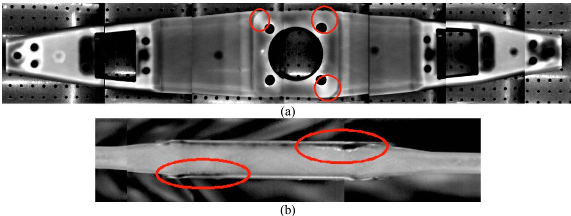
Figure 63. Pulsed thermography inspection results (a) top view and (b) side view showing delamination
