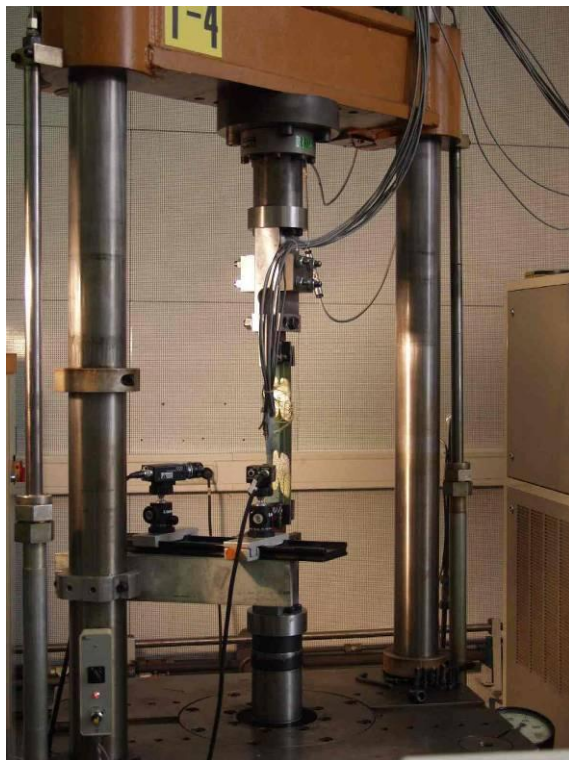
Figure 32 Clip welding - coupon in the test rig
