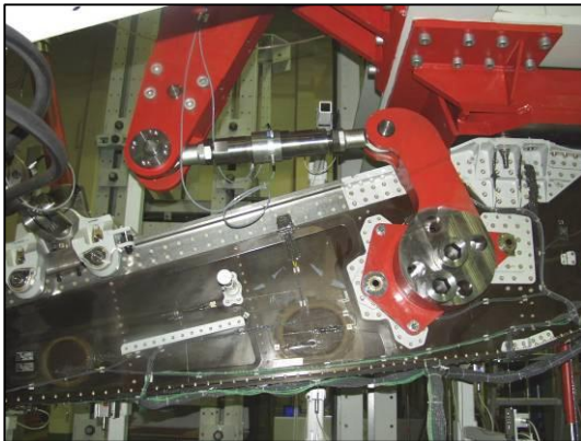
Figure 6 Rotary drive dummy for load introduction in A380 Flap Track Tests
