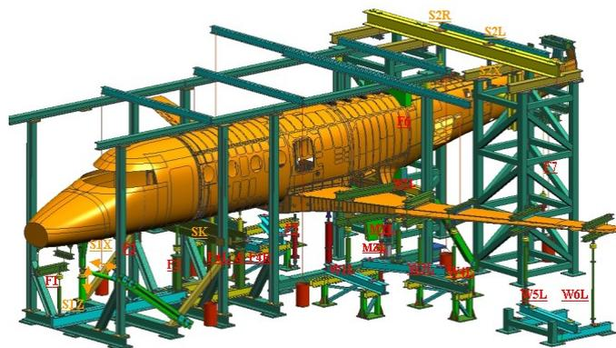
**Figure 11: Schematic Representation of the G150 Full-Scale Fatigue Test Setup**
