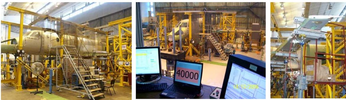
**Figure 12: G150 Executive Jet Full-Scale Fatigue Test (Center Photo: After Completing 40,000 Flights)**
