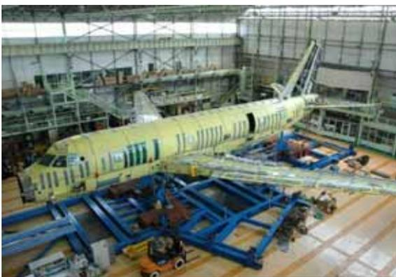
**Figure 12.39 P-X FSST Test Article**
