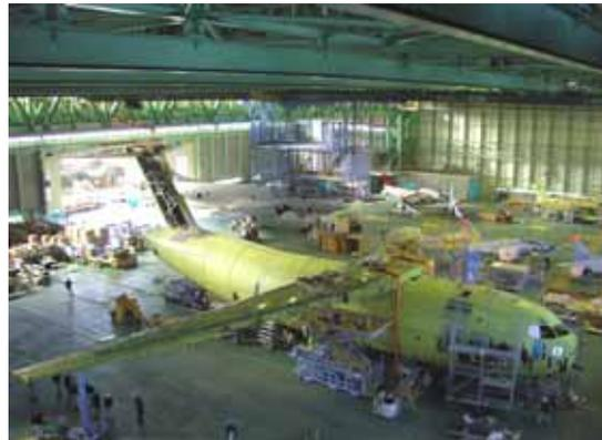
**Figure 12.40 C-X FSST Test Article**
