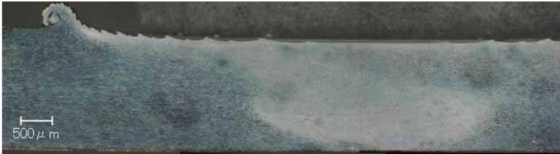
**Figure 12.5 Section Perpendicular to the Welding Line**
