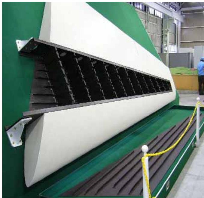
Figure 12.35 Proto-Typed Vertical Stabilizer Box Structure
