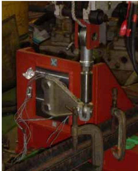
**Figure 12.12 Actual-Sized Element Test (Pitch Horn)**
