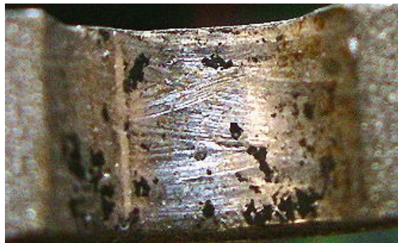
Fig. 5.1.1. Fretting wear at the rivet hole.
