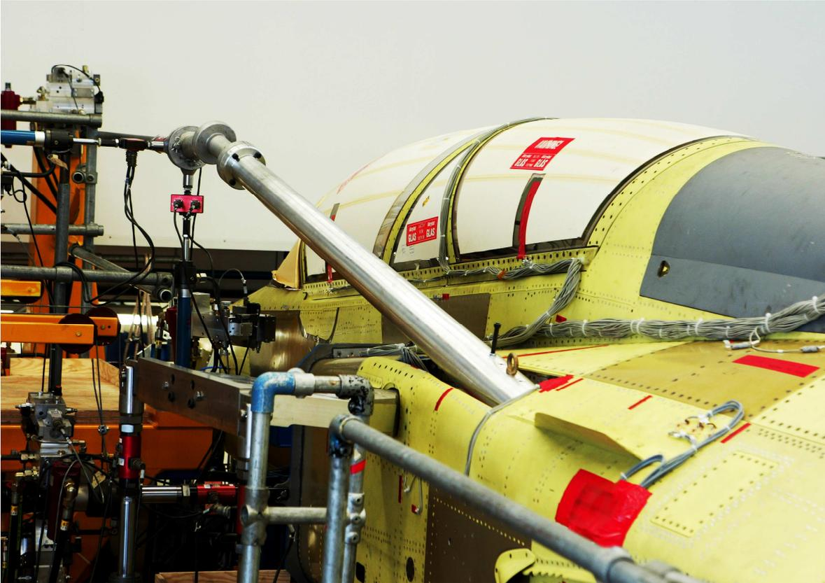
Figure 14. Photograph of the forward fuselage, D version, with the air-to-air refuelling probe dummy.
