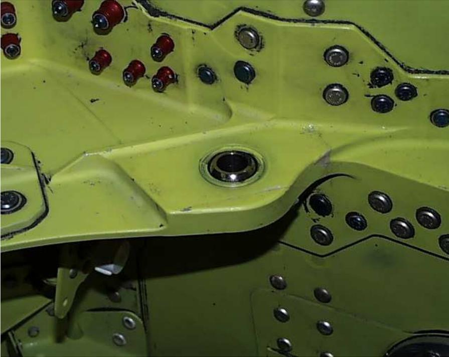
Figure 15. Cracked lug for the attachment of the actuator for the main landing gear door
