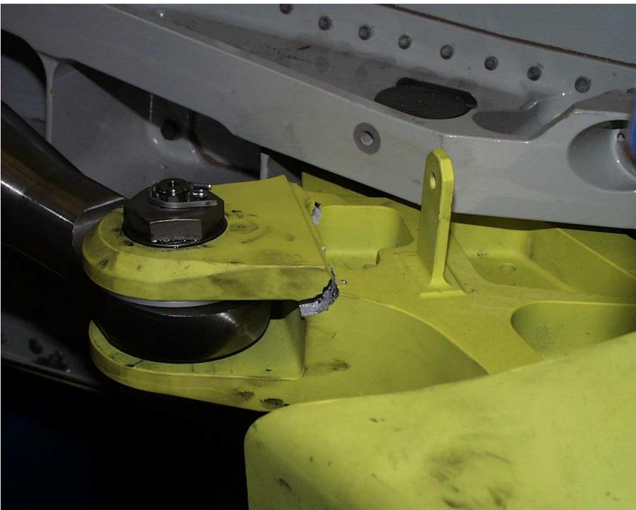
Figure 16. Cracked lug for the attachment of the actuator to the air-brake
