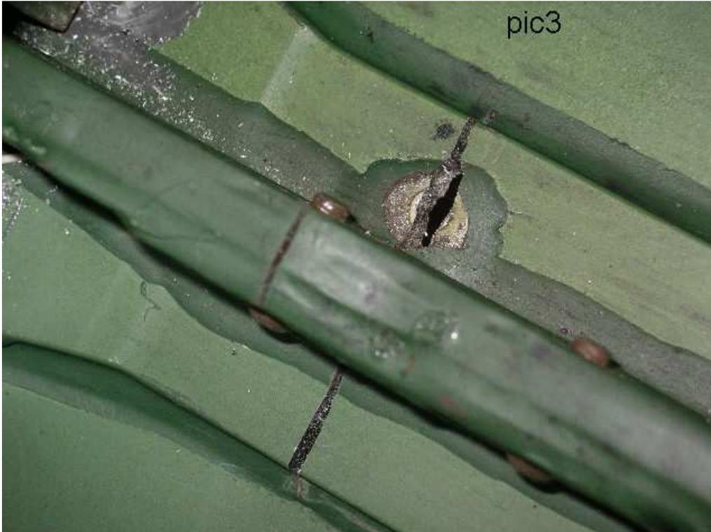
Figure 9. Saab 2000 Artificial crack in lower wing skin with an broken stringer
