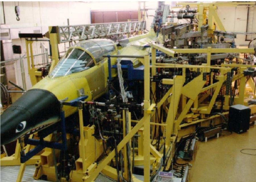
Figure 11. Photograph of the full scale fatigue test of the Gripen single seater, 39A.
