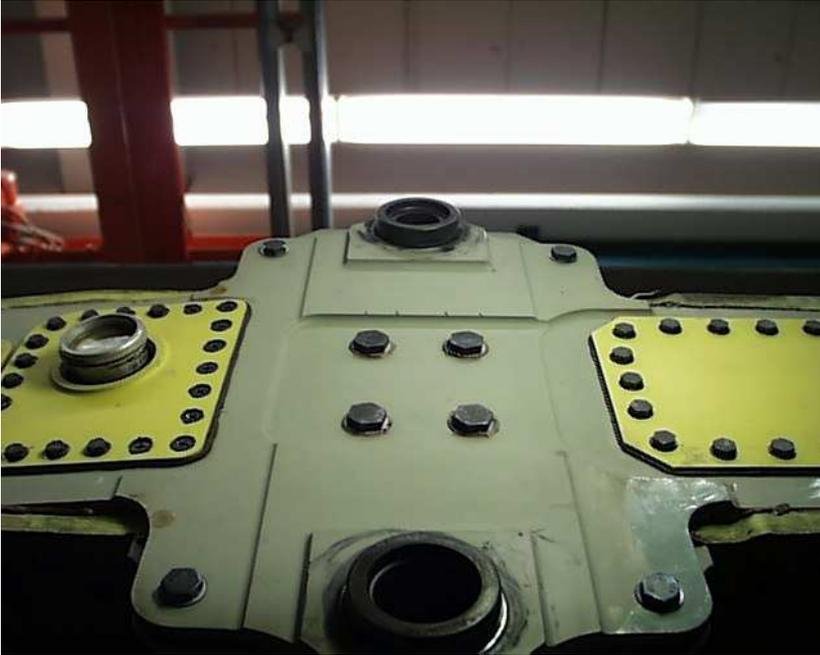
Figure 12. Surface cracks in radius in the root rib of the main wing due to residual stresses from assembly.
