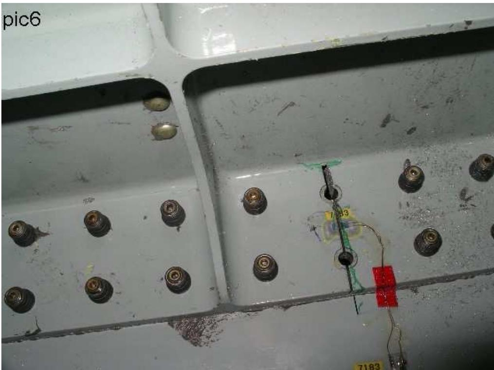
Figure 10. Saab 2000 Artificial crack in lower forward wing spar cap and in skin
