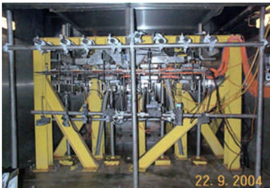
Figure 8 RTM Aileron in Environmental Chamber
