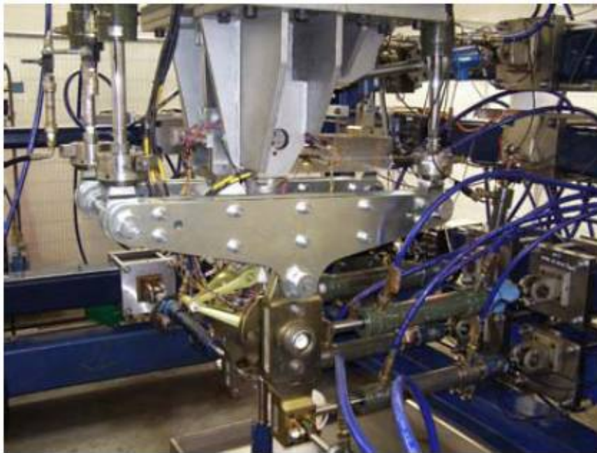
Figure 9 Harrier II main landing gear fatigue test
