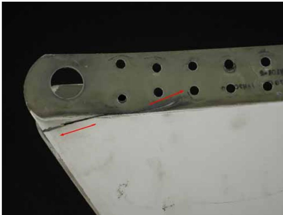
Figure 9.10-1 Crack in Rear Fairing
