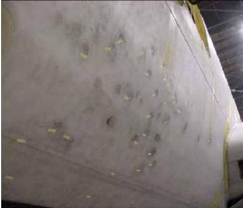
Figure 9.4-4 Typical Dents in Fuselage Structure
