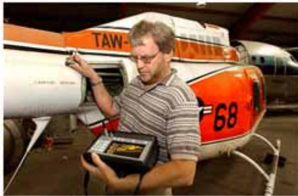
Figure 9.8-2 Crack Detection Application on 206 Tail Boom Using Modified Eddy Current Sliding Probe (Walking Probe) to Inspect Lap Joint
