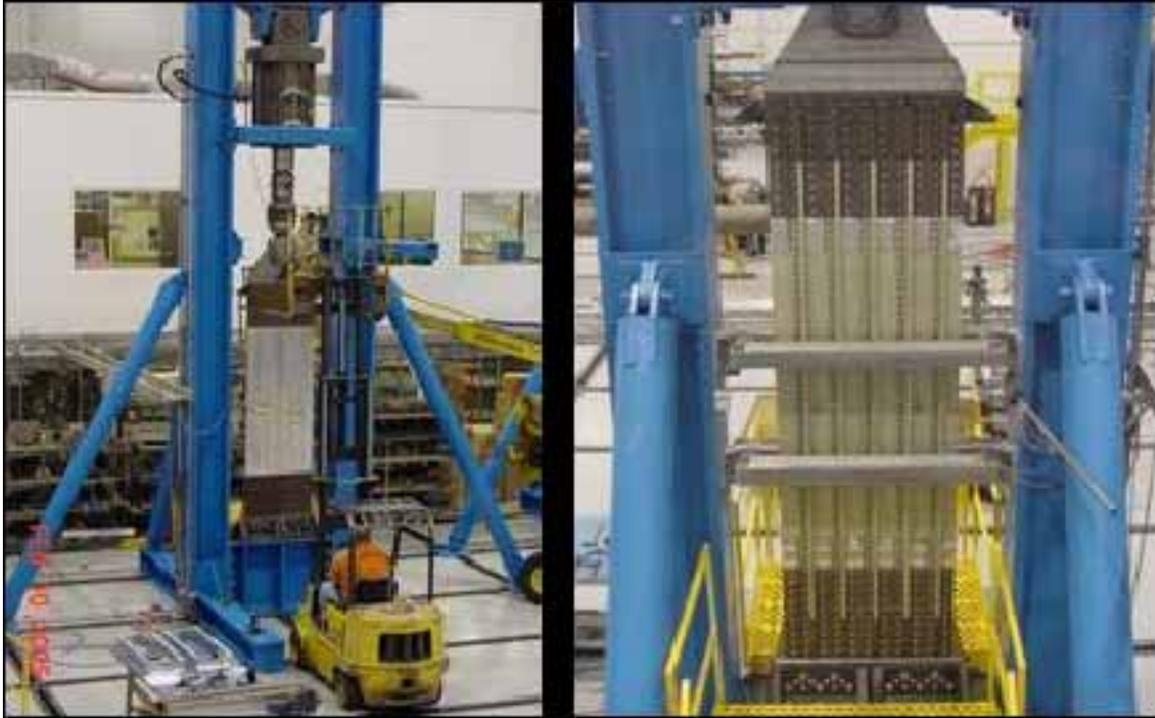
Figure 9.12-6 Alcoa Large-Scale Proof-of-Concept Testing - Adv. Lower Wing
