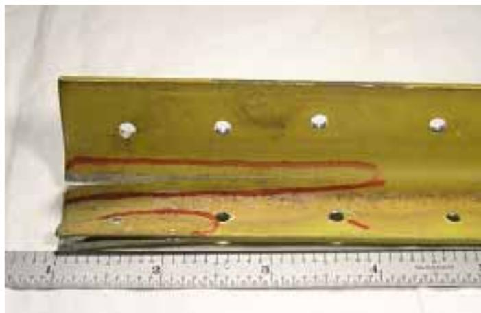
Figure 9.7-1 SCC and Exfoliation Damage Findings From T-37B Teardown Program Phase I
