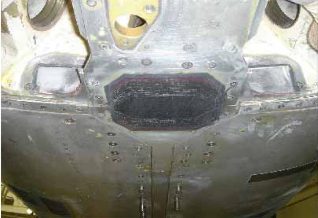
Figure 9.2-5 Bulkhead Bonded Repair
