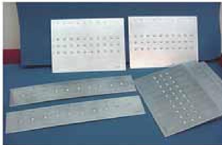
Figure 9.8-1 Example of POD Test Specimens Used in Blind Study
