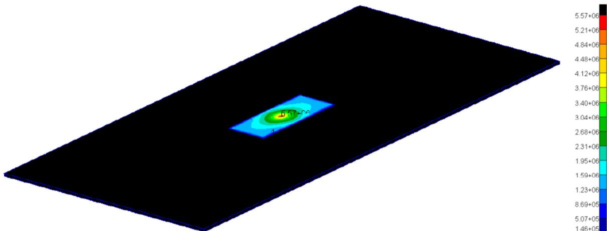
Figure 2 Modelled energy harvester, spring-steel cavity floor with centrally mounted SFC transducer. Stress distribution over 90 mm harvester under ( $F = 1$  N). Note: only stress of transducer crystal material displayed.
