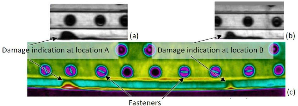
Figure 2 Non-destructive inspections of areas on bonded composite joint with known damage indications using (a)/(b) pulse echo ultrasonic inspection and (c) flash thermography
