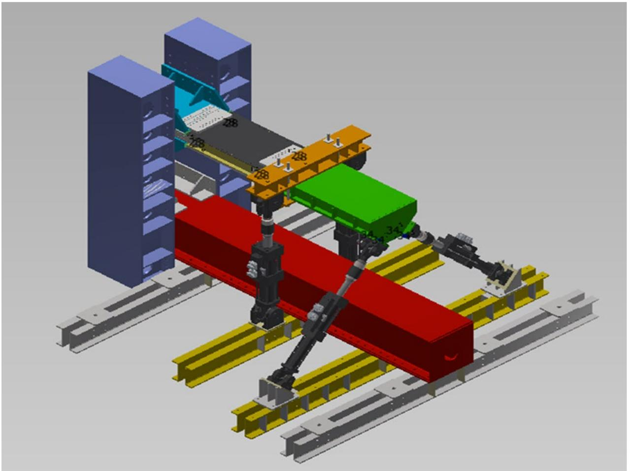
Figure 1 The large-scale aerospace multi-axial structural test capability design.
