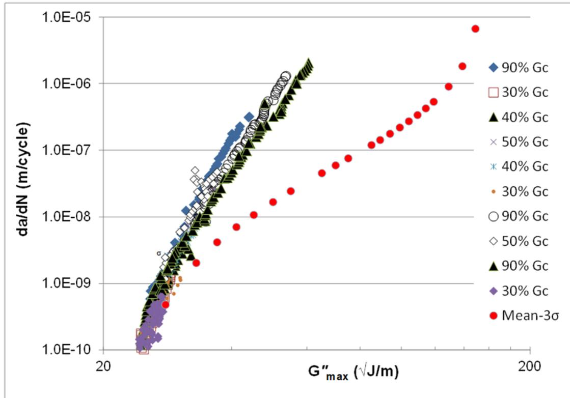
Figure 2 The 'threshold' normalised delamination growth curves for IM7-9773 and the upper bound (mean -  $3\sigma$ ) curves, from [3]. This is the same data as shown in Figure 1.
