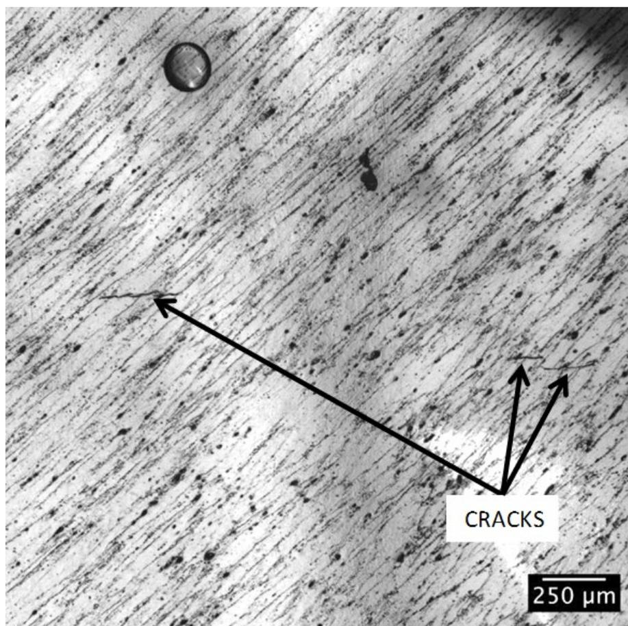
Figure 1 Fatigue cracks detected by acetate replica inspection in aluminium service structures.
