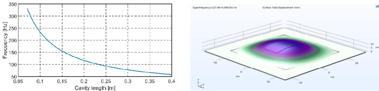
Figure 1 Rossiter analytical model of acoustic frequencies produced by cavity, and modelled fundamental mode at ~330 Hz for cavity-floor with bonded SFC
