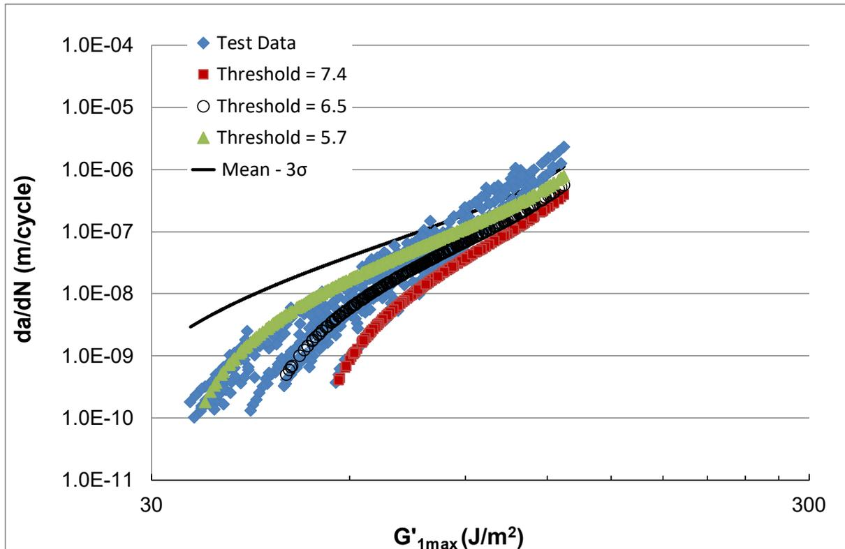
Figure 1 The 'toughness' normalised delamination growth curves for IM7-9773 and the upper bound (mean - 3σ curves, from [3]).
