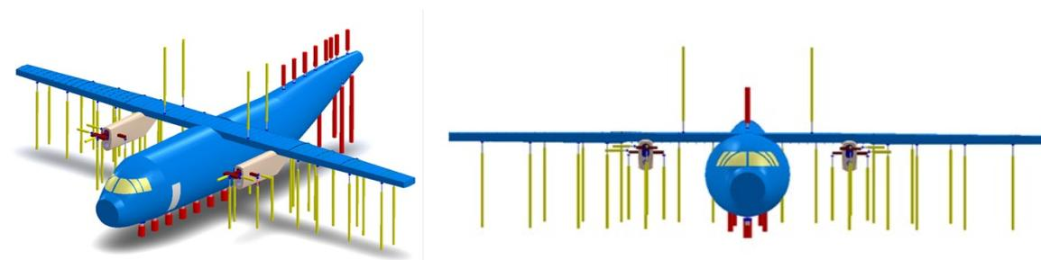
Figure 1 Representation of possible test actuator locations for the C-27J FSFT
