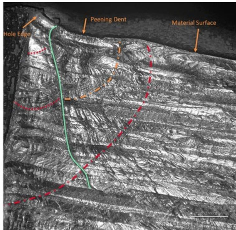
Figure 1 Example of Crack Initiation at the base of peening dent. Crack initiation locations at edge and dents annotated.
