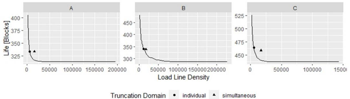
Figure 2 Effect of omission on life for various locations. Points show the effect of individual (local) versus simultaneous (global) omission for a select load line density.
