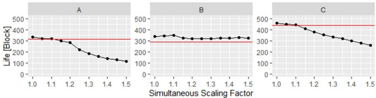
Figure 3 Effect of simultaneous (global) scaling on Life for various airframe locations (red line represents target life)
