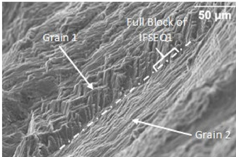
Figure 3 A high angle SEM image of the fracture surface of a specimen subject to the IFSEQ1 spectrum. Clear variations in surface features are observable across two different grains, suggesting a reliance on grain orientation
