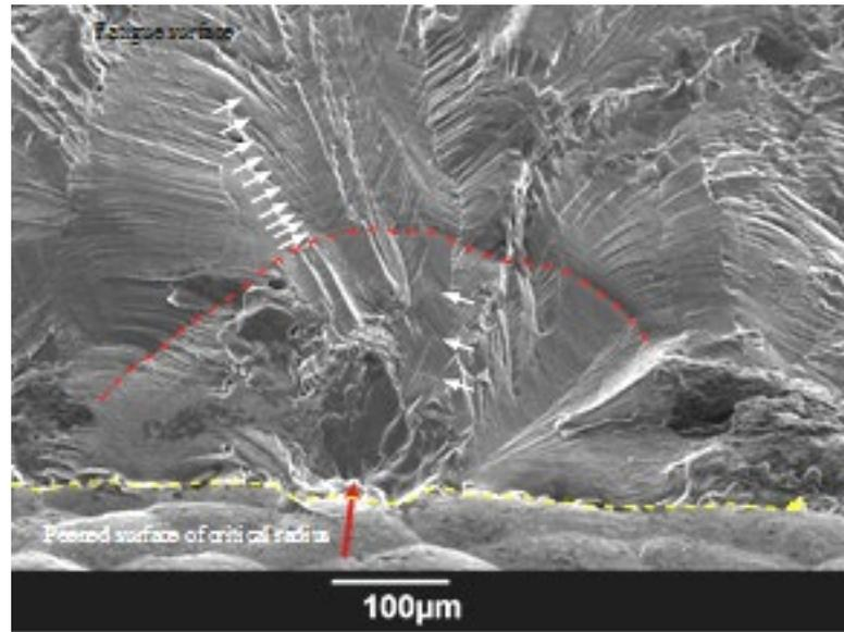
Figure 2 The origin region of crack KDIJ-03a. The original initiating discontinuity is marked with a red arrow, while the size of the crack at the time the repair was applied is indicated with a red dashed line. Crack growth progression marks (indicated with white arrows) have a much smaller spacing after the repair indicating the slower rate of crack growth. The peening dents on the surface of the coupon can be observed in the lower portion of the image.
