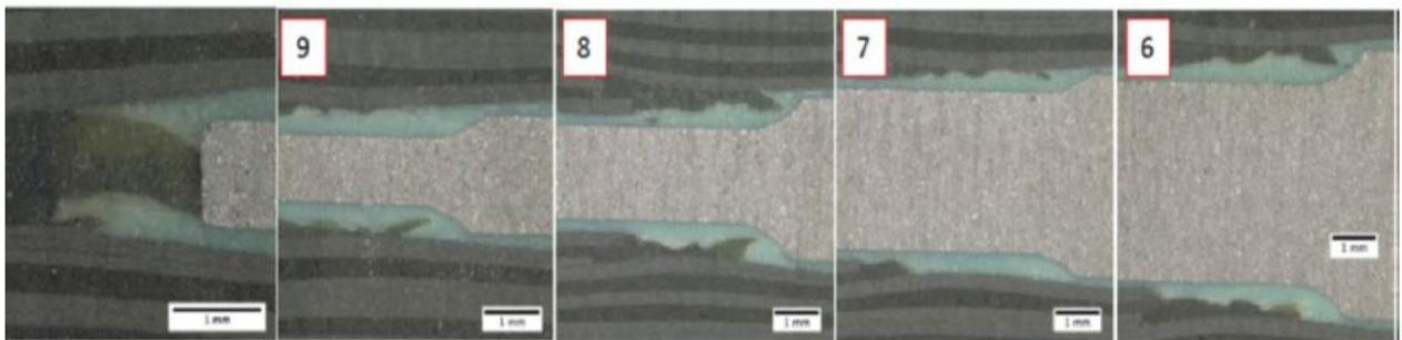
Figure 1 Optical micrograph of section through titanium to composite bonded step lap joint
