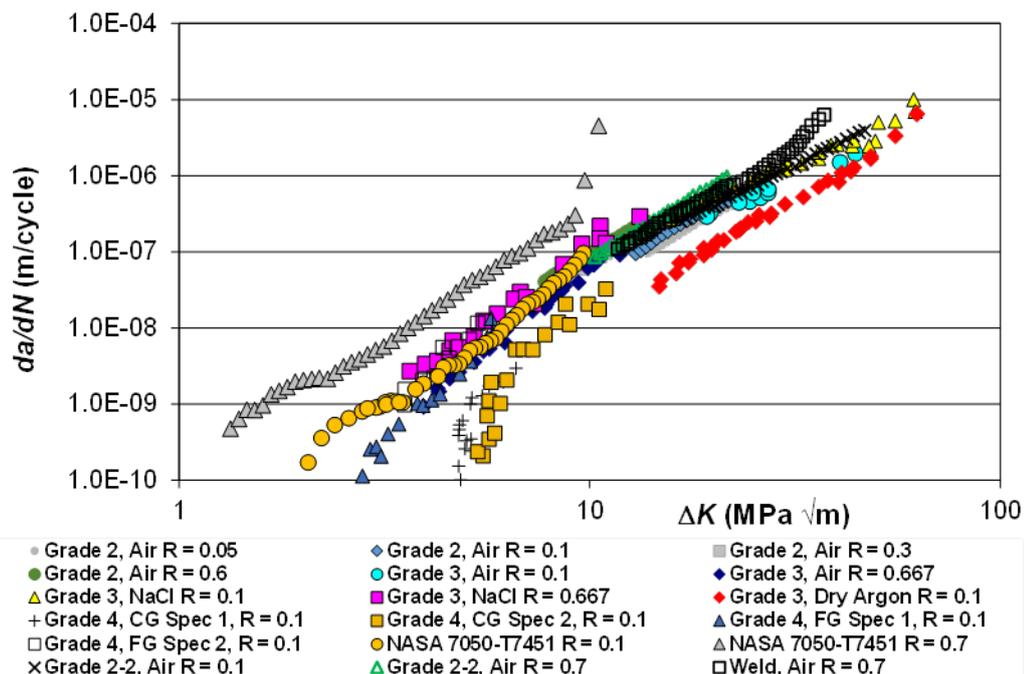
Figure 1 Crack growth in CP titanium and 7050-T7451
