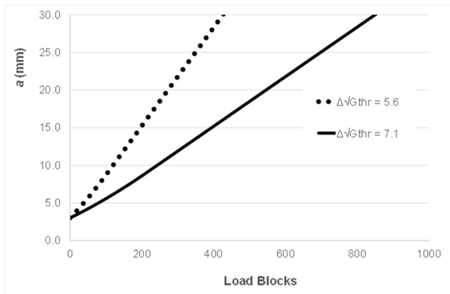
Figure 2 Predicted crack length, a, histories as a function of the number of load blocks for the specimen tested under a FALSTAFF flight-load spectrum with a remote maximum stress of 193.5 MPa
