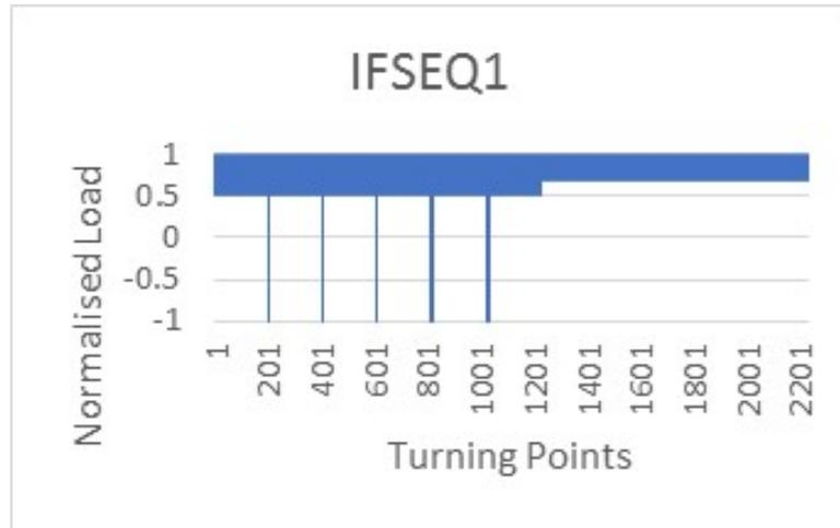
Figure 1 Normalised spectra IFSEQ1, designed to elucidate the effects of multiple underloads in succession. The spectrum consists of increasing numbers of underloads in succession (1-5), each followed by 100 cycles (200 turning points) of  $R = 0.5$  loading. 500 cycles of  $R = 0.7$  loads are applied at the end of each block to act as an additional marker band.
