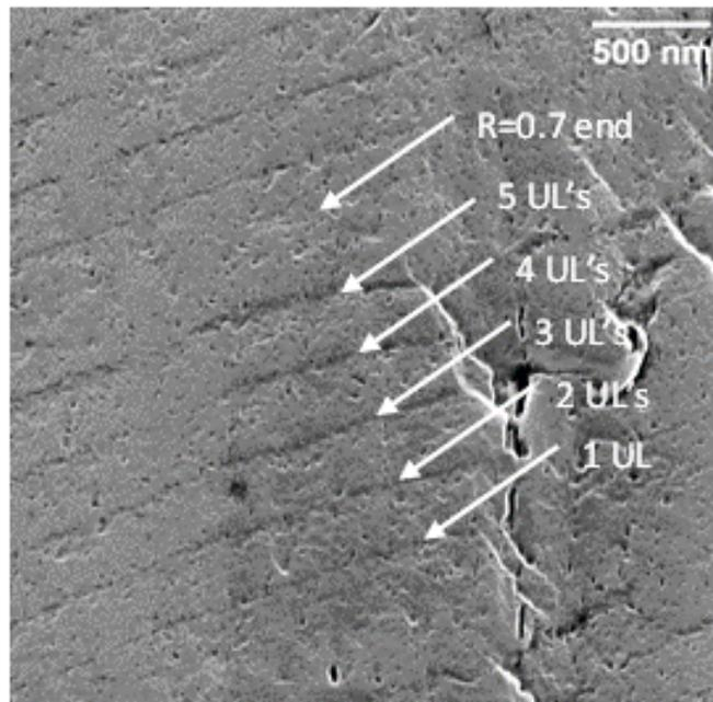
Figure 2 HIM image taken at an overall crack length of  $140 \mu\text{m}$ . This specimen was subject to IFSEQ1 spectrum, and the dark bands clearly define the locations of the underloads. The  $R = 0.5$  cycles are growing the crack at a little more than  $1 \text{ nm}$  per cycle. Rubbing has damaged the surface, but better images are expected with improved experimental techniques.
