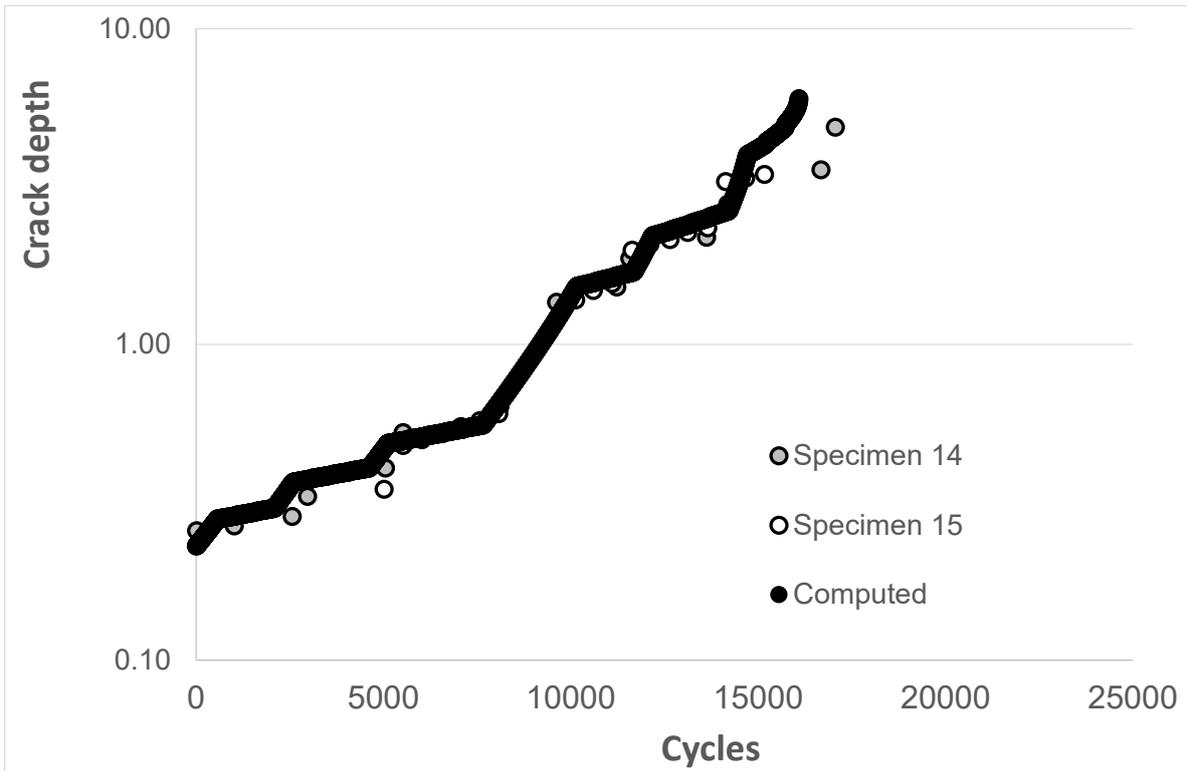
Figure 4 Durability analysis results for the baseline AerMet100 steel tests
