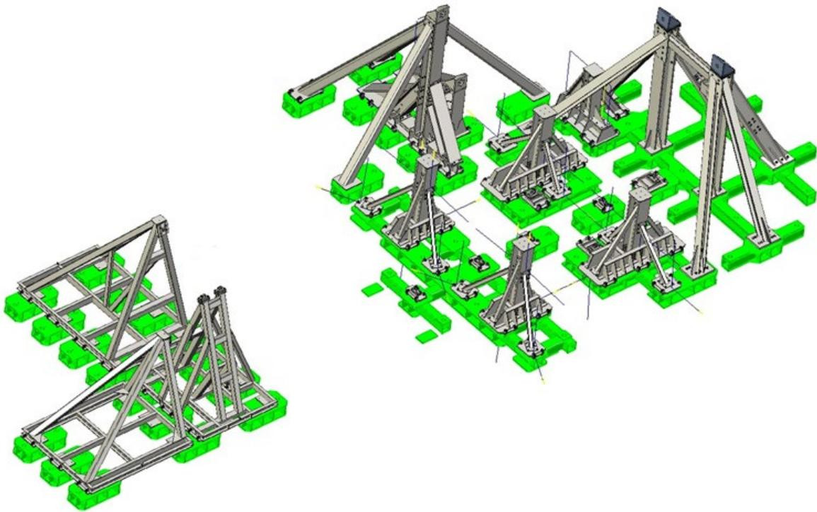
Figure 1 The HAFT-TD full-scale rig design
