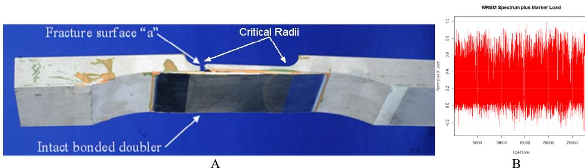
Figure 1 (A) The coupon designed to represent a critical radius detail on a bulkhead. This image of a coupon after fracture, showing the coupon had separated, however the doubler remained intact and bonded to each half of the coupon. (B) The fatigue spectrum plus marker load applied to the coupons.
