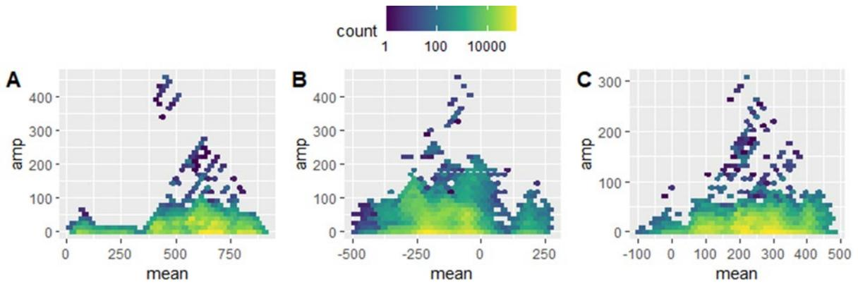
Figure 1 Rainflow density plots for three helicopter airframe locations (units MPa)
