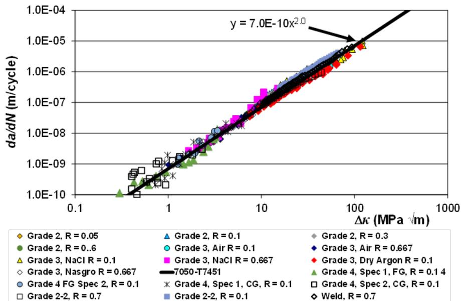
Figure 2 Crack growth curves replotted
