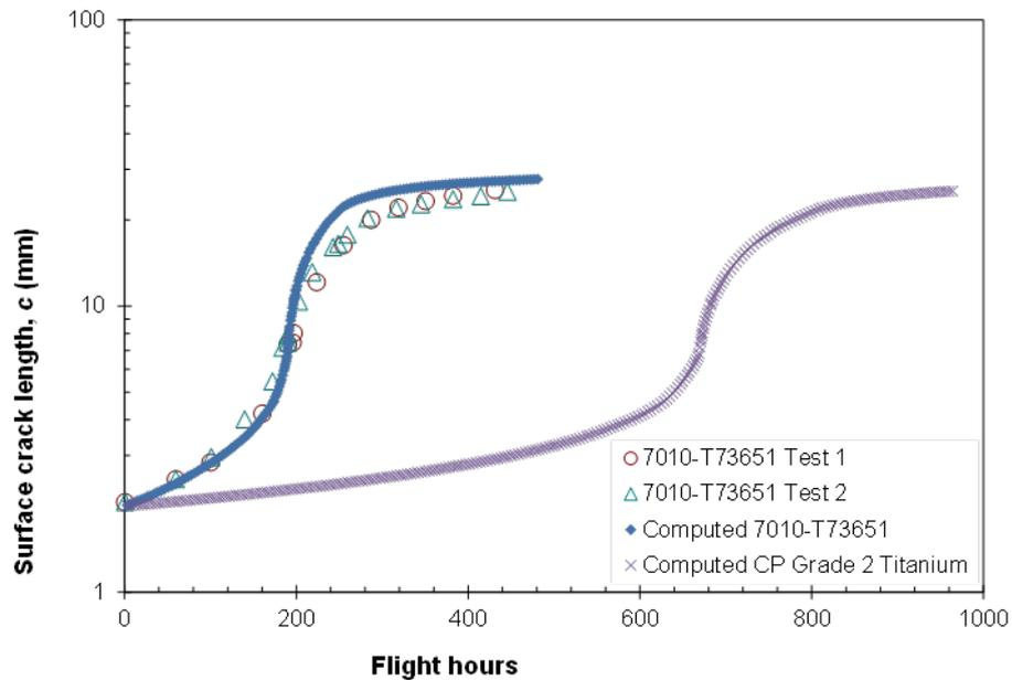
Figure 3 Computed lives for a 7010 and a CP titanium lift frame
