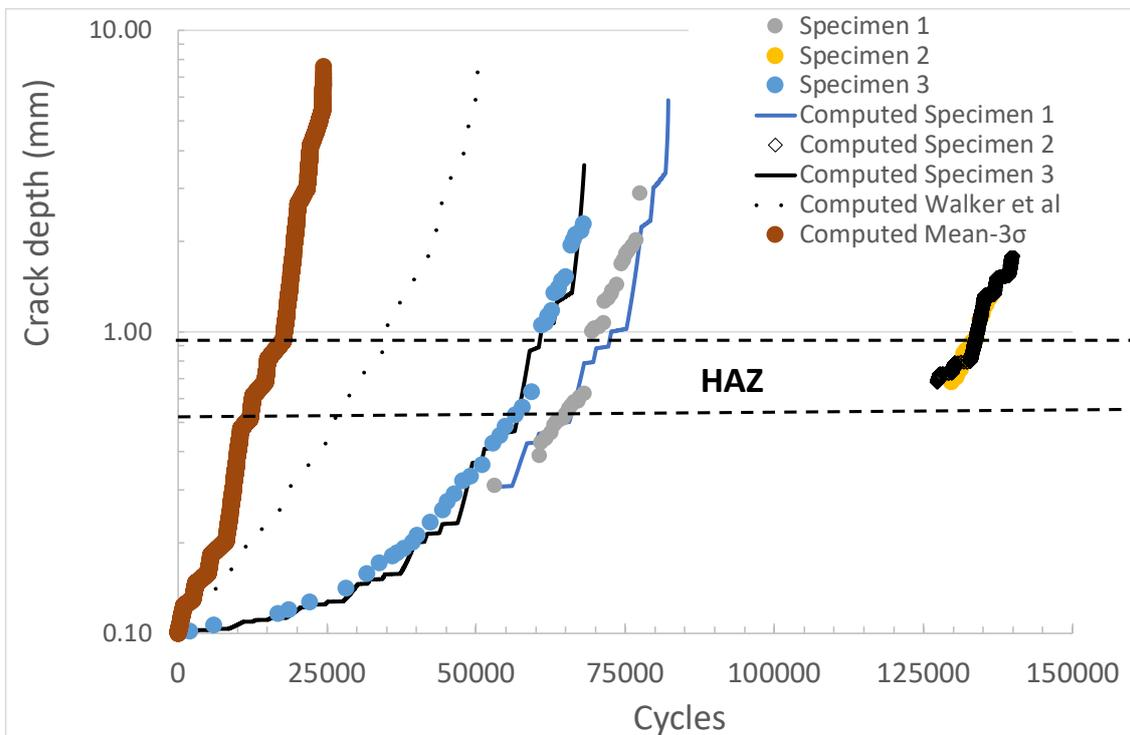
Figure 5 Durability analysis results for the LAD repairs to AerMet100 steel
