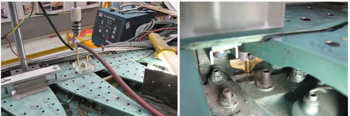
Figure 1 EDM setup (left) and a local view of the electrode and induced damage at a fastener hole (right).
