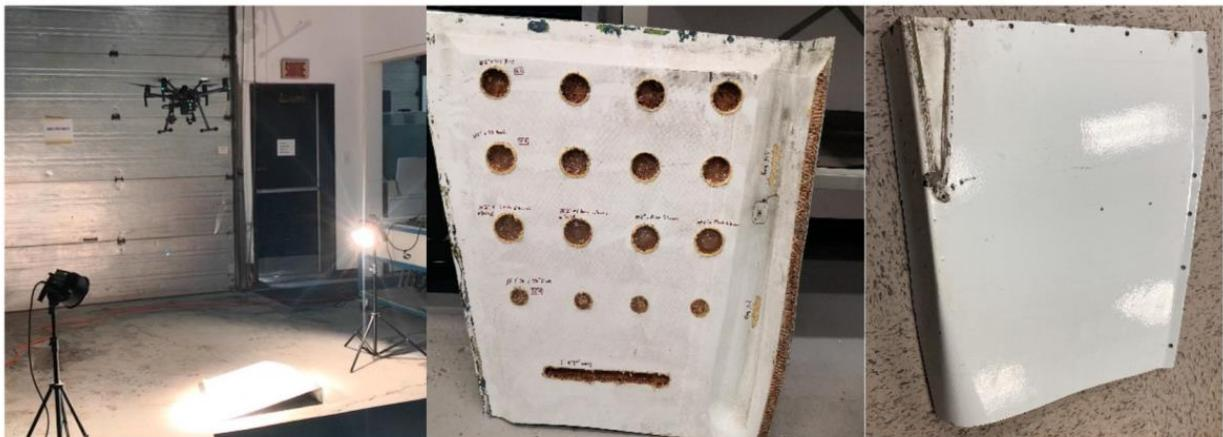
**Figure 36** Experimental setup (left), underside defects (middle), non-defective side (right).
