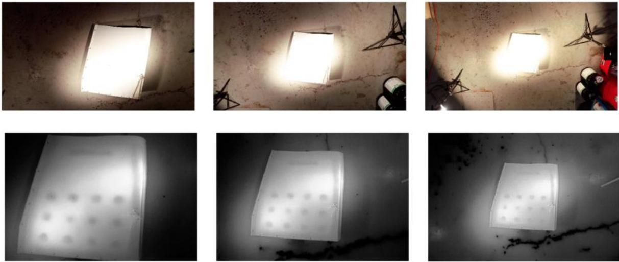
**Figure 37** Frames extracted from optical video (top) and corresponding thermal video (bottom) at increasing drone heights of 1.5 m, 2 m, and 3 m (from left to right, respectively) during active thermography inspection experiment.
