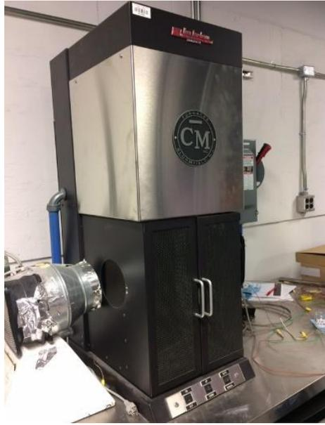
**Figure 41 CM cyclic oxidation furnace test for evaluating thermal barrier coatings durability and performance.**
