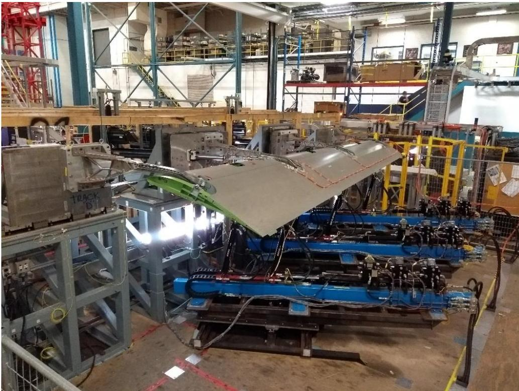
**Figure 6 Outboard flap test rig**
