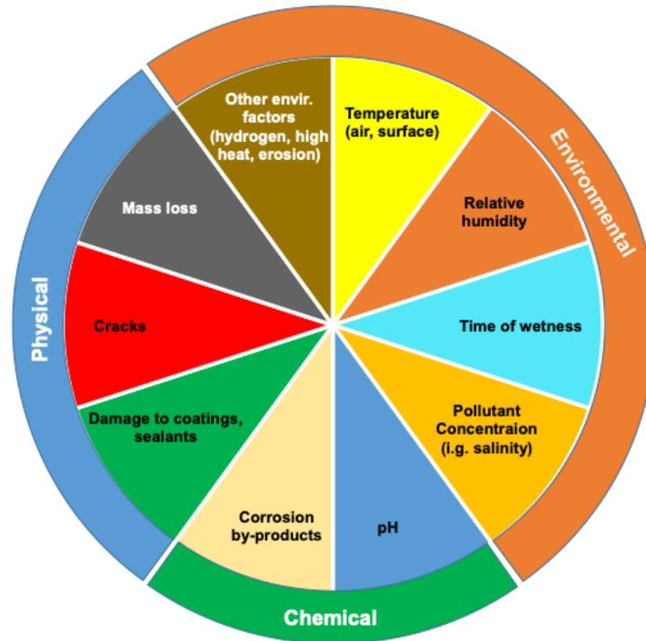
**Figure 39 Corrosion matrix of physical, chemical and environmental factors.**
