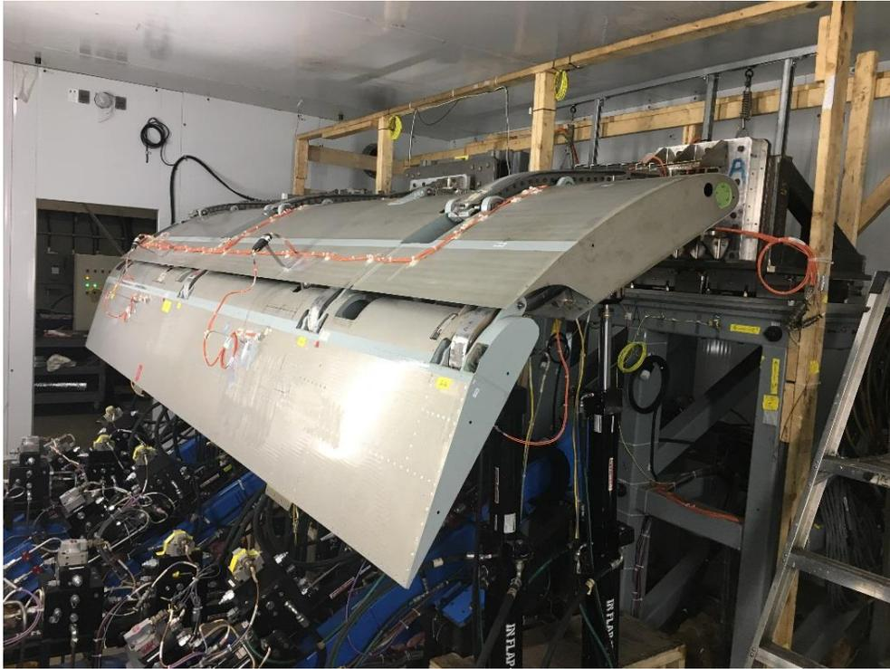
**Figure 5 Inboard flap test rig**
