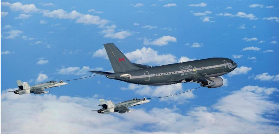
Figure 19 CC-150 Polaris in tanker configuration ([Photo Detail - IS2012-2003-150 Canadian Forces Imagery Gallery](#))
