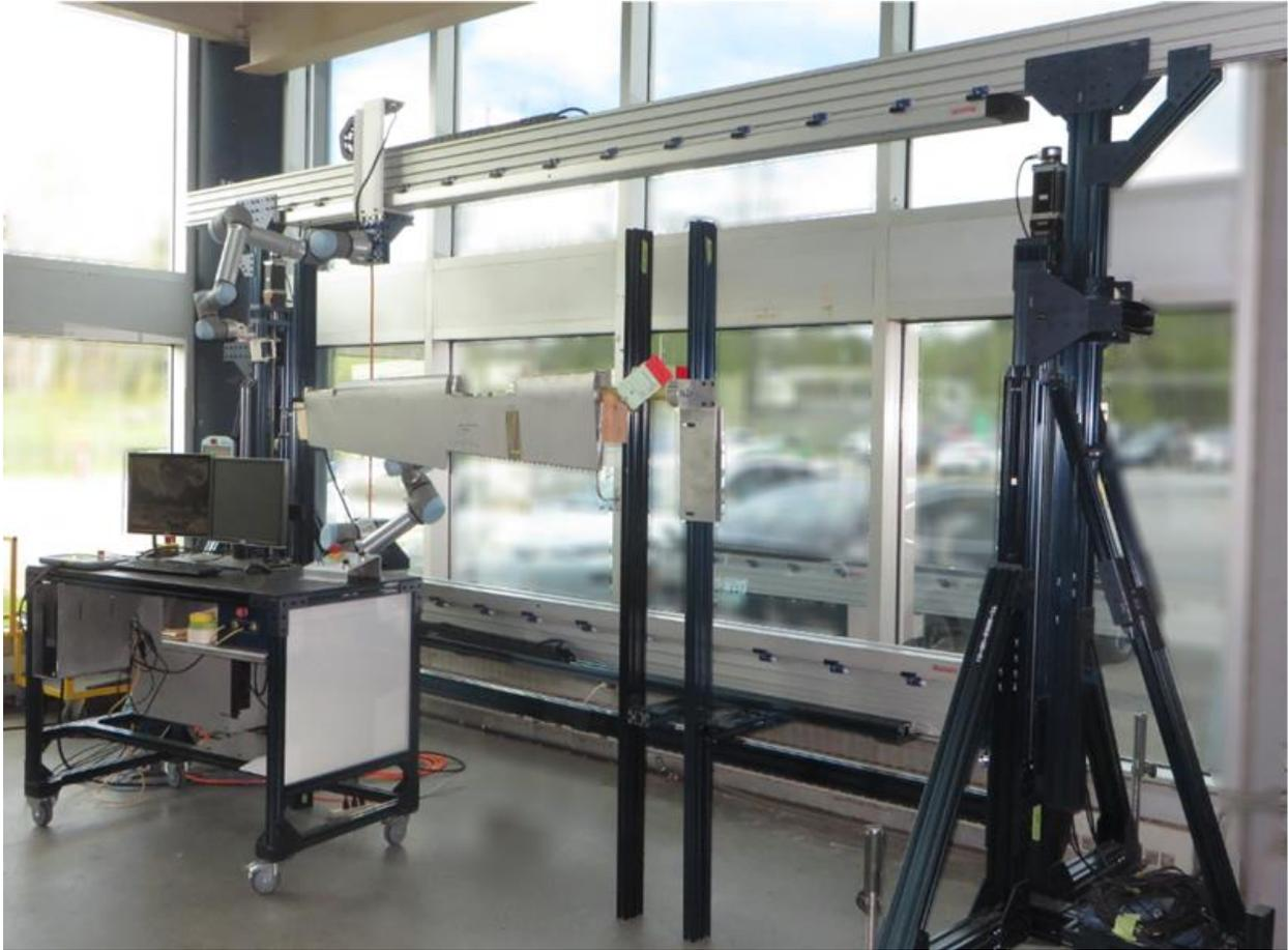
**Figure 33 Robotized Component Inspection**
