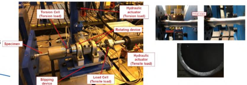
Figure 4 : Fatigue Initiation Parameters Investigation
