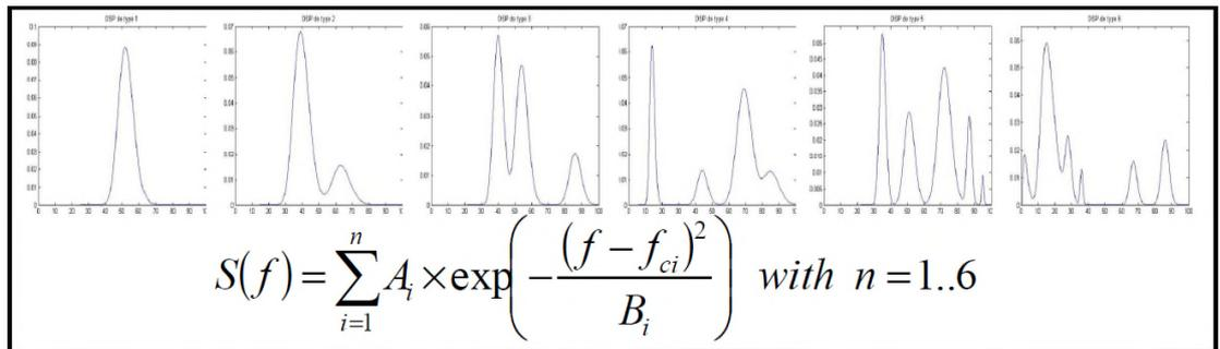
For each one, many corresponding temporal signal were also generated then the damage was calculated for each signal by “classical” method (Rainflow counting and Miner’s rule were used). The average of all these calculations (for each power spectral density) was the reference. The damage was also calculated directly from the power spectral densities with the different previous models. A comparison of the results led to assess their accuracy, scattering and conservatism.
