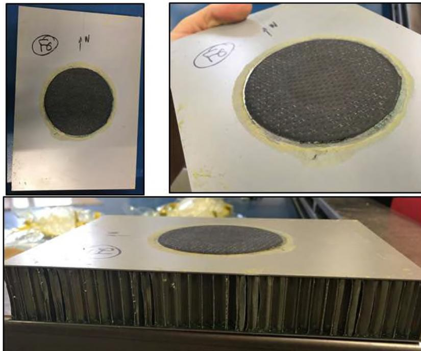
*Composite repair on a coupon*
