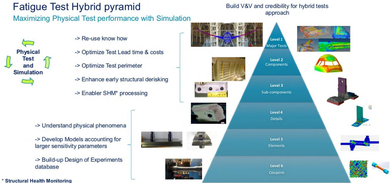
Figure 1: Hybrid Test Pyramid
