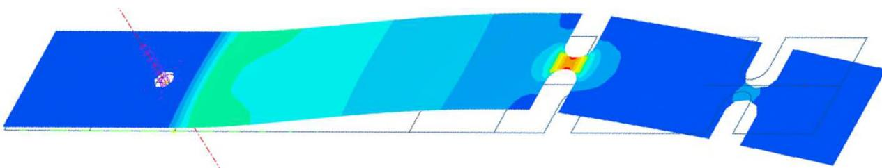
This optimization and the random excitation definition were made thanks to finite elements modelling (FEM) of the coupons and damage calculations with the different previous models.
