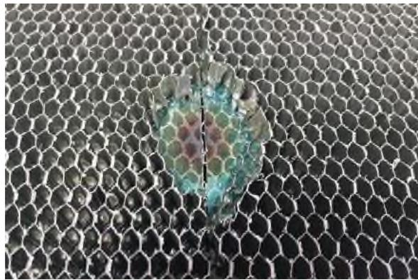
*Post mortem control of the heating method on a coupon*
