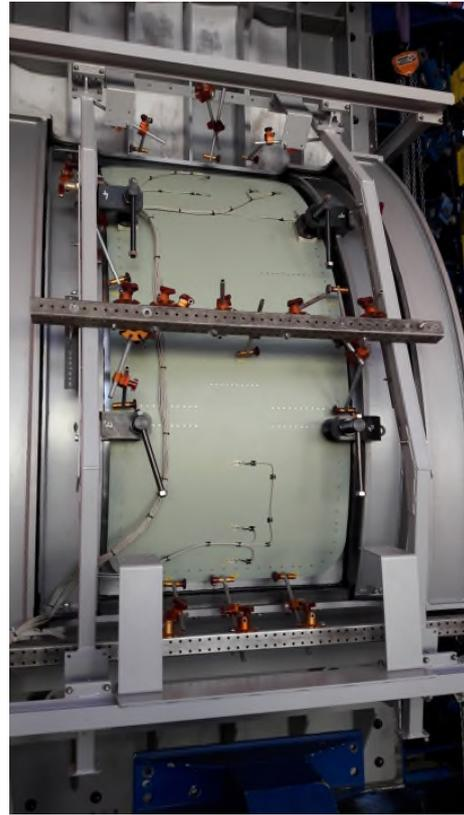
*Test rig and test specimen in test installation for a 3D positioning check*
