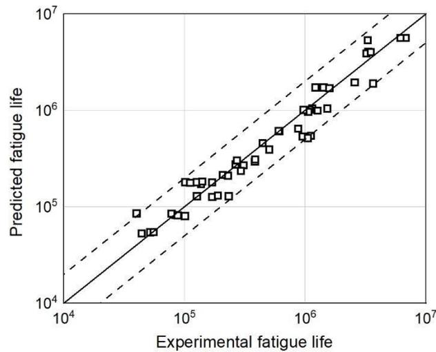
Figure 4: Comparison between predicted fatigue life from the proposed model and experimental fatigue life obtained from one of the materials investigated. Only internal defect configurations are reported here
