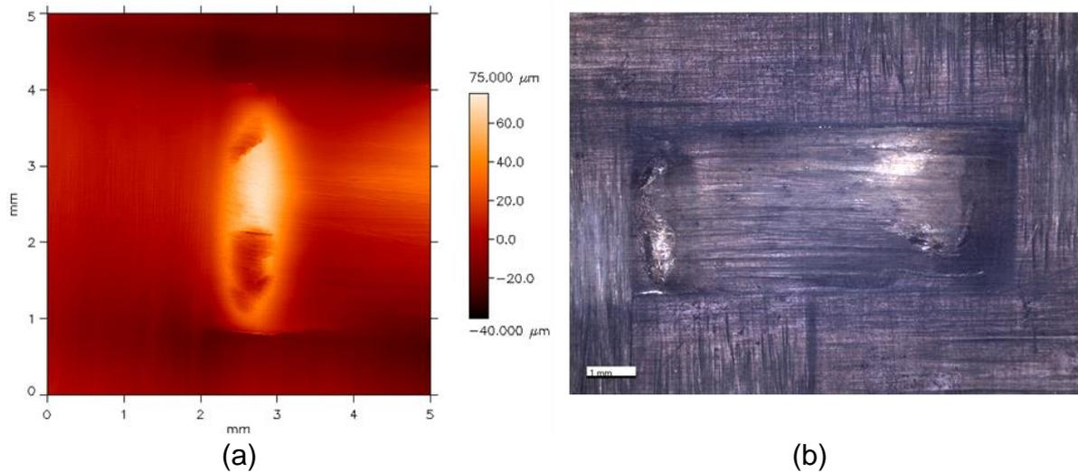
Figure 9: Topographic diagram by white light interferometry (a) and macroscopic photograph (b) of a localized instability
