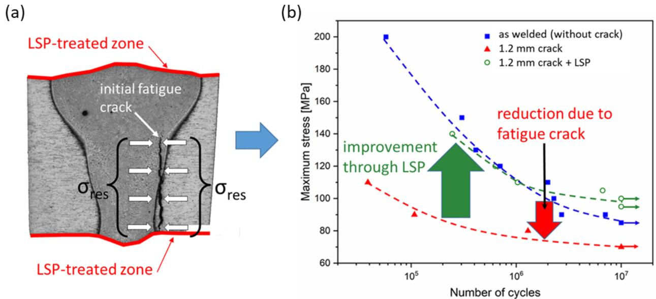
Figure 7: (a) Schematic of the specimen with an initial surface fatigue crack and (b) fatigue test results of laser beam welded specimens, laser beam welded specimens with the fatigue crack and laser beam welded specimens with the fatigue crack after LSP-treatment.
