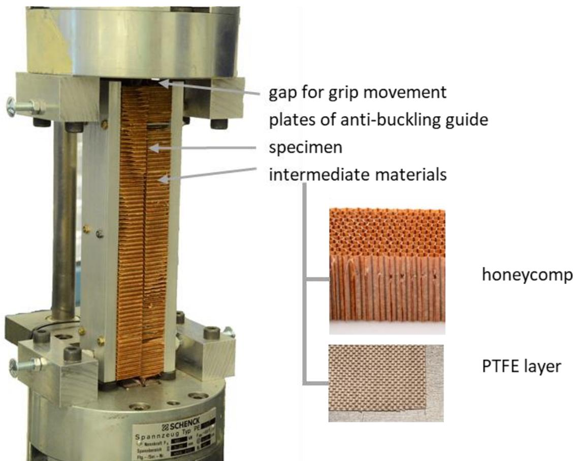
Figure 8: Test set-up with anti-buckling device and examples for intermediate materials
