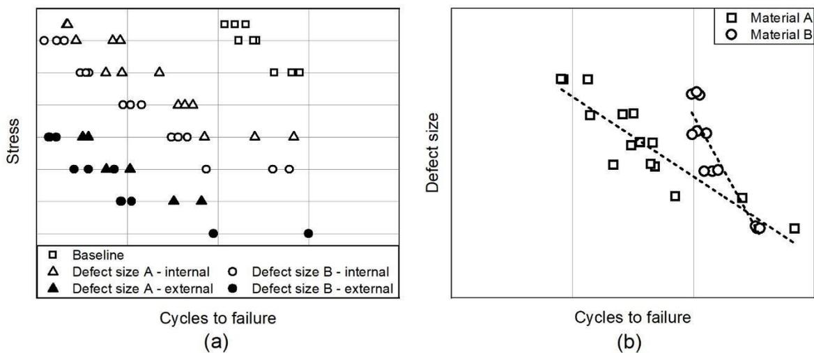
Figure 3: (a) Experimental fatigue results with a focus on the difference between internal and external defects for similar size; (b) Influence of internal defect size identified by fractographic analysis on the cycles to failure for a given stress level
