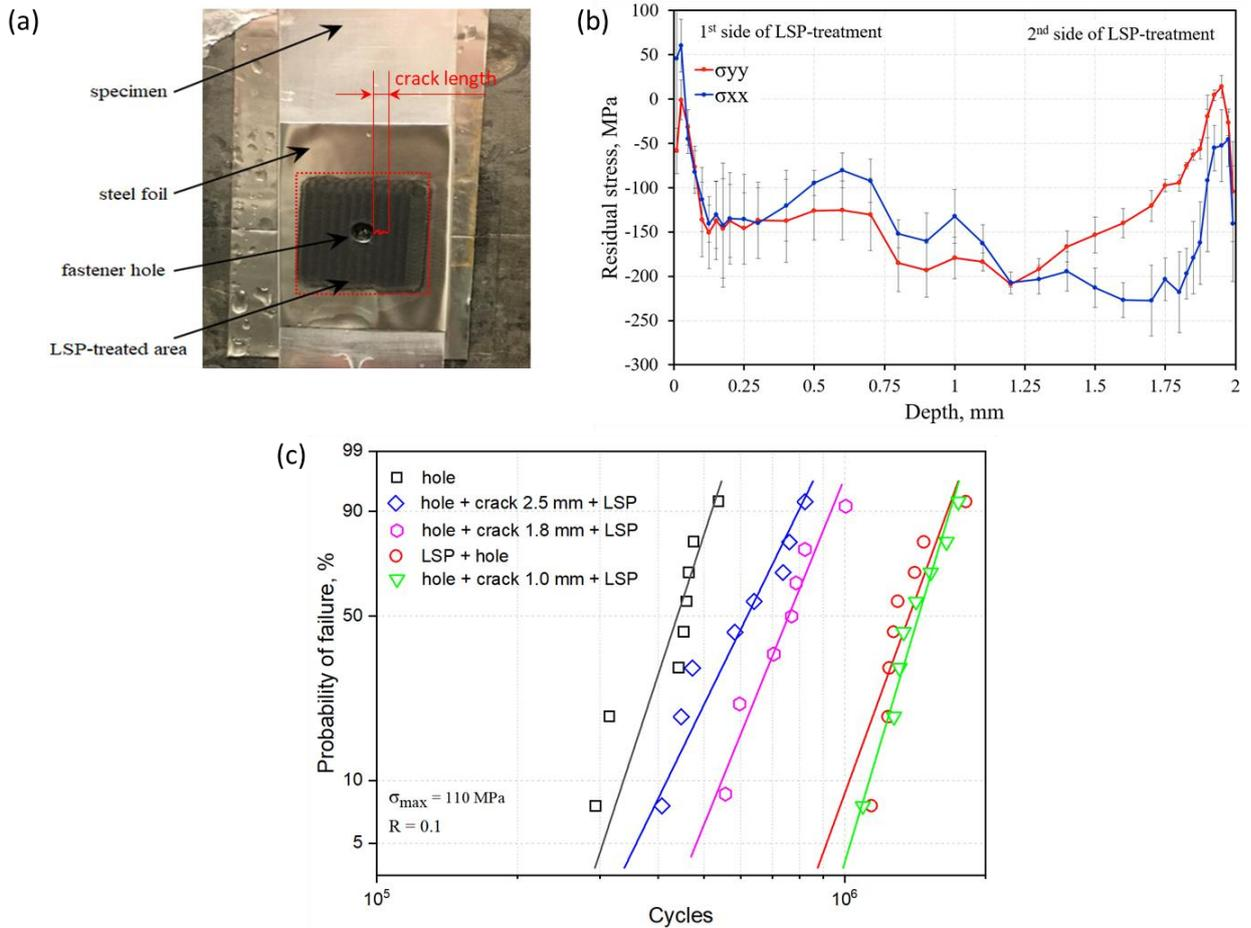
Figure 6: (a) AA2024-T3 specimen with a fastener hole after LSP, (b) depth resolved residual stress profile in LSP-treated specimen and (c) fatigue test results of the base material specimens (hole), the specimens with initial crack and LSP (hole + crack + LSP), the specimens only with LSP (hole + LSP).
