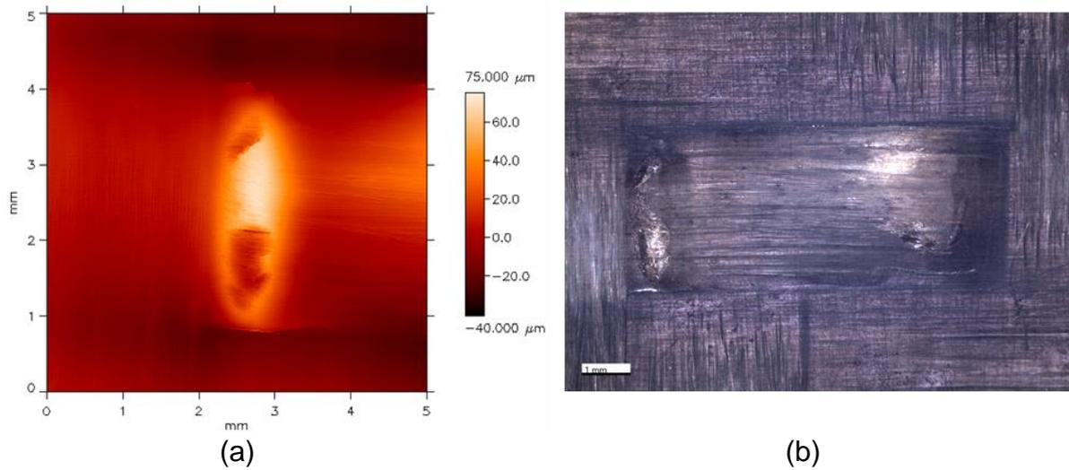
Figure 9: Topographic diagram by white light interferometry (a) and macroscopic photograph (b) of a localized instability
