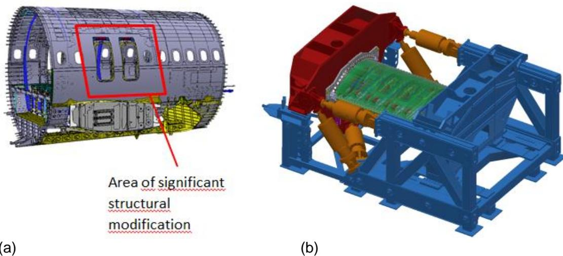
Figure 1: (a) Location of structural modification in center fuselage; (b) F&DT test rig with panel set-up
