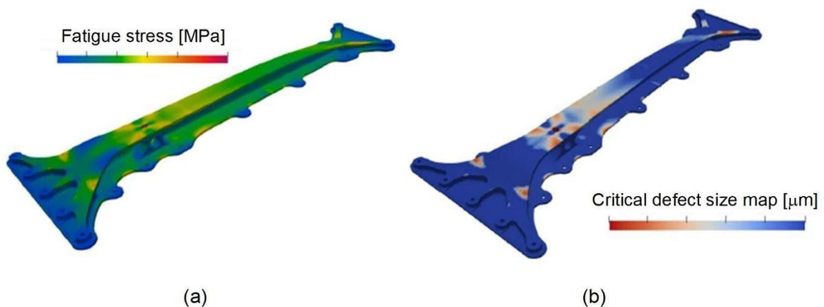
Figure 5: Example of critical defect size map as a function of stress and target life
