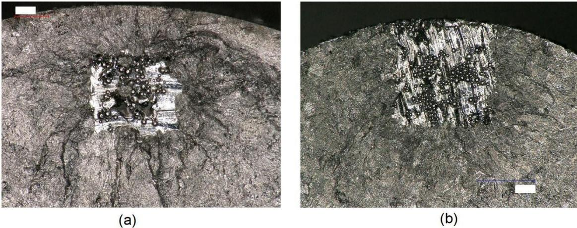
Figure 2: Fracture surface of two fatigue coupons made of the same material with a focus on the two defect position configurations: internal (a) and external (b)
