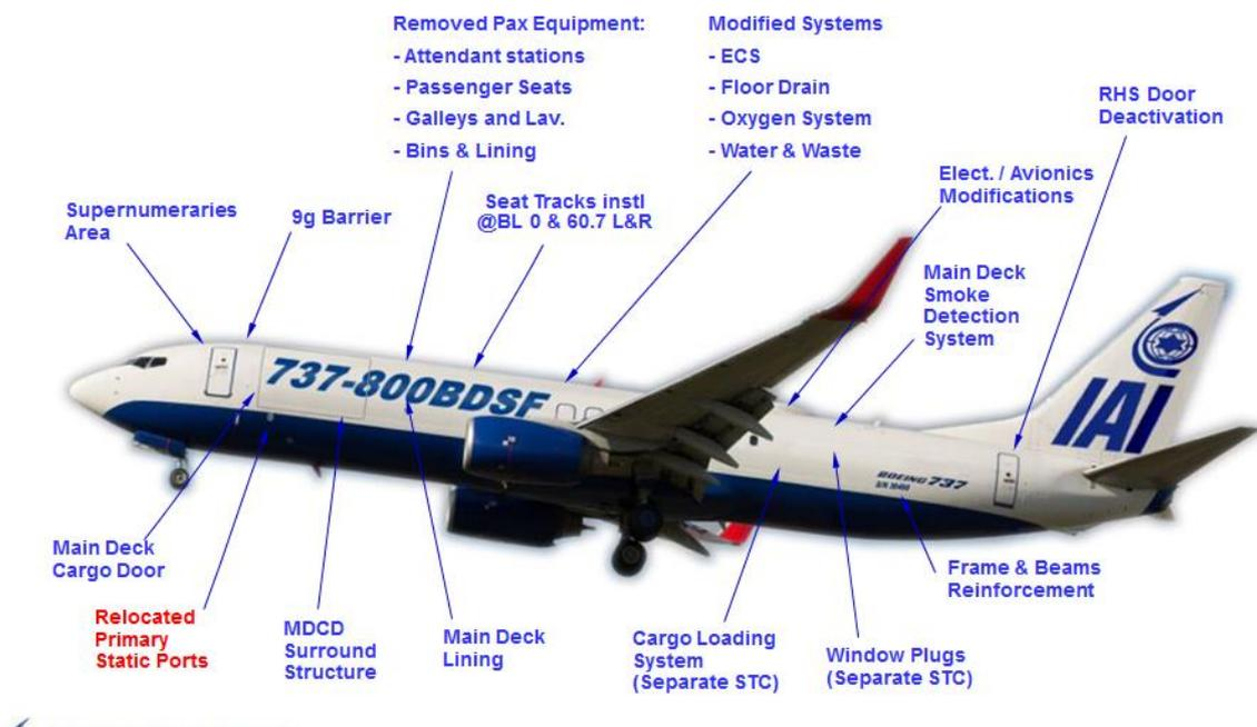
**Figure 11. Modification at the 737-800BDSF aircraft**
