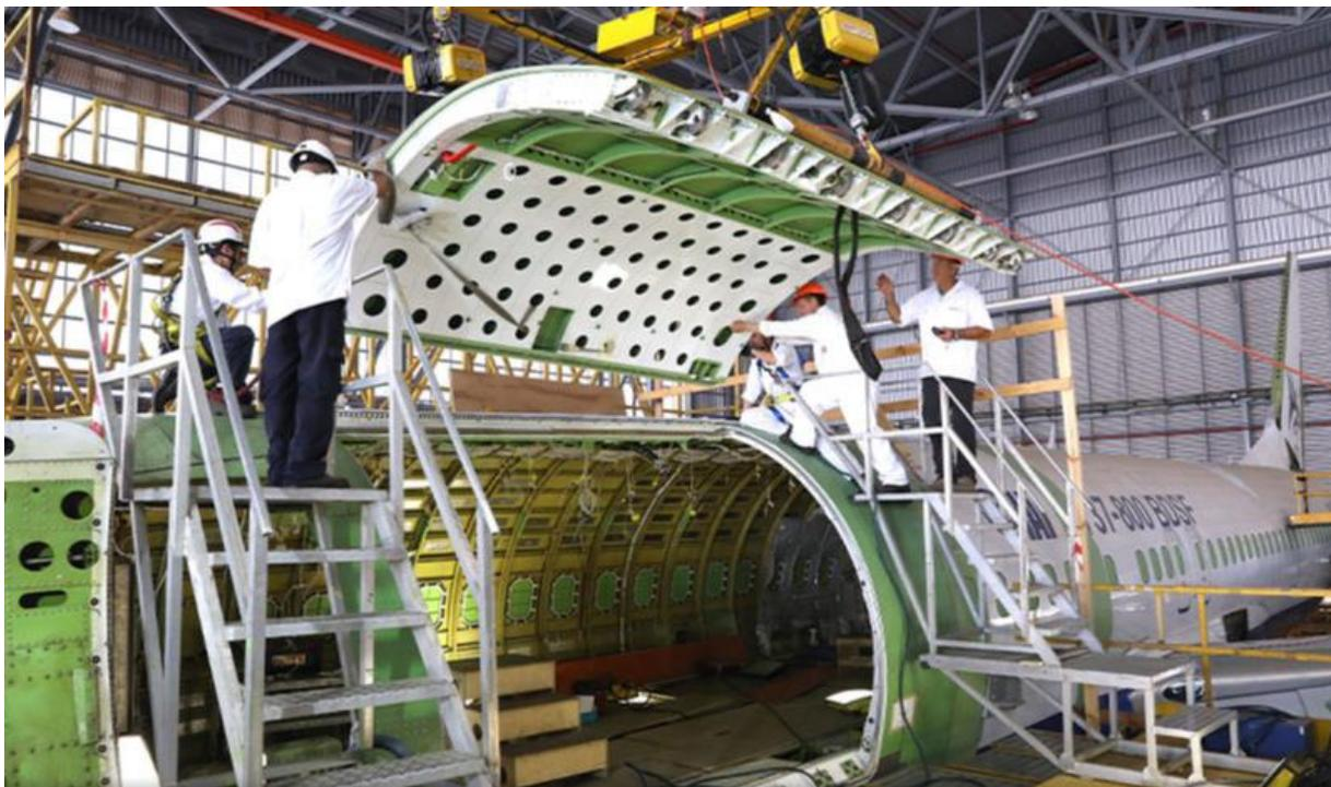
**Figure 12. Converted 737-800BDSF aircraft at the conversion line**
