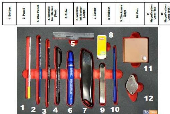
Fig. 37 – Content of the Detailed Visual Inspection toolbox.
