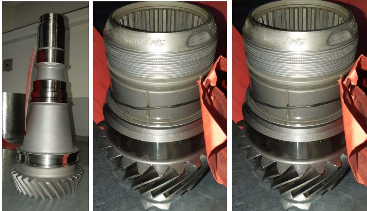
AW139 TR TakeOff Pinion      AW169 Pinion, 2<sup>nd</sup> stage, RH      AW609 Pinion, 2<sup>nd</sup> stage, RH
