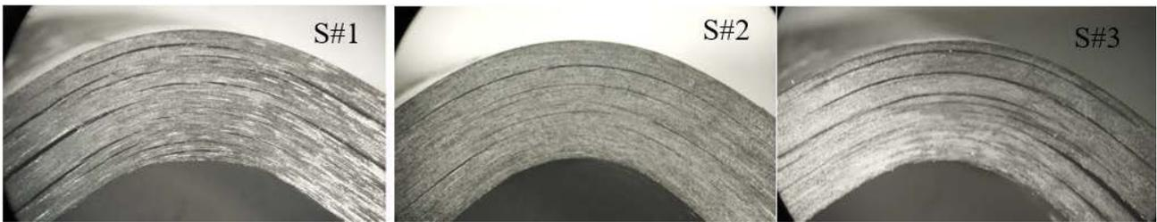
Fig. 31 - Interlaminar crack evolution for Zero specimens,  $[0]_{48}$ .
