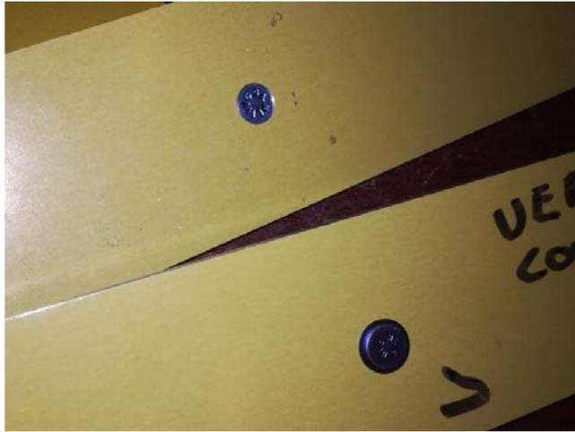
Fig. 23 - Bolted cracked lap shear specimens. Both flat and flush head Hi-Loks have been employed.
