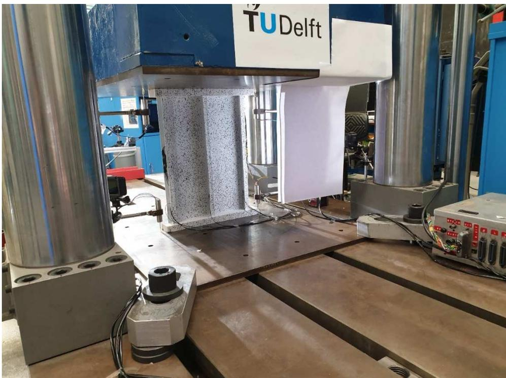
Figure 24 Test panel with a delamination in the skin – middle stringer interface representing Barely Visible Impact Damage.
