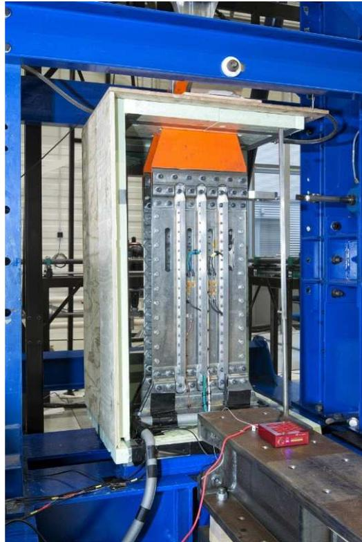
*Figure 49 SHM test bench with double stiffened aluminium panel in climate chamber with the fibre optic interrogator (Gator, small red box) from PhotonFirst. The FBGs were mounted on the back side of the panel.*
