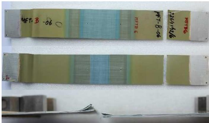
Figure 18. Failed MFT-B-06 specimen; pristine and tested in HTA for fatigue and RTA for the residual strength test: IML view (top), OML view (middle) and side view detail of the failure region (bottom).
