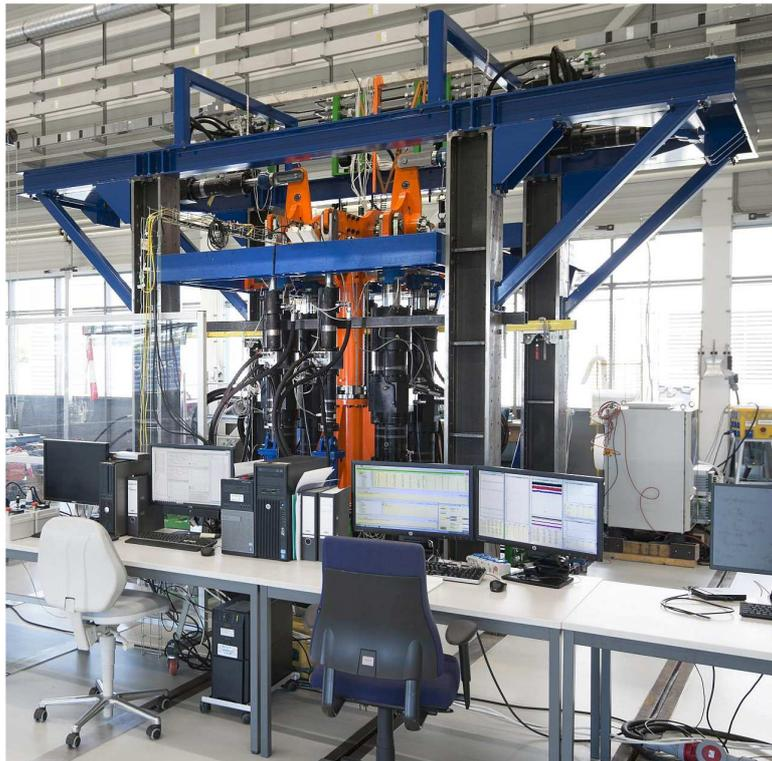
Figure 47 Landing gear health monitoring test bench at NLR.
