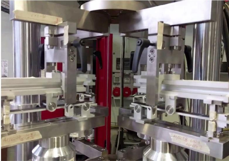
Figure 29 Multi-specimen test rig used to characterize the fatigue behaviour under mode II loading.
