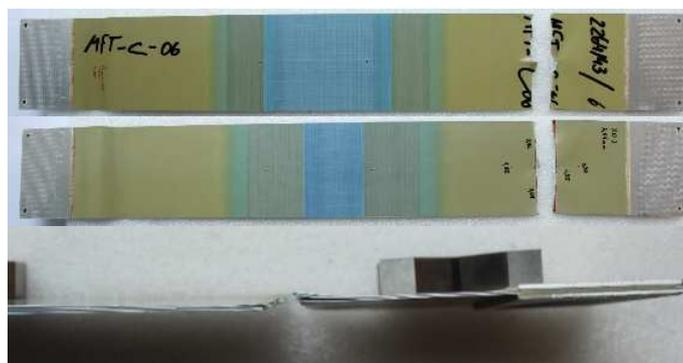
Figure 19. Failed MFT-C-06 specimen; impacted (20J) and tested in RTA: IML view (top), OML view (middle) and side view detail of the failure region (bottom).
