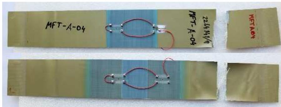
Figure 17. Failed MFT-A-04 specimen with intact crack wires positioned at 1mm from the hole edge.
