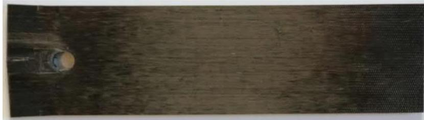
**a) Bearing failure Lam ID 3, 100% UD**
