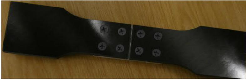
Figure 3.1.5. Hybrid coupon specimen.
