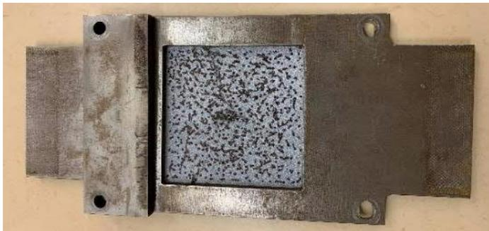
Figure 3.3-3. Specimen mounted in the support device.
