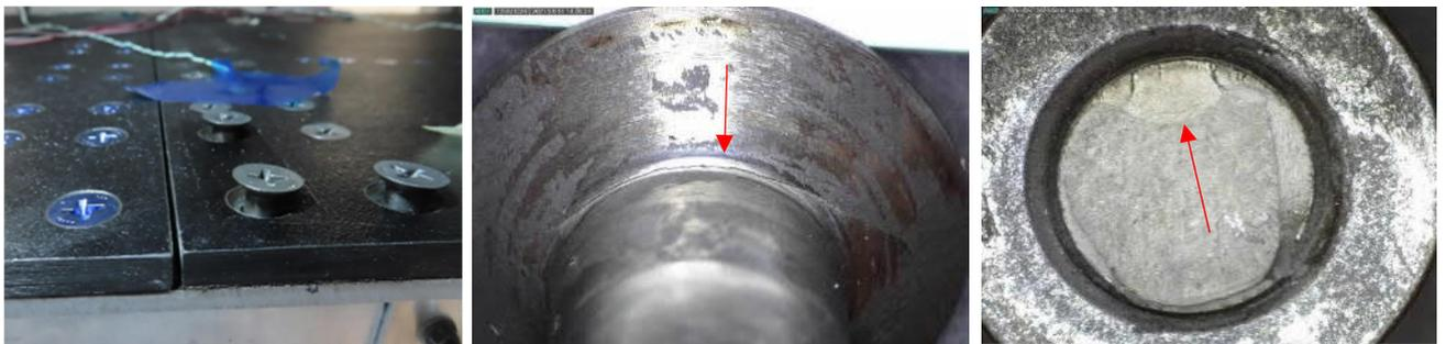
Figure 3.1-4. Three failed bolts in the main joint (left), fatigue crack under bolt the head (middle) and fatigue crack in the bolt thread (right).
