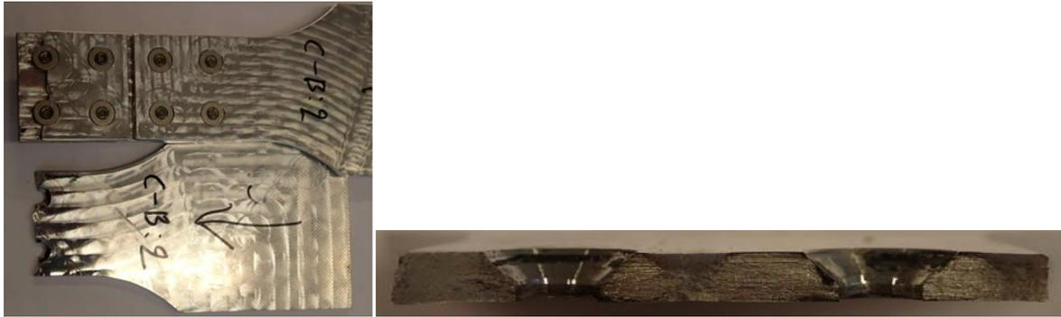
Figure 2.2-7. Failure mode I in C-B specimen.
