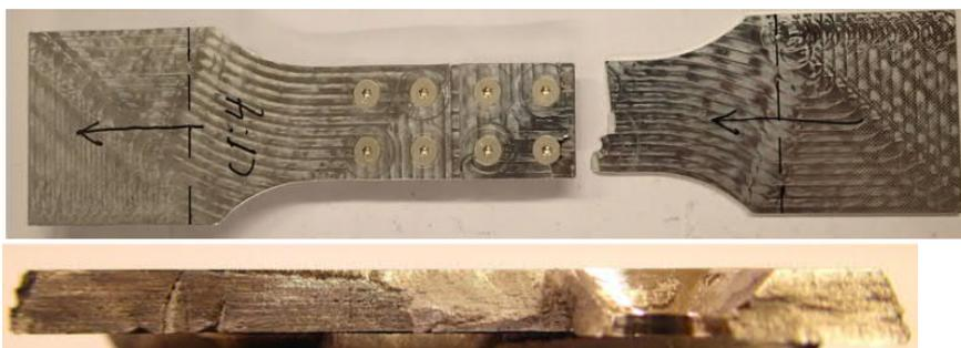
Figure 2.2-6. Failure mode I\* in C specimen.
