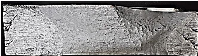
Figure 4. 21: CAA sample, fracture surface after fatigue testing with many initiation origins at etch pits
