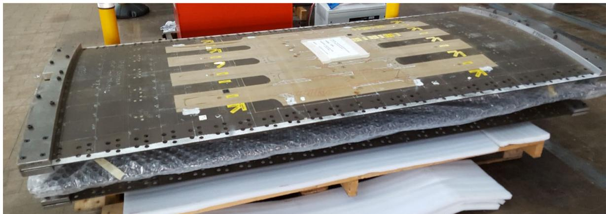
Figure 4. 30: Second test specimen: Fuselage composite panels from an A-350 static test
