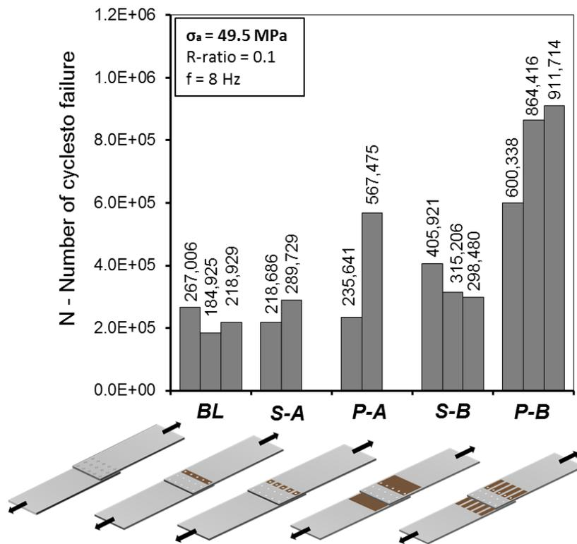
Figure 2: Histogram of the fatigue lives of peened and unpeened joints. The peening pattern corresponding to each group of histogram bars are shown below the chart.
