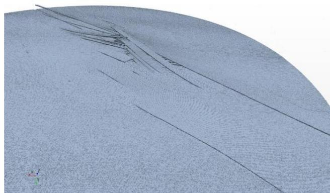
Figure 1: A 3D reconstruction of a damage composite specimen from X-CT data.
