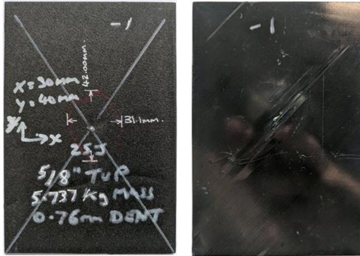
Figure 2: Composite specimen (provided by QUB), left – front, right – back
