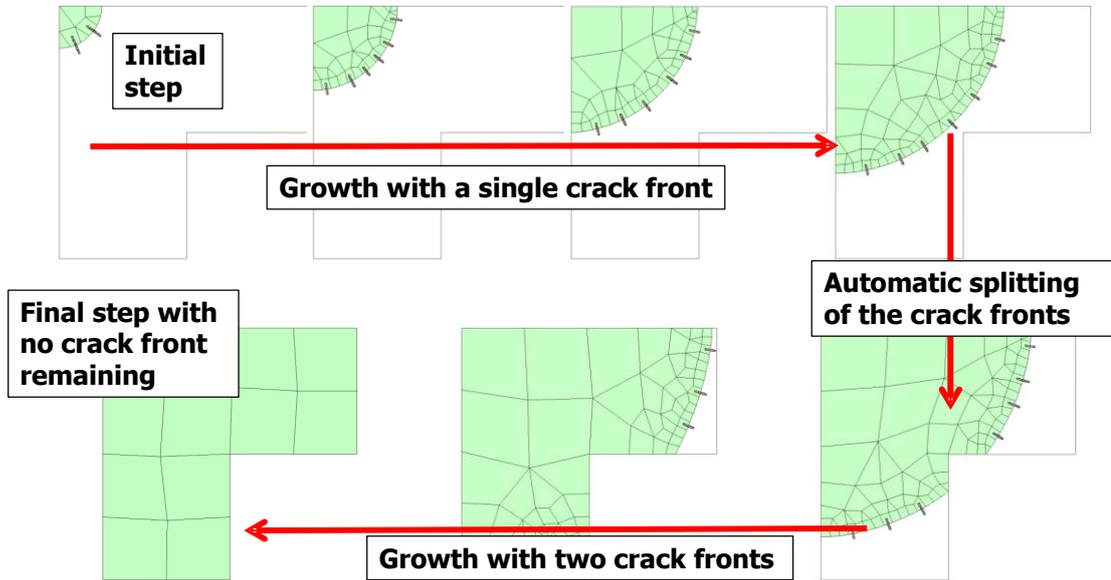
Figure 2: Automatic splitting of a corner crack
