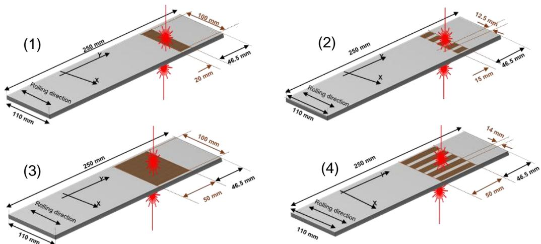
Figure 1: Peening patterns applied to bolted lap joint elements prior to assembly.
