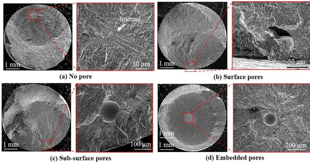
Fig. 3: SEM images of fracture surfaces (left) and crack initiation location of the corresponding sample in higher magnification (right).
