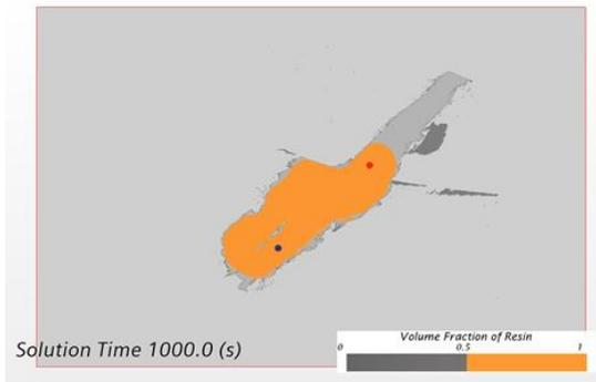
Figure 5: Reduced-order method simulation result of one of the cases, red and blue dots indicate injection port and outlet vent respectively.
