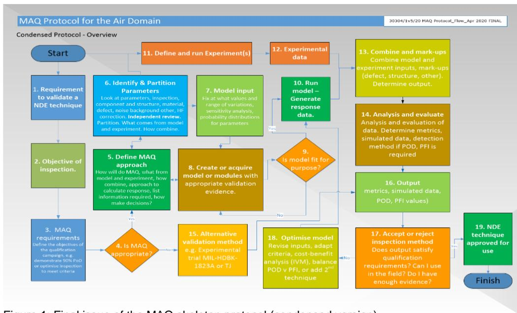
Figure 1: Final issue of the MAQ skeleton protocol (condensed version)
