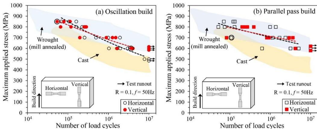
Fig. 2: S-N data for the oscillation and parallel pass builds and best fitted lines. Encircled data points indicate crack initiation from a surface pore. Their wrought [2] and cast [2] counterparts are also shown.
