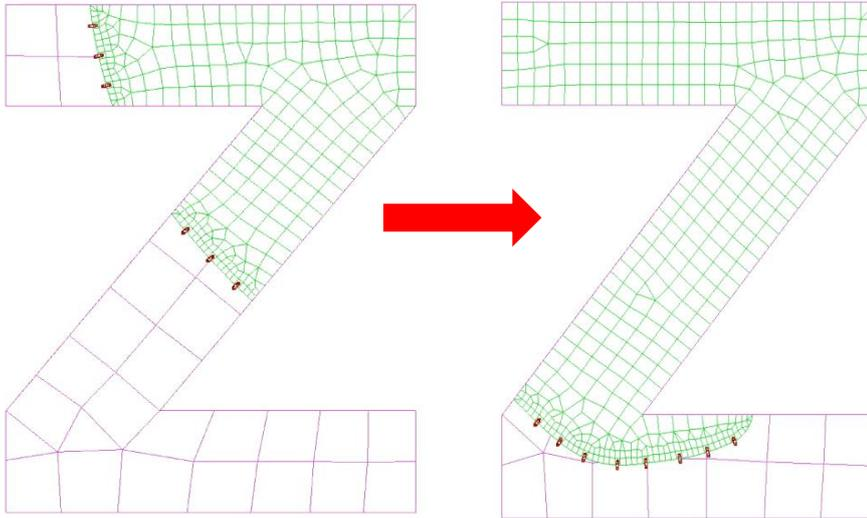
Figure 5: Corner crack through a "Z" specimen
