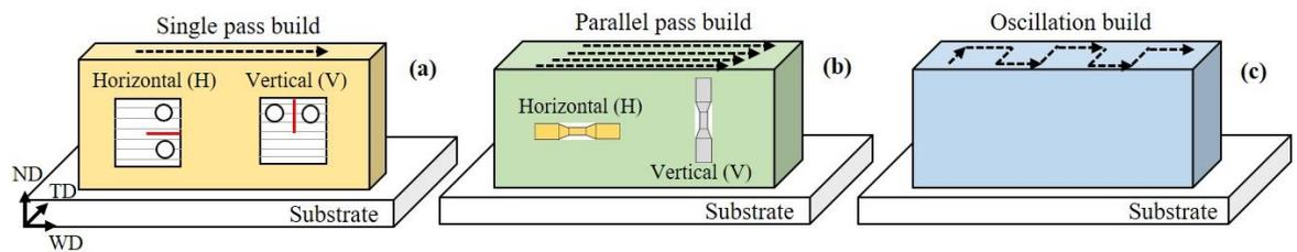
Fig. 1: Schematic of WAAM Ti64 walls (a) single pass, (b) parallel pass, (c) oscillation deposition strategies. WD: welding heat source travel direction, TD: transverse direction, ND: normal direction. Extracted test samples for fatigue crack growth and HCF are also shown.
