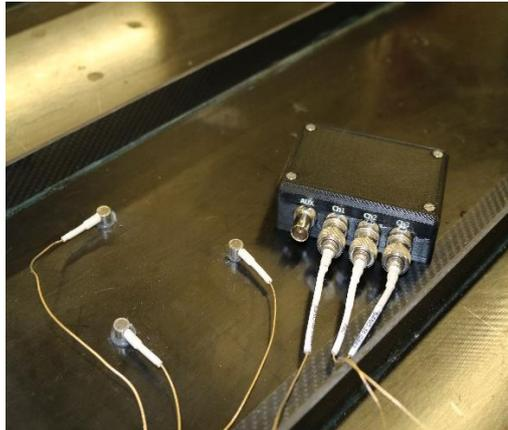
Figure 1: Wireless sensor and PZT's on composite panel
