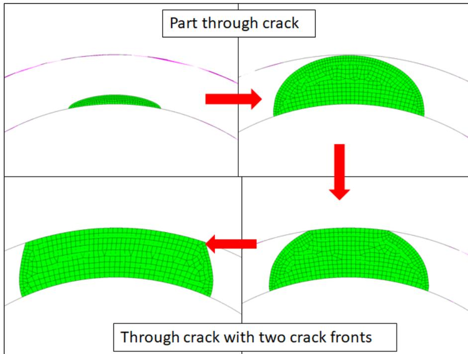
Figure 3: Inner crack breaking through a thin walled pipe
