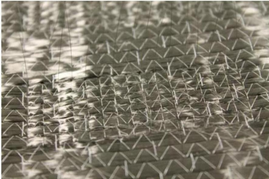
Figure 1 - A close-up of the SMA tufted composite.
