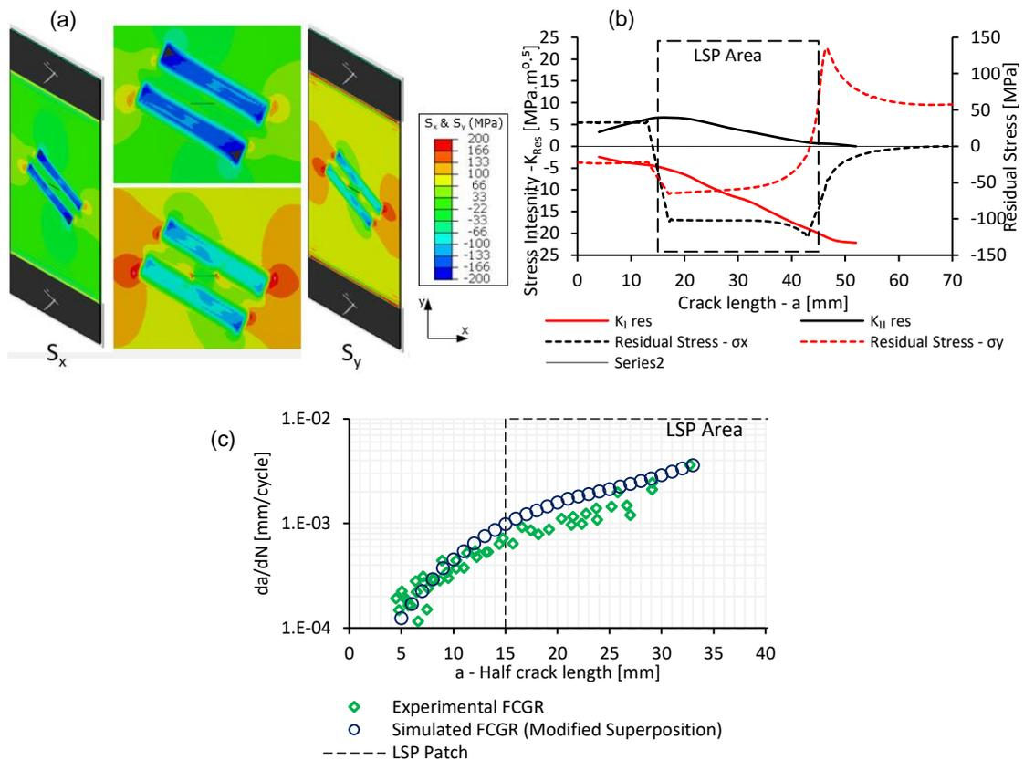
Figure 3: (a) finite element analysis of a crack in the presence of a laser peening induced residual stress field, (b) residual stress established  $K_{I,res}$  and  $K_{II,res}$  across the crack path of the angled laser peening samples, (c) comparison of the experimental and predicted fatigue crack growth rates
