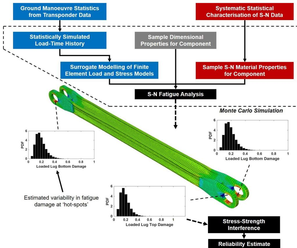
Figure 1: A flowchart overview of the probabilistic fatigue methodology applied to a landing gear component (3D model created in ABAQUS®).
