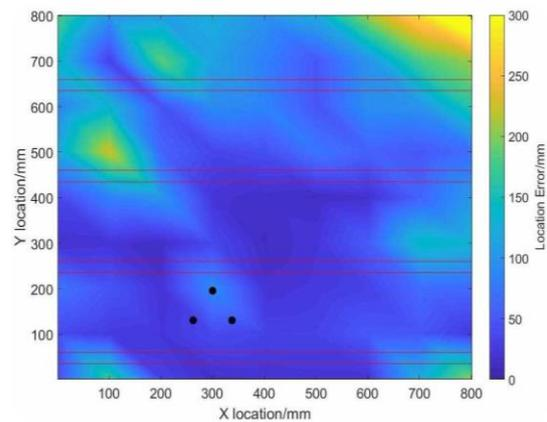
Figure 2: Absolute location error of sensor node on complex composite panel. Sensors in black, stiffeners in red.
