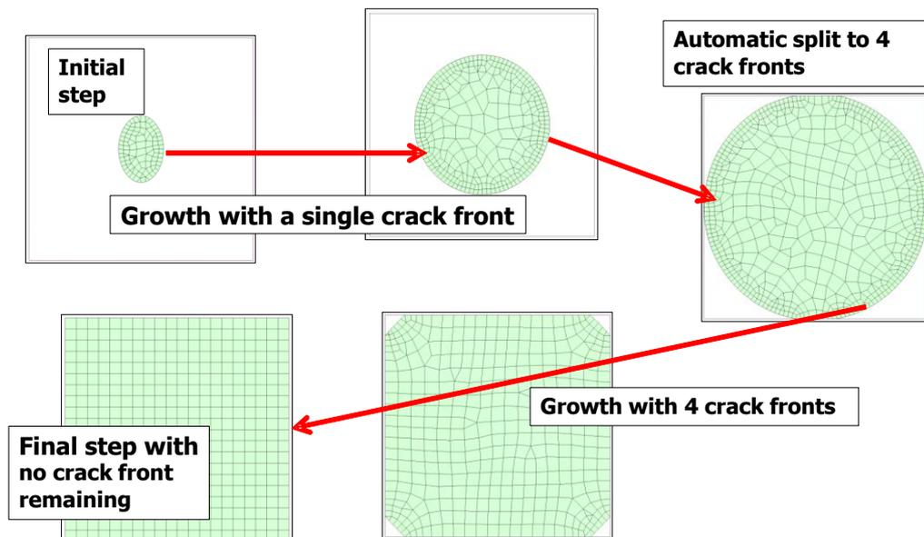
Figure 4: Automatic splitting of an embedded crack
