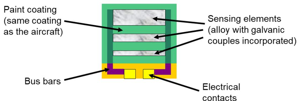
Figure 2: Smart Witness Plate Corrosion Sensor Diagram
