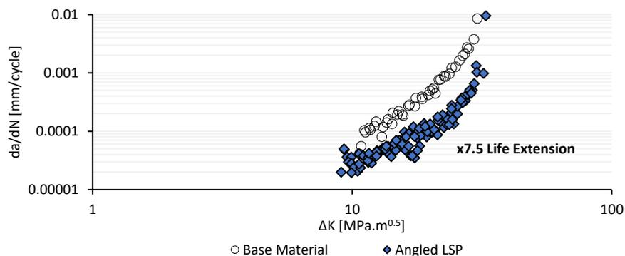
Figure 2: Effect of angled laser peened patch on fatigue crack growth rate
