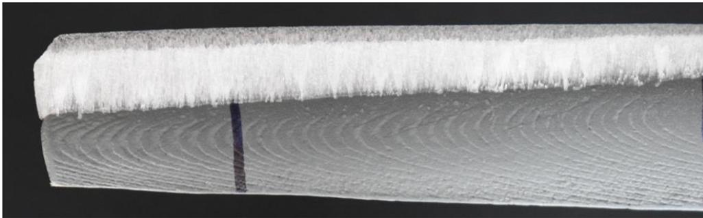
Figure 1 - Preliminary image from a blade icing experiment formed in a cloud and environmental chamber.
