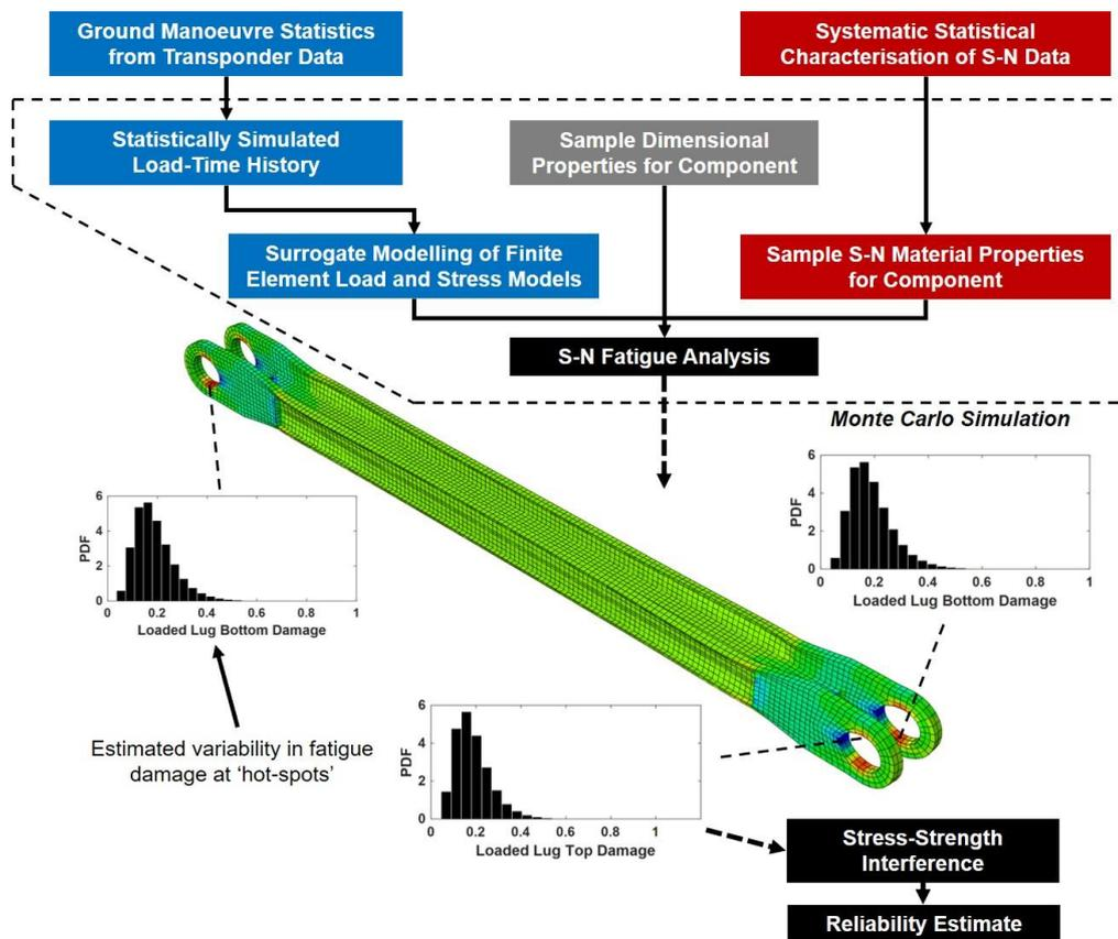
Figure 1: A flowchart overview of the probabilistic fatigue methodology applied to a landing gear component (3D model created in ABAQUS®).
