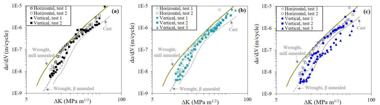
Fig. 4: Fatigue crack growth rate: (a) single pass, (b) parallel pass, (c) oscillation builds, and comparison with conventional Ti64 alloys from AMS 4992:  $\beta$  annealed cast (10 mm thick)[2],  $\beta$  annealed wrought (L-T, 10 mm thick, 1050°C 1hr, furnace cooling, stabilisation annealing 730°C 2hr, furnace cooling)[6], and mill annealed wrought plates (L-T orientation, 6.35 mm thick)[2].
