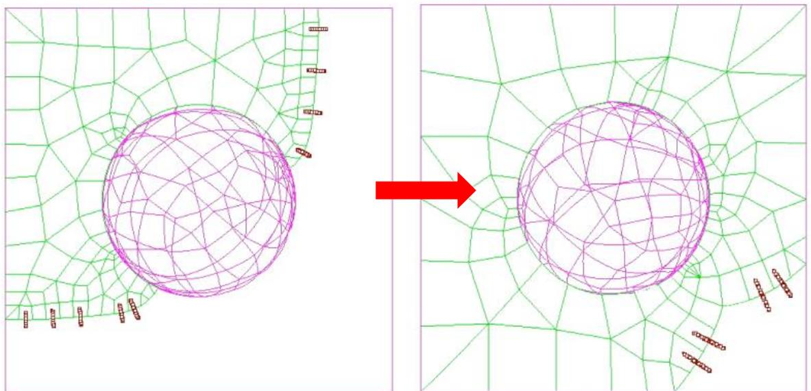
Figure 7: Corner crack split by an internal cavity
