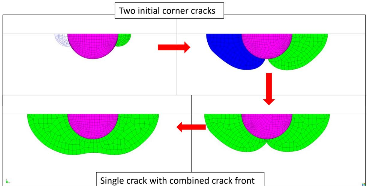
Figure 6: Coplanar cracks automatically joining
