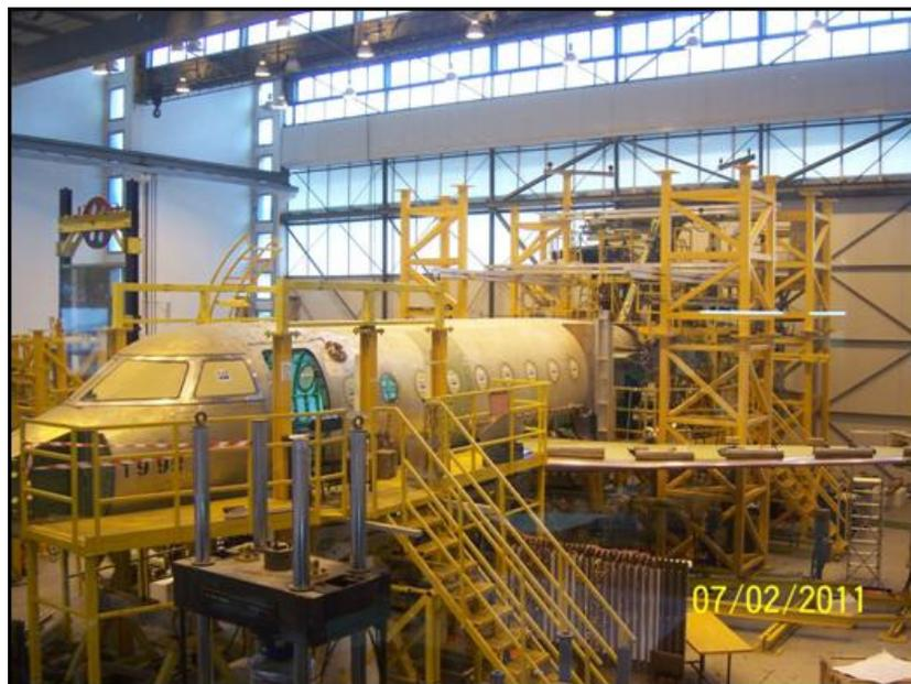
Figure 5: Complete G280 Airframe Mounted in its Fixture and Ready for Fatigue Testing
