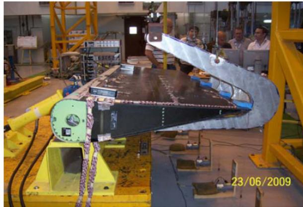
**Figure 7: The G280 Rudder in its Test Fixture**
