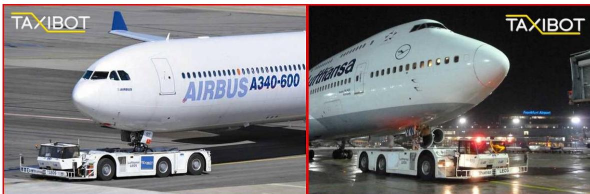
**Figure 28: Airbus A340-600 and Boeing B747-400 towed by TaxiBot**
