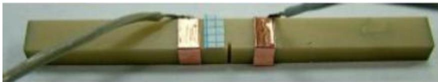
Figure 32: Four-point bend specimen with copper electrodes attached.
