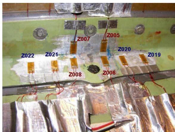
**Figure 4: An example of strain gage instrumentation of the RHS drag angle**
