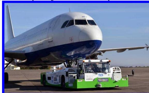
**Figure 29: TaxiBot NB prototype towing the Airbus A320-200**
