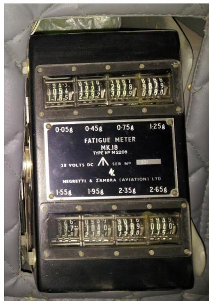
Fig. 11 - Typical fatigue meter, used on the G222 I.A.F. fleet.
