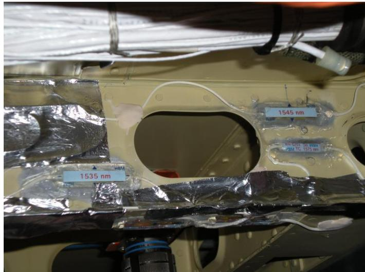
**Fig. 7 - FOBG instrumentation of a AW109SP prototype baggage door for evaluating the sensor system.**
