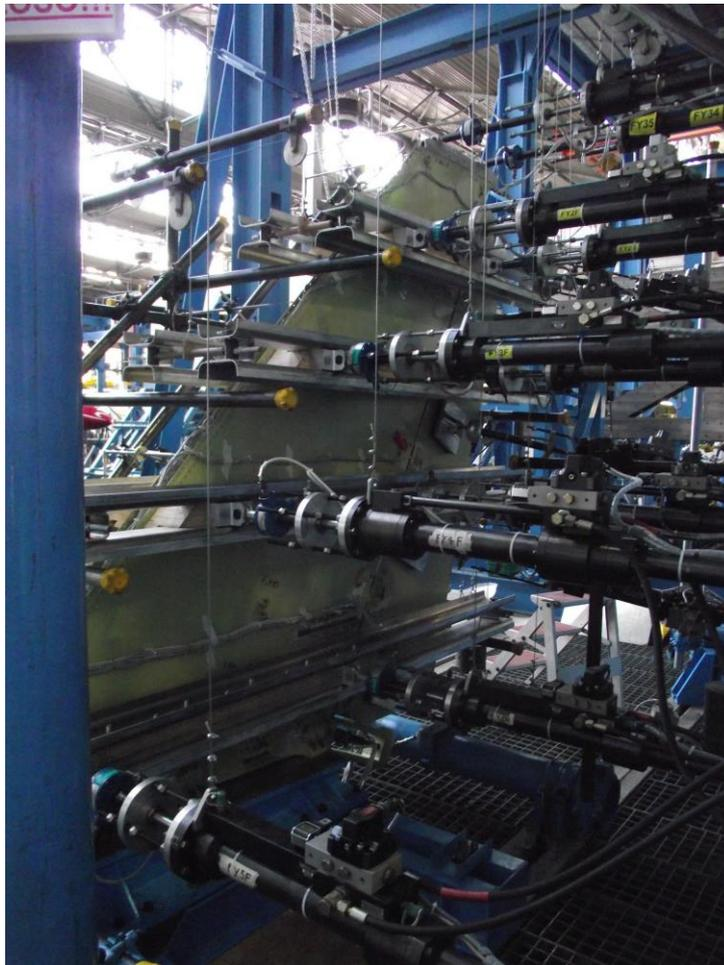
**Fig. 34 - Picture of the M-346 VT fatigue test set-up.**
