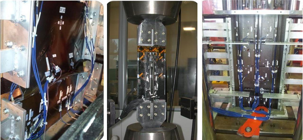
Fig. 38 - C-Series Bombardier program: example of element and sub-component tests.
