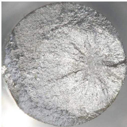
Fig. 17 - Fracture surface of a failed Inconel 718 specimen. (Specimen: C1, Long.; T=400 °C; R=-1; S<sub>max</sub>=600 MPa; N=1921800).
