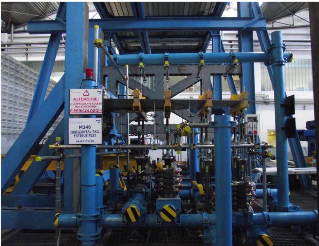
Fig. 32 - Picture of the M-346 HT fatigue test set-up.
