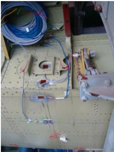
*Fig. 4. Strain gauges installed on the test specimen*
