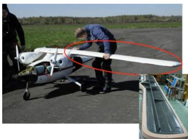
**Fig. 14. CFRP-wing structure of SAMONIT1**
