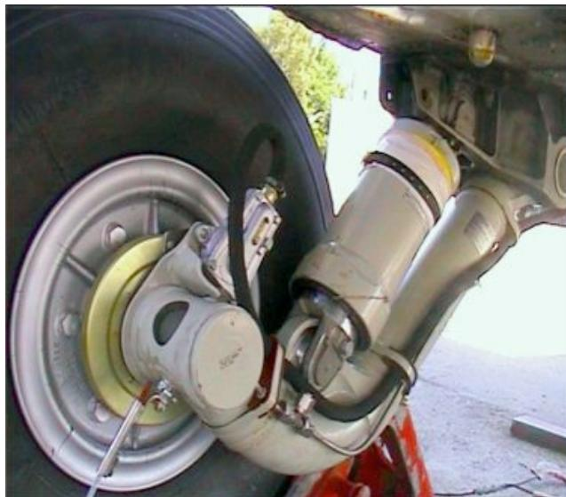
**Fig. 1. The new main landing gear of PZL M28 aircraft**
