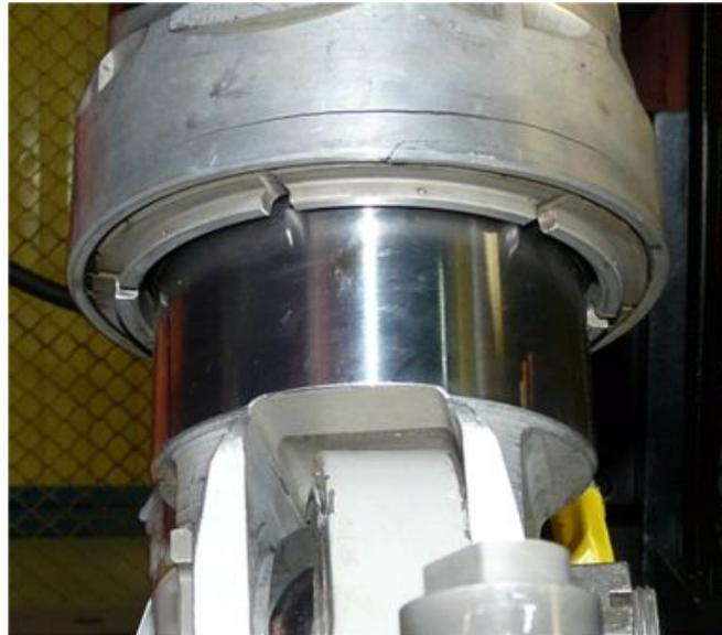
**Fig. 6. The new landing gear shock absorber with a visible crack at the bottom end of the cylinder**
