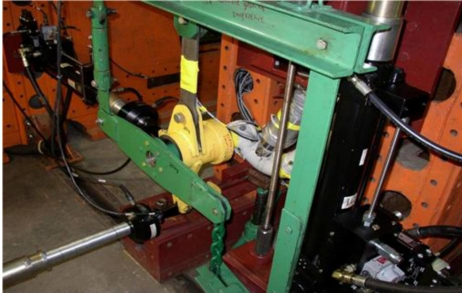
**Fig. 4. The main landing gear on a stand during fatigue testing (front-side view). The test is performed in the structural tests laboratory of Polskie Zakłady Lotnicze Sp. z o.o.. The test program was adapted from that prepared by the Institute of Aviation in Warsaw for the previous main landing gear**
