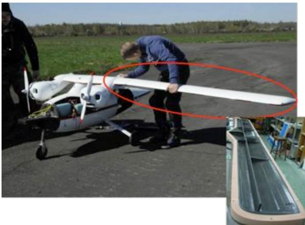
*Fig. 14. CFRP-wing structure of SAMONIT1*
