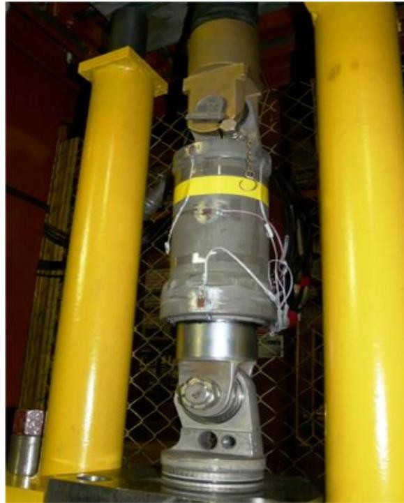
*Fig. 8. The modified shock absorber on a stand during fatigue testing*
