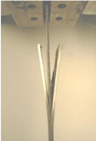
***Fig. 2. Specimen during the wedge test***
